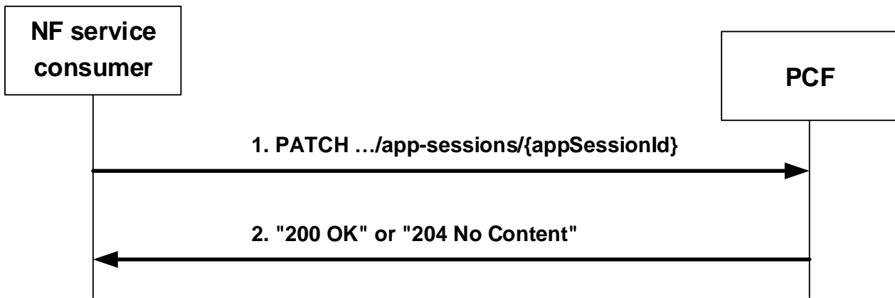
Figure 4.2.3.2-1: Modification of service information using HTTP PATCH
