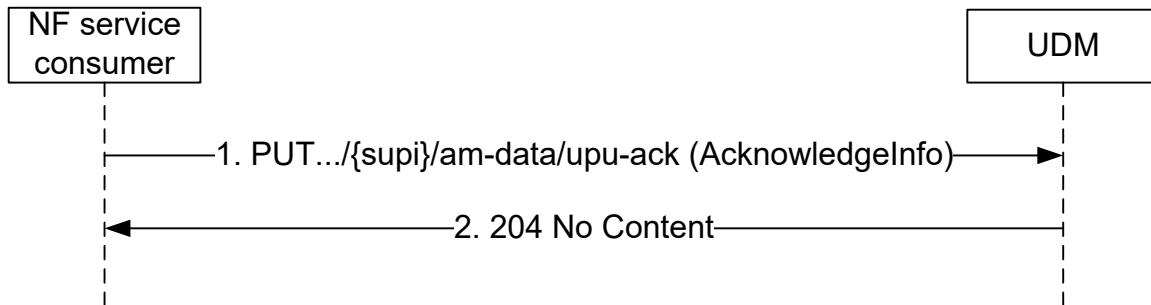
**Figure 5.2.2.6.3-1: Providing acknowledgement of UE parameters update**
