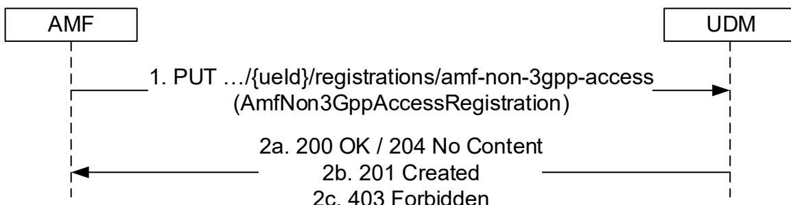
**Figure 5.3.2.2.3-1: AMF registering for non 3GPP access**
