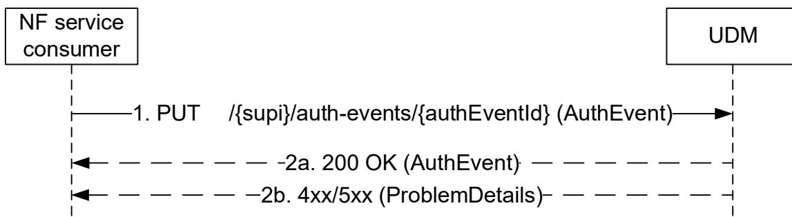
**Figure 5.4.2.3.3-1: NF service consumer removes the authentication result**
