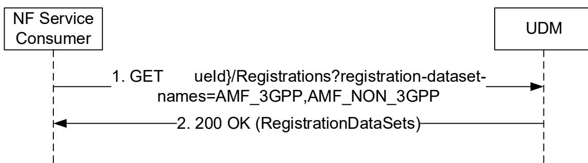
**Figure 5.3.2.5.10-1: Retrieval of Multiple UE Registration Data Sets**
