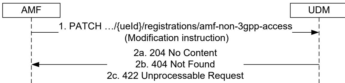
**Figure 5.3.2.6.3-1: AMF registration parameter update for non-3GPP access**
