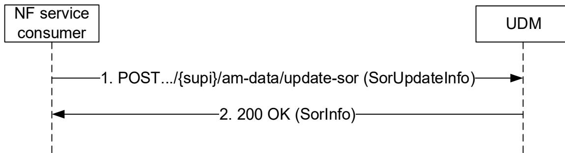
**Figure 5.2.2.6.6-1: Triggering update of Steering Of Roaming information**
