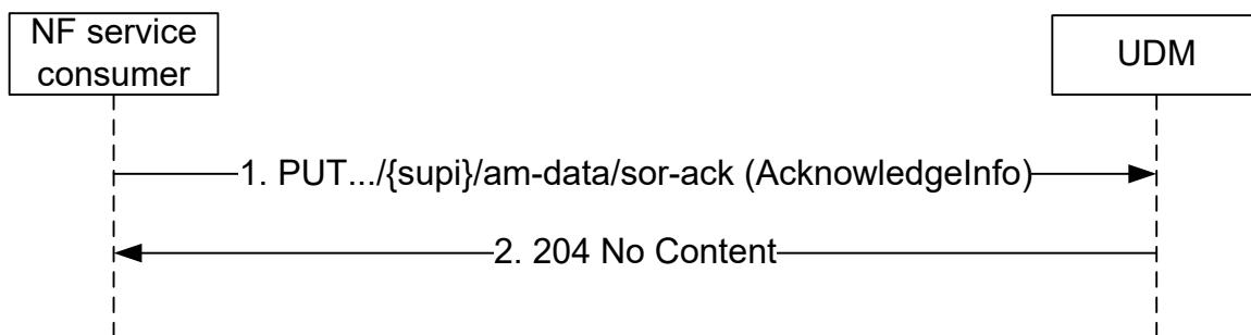
**Figure 5.2.2.6.2-1: Providing acknowledgement of Steering of Roaming**
