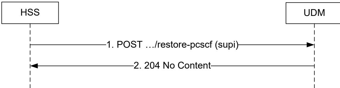
**Figure 5.3.2.8.2-1: P-CSCF-RestorationTrigger**
