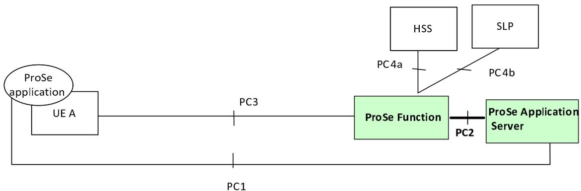
Figure 4.1.1: PC2 reference point in ProSe Architecture
