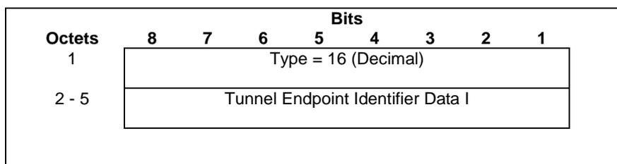
Figure 8.3-1: Tunnel Endpoint Identifier Data I Information Element
