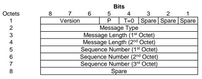
Figure 5.3-1: The format of Echo and Version Not Supported Indication messages Header
