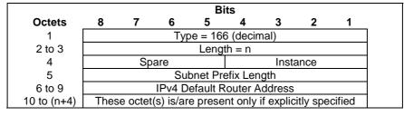
Figure 8. 97-1: IPv4 Configuration Parameters (IP4CP)
