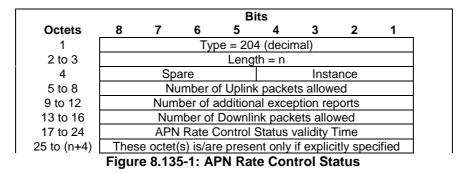
Octets 17 to 24 are coded as the time in seconds relative to 00:00:00 on 1 January 1900 (calculated as continuous time without leap seconds and traceable to a common time reference) where binary encoding of the integer part is in the 32 most significant bits and binary encoding of the fraction part in the 32 least significant bits. The fraction part is expressed with a granularity of  $1/2^{**}32$  second.
