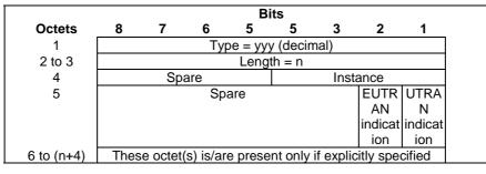
Figure 8.116-1: WLAN Offloadability Indication
