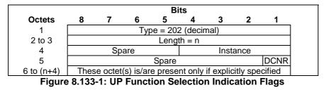
For each message, the applicable flags of the UP Function Selection Indication Flags IE shall be clearly specified in the individual message clause. The remaining flags of the UP Function Selection Indication Flags IE not so indicated shall be discarded by the receiver.
