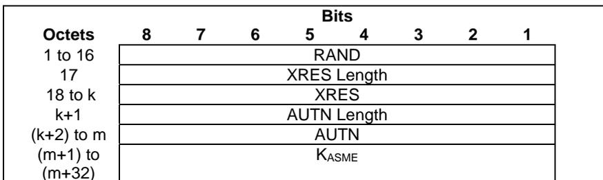
Figure 8.38-9: Authentication Quadruplet
