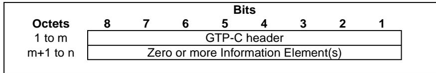
Figure 5.6-1: GTP-C Header followed by subsequent Information Elements
