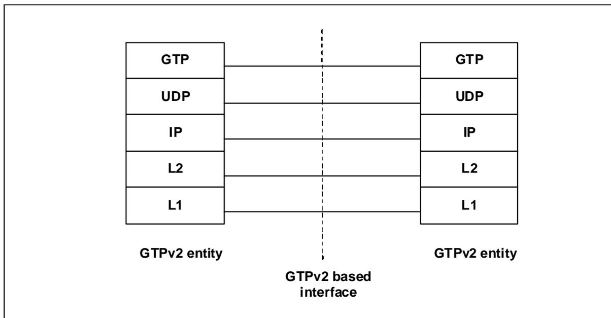
**Figure 4.2.0-1: GTPv2 stack**
