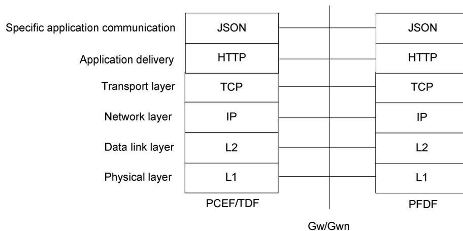
**Figure 6.1.1: Protocol stack of the Gw/Gwn reference point**
