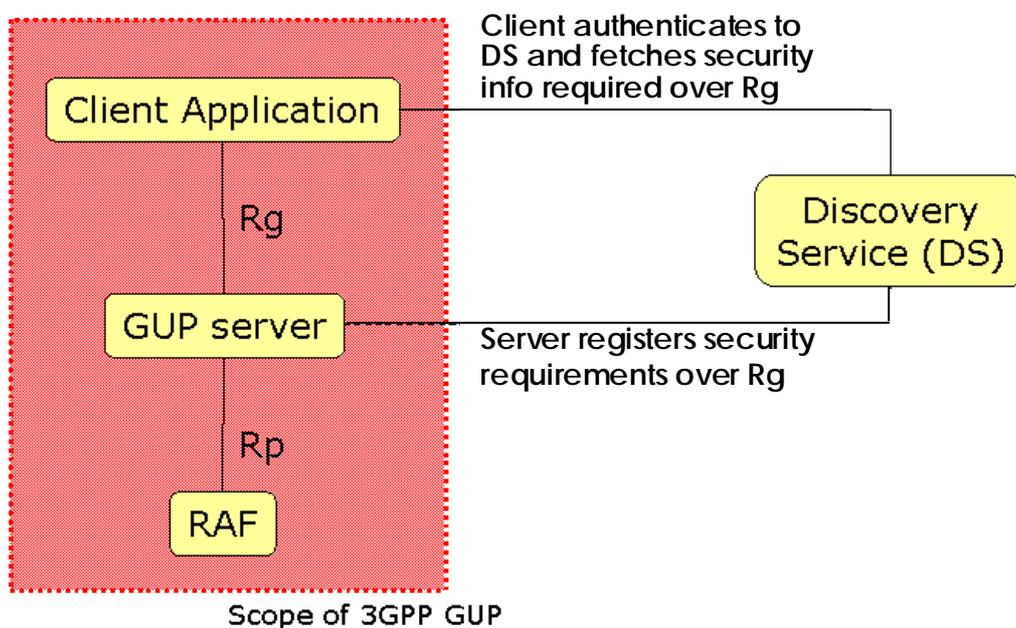
**Figure 1: GUP Authentication, Authorization and Security architecture.**
