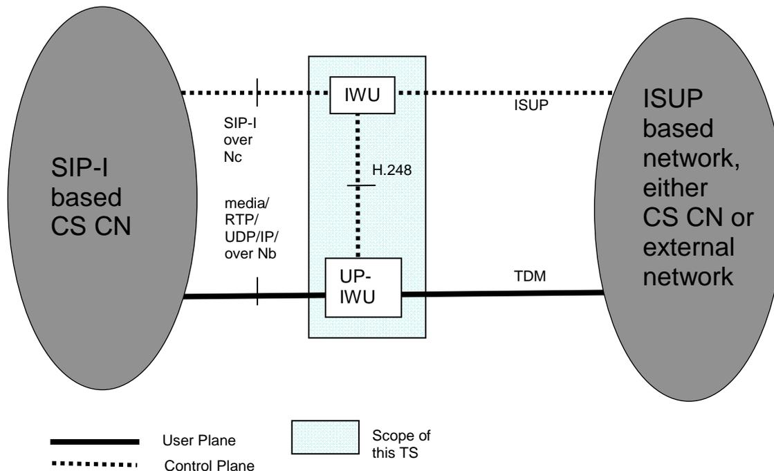
NOTE: The IWU is a logical function that may reside with other 3GPP logical functions in the same physical nodes, e.g. in an (G)MSC Server. The figure shows only the logical separation.
