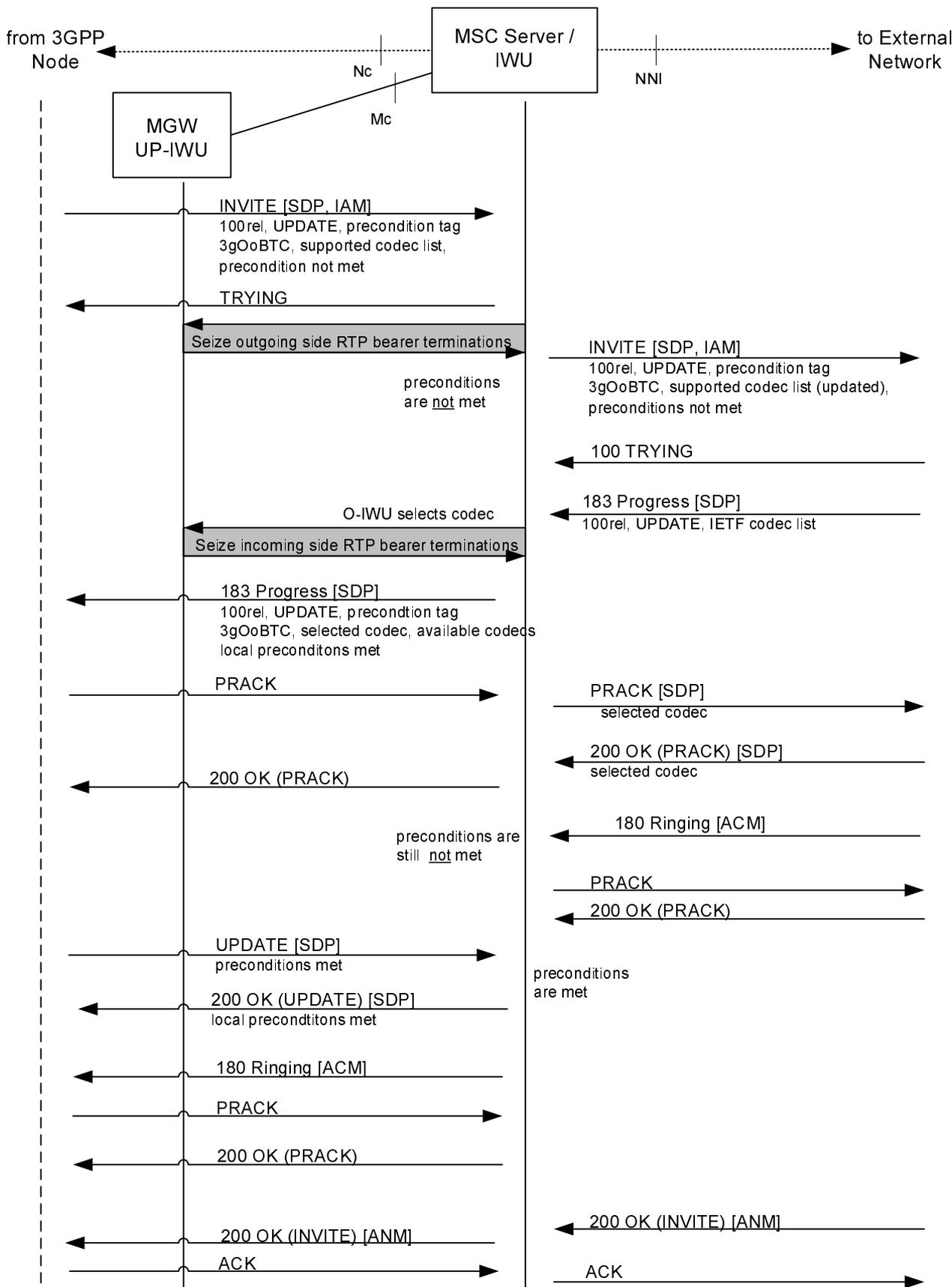
Figure 4.6.3.2.1: Outgoing Call (message sequence chart), example with support of 100rel but no support for preconditions
