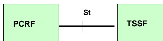
Figure 4c.2.1: The PCC architecture with the St for non-roaming scenario
