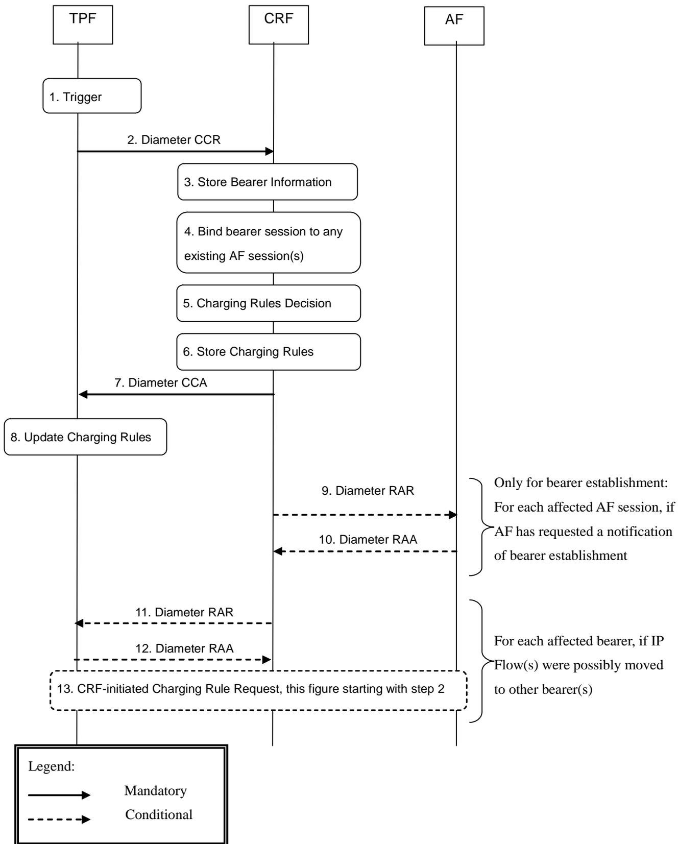
1. The TPF receives a trigger for a Charging Rule Request, such as the establishment or modification of a bearer or an RAR from the CRF.
