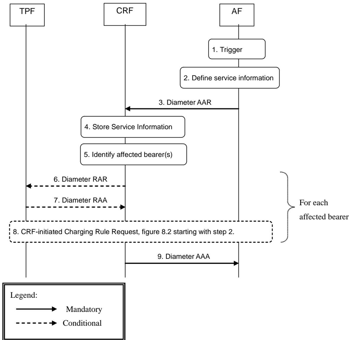
1. The AF receives an internal or external trigger to provide Service Information, at a set-up of a new AF session or at a modification of an existing AF session.
