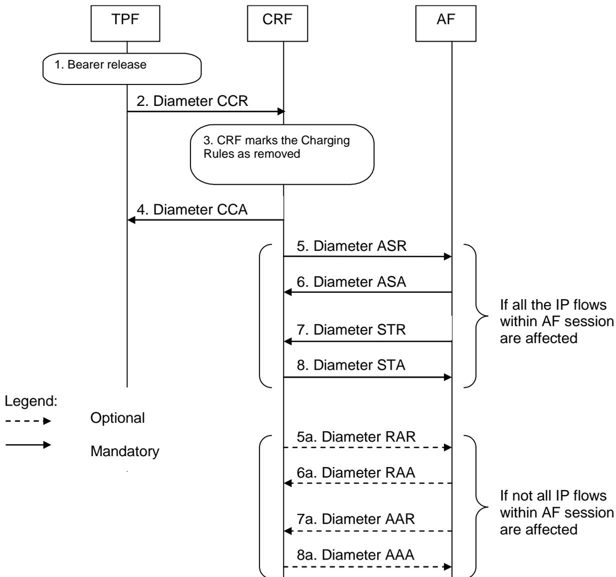
1. A bearer is deactivated. For GPRS, the SGSN deactivates the PDP context carrying IP flow(s) of by sending the Delete PDP Context Request message to the GGSN.
