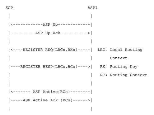
Note: In the case of an unsuccessful registration attempt (e.g., Invalid RKn), the Register Response message will contain an unsuccessful indication and the ASP will not subsequently send an ASP Active message.
