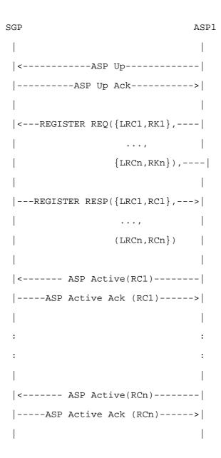
Note: In the case of an unsuccessful registration attempt (e.g., Invalid RKn), the Register Response message will contain an unsuccessful indication and the ASP will not subsequently send an ASP Active message. Each LRC/RK pair registration is considered independently.
