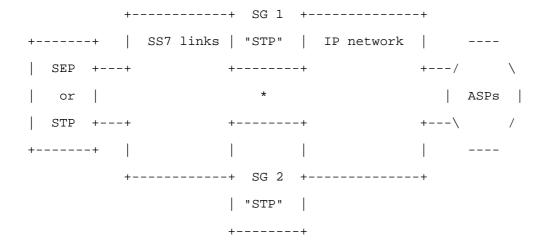
\* Note:. SG-to ûSG communication is recommended for carrier grade networks, using an MTP3 linkset or an equivalent, to allow re-routing between the SGs in the event of route failures. Where SGPs are used, inter-SGP communication is recommended. Inter-SGP protocol is outside of the scope of this document.
