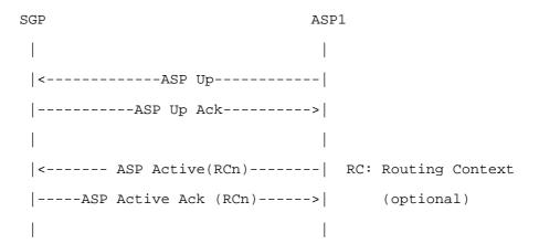
Note: If the ASP Active message contains an optional Routing Context parameter, The ASP Active message only applies for the specified RC value(s). For an unknown RC value, the SGP responds with an Error message.
