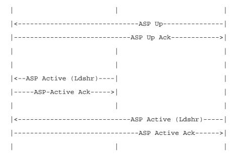
5.1.4 Three ASPs in an Application Server ("n+k" sparing, load-sharing case)
