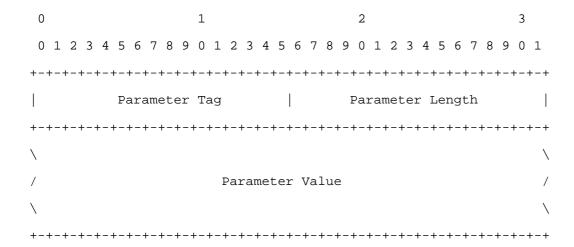
Where more than one parameter is included in a message, the parameters may be in any order, except where explicitly mandated. A receiver SHOULD accept the parameters in any order.
