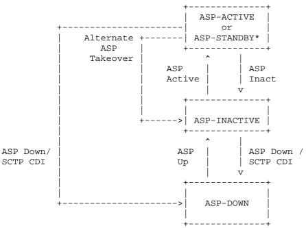
\*Note: ASP-ACTIVE and ASP-STANDBY differ only in whether the ASP is currently receiving Data traffic within the AS.
