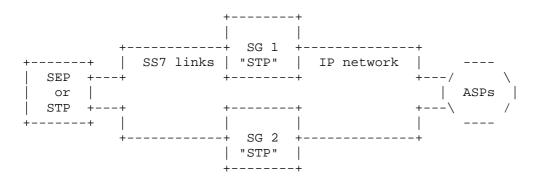
Note: there is no SG-to-SG communication shown, so each SG can be reached only via the direct linkset from the SS7 network.
