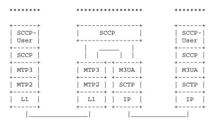
STP - SS7 Signalling Transfer Point
