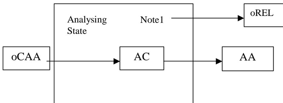
Note 1: The release event (oREL) can occur in any state resulting in a transition to Releasing state.
