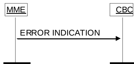
Figure 4.3.3B.2-2: Error Indication procedure, MME originated. Successful operation.
