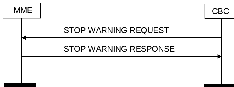
Figure 4.3.3A.3-1: Stop Warning procedure, Unsuccessful operation.
