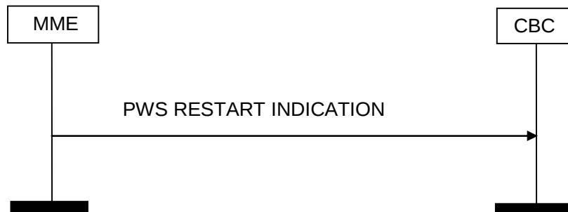
Figure 4.3.3E.2-1: PWS Restart Indication, Successful Operation.
