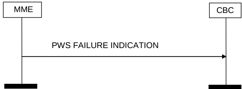
Figure 4.3.3F.2-1: PWS Failure Indication, Successful Operation.
