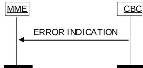
Figure 4.3.3B.2-1: Error Indication procedure, CBC originated. Successful operation.
