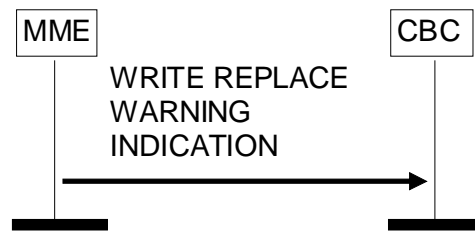
Figure 4.3.3C.2-1: Write Replace Warning Indication procedure, MME originated. Successful operation.
