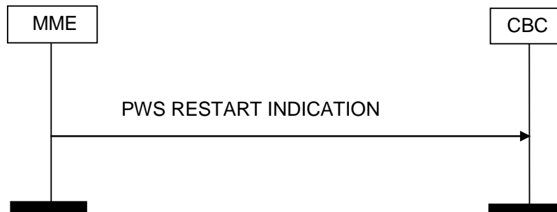
Figure 4.3.3E.2-1: PWS Restart Indication, Successful Operation.
