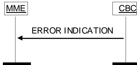
Figure 4.3.3B.2-1: Error Indication procedure, CBC originated. Successful operation.
