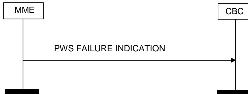
Figure 4.3.3F.2-1: PWS Failure Indication, Successful Operation.
