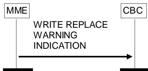
Figure 4.3.3C.2-1: Write Replace Warning Indication procedure, MME originated. Successful operation.
