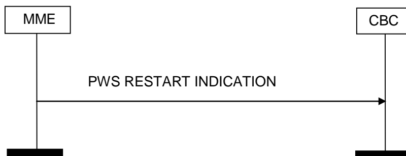
Figure 4.3.3E.2-1: PWS Restart Indication, Successful Operation.
