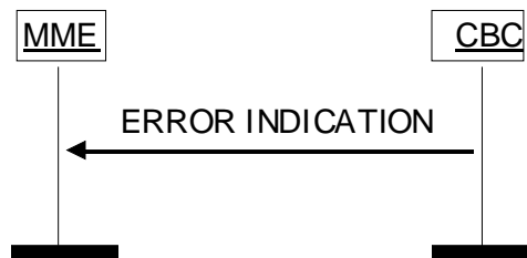
Figure 4.3.3B.2-1: Error Indication procedure, CBC originated. Successful operation.
