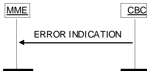
Figure 4.3.3B.2-1: Error Indication procedure, CBC originated. Successful operation.
