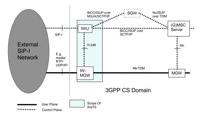
NOTE 1: If needed a SGW is applied for conversion (both ways) of the transport level between the IWU and the (G)MSC. The SGW may be implemented as a stand-alone entity or it may be located in another entity of the CS Domain. A SGW function is not required for certain signalling transports, where M3UA+SCTP+IP is used in CS network and IWU. The implementation options are not further discussed in the present document.
