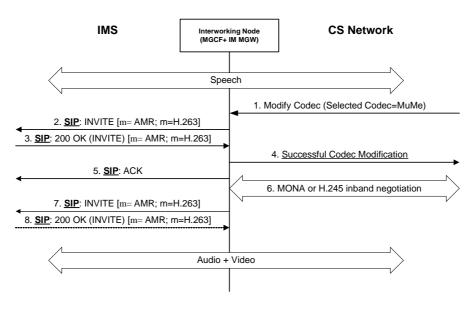
Figure E.2.5.2.1.2.2.1: CS network originated modification from speech to multimedia when the CS leg supports BICC
