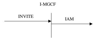
Figure 3: Receipt of an Invite request (continuity procedure supported in the ISUP network)
