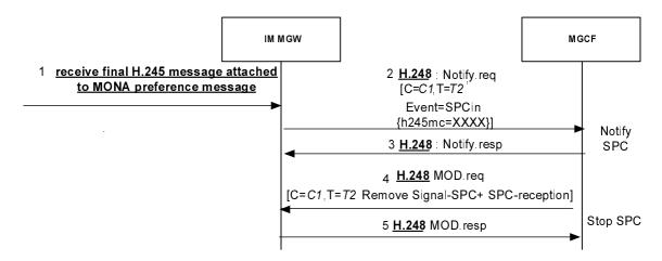
NOTE 2: The Context model in figure E.4.2.2.1 is assumed in this call flow. Figure E.4.2.7.4.4.1: Mn interactions for terminating SPC procedure.
