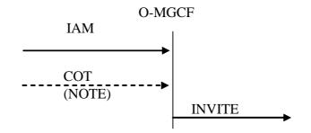
NOTE: Waiting for the COT is recommended, if the Continuity Check indicator in the Nature of Connection Indicators parameter in the incoming IAM is set to indicate either '*continuity check required on this circuit* or '*continuity check performed on previous circuit*
