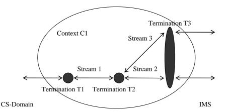
Termination: T1 CS-Domain (CS-Bearer (BS30) for H.245 control, Speech, Video) T2 Multiplexing (H.245 control, Speech, Video) T3 Video (own RTP-stream) + Speech (own RTP-stream)
