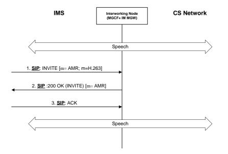
Figure E.2.5.2.2.2.1: IM CN subsystem originated modification from speech to multimedia when the CS leg supports ISUP or BICC without SCUDIF
