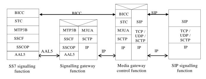
Figure 26: Control Plane interworking between CS networks supporting BICC over MTP3B over AAL5 and the IM CN subsystem
