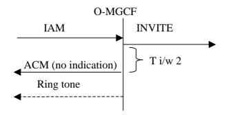
Figure 17: Sending of ACM (Ti/w<sub>2</sub> elapses)
