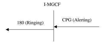
Figure 7: Receipt of CPG (Alerting)
