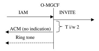
Figure 17: Sending of ACM (Ti/w<sub>2</sub> elapses)
