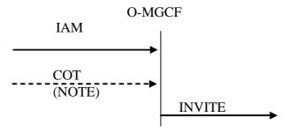
NOTE: Waiting for the COT is a network option. Furthermore, it only applies if the Continuity Check indicator in the Nature of Connection Indicators parameter in the incoming IAM is set to indicate either "continuity check required on this circuit" or "continuity check performed on previous circuit"
