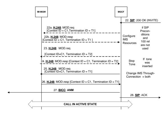
Figure 38/2: Basic CS Network Originating Session, BICC Backward Bearer Establishment (message sequence chart continue)
