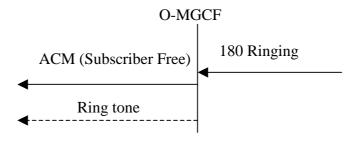
Figure 16: Sending of ACM (Receipt of first 180 ringing)
