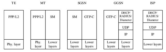
Figure 11a: Signalling plane of non transparent case
