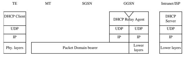
Figure 16c: Protocol stack for access with DHCP end-to-end
