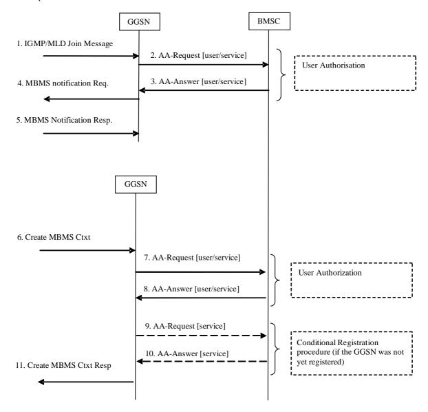
Figure 26; Activation of an MBMS multicast service
