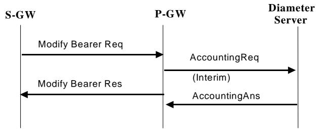
Figure 25d.2: Diameter accounting update for bearer modification
