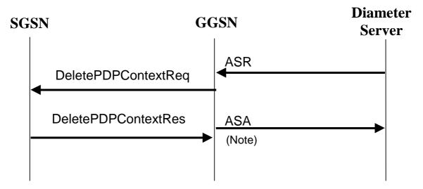
NOTE: As showed on figure 25d, the GGSN need not wait for the DeletePDPContextResponse from the SGSN to send the ASA to the Diameter server.
