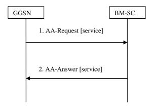
Figure 29: MBMS Registration procedure
