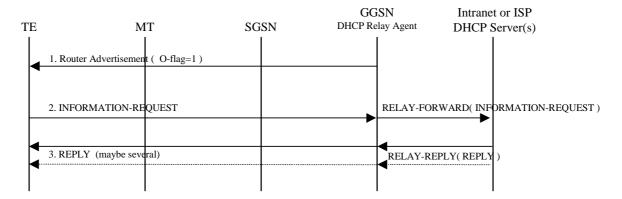
Figure 16f: DHCPv6 Other configuration signal flow
