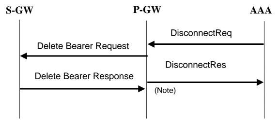
NOTE: As shown on figure 25a.3, the P-GW need not wait for the Delete Bearer Response from the S-GW to send the RADIUS DisconnectResponse to the AAA server.
