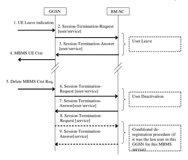
Figure 32: MBMS Service deactivation procedure
