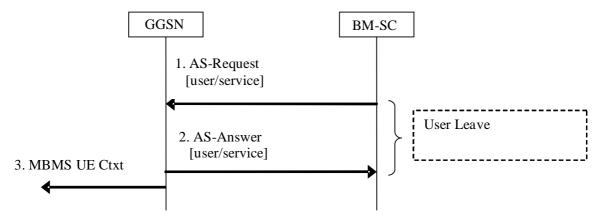
Figure 32a: BM-SC initiated MBMS Service deactivation procedure
