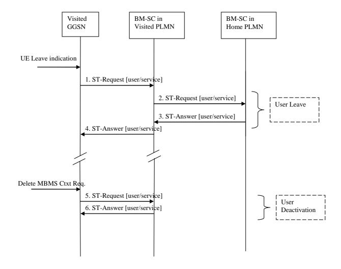
Figure 31: Deactivation of an MBMS multicast service in roaming scenario with service provided in the visited PLMN
