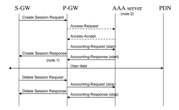
NOTE 1: If some external applications require RADIUS Accounting request (Start) information before they can process user packets, then the selected APN (P-GW) may be configured in such a way that the P-GW drops user data until the Accounting Response (START) is received from the AAA server. The P-GW may wait for the Accounting Response (START) before sending the Create Session Response. The P-GW may reject the bearer if the Accounting Response (START) is not received.
