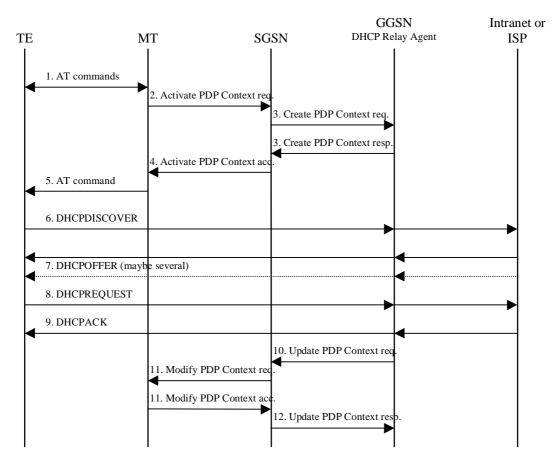
Figure 16d: DHCPv4 signal flow
