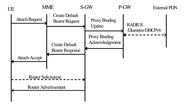
Figure 11bd: IPv6 Stateless Address Autoconfiguration for PMIP-based S5/S8
