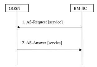
Figure 31: MBMS De-Registration procedure BM-SC initiated
