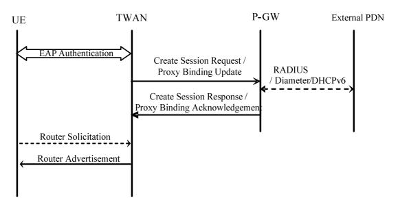
Figure 11be: IPv6 Stateless Address Autoconfiguration for trusted WLAN access for GTP/PMIP-based S2a
