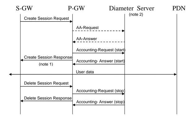
NOTE 1: If some external applications require Diameter Accounting request (Start) information before they can process user packets, then the selected APN (P-GW) may be configured in such a way that the P-GW drops user data until the Accounting Answer (START) is received from the Diameter server. The P-GW may wait for the Accounting Answer (START) before sending the Create Session Response. The P-GW may reject the bearer if the Accounting Answer (START) is not received.
