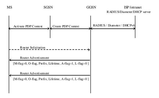
Figure 11bb: IPv6 Stateless Address Autoconfiguration
