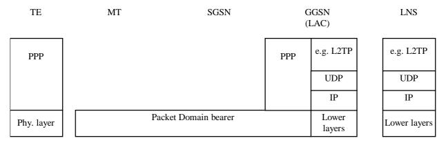
Figure 15: Protocol stack for virtual dial-up access with PPP frame tunnelling
