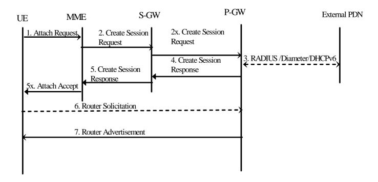
Figure 11bc: IPv6 Stateless Address Autoconfiguration for GTP-based S5/S8
