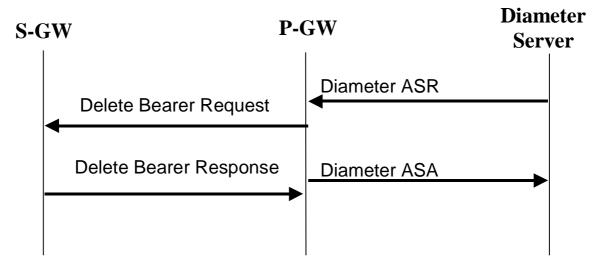
Figure 25d.3: Server-initiated Bearer Termination with Diameter
