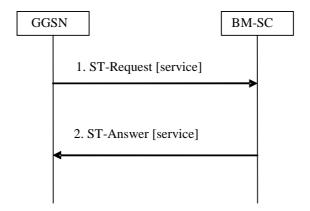
Figure 30: MBMS De-Registration procedure
