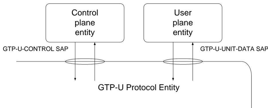
Figure 62: The GTP-U-Control SAP and GTP-U-DATA SAP
