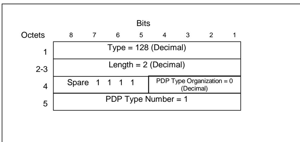
Figure 38: End User Address Information Element for PPP
