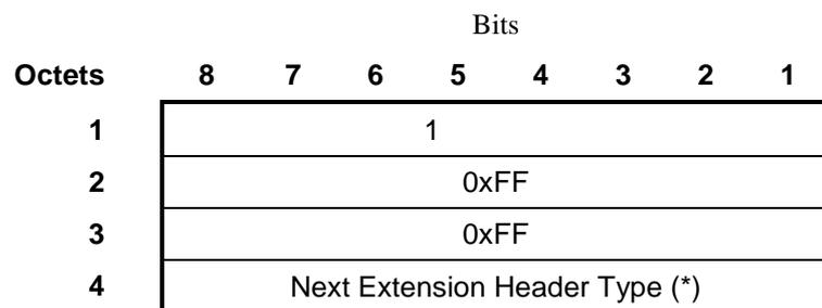
Figure 8: Suspend Response Extension Header
