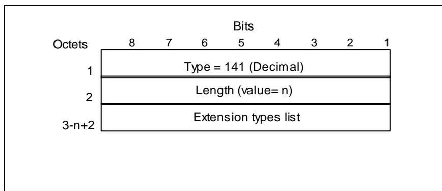
Figure 55: Extension Header Type List Information Element
