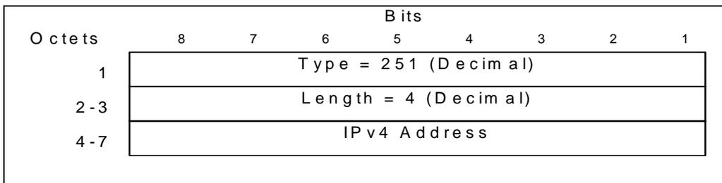
Figure 58a: Ipv4 Charging Gateway Address Information Element
