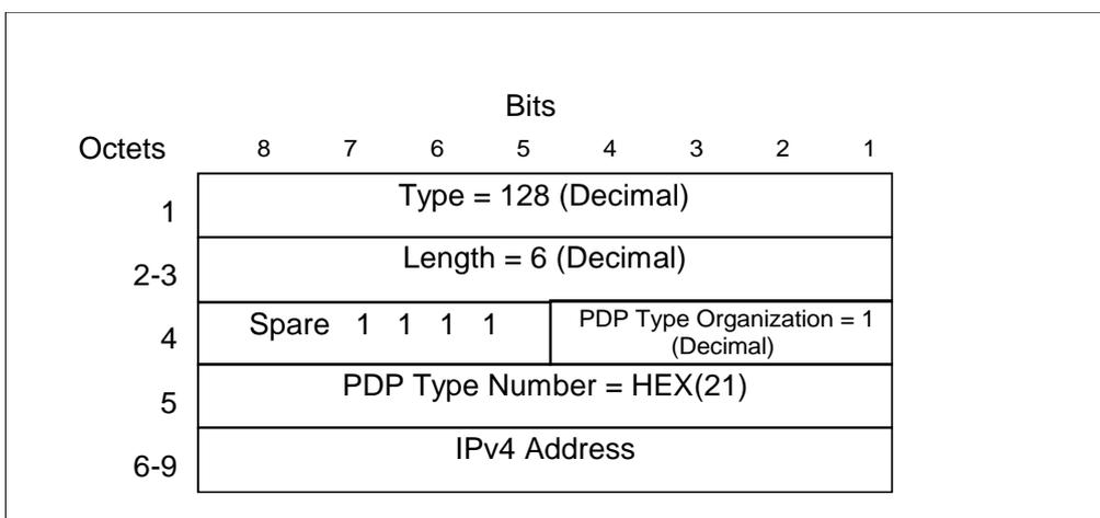
Figure 36: End User Address Information Element for IPv4
