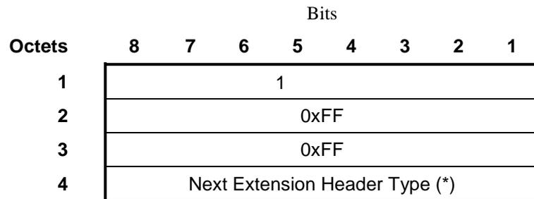
Figure 7: Suspend Request Extension Header
