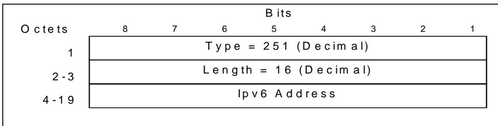
Figure 58b: Ipv6 Charging Gateway Address Information Element
