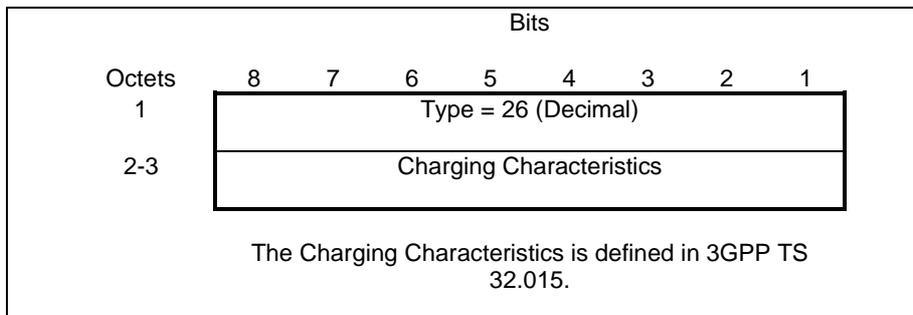
Figure 31: Charging Characteristics Information Element
