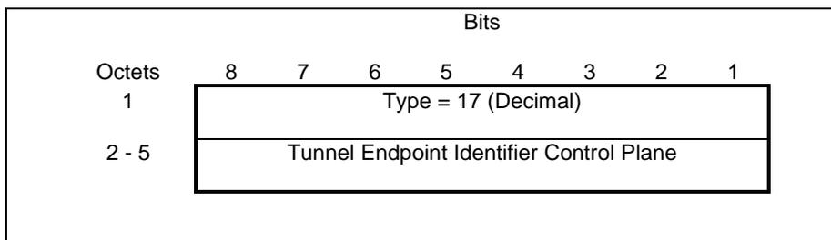
Figure 22: Tunnel Endpoint Identifier Control Plane Information Element
