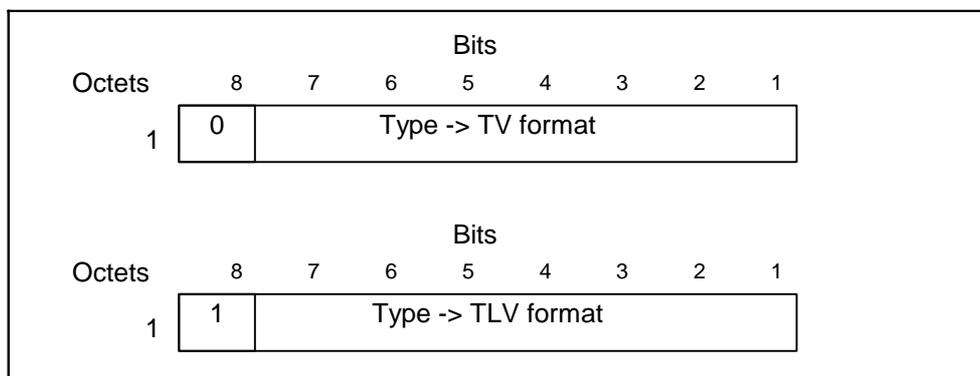
Figure 8: Type field for TV and TLV format
