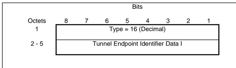
Figure 21: Tunnel Endpoint Identifier Data I Information Element
