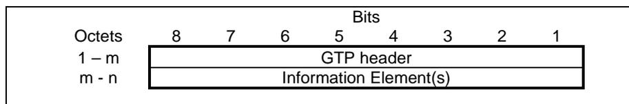
Figure 61: GTP Header followed by subsequent Information Elements
