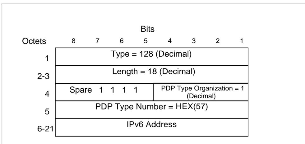
Figure 37: End User Address Information Element for IPv6
