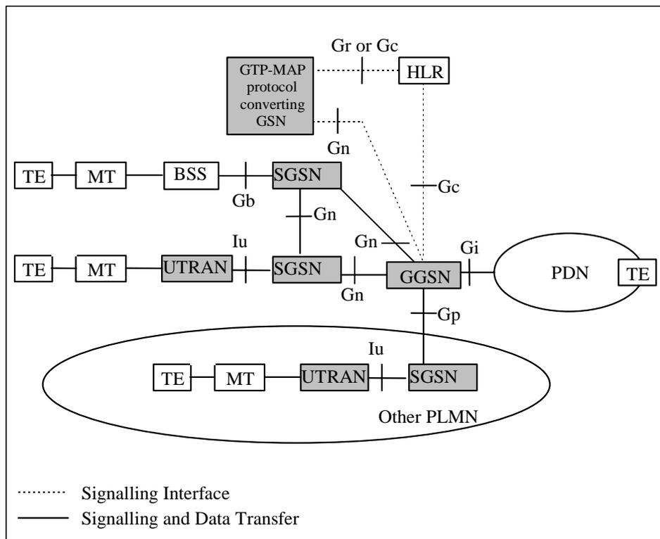
**Figure 1: GPRS Logical Architecture with interface name denotations**
