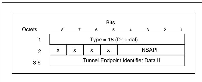
Figure 23: Tunnel Endpoint Identifier Data II Information Element
