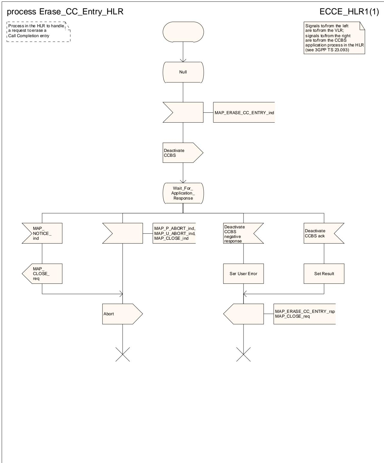
Figure 22.14.3/1: Process Erase\_CC\_Entry\_HLR
