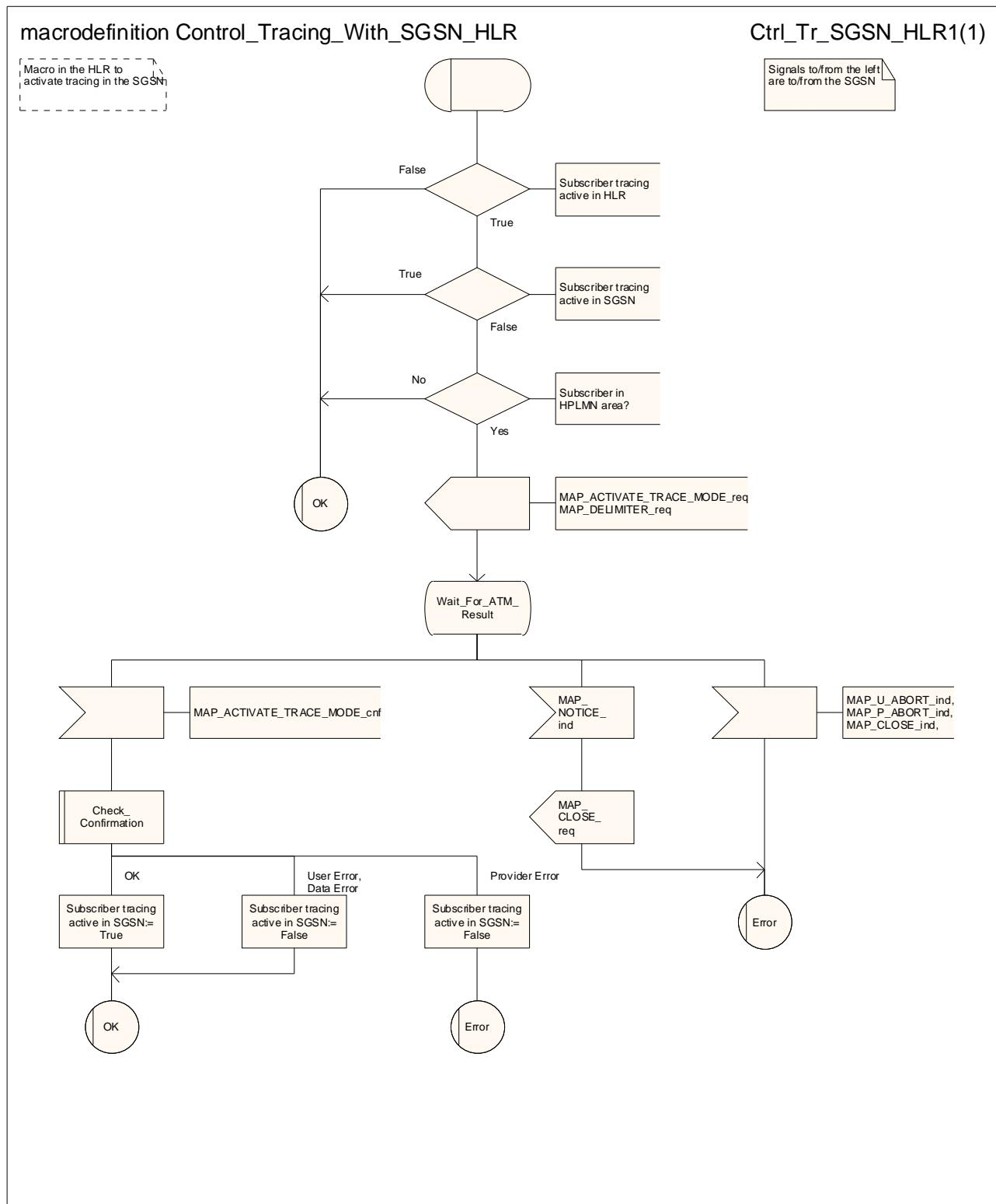
**Figure 25.9/7: Macro Control\_Tracing\_With\_SGSN\_HLR**
