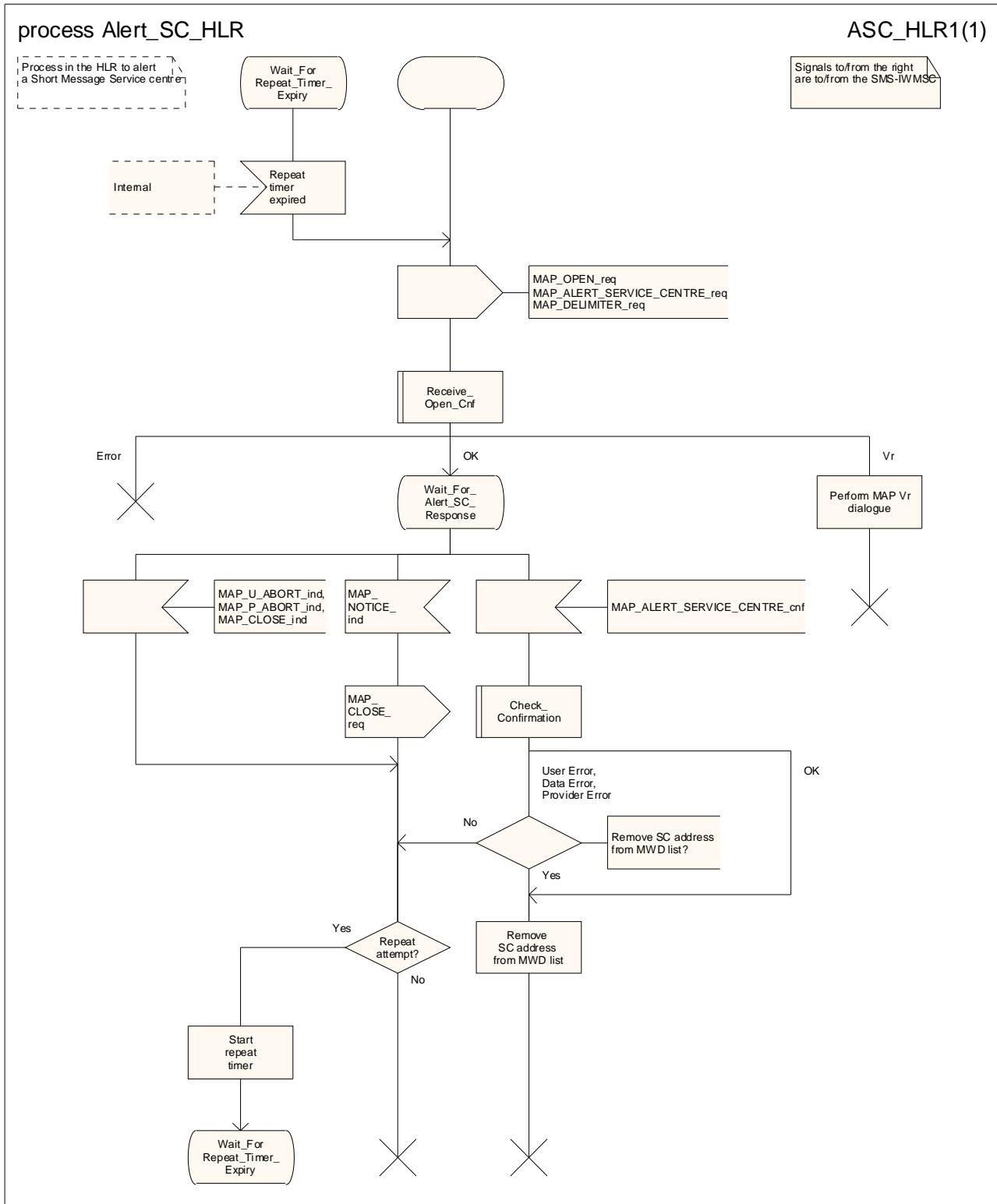
Figure 25.10/4: Process Alert\_SC\_HLR
