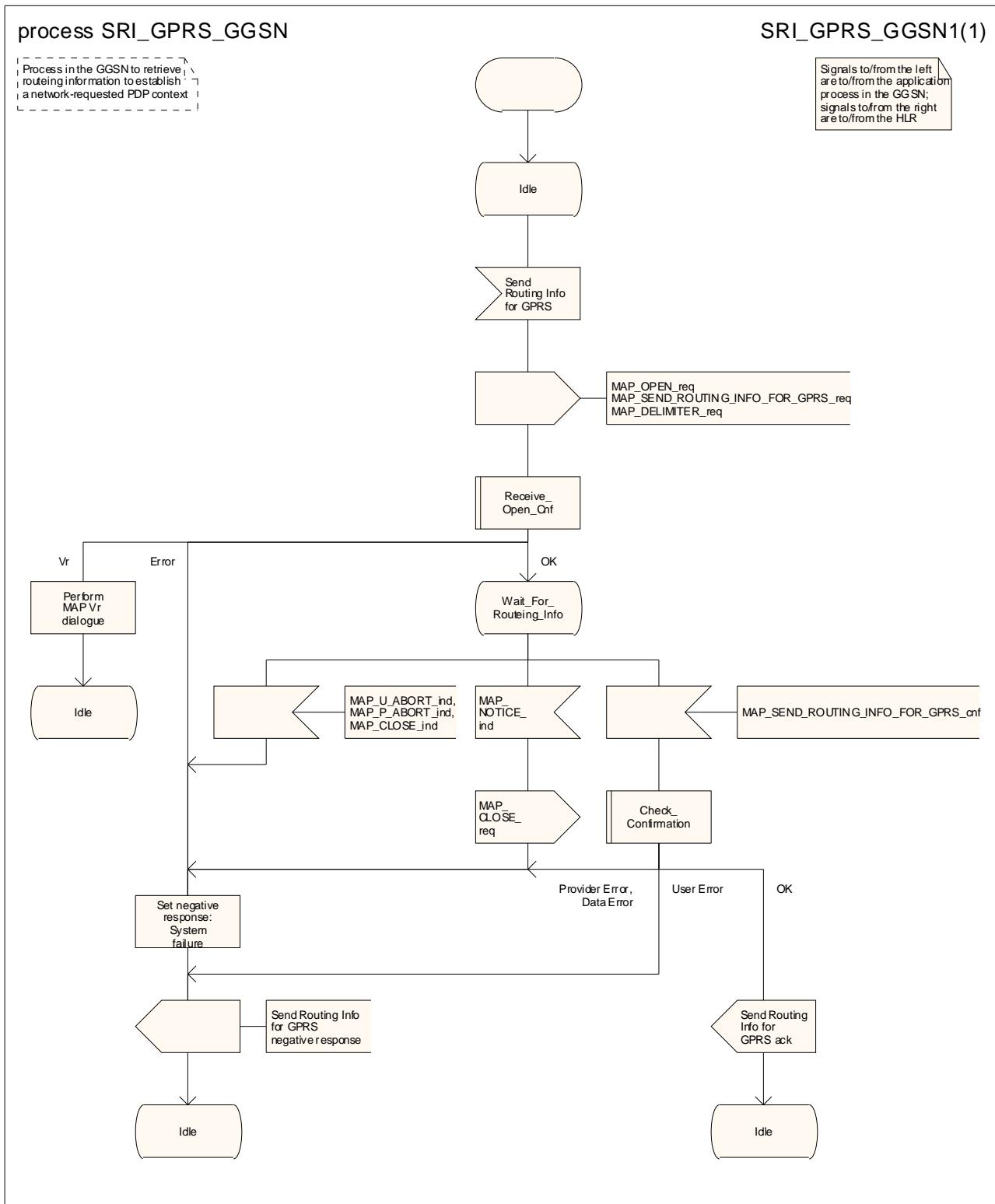
Figure 24.1/1: Process SRI\_GPRS\_GGSN
