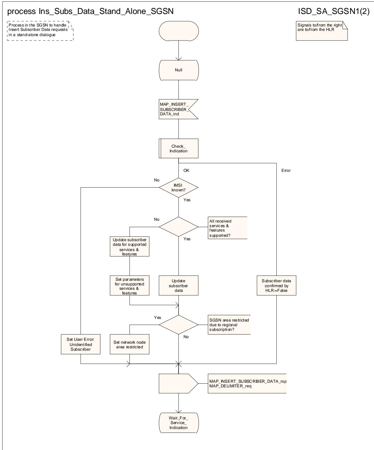
Figure 20.3/11 (sheet 1 of 2): Process Ins\_Subs\_Data\_Stand\_Alone\_SGSN
