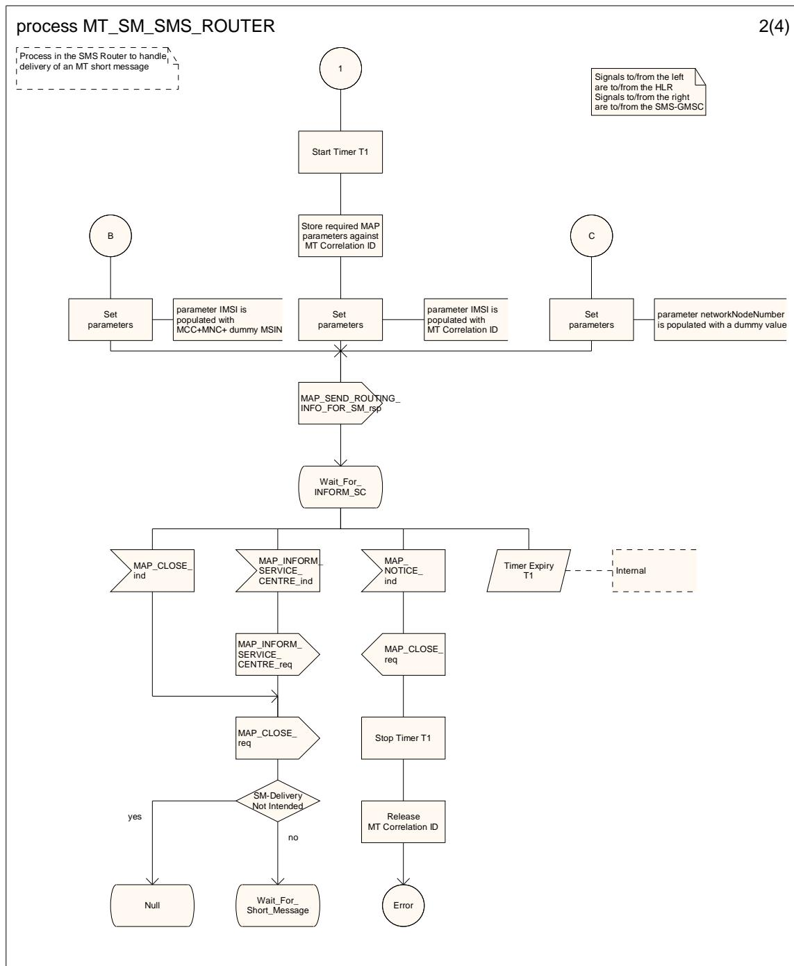
Figure 23.3/14 (sheet 2 of 4): Process MT\_SM\_SMS\_ROUTER
