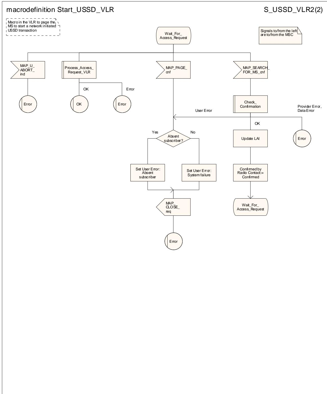
Figure 22.10.3/2 (sheet 2 of 2): Macro Start\_USSD\_VLR
