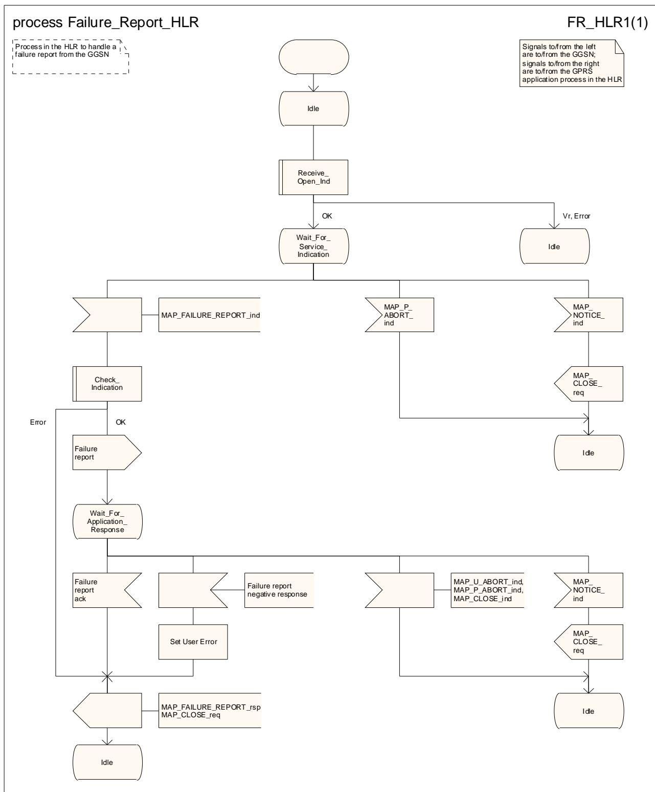
**Figure 24.2/2: Process Failure\_Report\_HLR**
