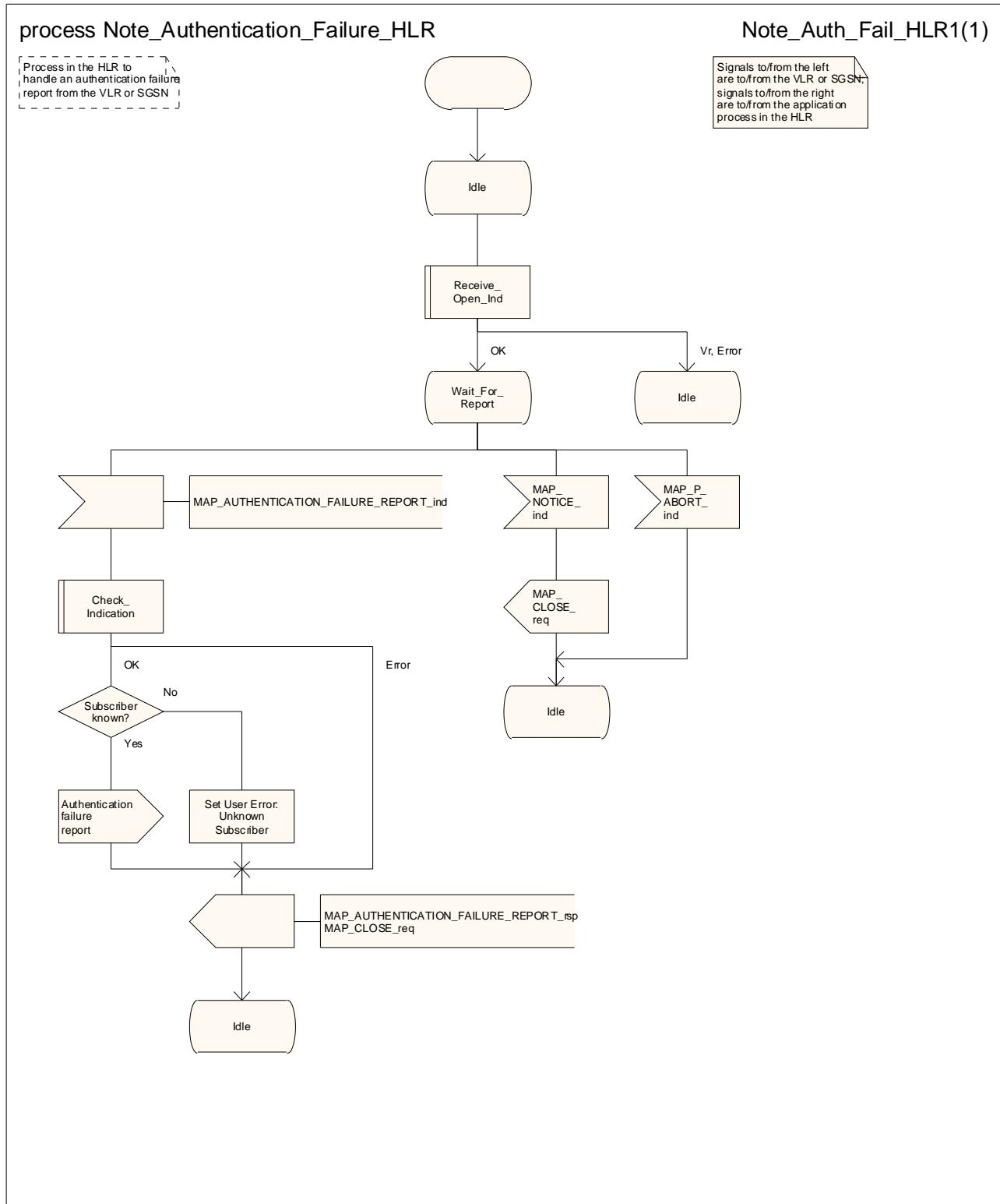
Figure 25.5/11: Process Note\_Authentication\_Failure\_HLR
