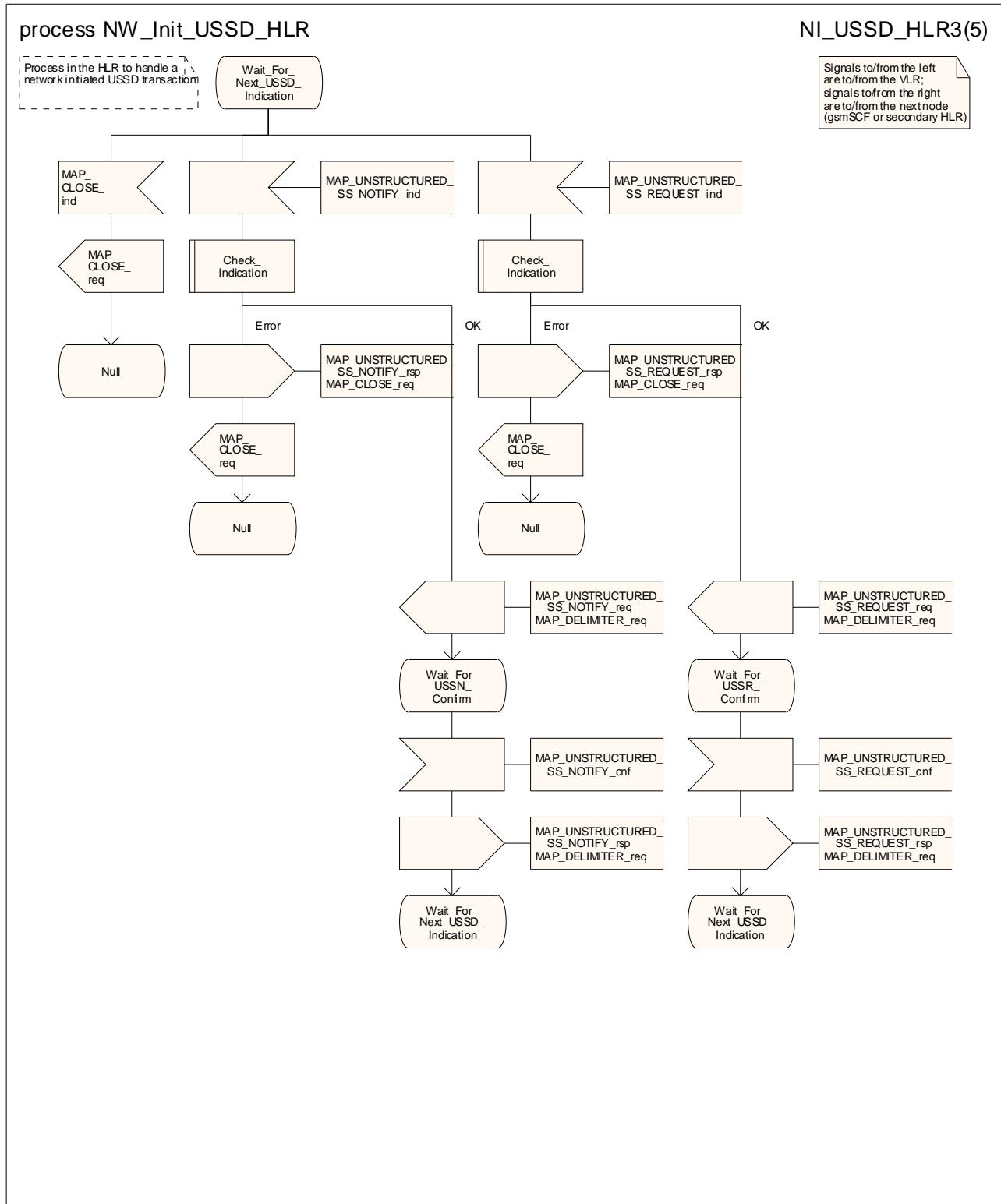
Figure 22.10.4/1 (sheet 3 of 5): Process NW\_Init\_USSD\_HLR
