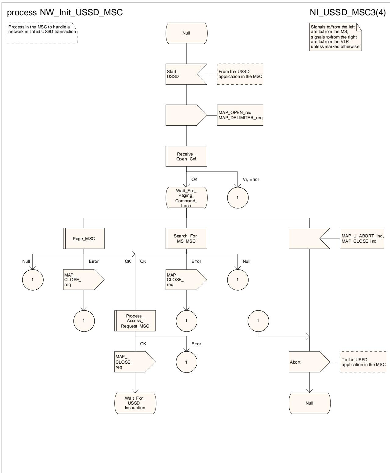
Figure 22.10.2/1 (sheet 1 of 4): Process NW\_Init\_USSD\_MSC
