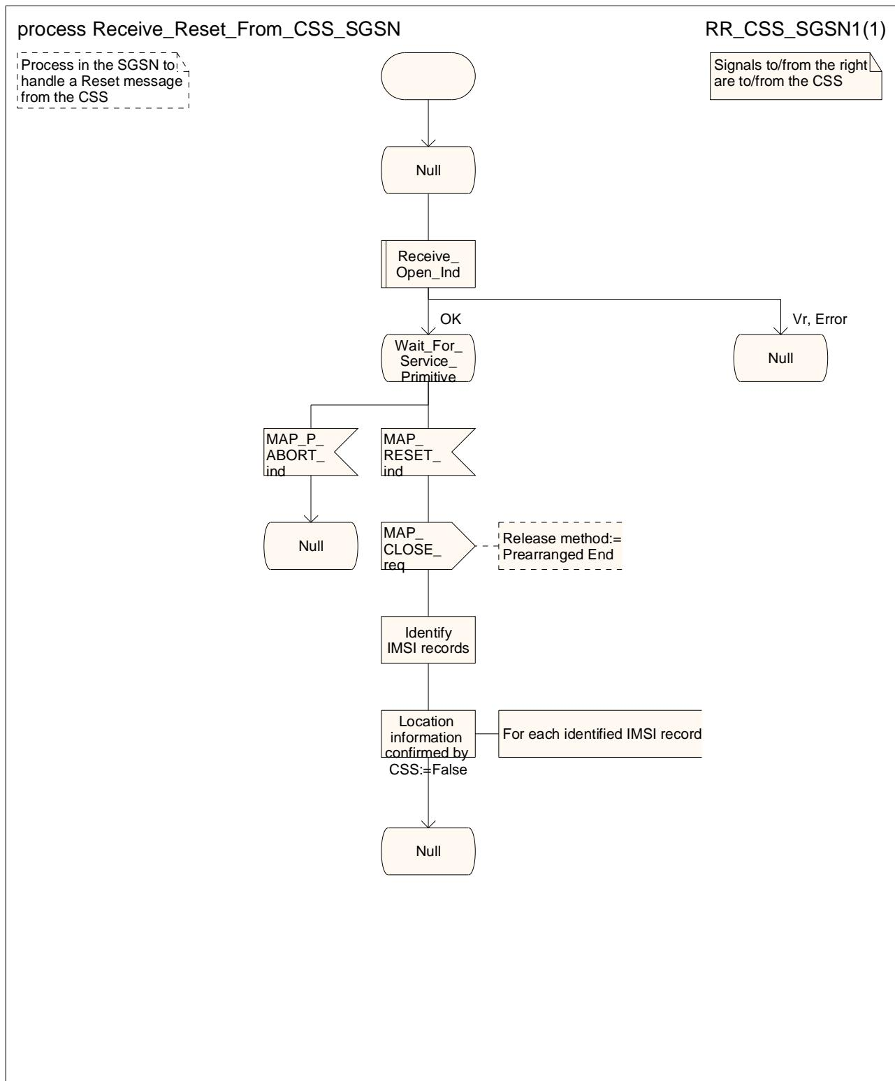
Figure 19.3.3/7: Process Receive\_Reset\_From\_CSS\_SGSN
