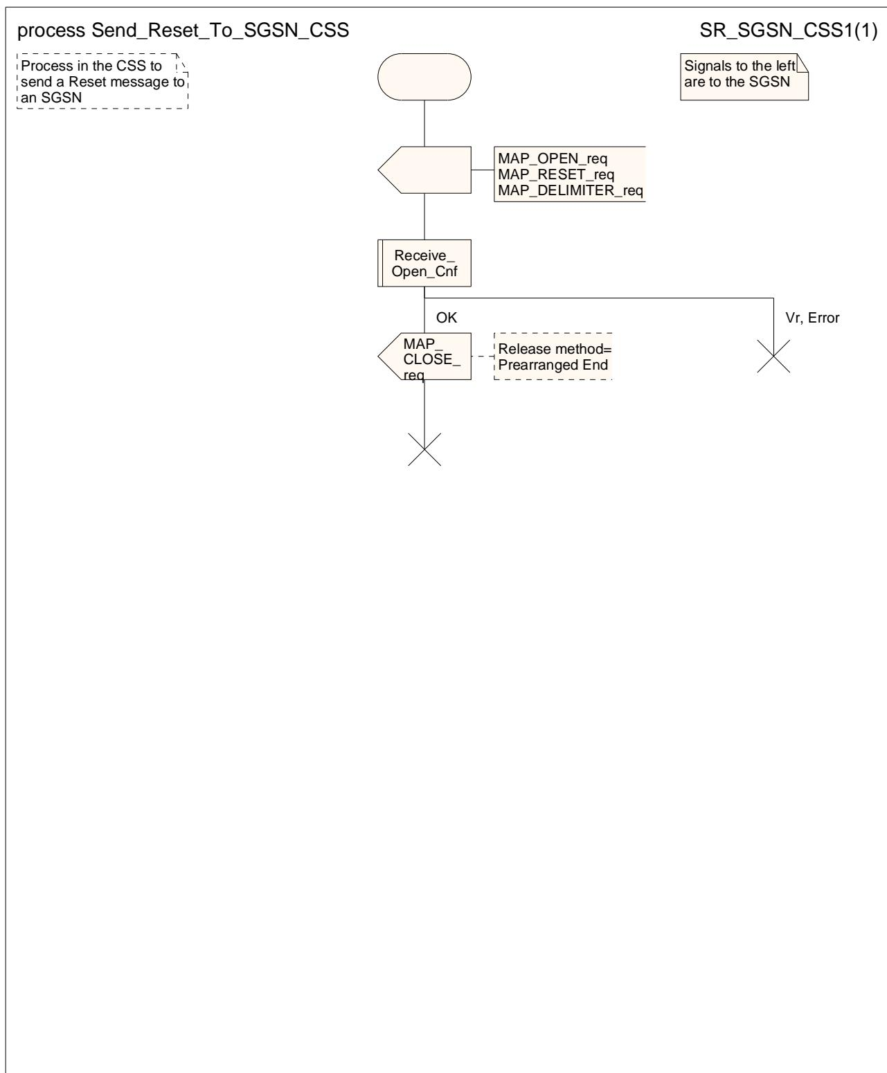
Figure 19.3.3/5: Process Send\_Reset\_To\_SGSN\_CSS
