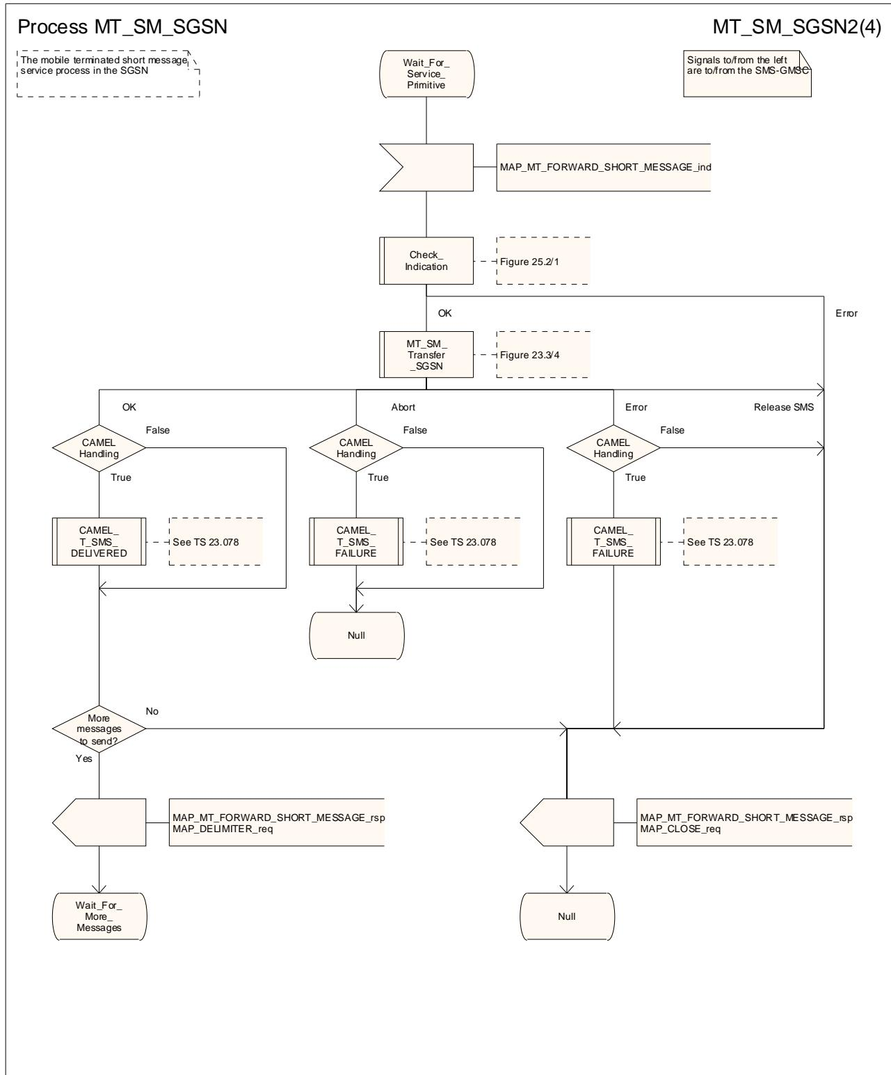
Figure 23.3/10 (sheet 2 of 4): Process MT\_SM\_SGSN
