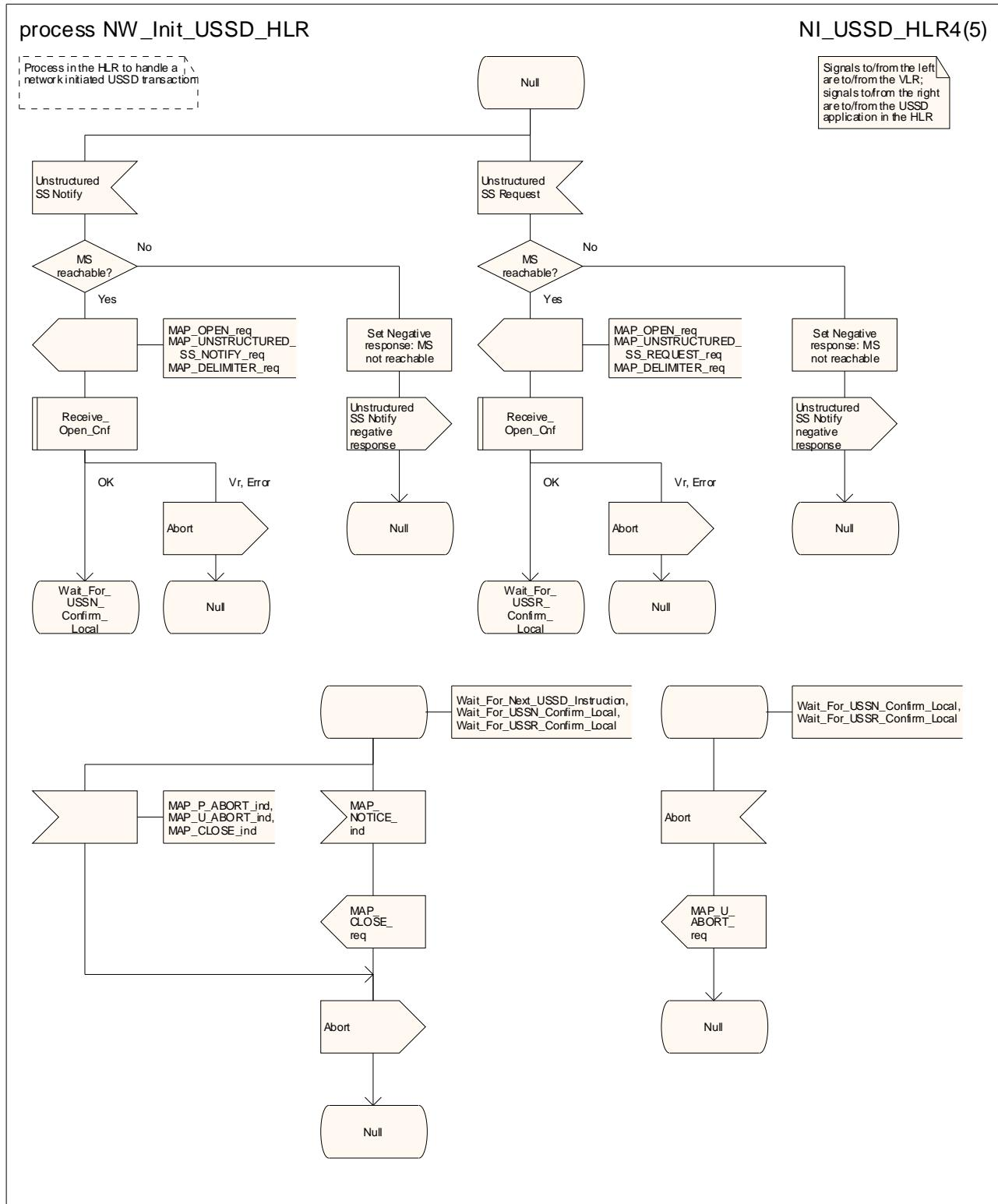
Figure 22.10.4/1 (sheet 4 of 5): Process NW\_Init\_USSD\_HLR
