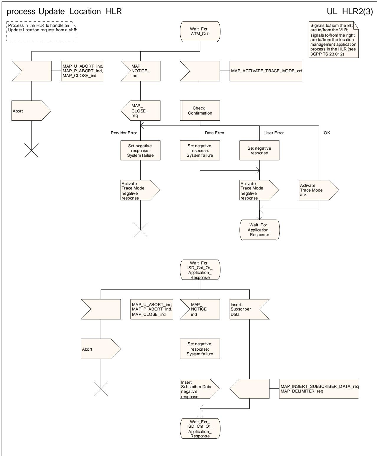
**Figure 19.1.1/13 (sheet 2 of 3): Process Update\_Location\_HLR**
