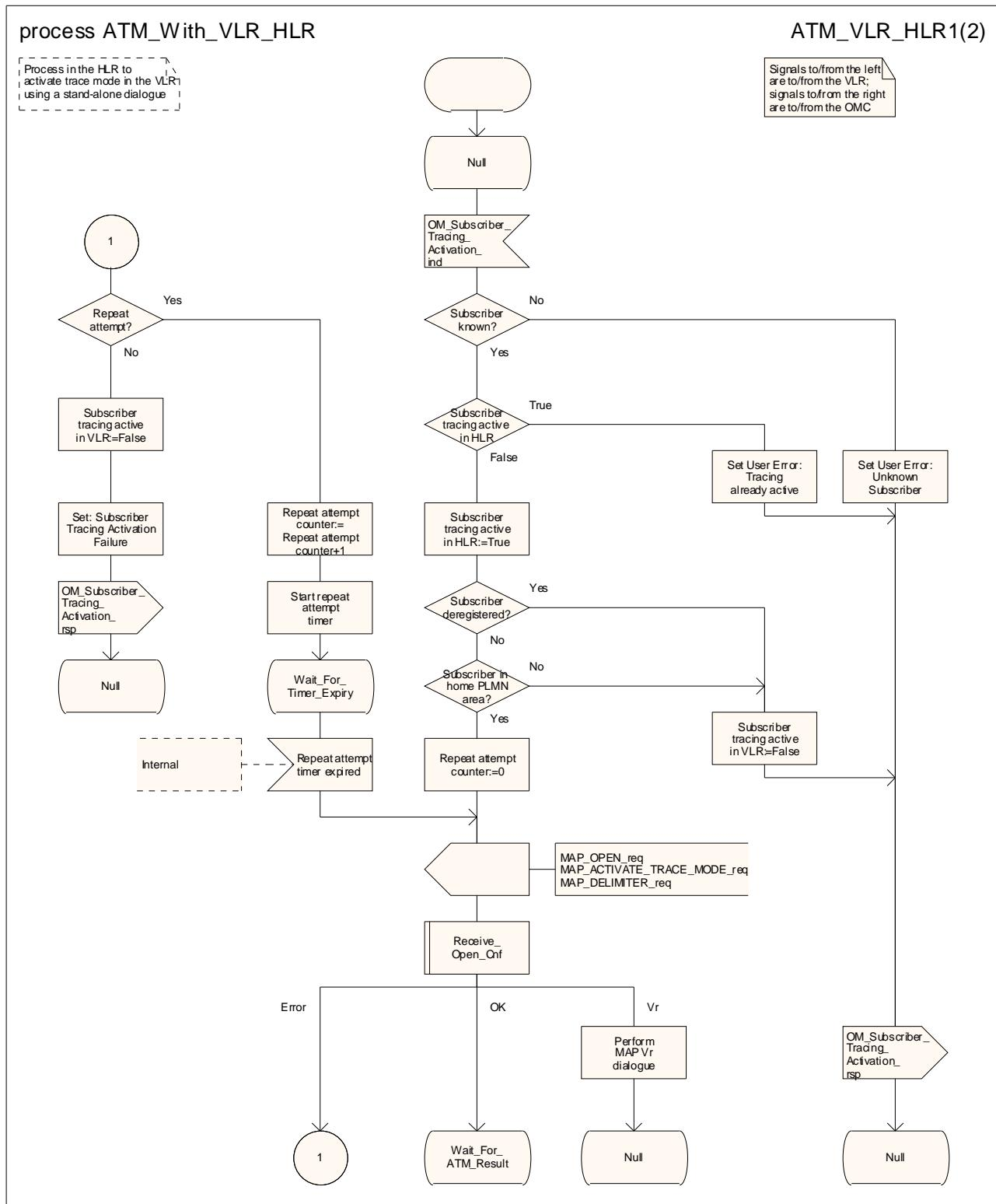
Figure 20.2/8 (sheet 1 of 2): Process ATM\_With\_VLR\_HLR
