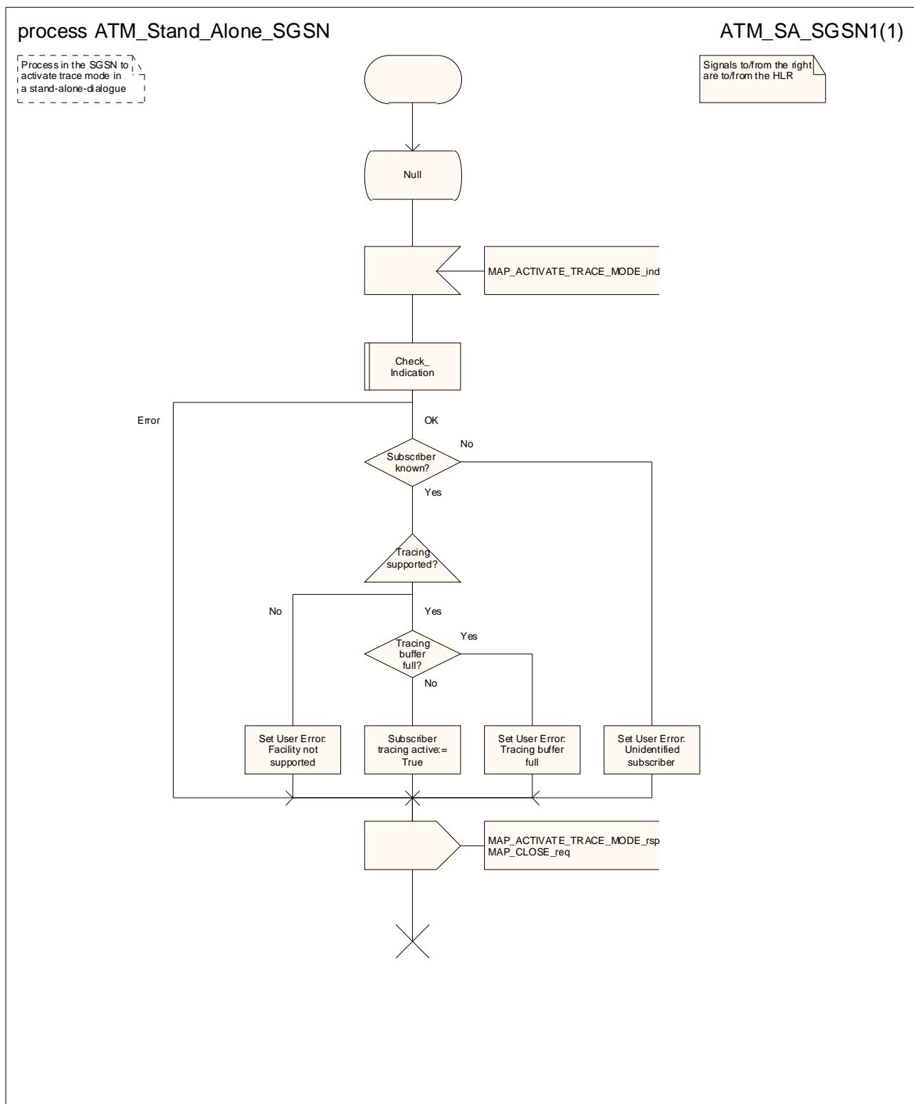
Figure 20.2/11: Process ATM\_Standalone\_SGSN
