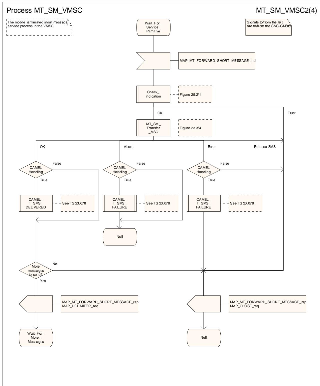
Figure 23.3/6 (sheet 2 of 4): Procedure MT\_SM\_VMSC
