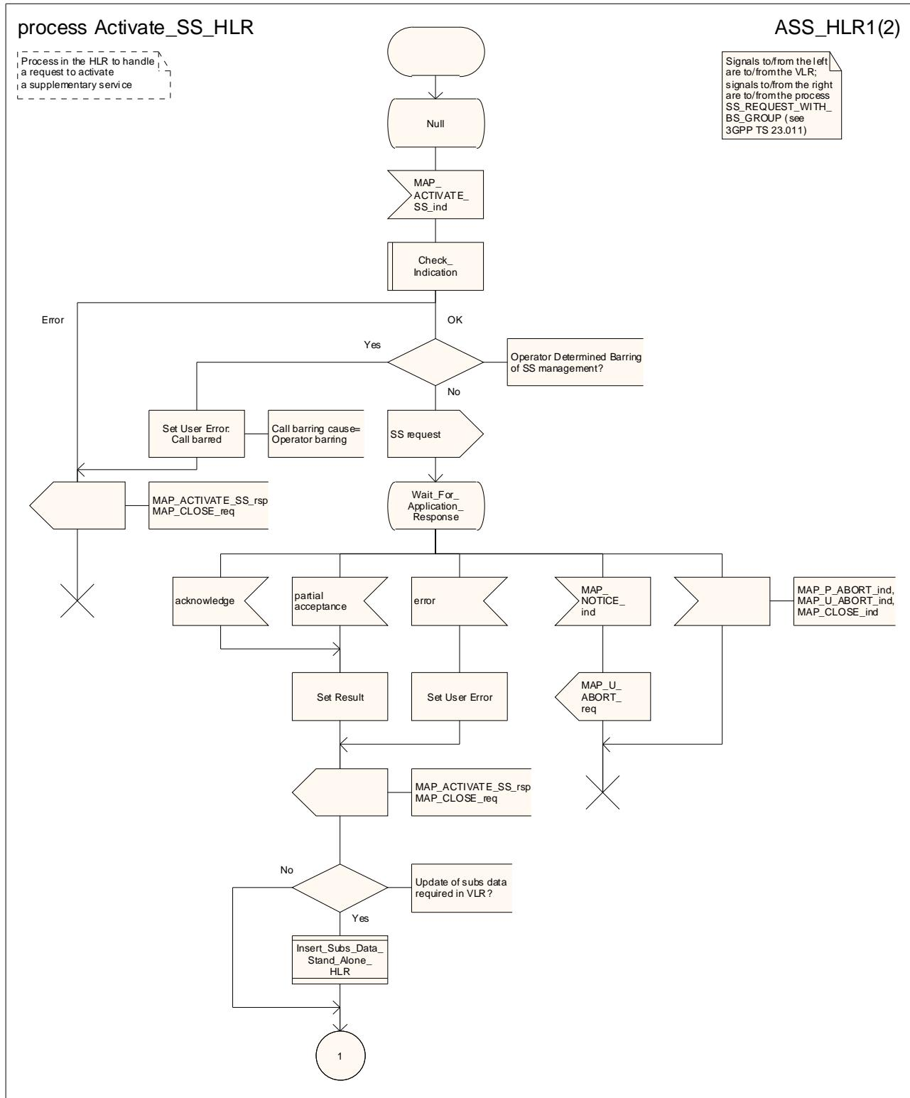
Figure 22.4.4/1 (sheet 1 of 2): Process Activate\_SS\_HLR
