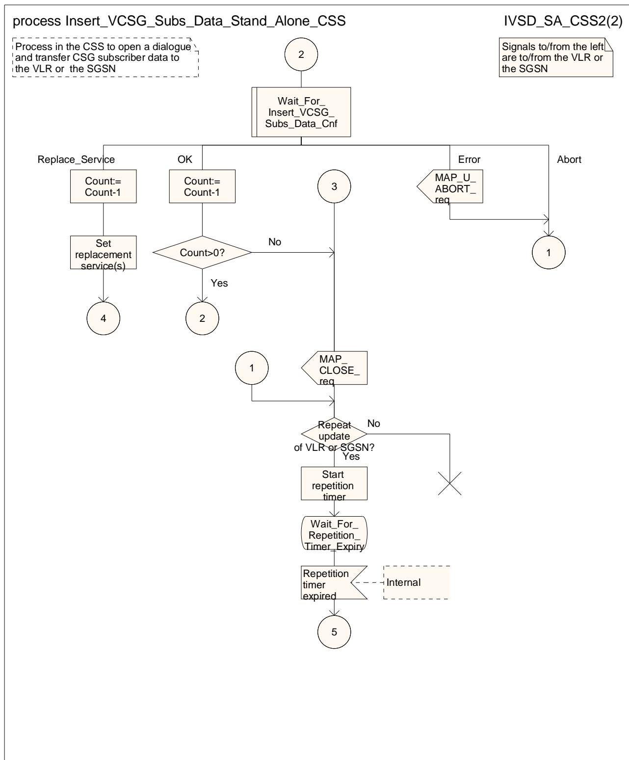
Figure 25.7/8 (sheet 2 of 2): Process Insert\_VCSG\_Subs\_Data\_Stand\_A lone\_CSS
