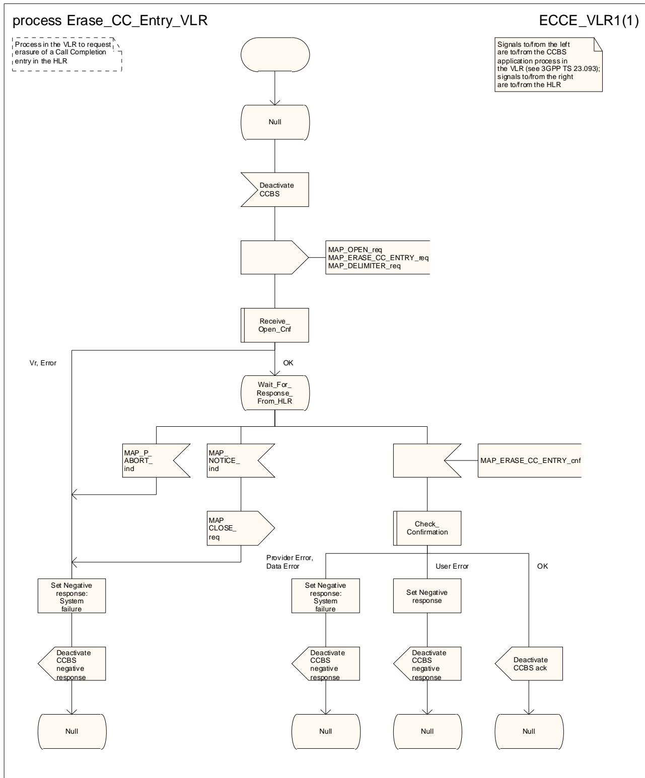
**Figure 22.14.2/1: Process Erase\_CC\_Entry\_VLR**
