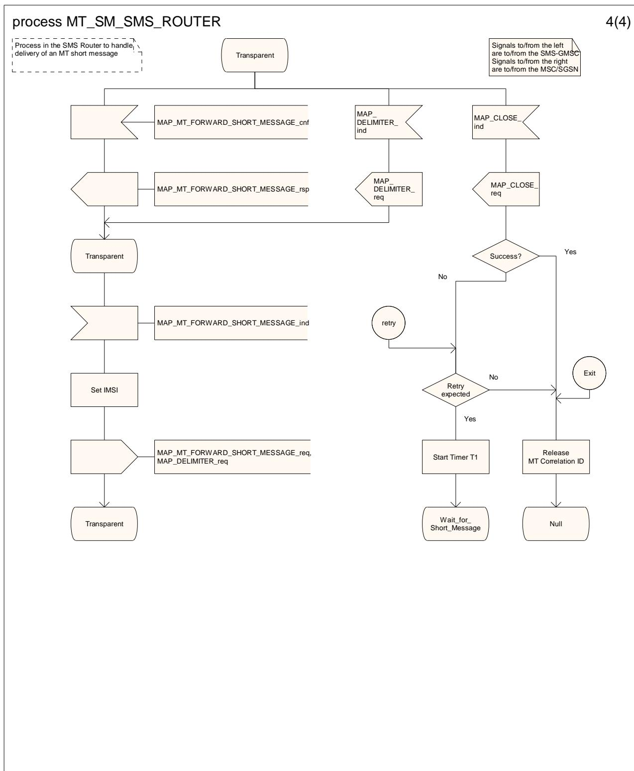
Figure 23.3/14 (sheet 4 of 4): Process MT\_SM\_SMS\_ROUTER
