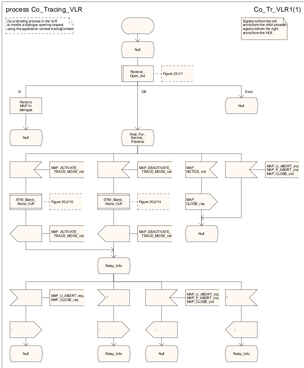
Figure 20.1/1: Process Co\_Tracing\_VLR
