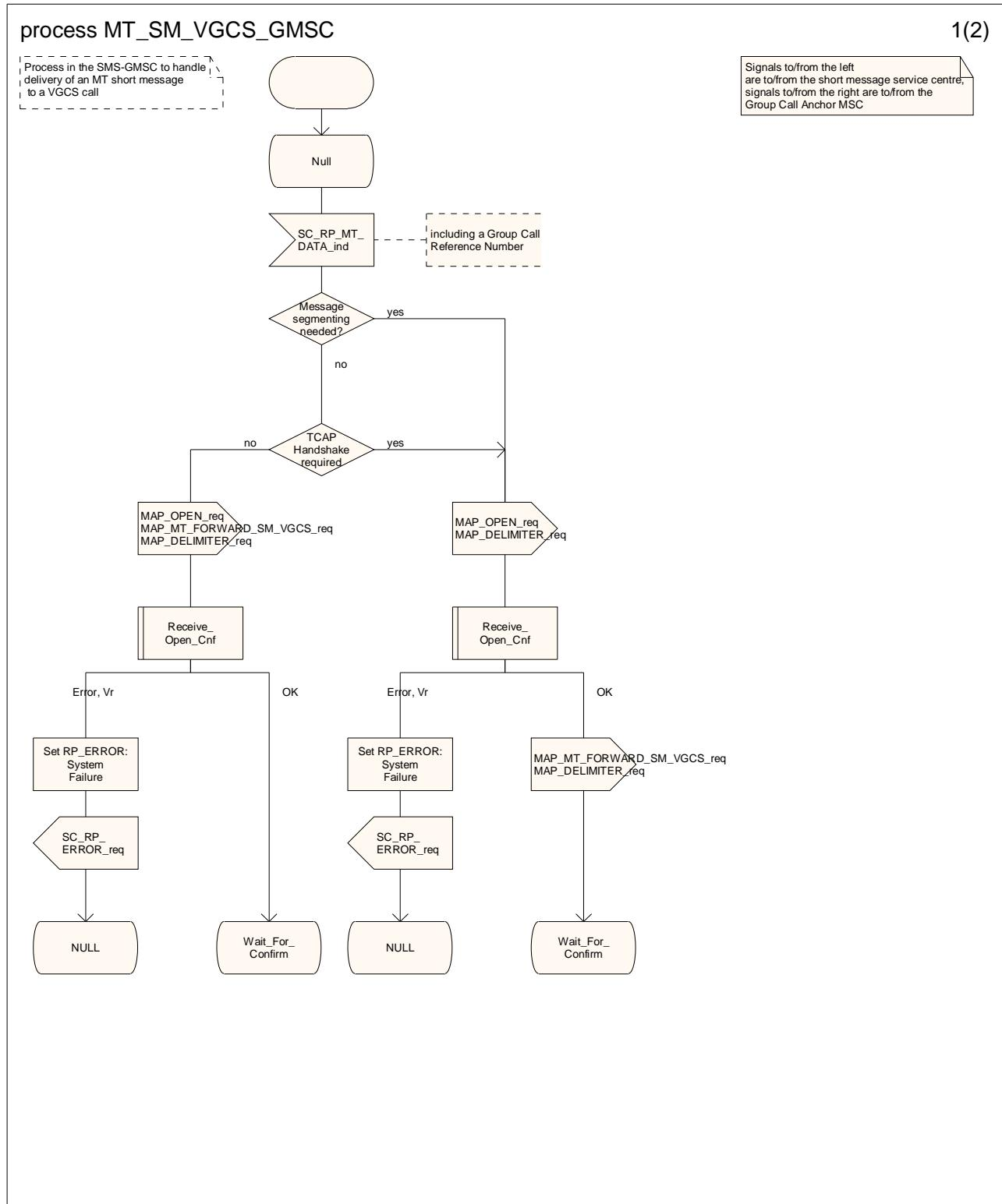
Figure 23.7/2 (sheet 1 of 2): Process MT\_SM\_VGCS\_GMSC
