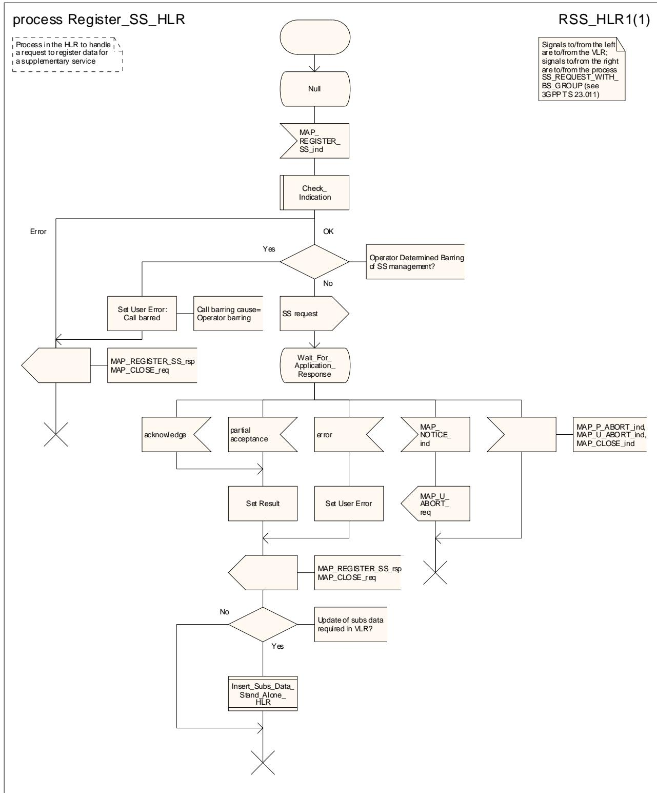
Figure 22.2.4/1: Process Register\_SS\_HLR
