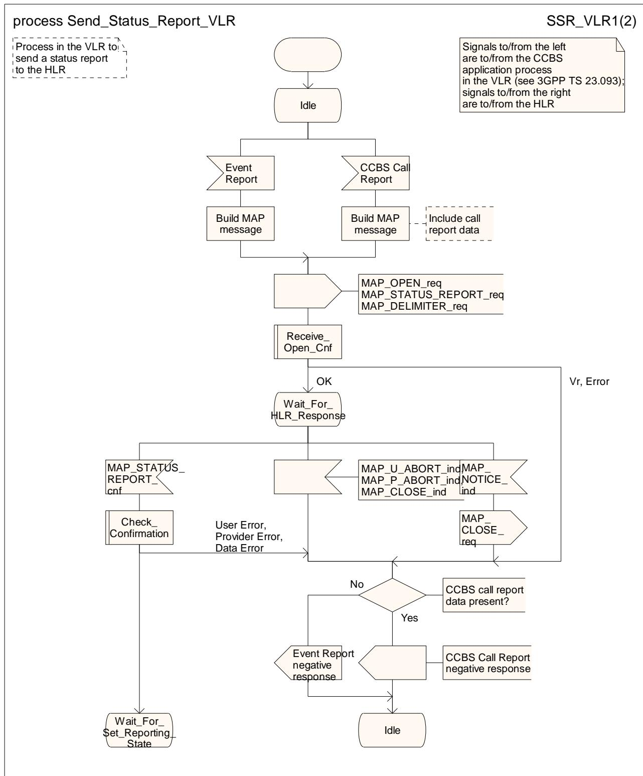
Figure 21.6/10 (sheet 1 of 2): Process Send\_Status\_Report\_VLR
