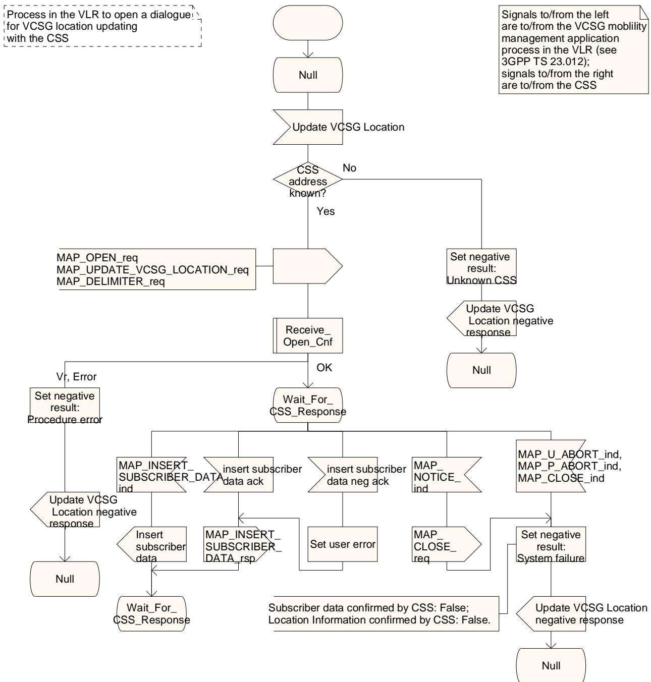
Figure 19.1.1A/2 (sheet 1 of 2): Process Update\_VCSG\_Location\_VLR
