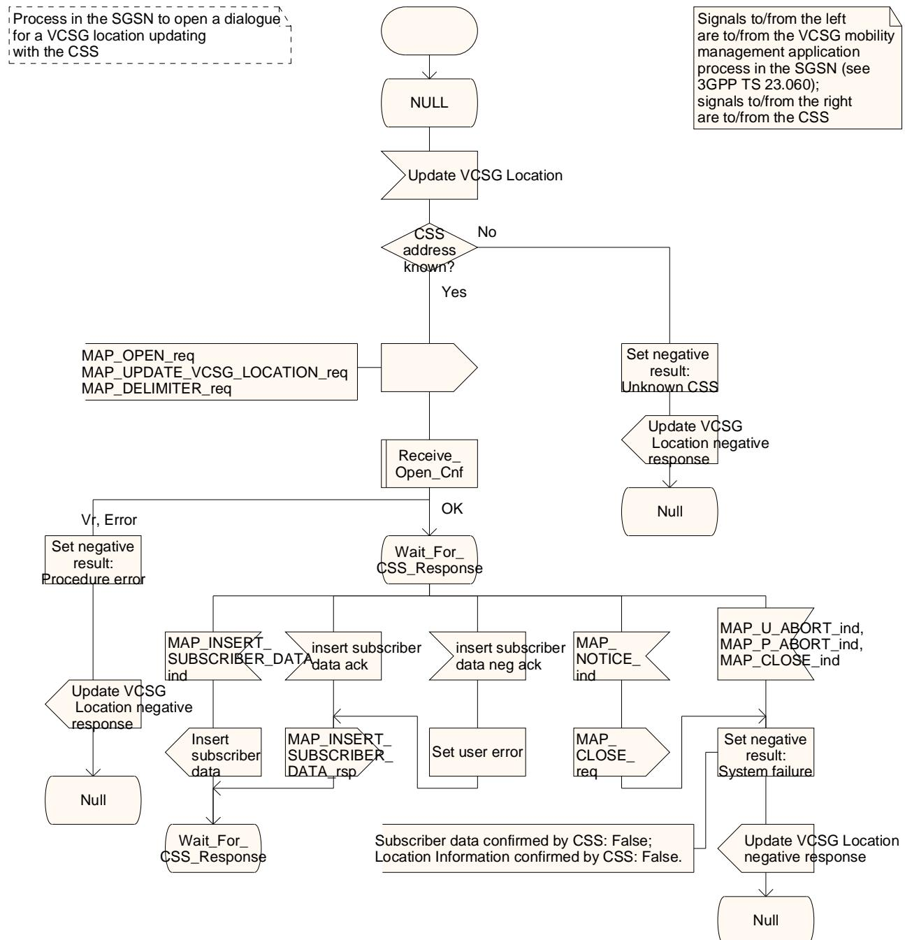
Figure 19.1.1A/3 (sheet 1 of 2): Process Update\_VCSG\_Location\_SGSN
