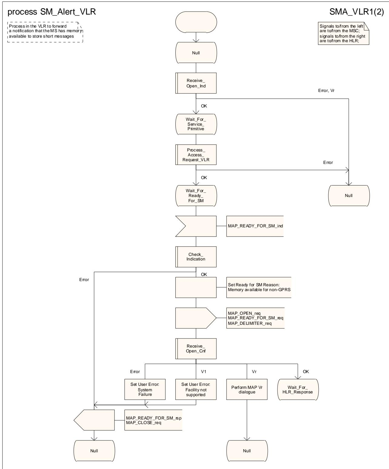
**Figure 23.4/5 (sheet 1 of 2): Procedure SM\_Alert\_VLR**
