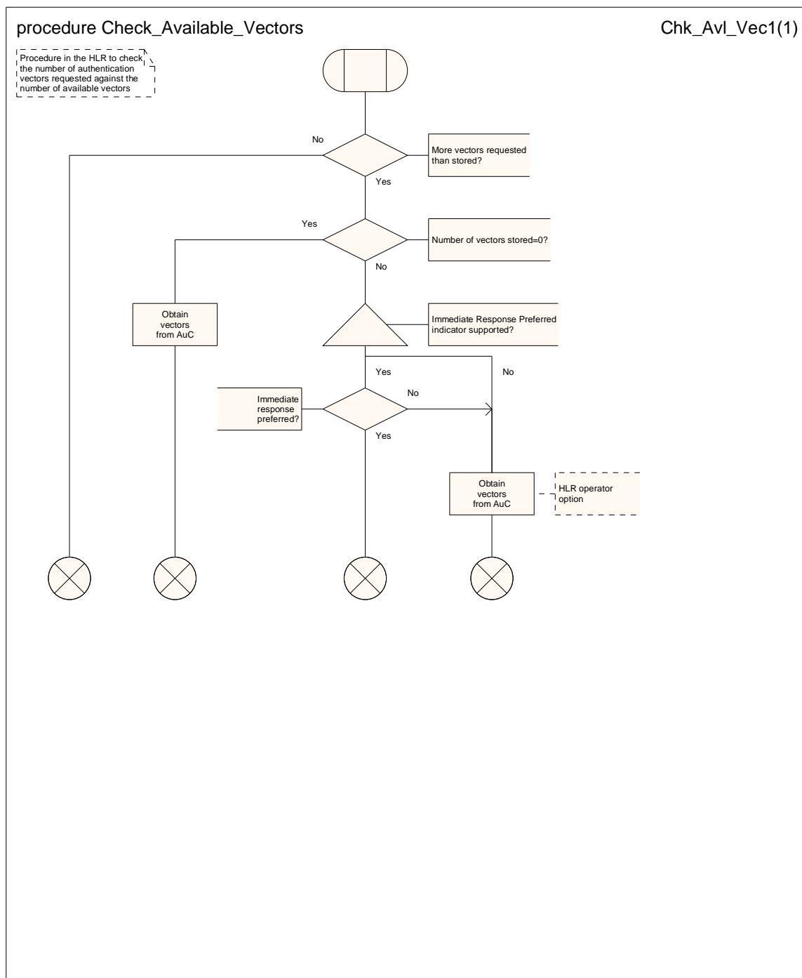
Figure 25.5/7: Procedure Check\_Available\_Vectors
