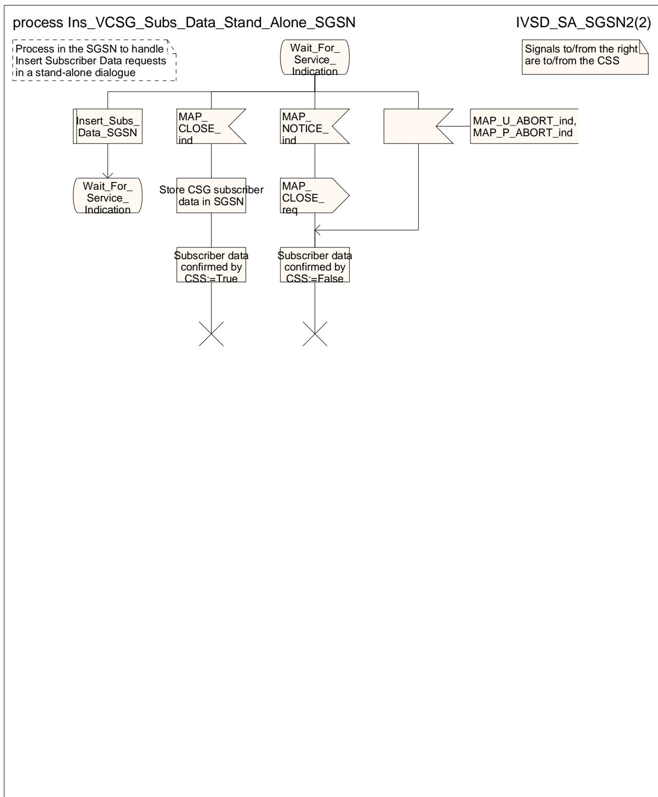
Figure 20.3A/10 (sheet 2 of 2): Process Ins\_VCSG\_Subs\_Data\_Stand\_Alone\_SGSN
