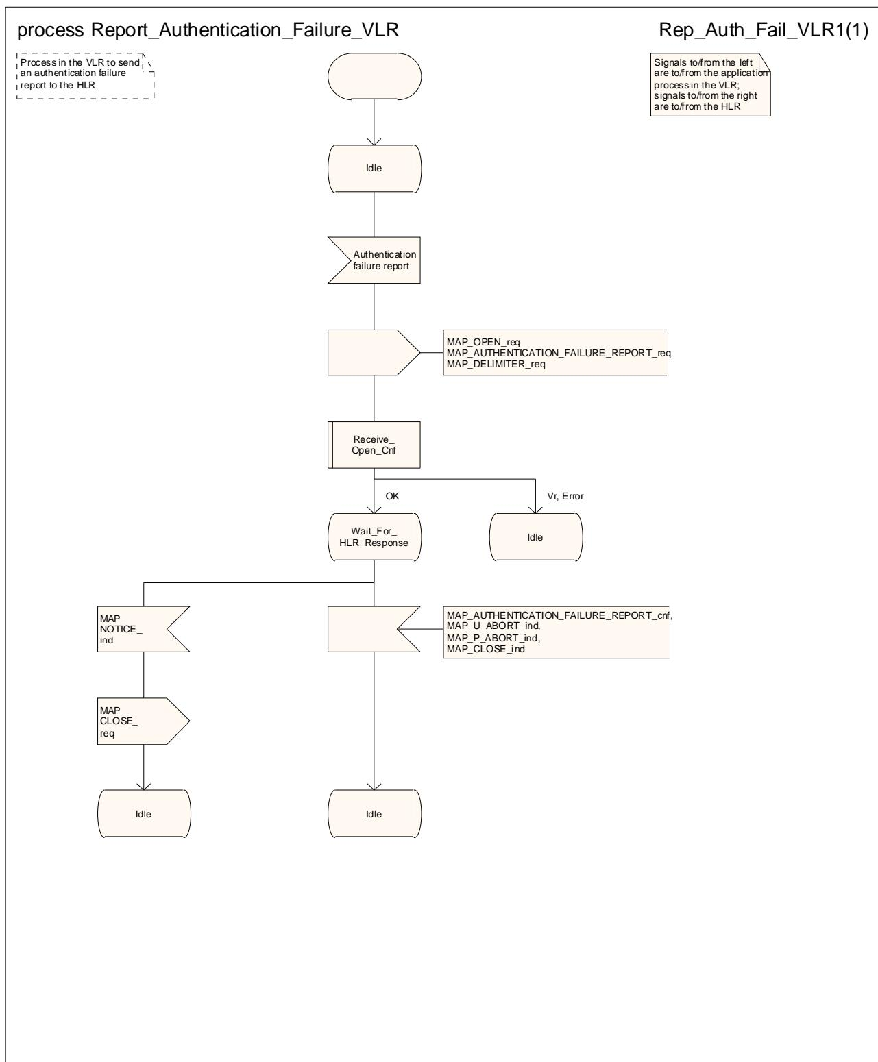
Figure 25.5/9: Process Report\_Authentication\_Failure\_VLR
