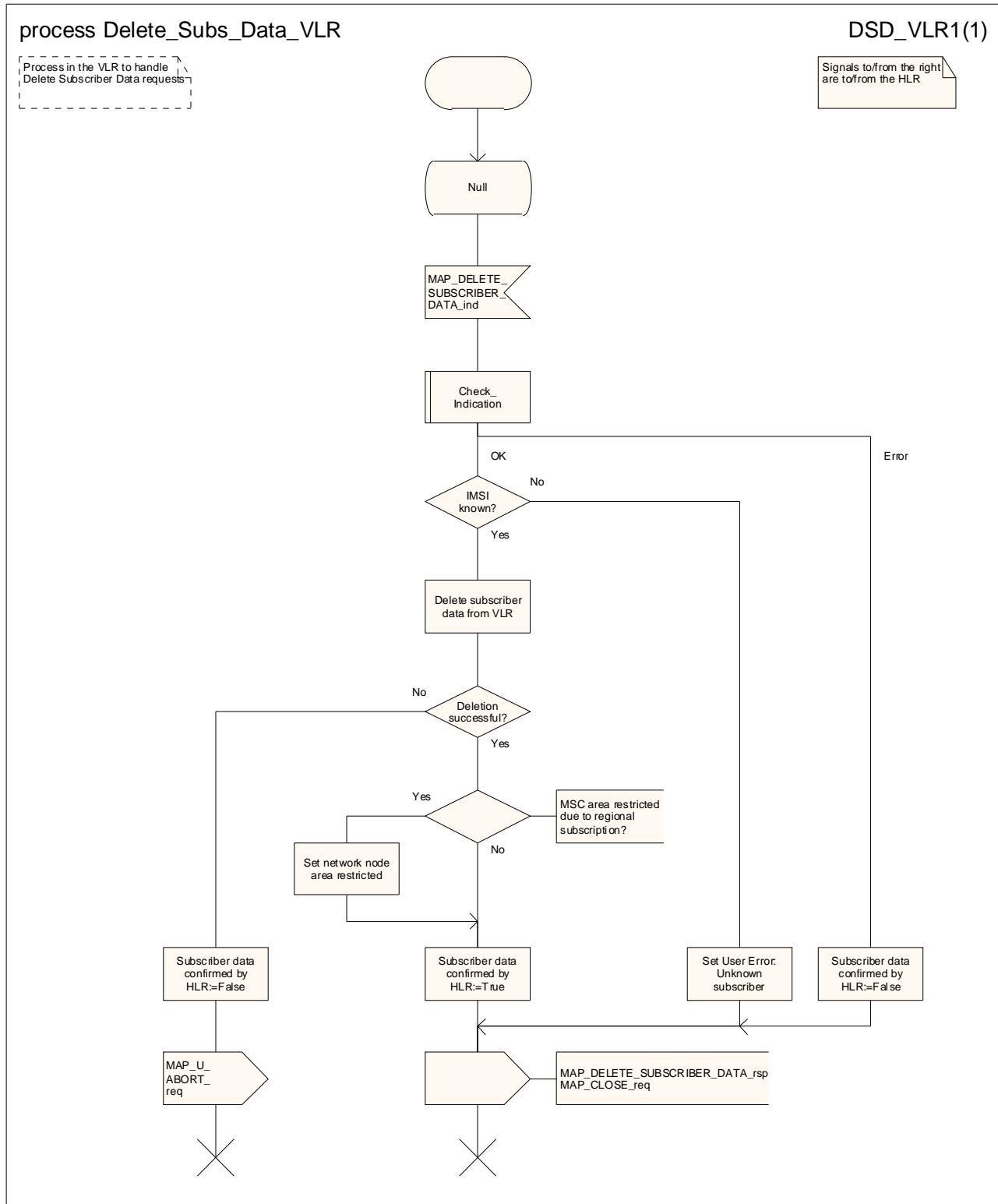
Figure 20.3/10: Process Delete\_Subs\_Data\_VLR
