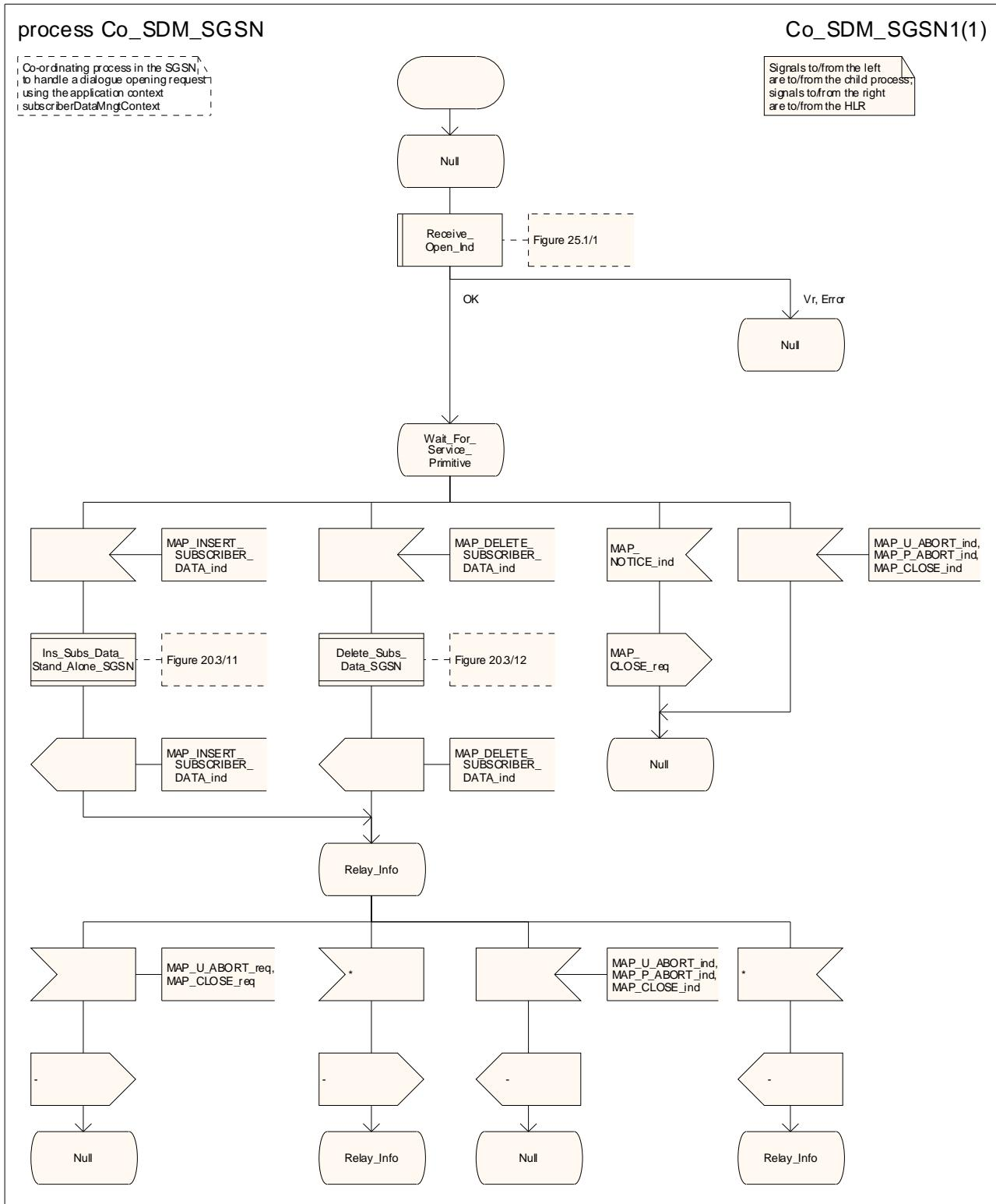
Figure 20.1/4: Process Co\_SDM\_SGSN
