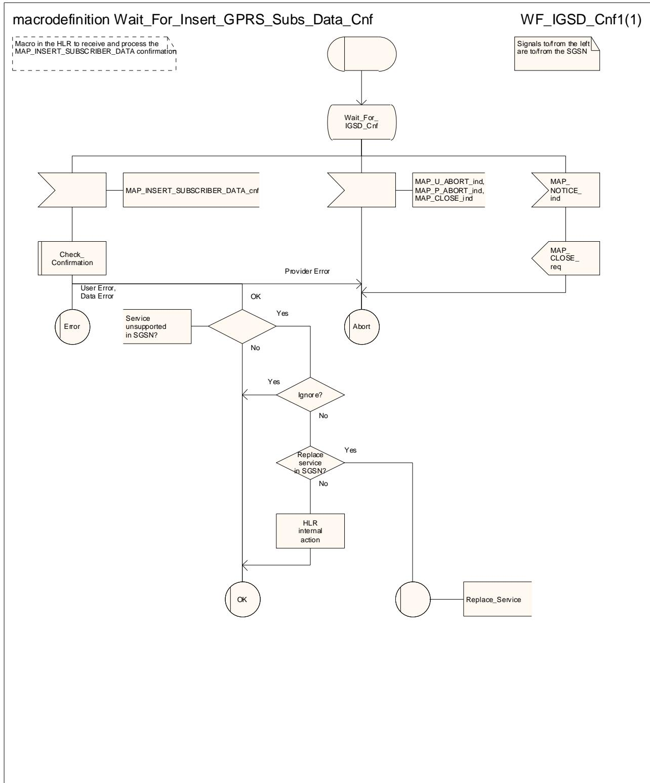
Figure 25.7/6: Macro Wait\_for\_Insert\_GPRS\_Subs\_Data\_Cnf
