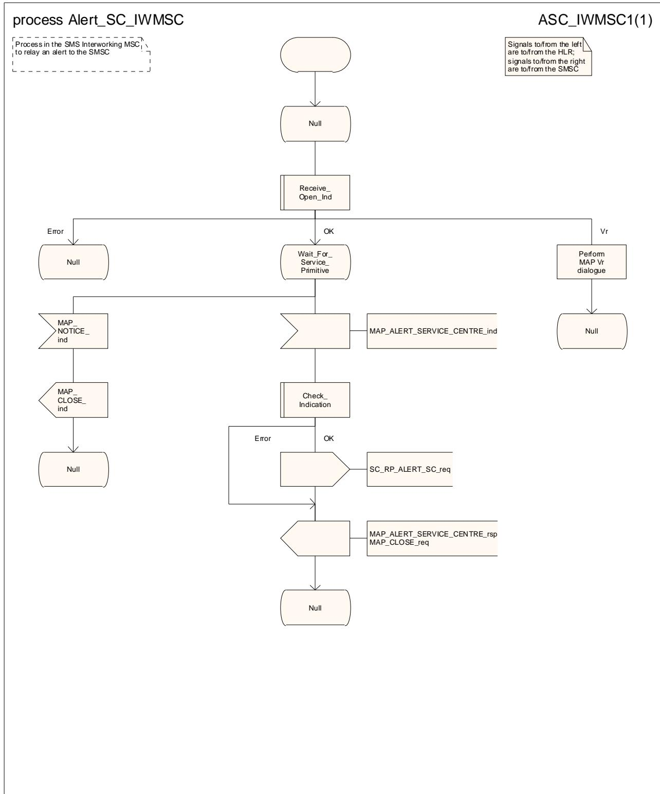
**Figure 23.4/8: Process Alert\_SC\_IWMSC**
