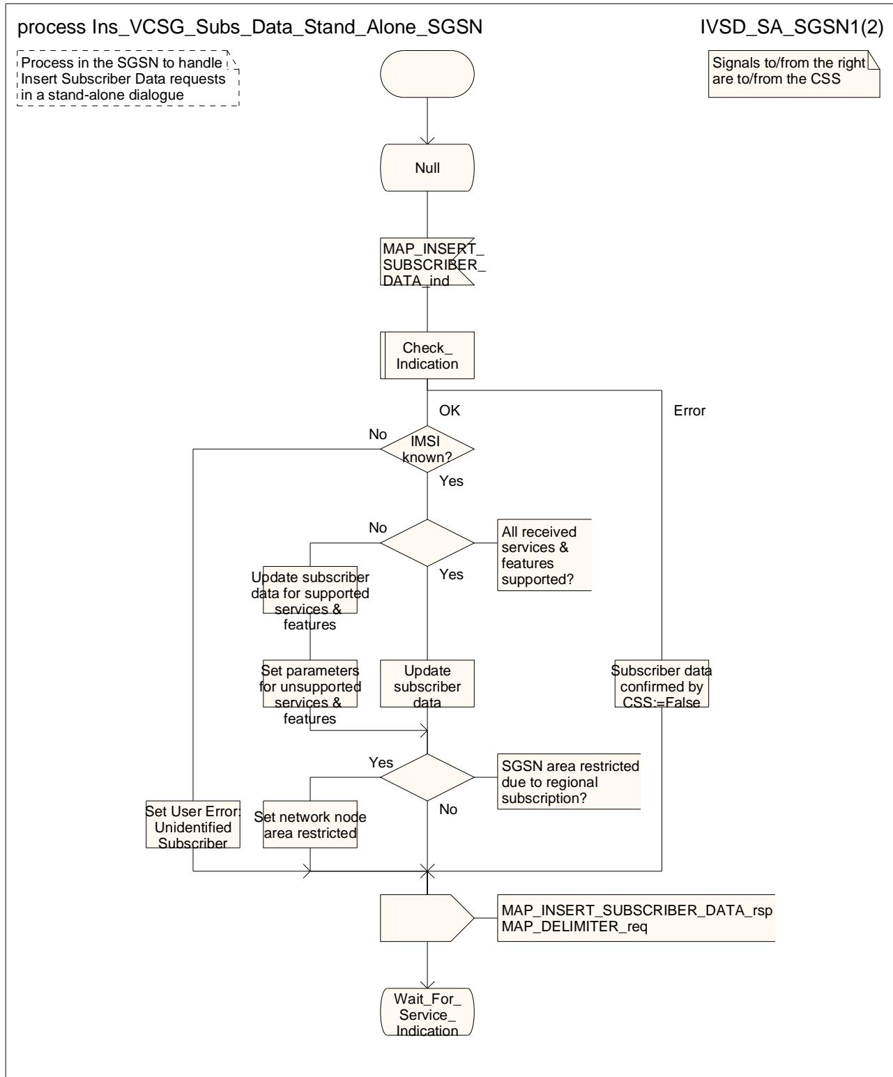
Figure 20.3A/10 (sheet 1 of 2): Process Ins\_VCSG\_Subs\_Data\_Stand\_Alone\_SGSN
