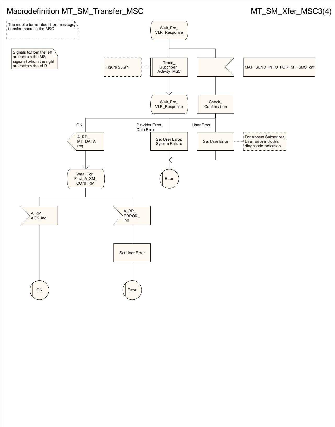
**Figure 23.3/7 (sheet 3 of 4): Macro MT\_SM\_Transfer\_MSC**
