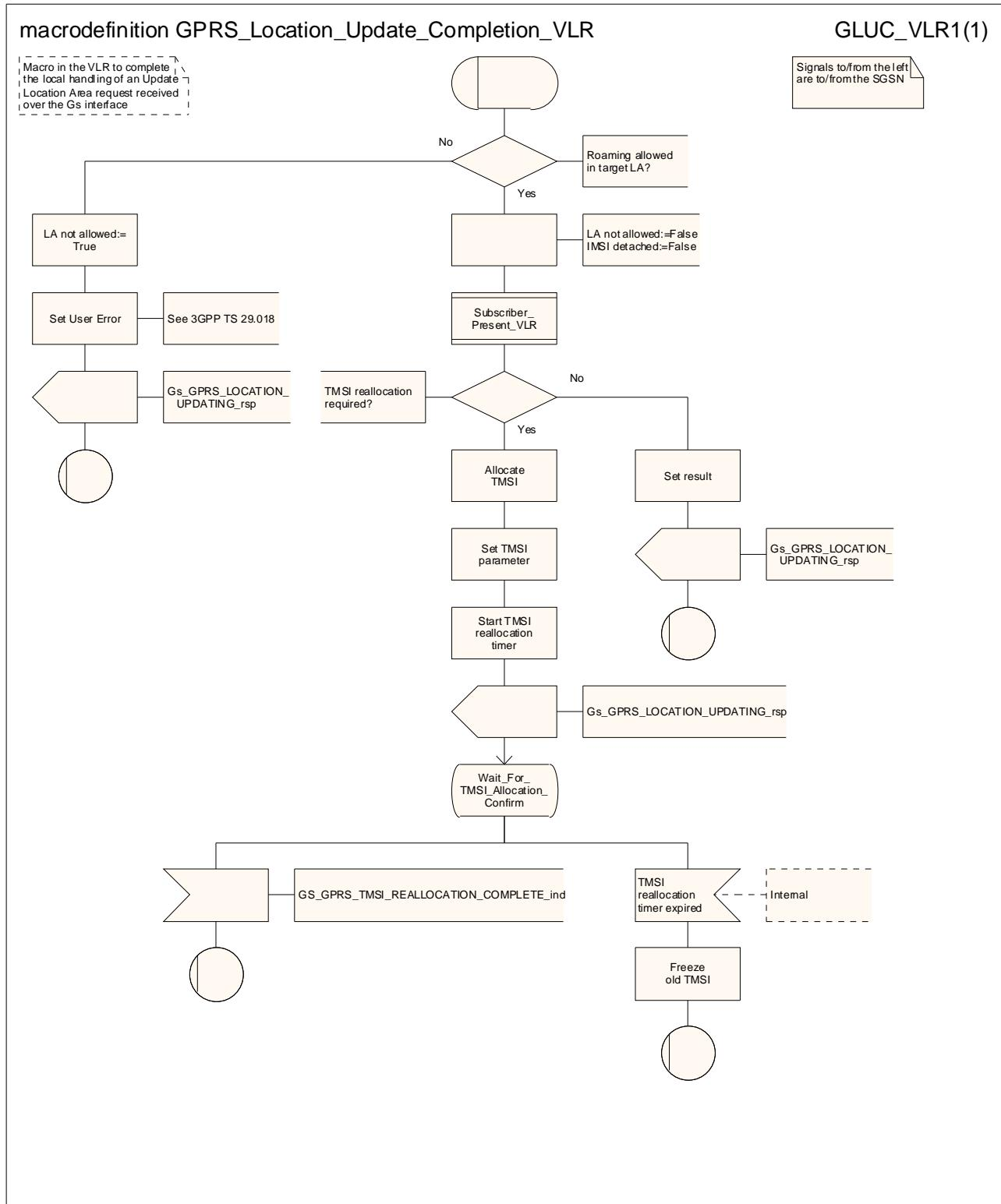
Figure 19.1.1/9: Macro GPRS\_Location\_Update\_Completion\_VLR
