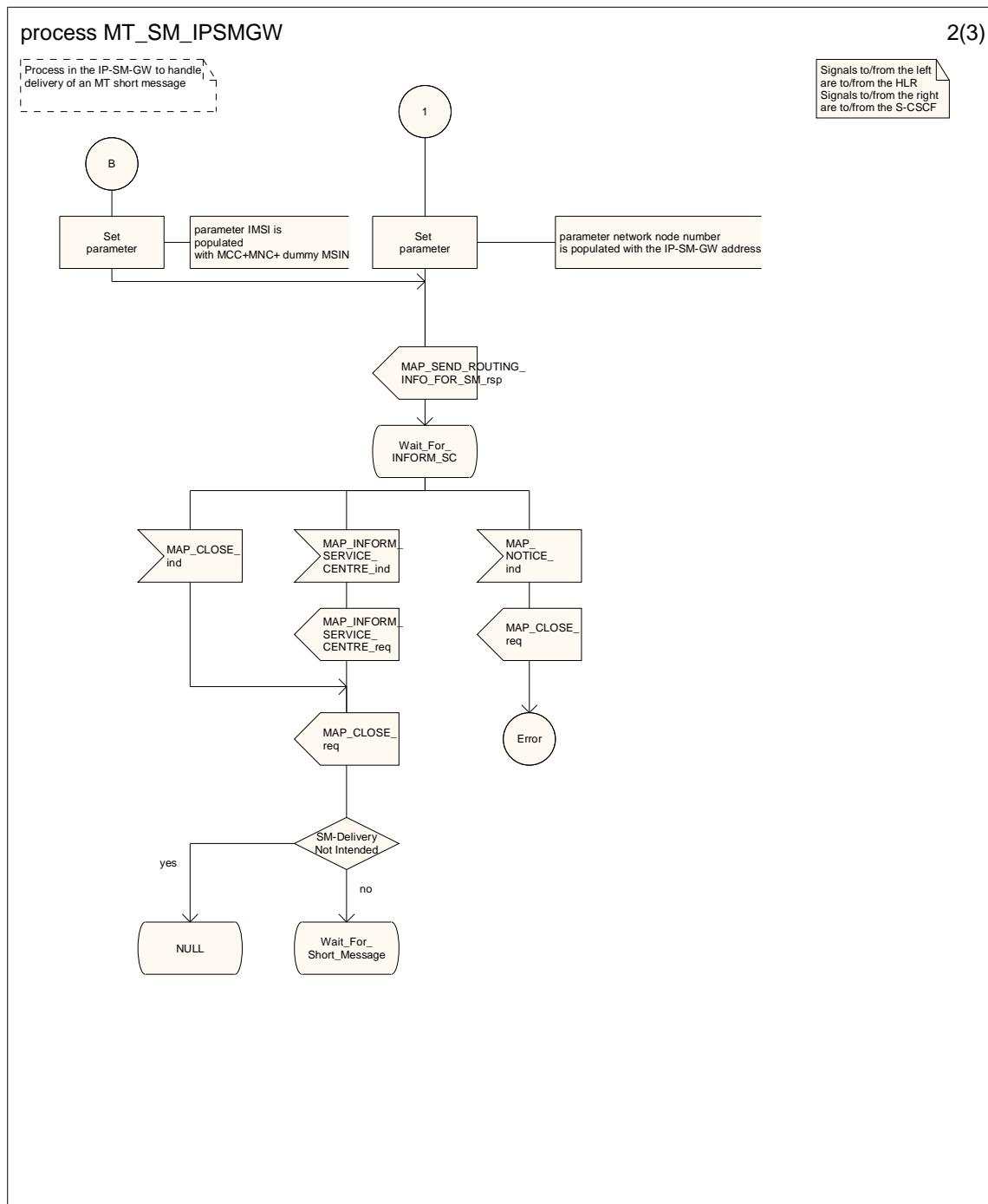
Figure 23.3/15 (sheet 2 of 3): Process MT\_SM\_IPSMGW
