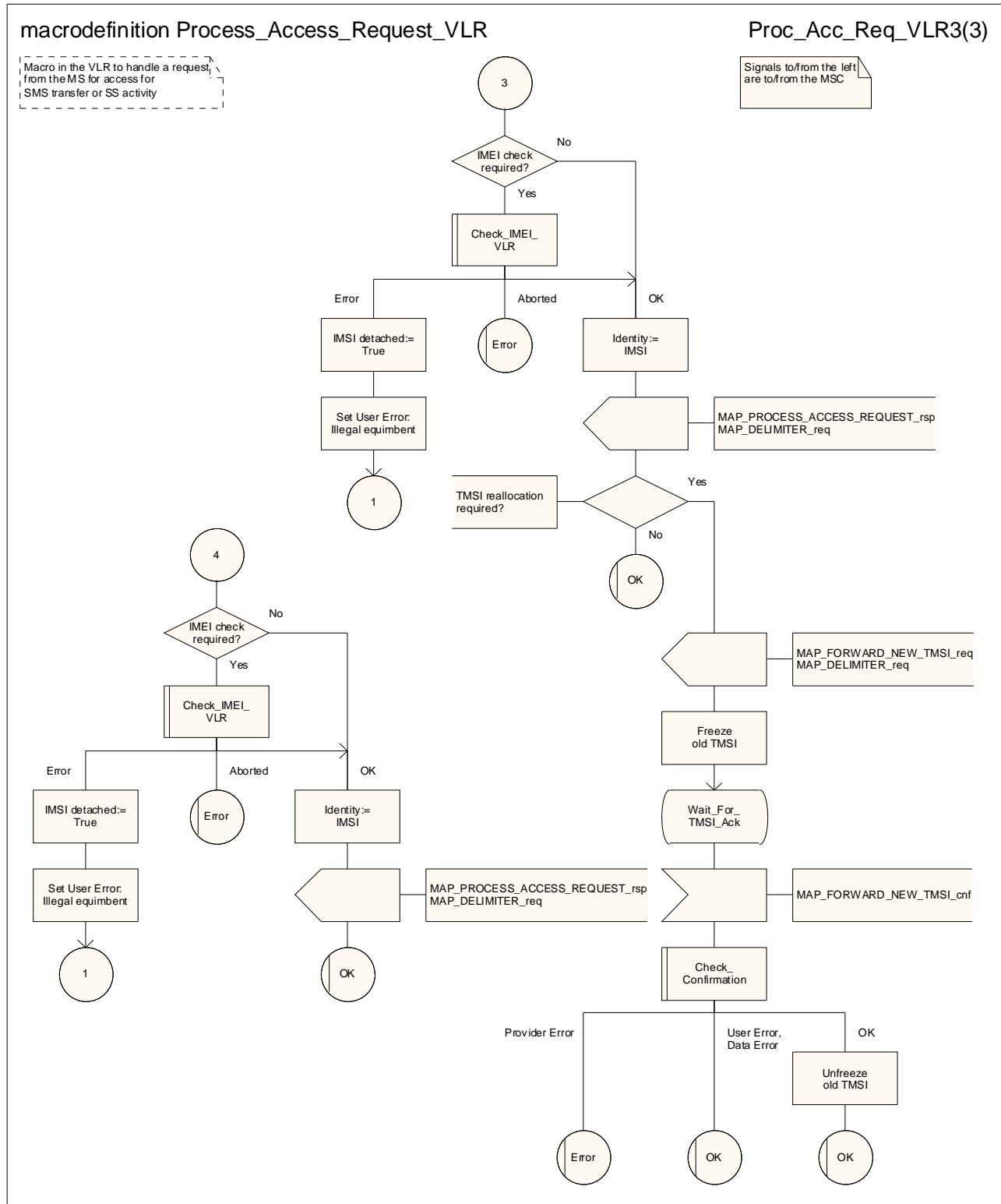
Figure 25.4/2 (sheet 3 of 3): Macro Process\_Access\_Request\_VLR
