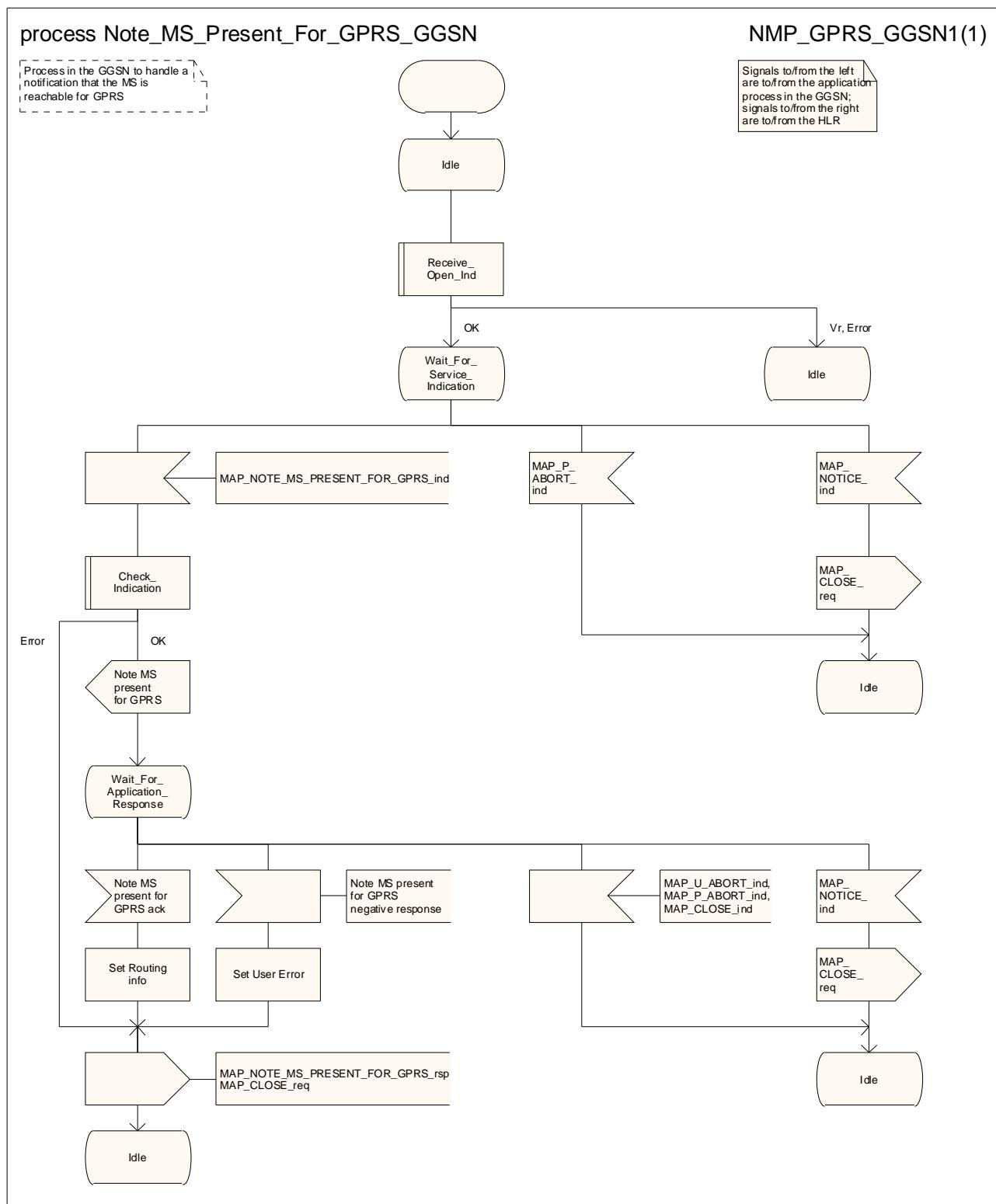
**Figure 24.3/2: Process Note\_MS\_Present\_For\_GPRS\_GGSN**
