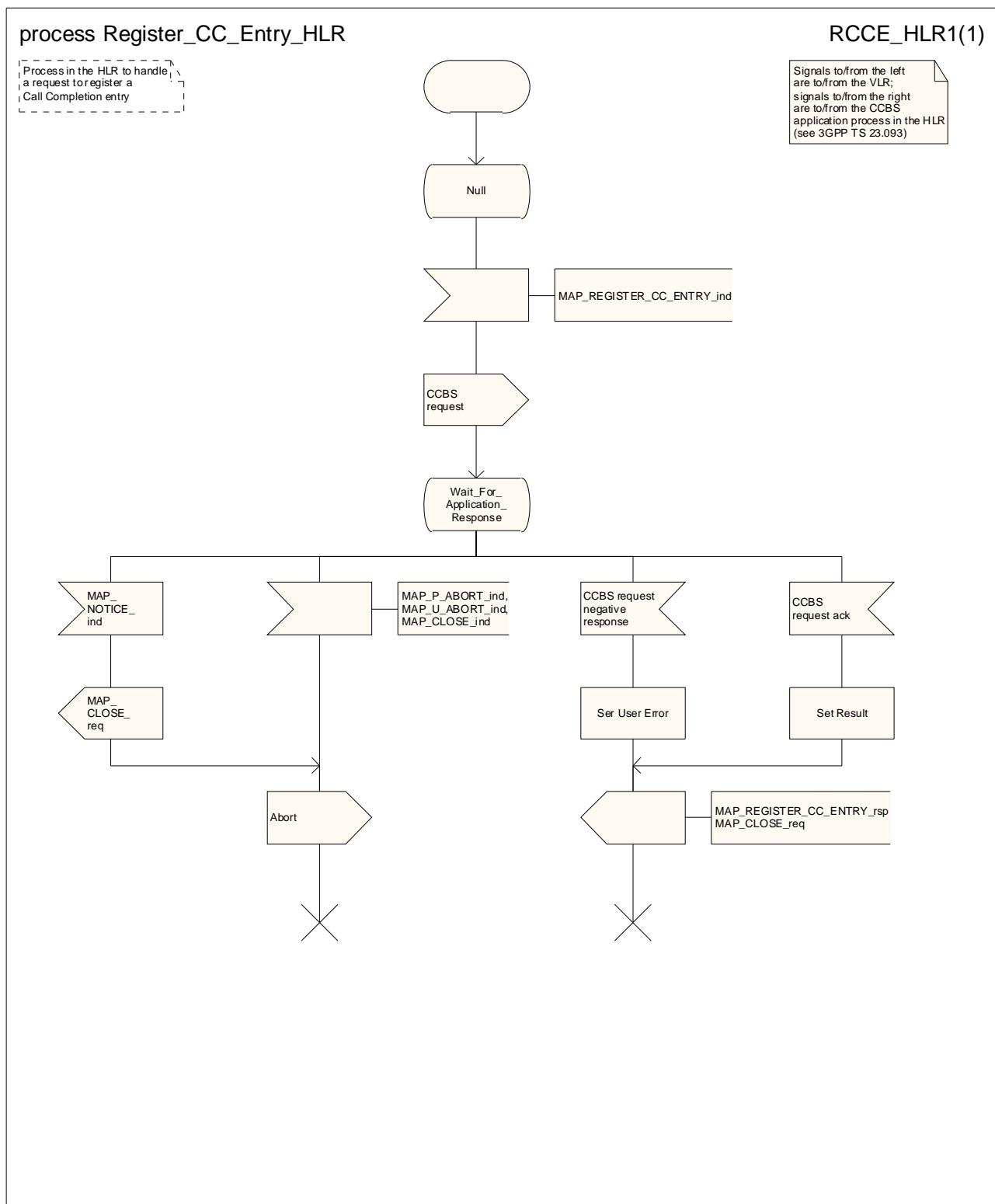
Figure 22.13.3/1: Process Register\_CC\_Entry\_HLR
