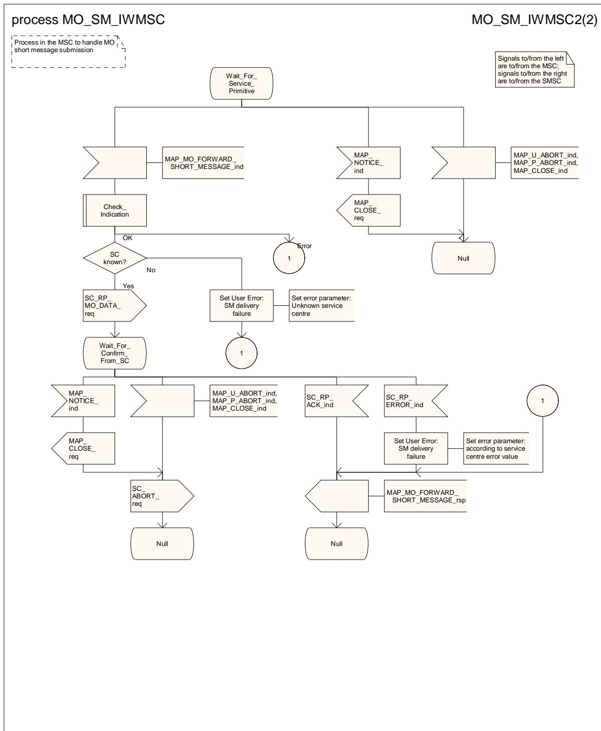
Figure 23.2/5 (sheet 2 of 2): Process MO\_SM\_IWMSC
