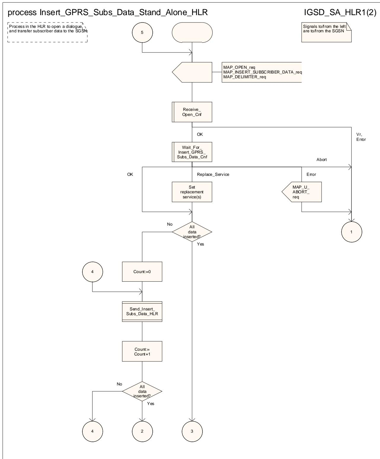
Figure 25.7/4 (sheet 1 of 2): Process Insert\_GPRS\_Subs\_Data\_Stand\_Alone\_HLR
