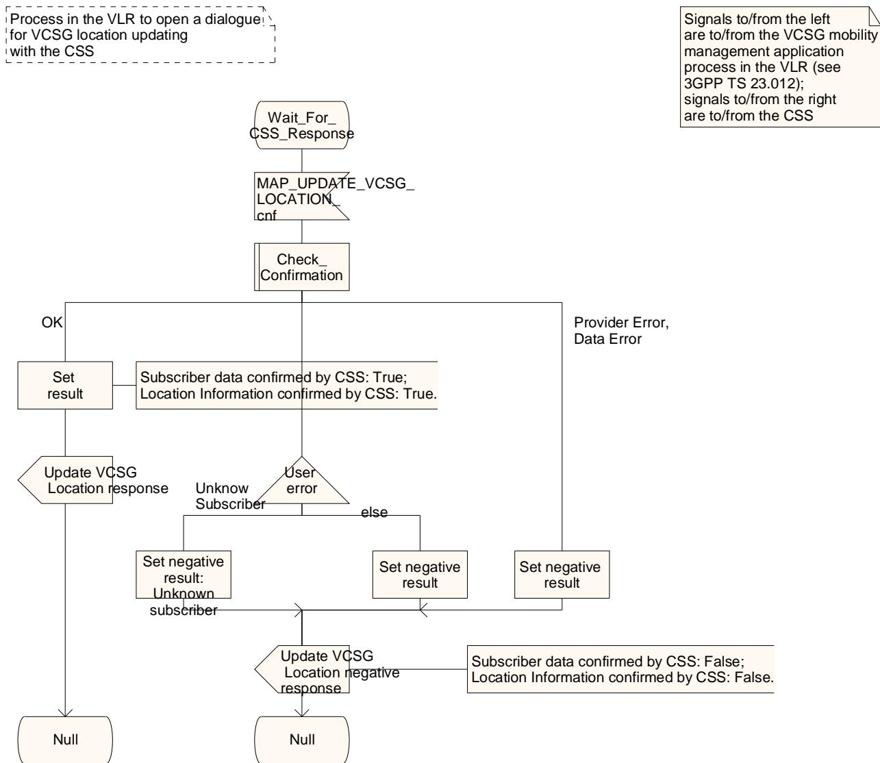
Figure 19.1.1A/2 (sheet 2 of 2): Process Update\_VCSG\_Location\_VLR
