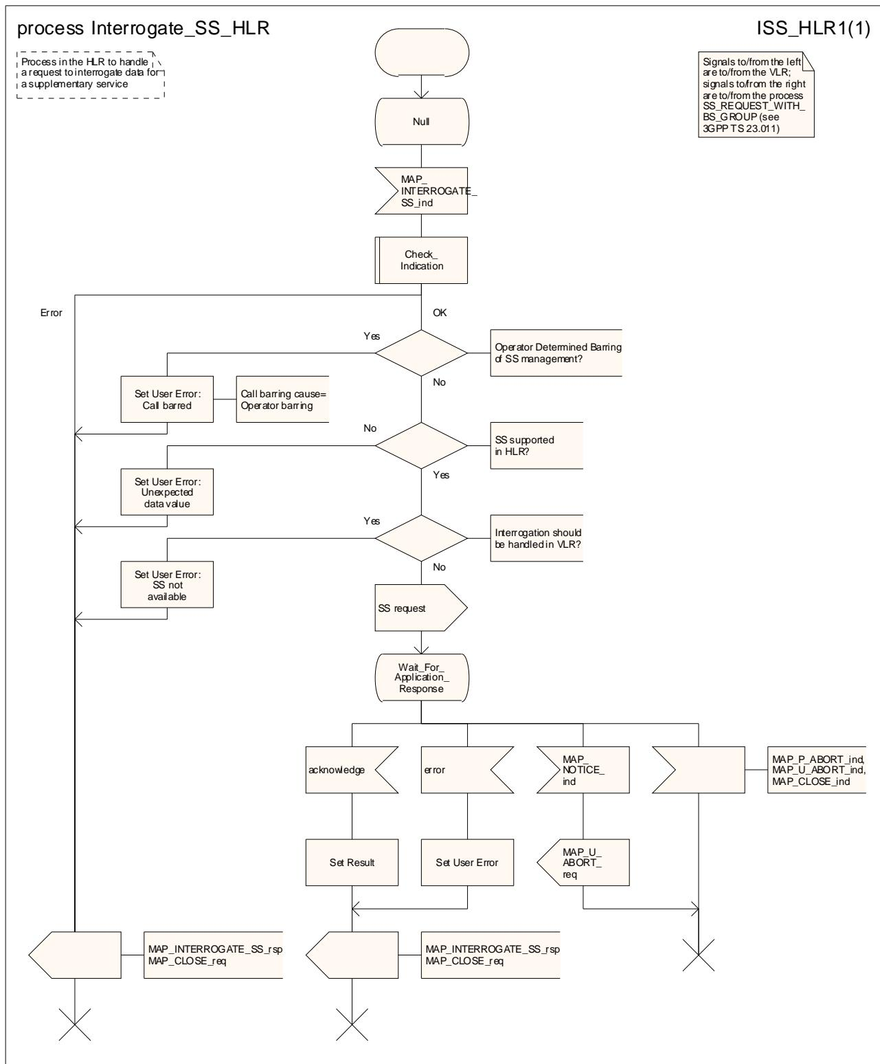
Figure 22.6.4/1: Process Interrogate\_SS\_HLR
