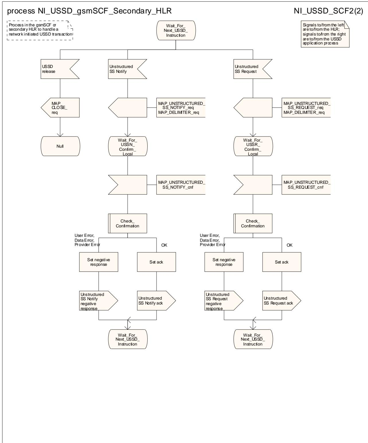
Figure 22.10.5/1 (sheet 2 of 2): Process NW\_Init\_USSD\_gsmSCF\_Secondary\_HLR
