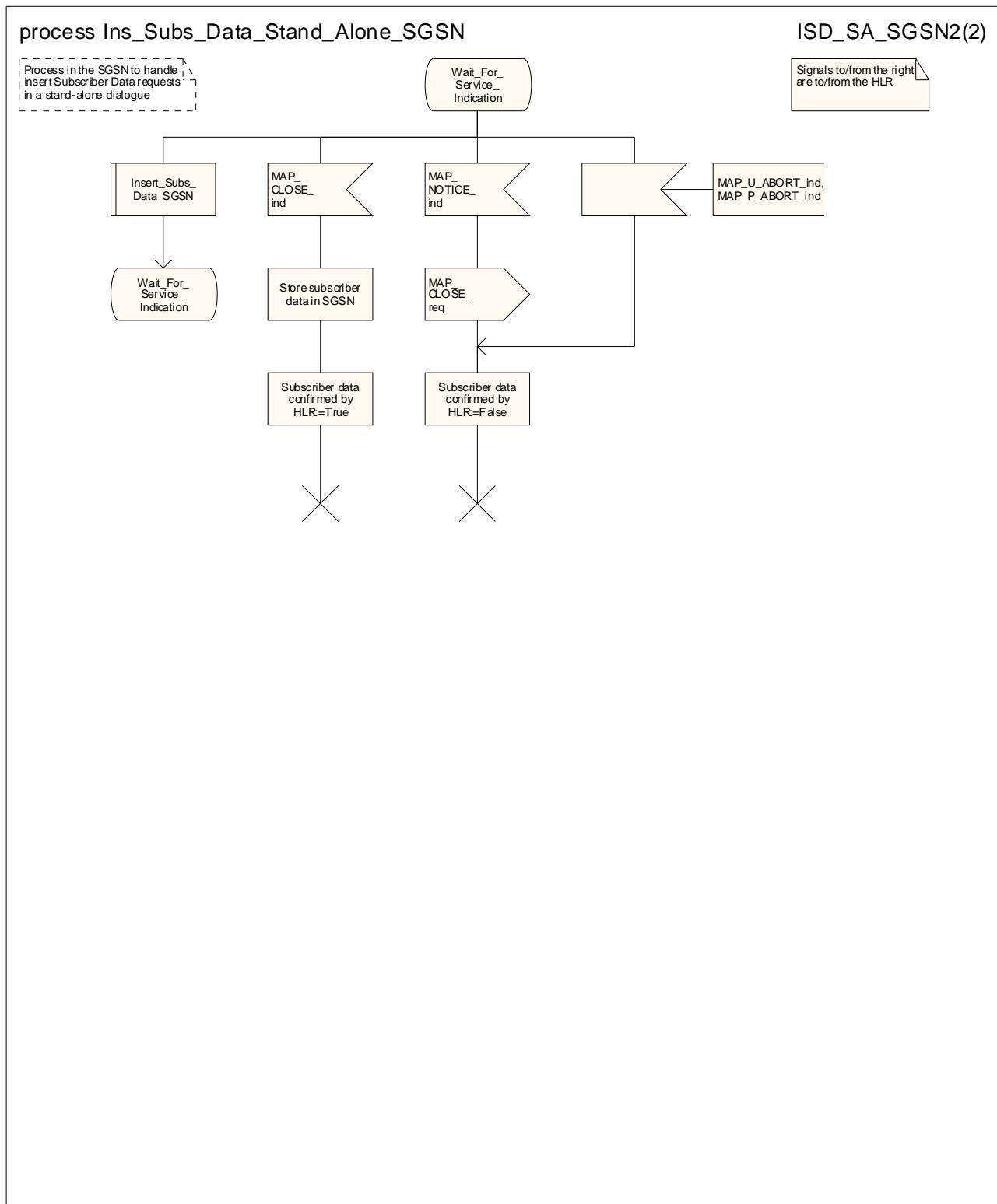
Figure 20.3/11 (sheet 2 of 2): Process Ins\_Subs\_Data\_Stand\_Alone\_SGSN
