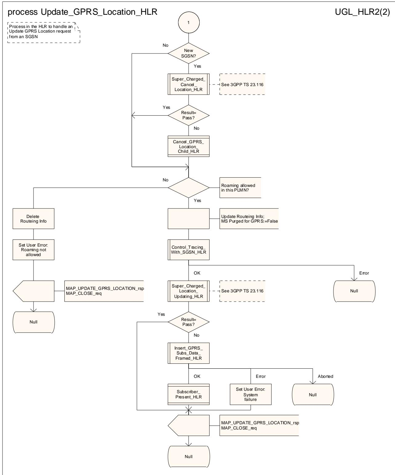
Figure 19.1.1/14 (sheet 2 of 2): Process Update\_GPRS\_Location\_HLR
