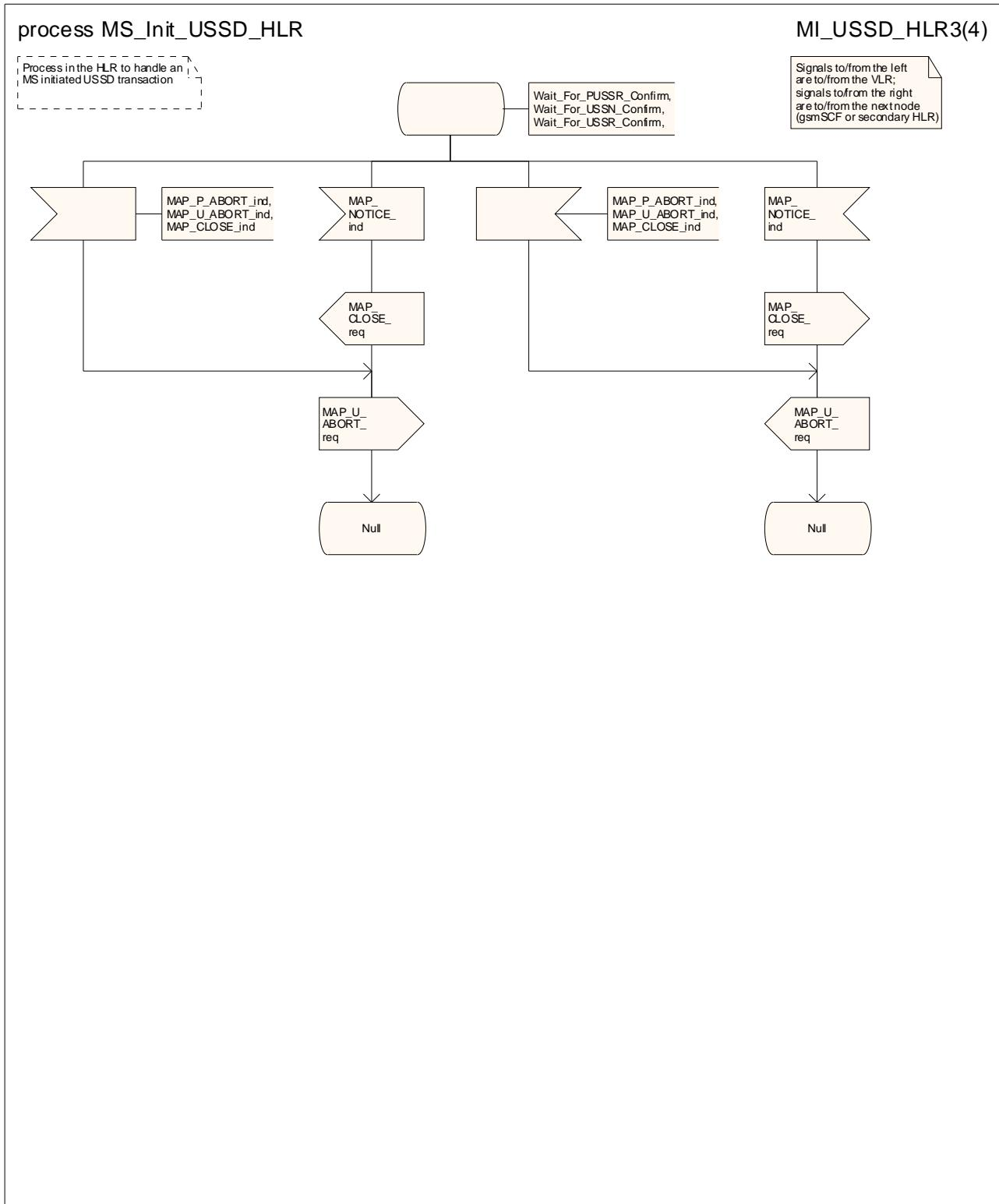
Figure 22.9.4/1 (sheet 3 of 4): Process MS\_Init\_USSD\_HLR
