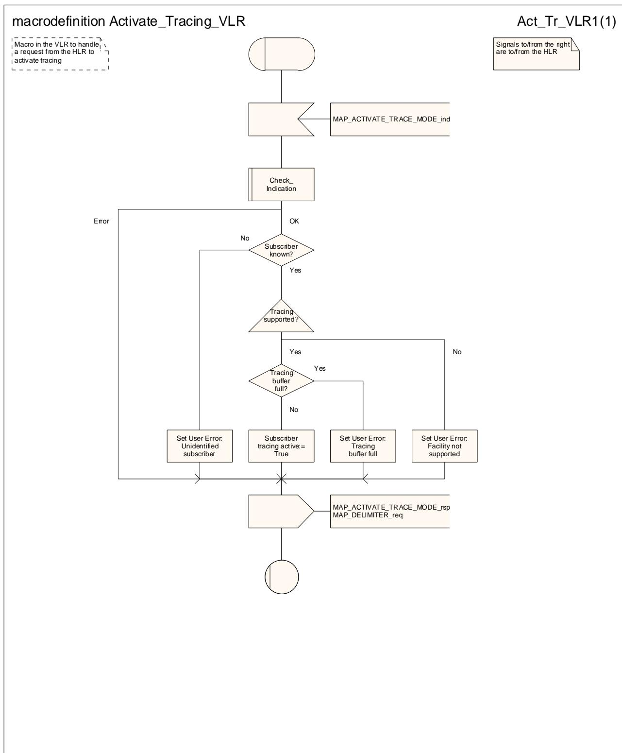
**Figure 25.9/4: Macro Activate\_Tracing\_VLR**
