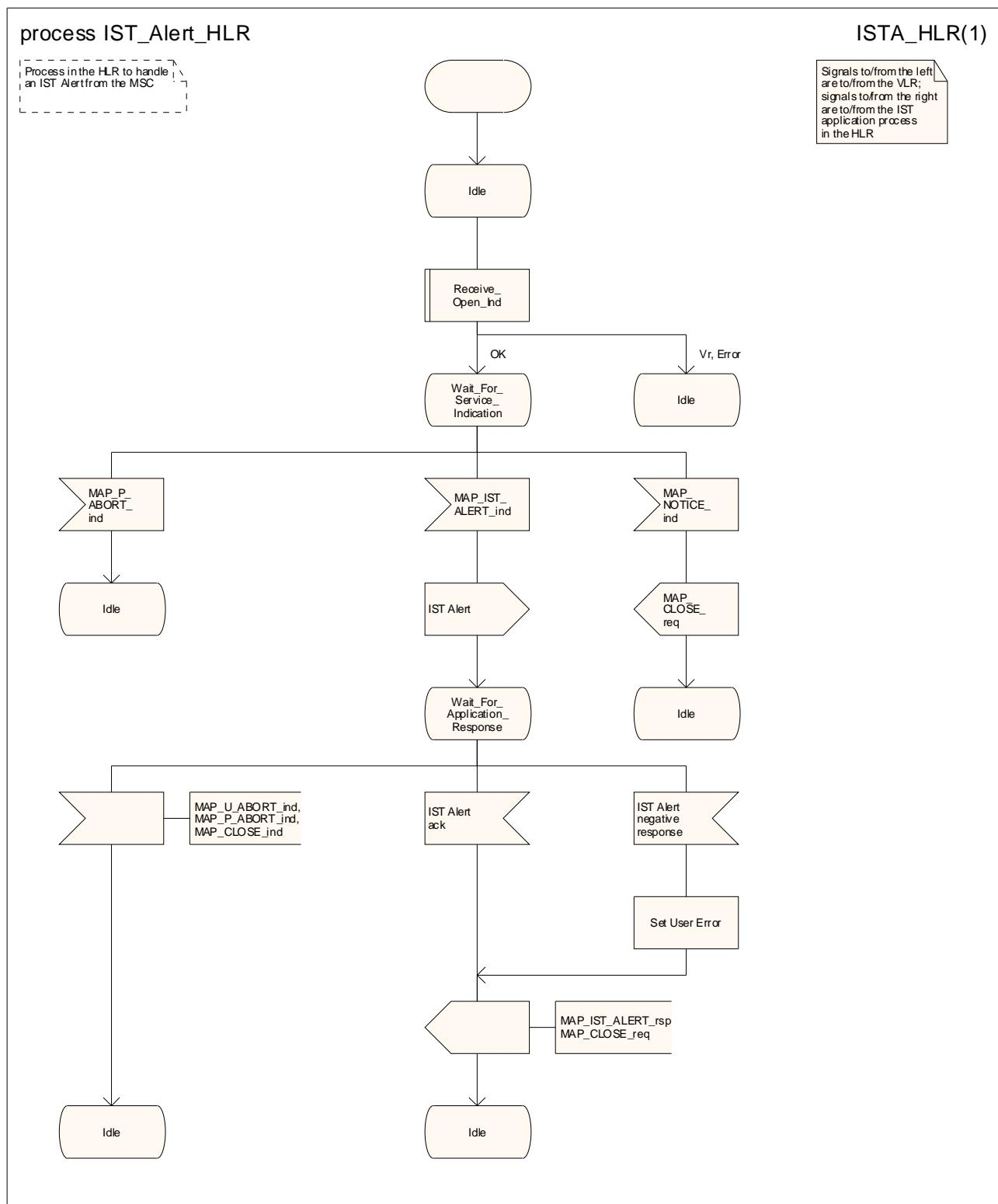
Figure 21.9/4: Process IST\_Alert\_HLR
