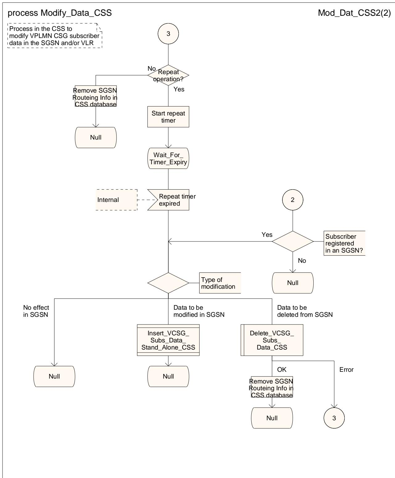
Figure 20.3A/6 (sheet 2 of 2): Process Modify\_Data\_CSS
