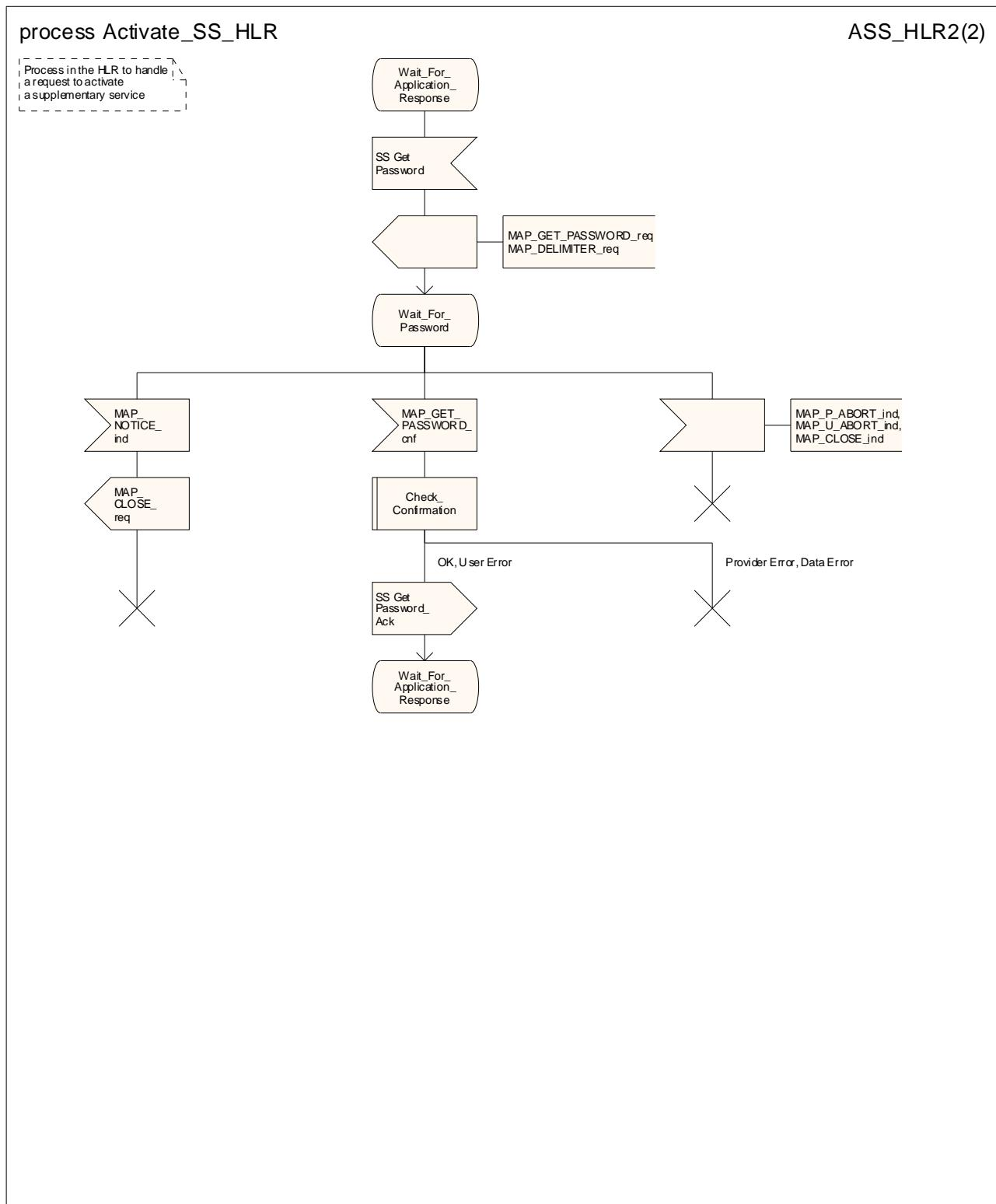
Figure 22.4.4/1 (sheet 2 of 2): Process Activate\_SS\_HLR
