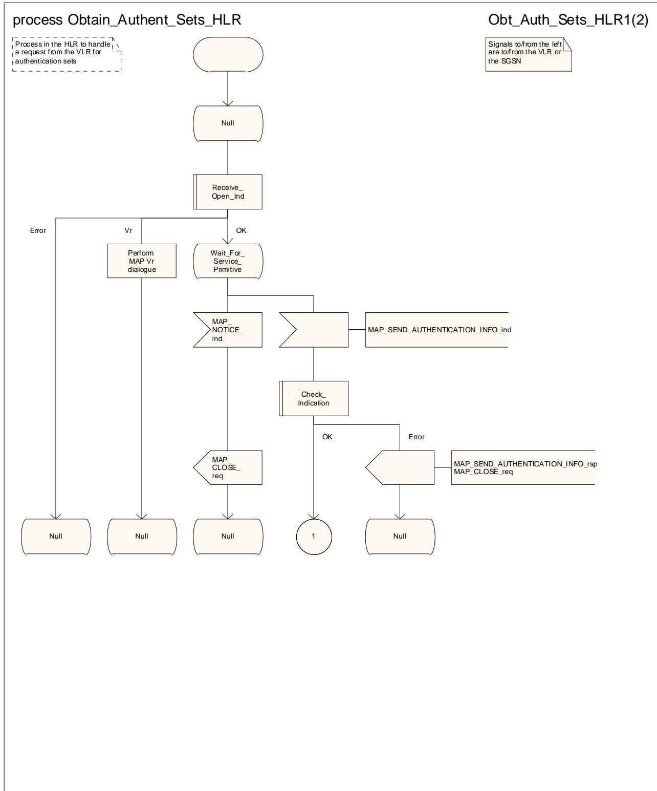
Figure 25.5/6 (sheet 1 of 2): Process Obtain\_Authent\_Sets\_HLR
