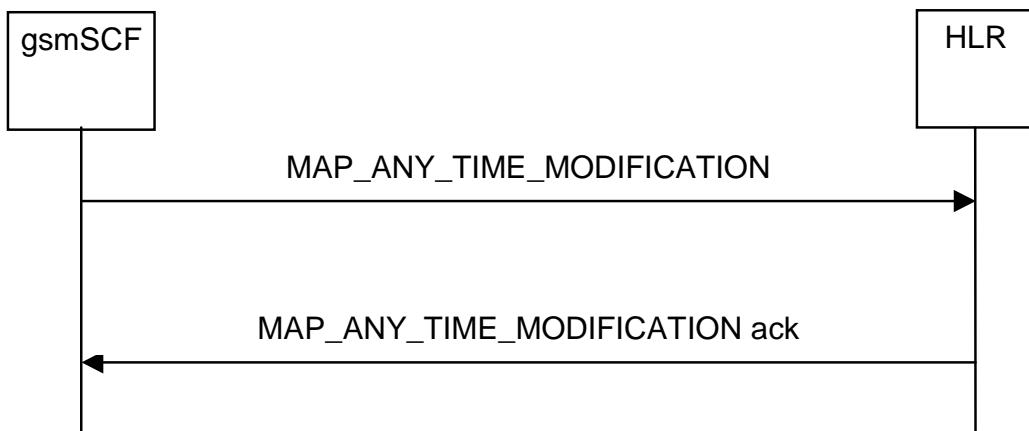
**Figure 24A.3/1: Message flow for any time modification**
