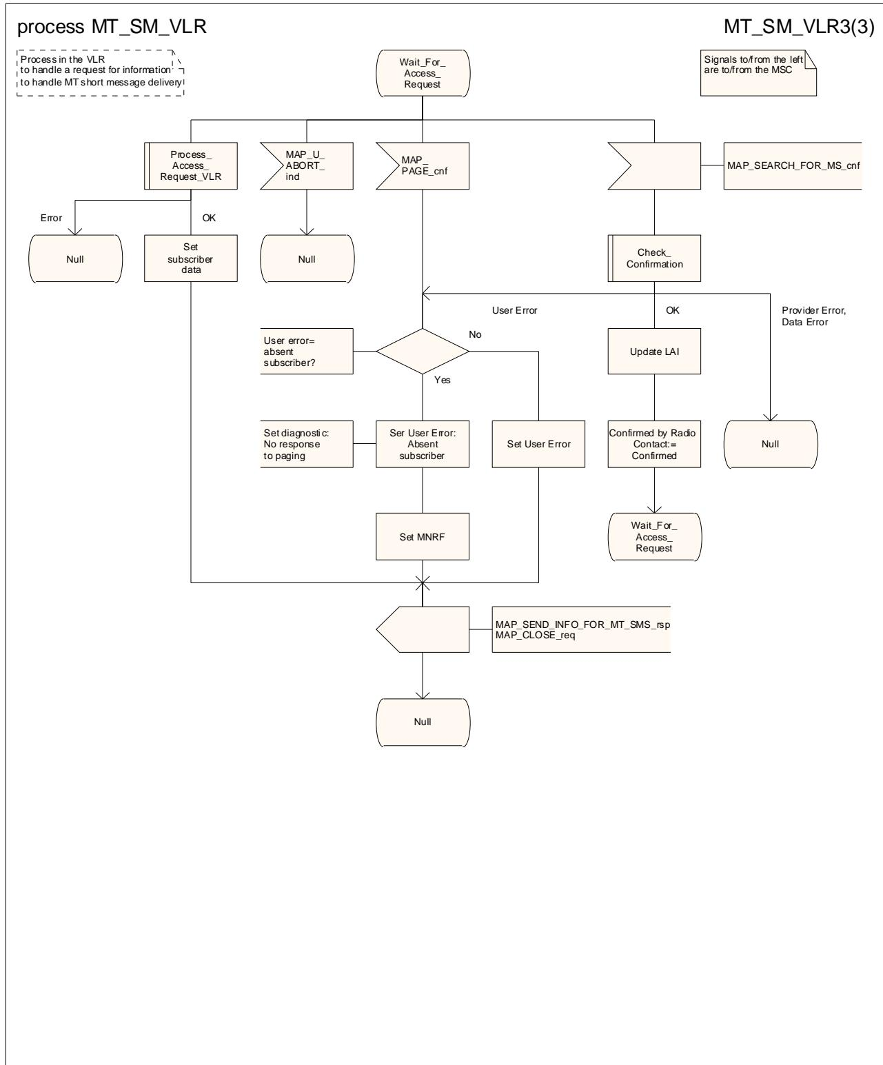
Figure 23.3/9 (sheet 3 of 3): Process MT\_SM\_VLR
