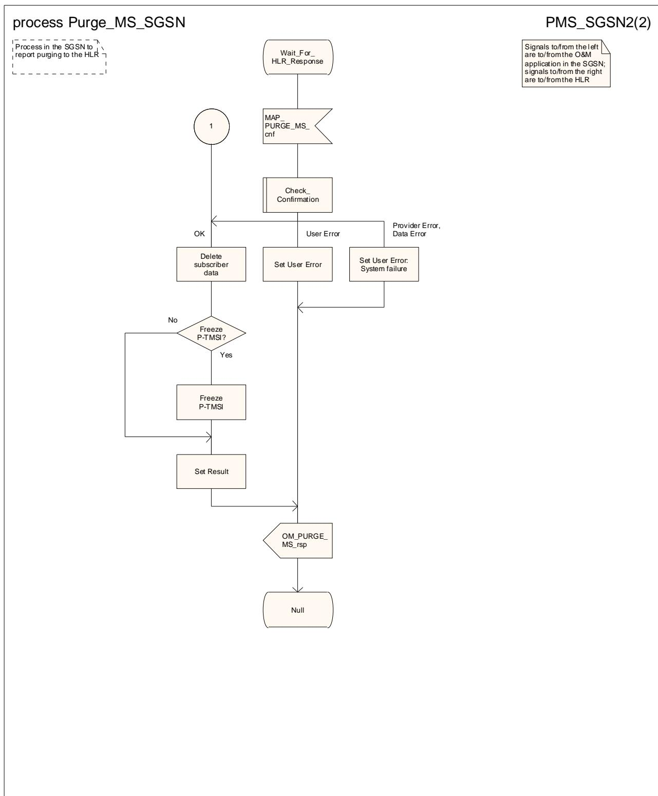
Figure 19.1.4/4 (sheet 2 of 2): Process Purge\_MS\_SGSN
