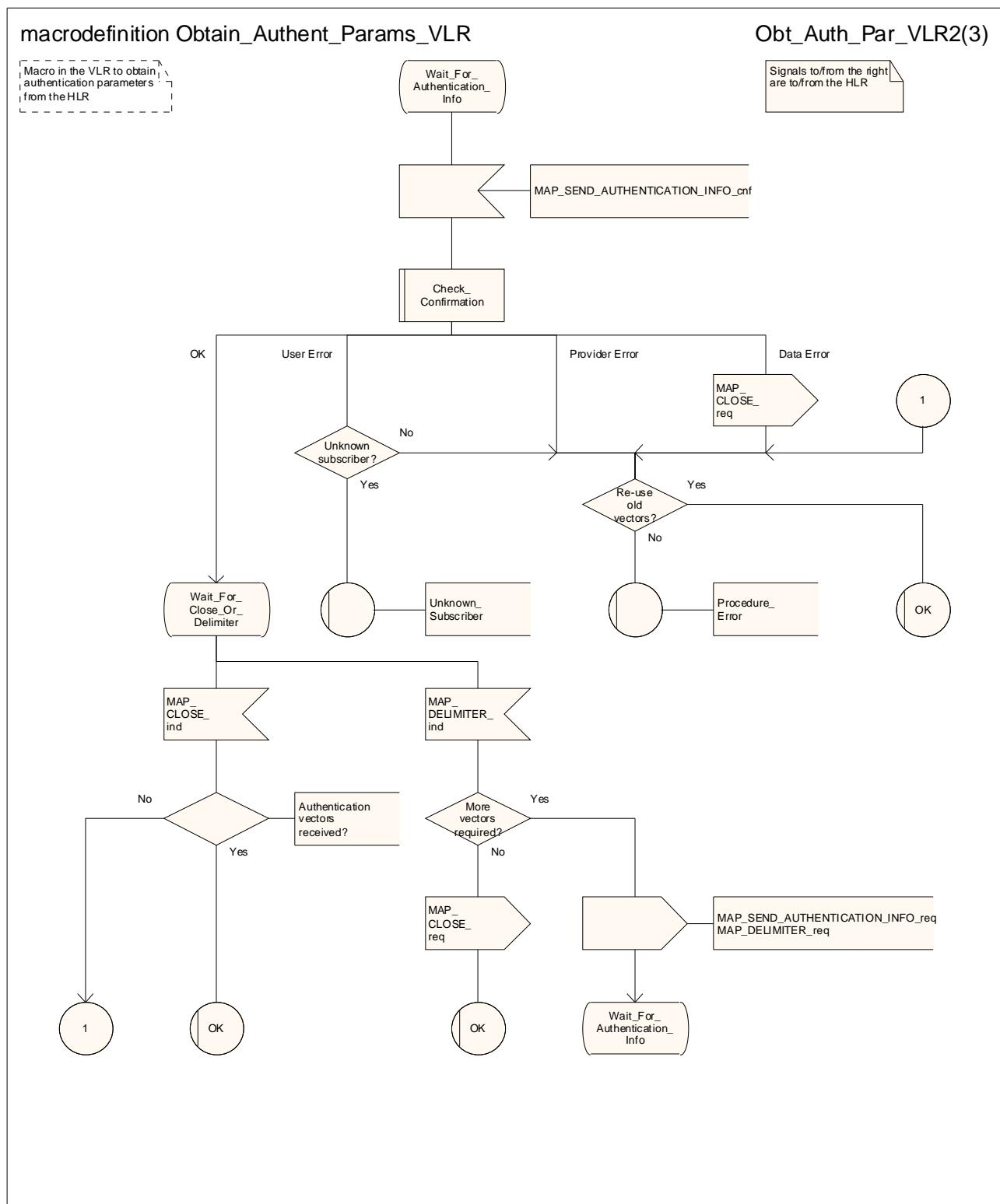
Figure 25.5/3 (sheet 2 of 3): Macro Obtain\_Authent\_Params\_VLR
