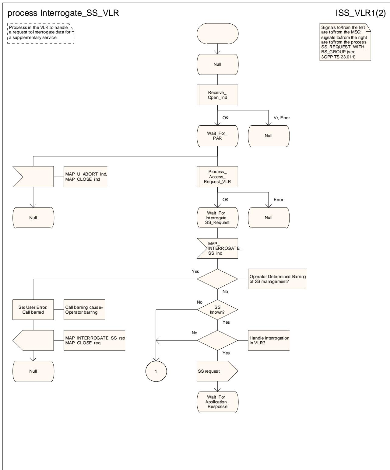
**Figure 22.6.3/1 (sheet 1 of 2): Process Interrogate\_SS\_VLR**
