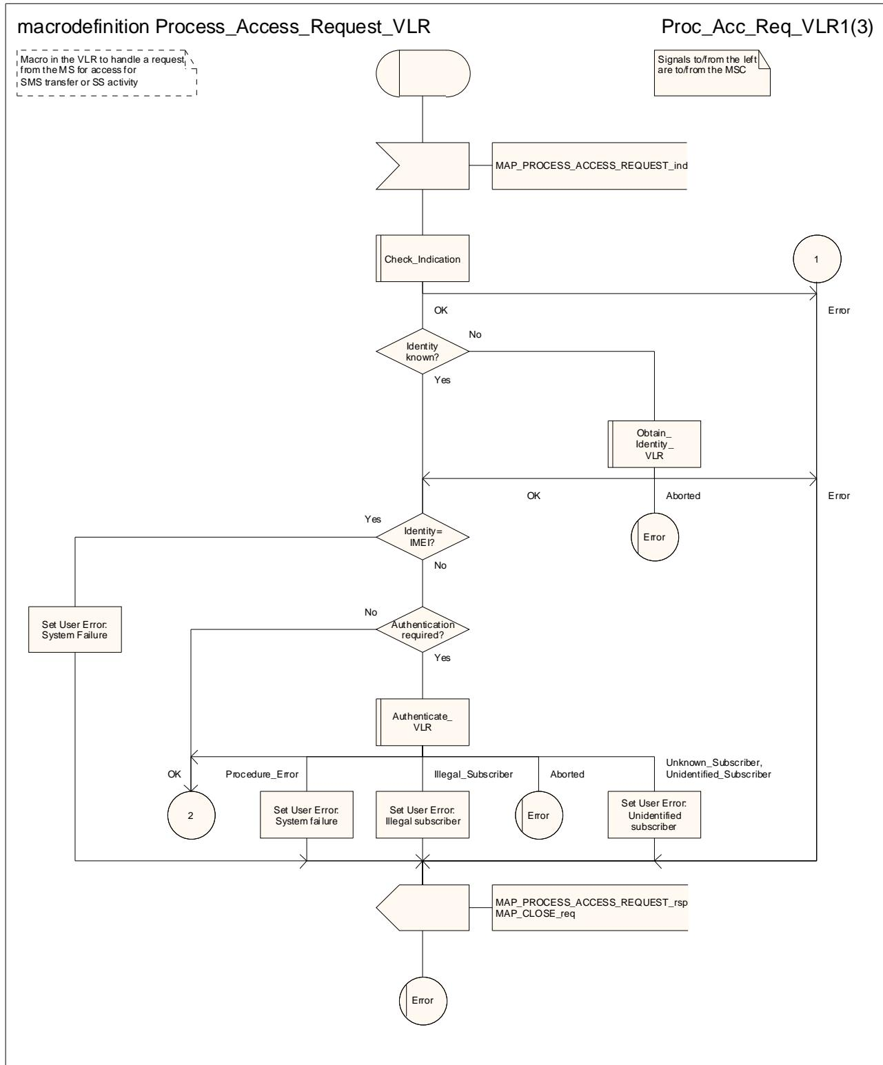
Figure 25.4/2 (sheet 1 of 3): Macro Process\_Access\_Request\_VLR
