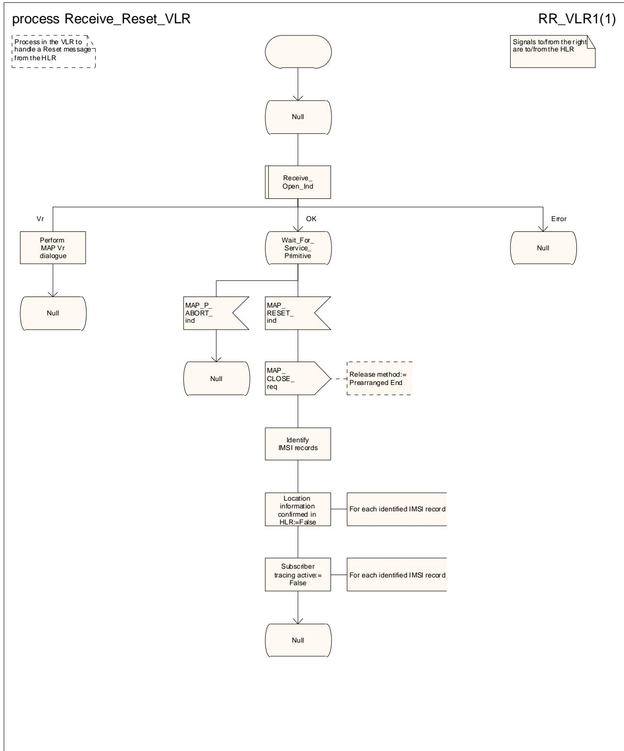
**Figure 19.3.2/6: Process Receive\_Reset\_VLR**
