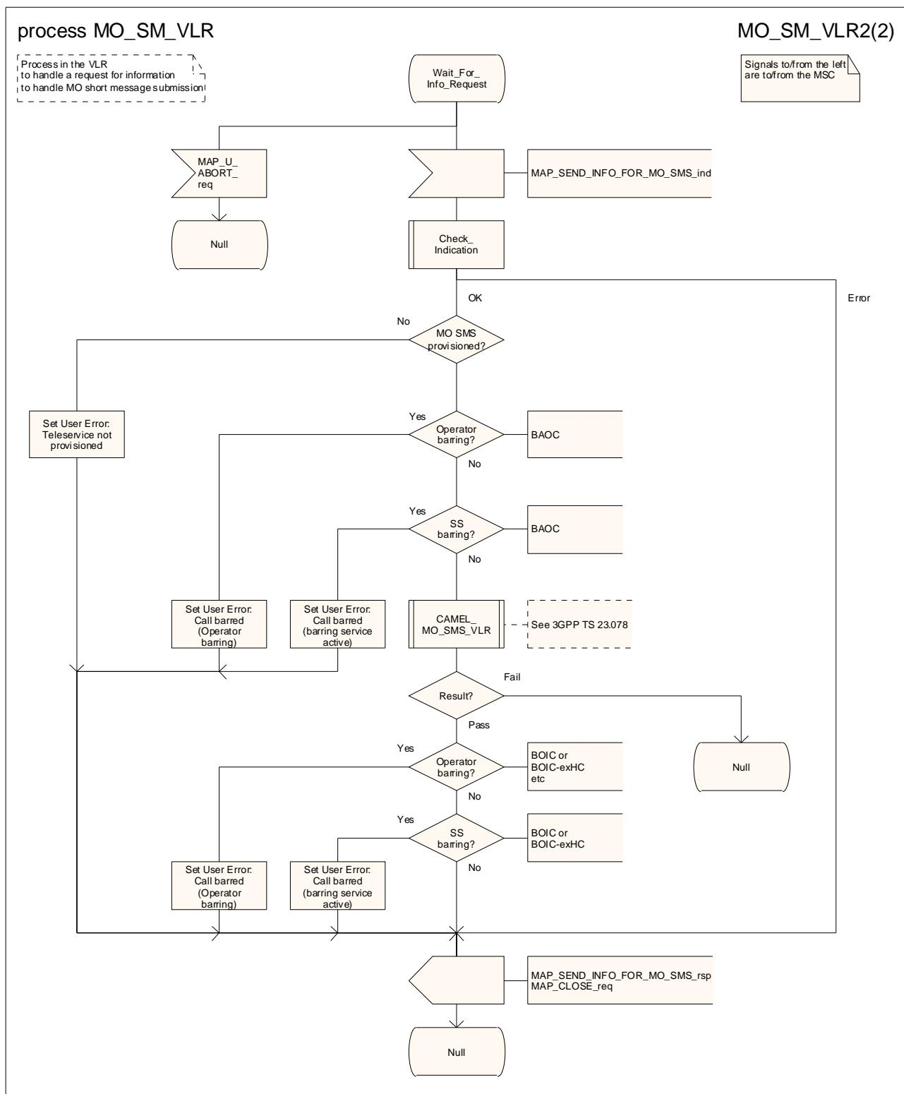
**Figure 23.2/3 (sheet 2 of 2): Process MO\_SM\_VLR**
