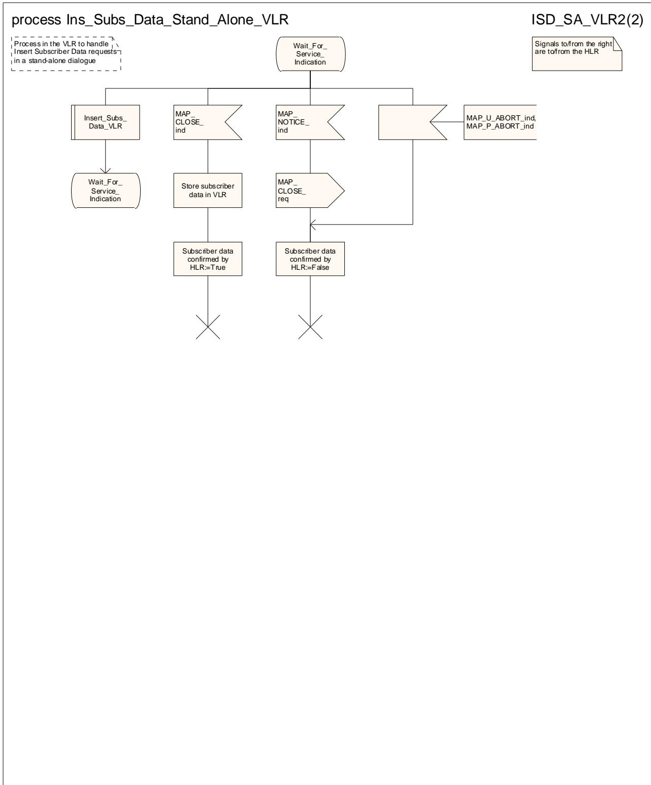
Figure 20.3/9 (sheet 2 of 2): Process Ins\_Subs\_Data\_Stand\_Alone\_VLR
