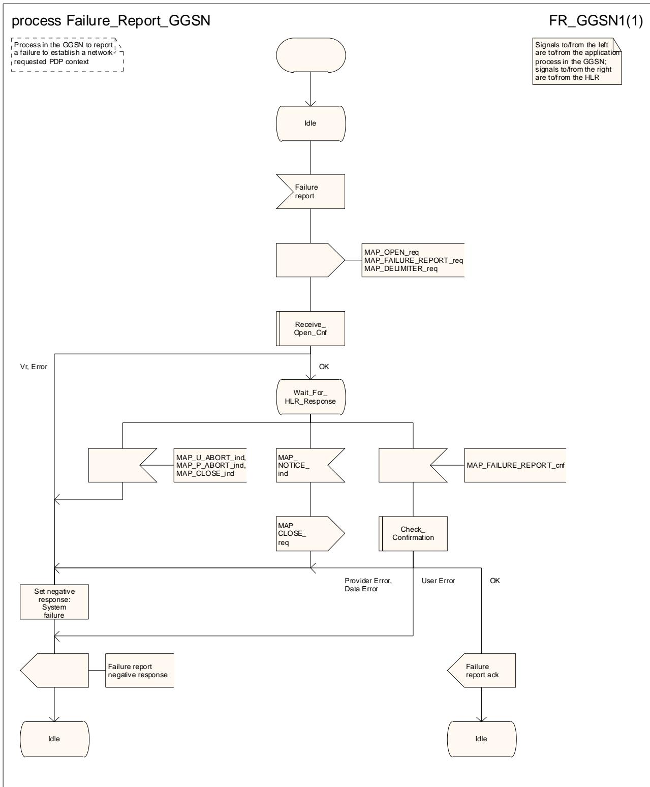
Figure 24.2/1: Process Failure\_Report\_GGSN
