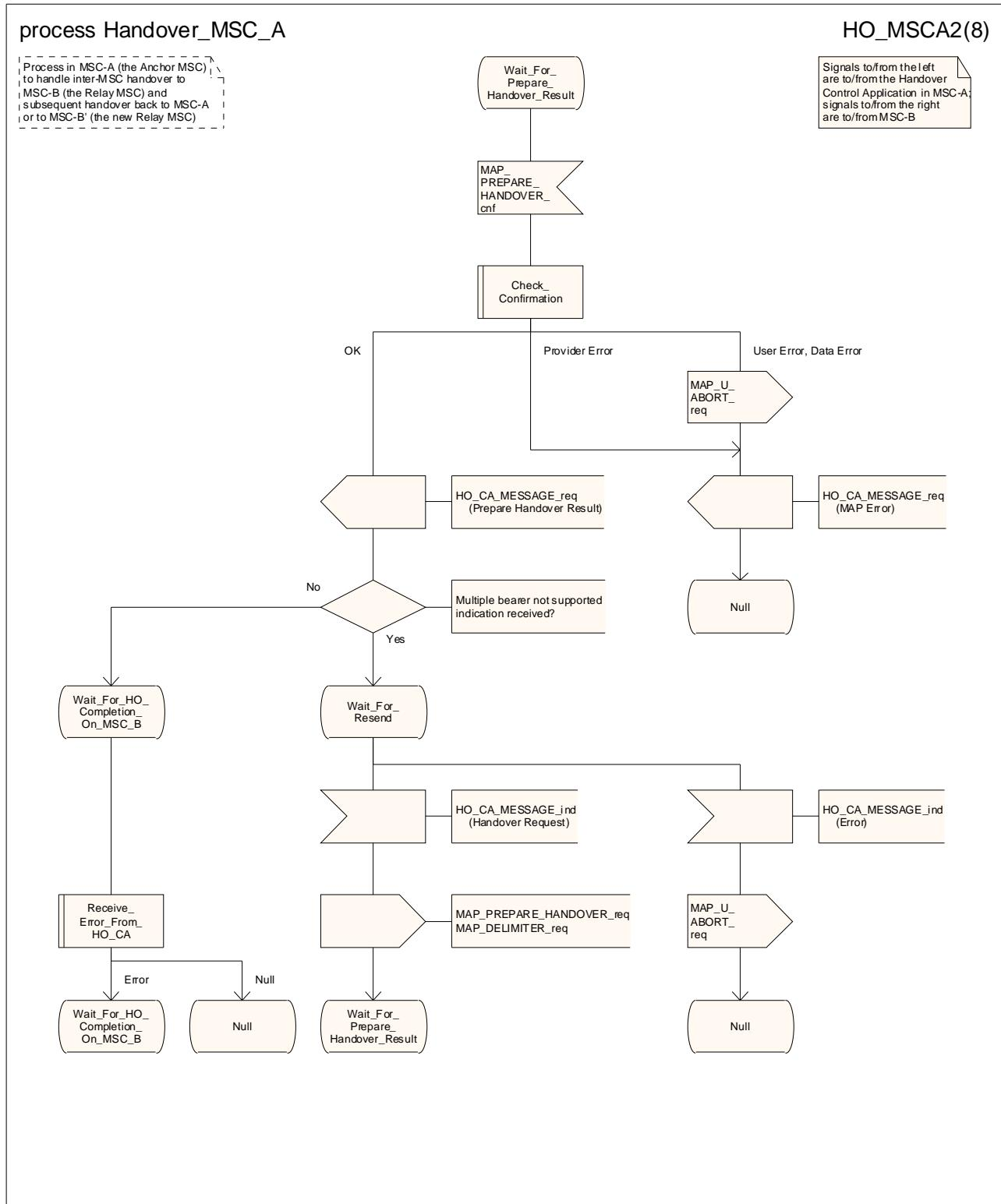
Figure 19.2/4 (sheet 2 of 8): Process HO\_MSC\_A
