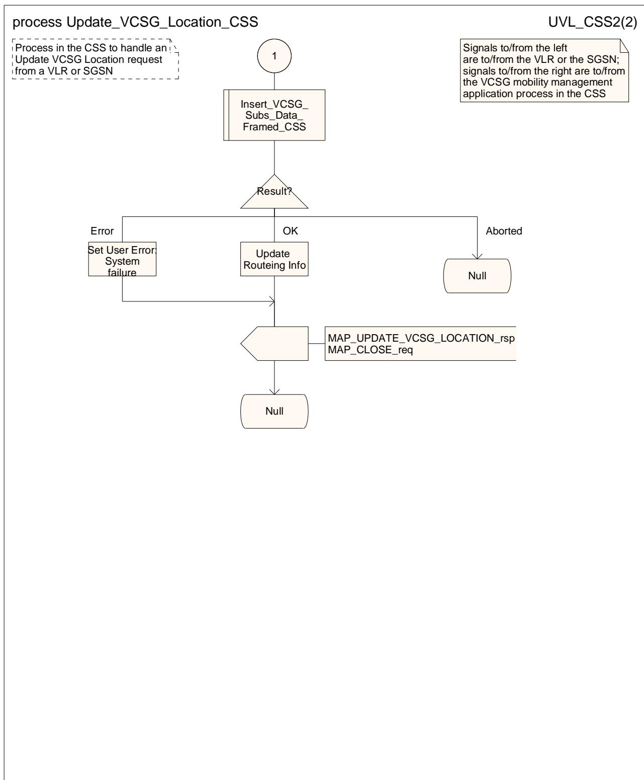
Figure 19.1.1A/4 (sheet 2 of 2): Process Update\_VCSG\_Location\_CSS
