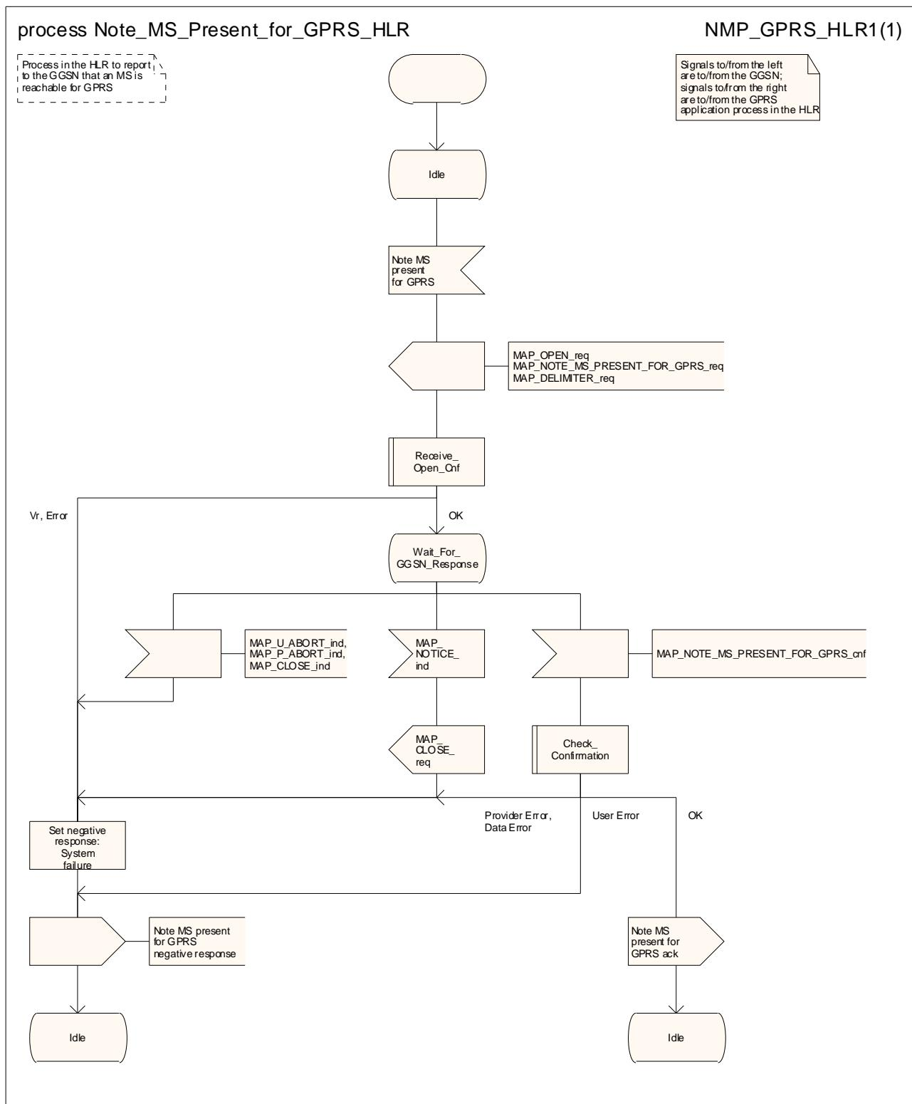
**Figure 24.3/1: Process Note\_MS\_Present\_For\_GPRS\_HLR**
