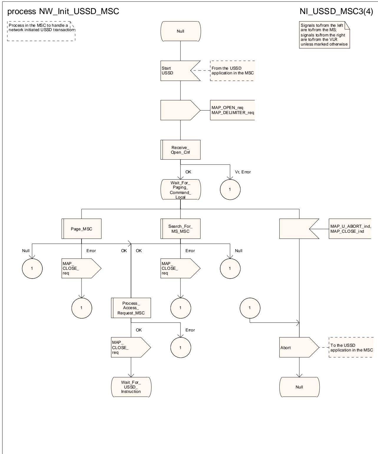
Figure 22.10.2/1 (sheet 3 of 4): Process NW\_Init\_USSD\_MSC
