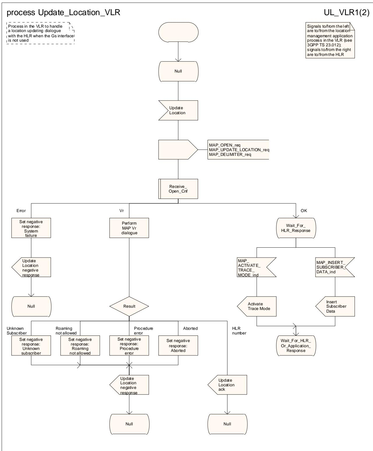
Figure 19.1.1/6 (sheet 1 of 2): Process Update\_Location\_VLR
