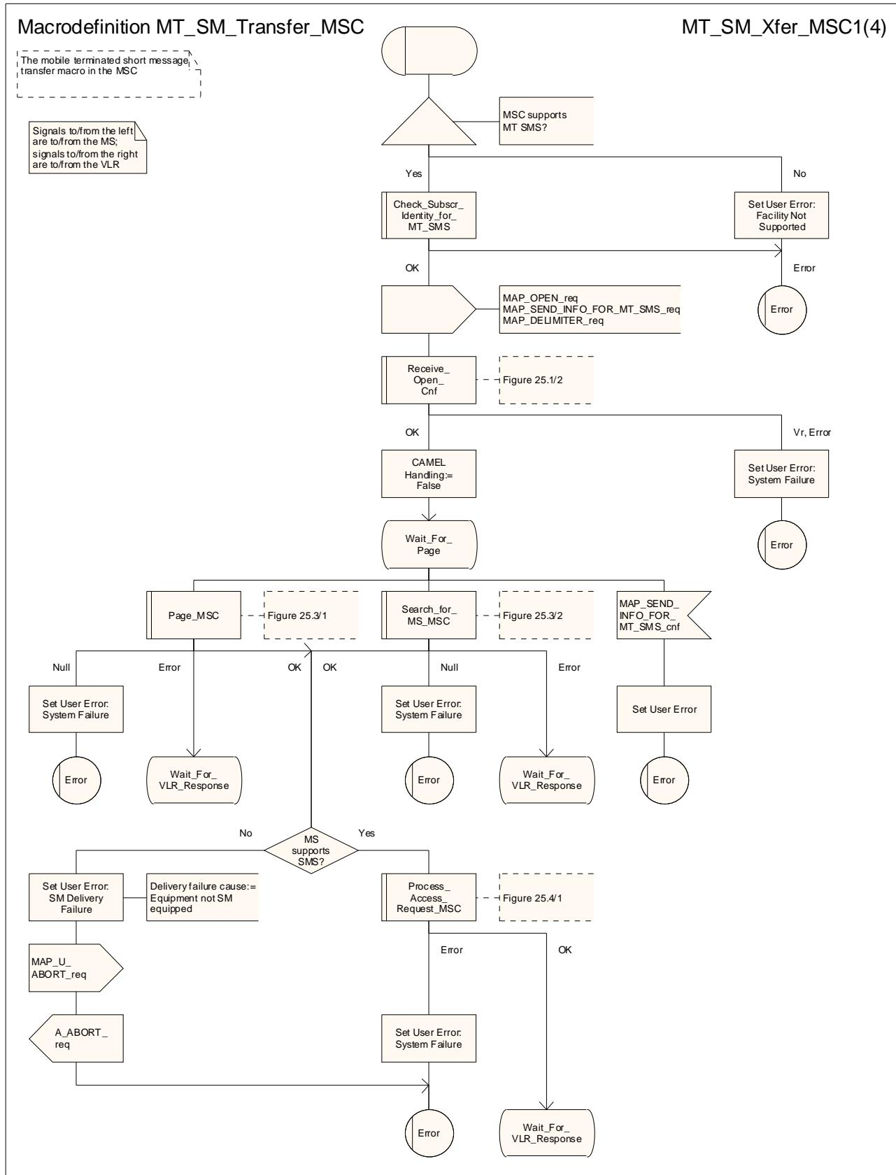
**Figure 23.3/7 (sheet 1 of 4): Macro MT\_SM\_Transfer\_MSC**
