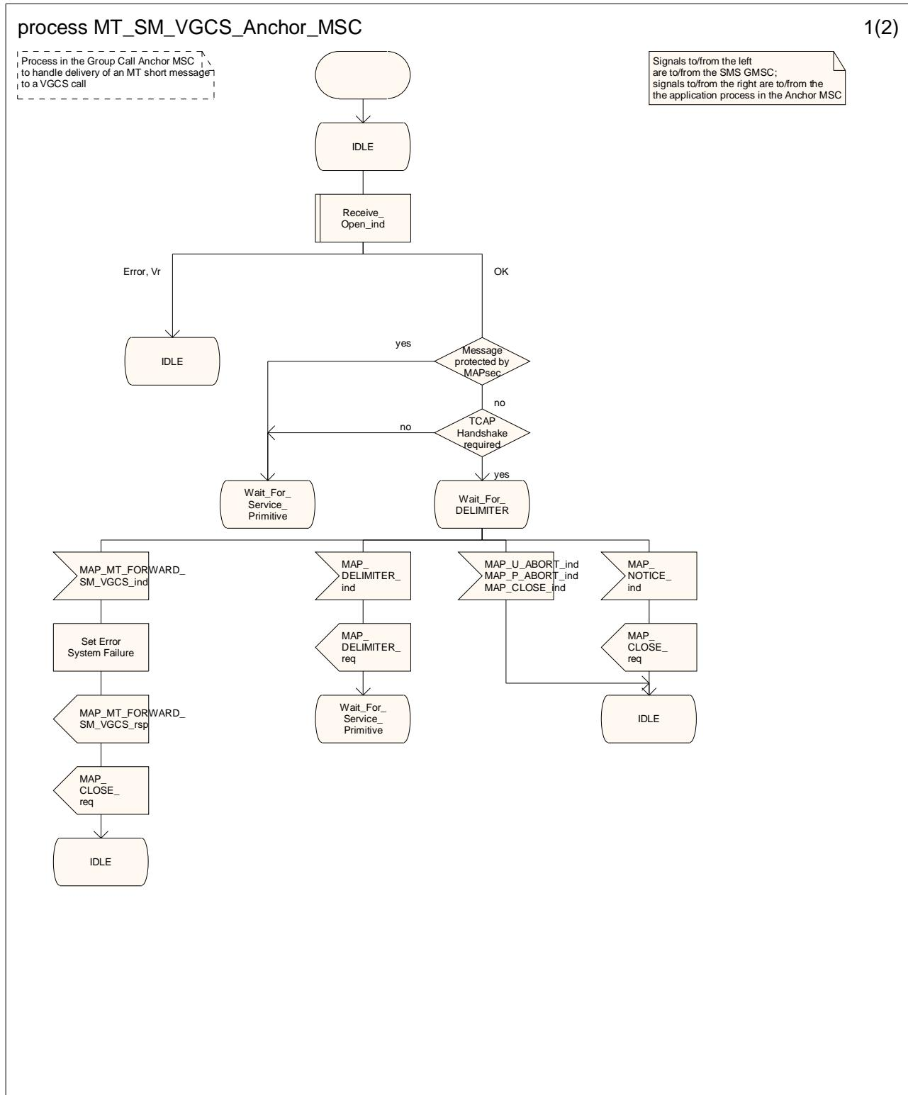
Figure 23.7/3 (sheet 1 of 2): Process MT\_SM\_VGCS\_Anchor MSC
