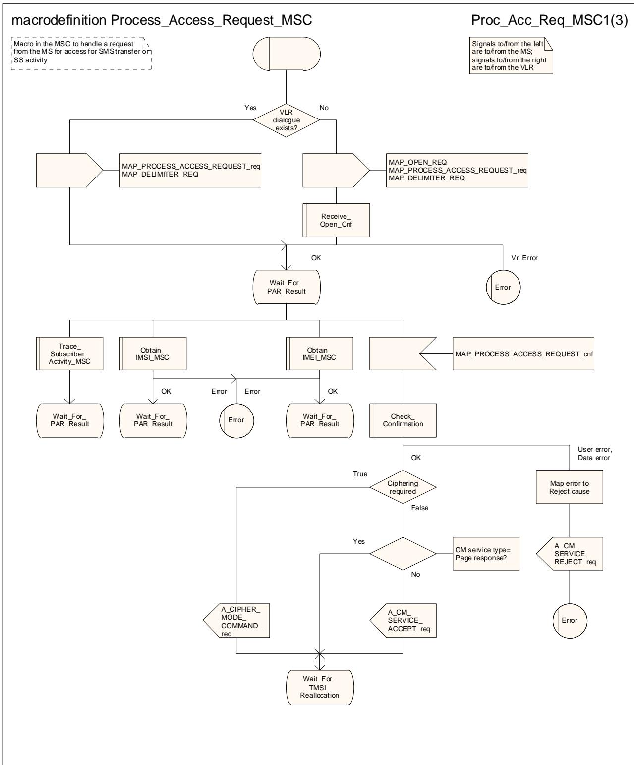
Figure 25.4/1 (sheet 1 of 3): Macro Process\_Access\_Request\_MSC
