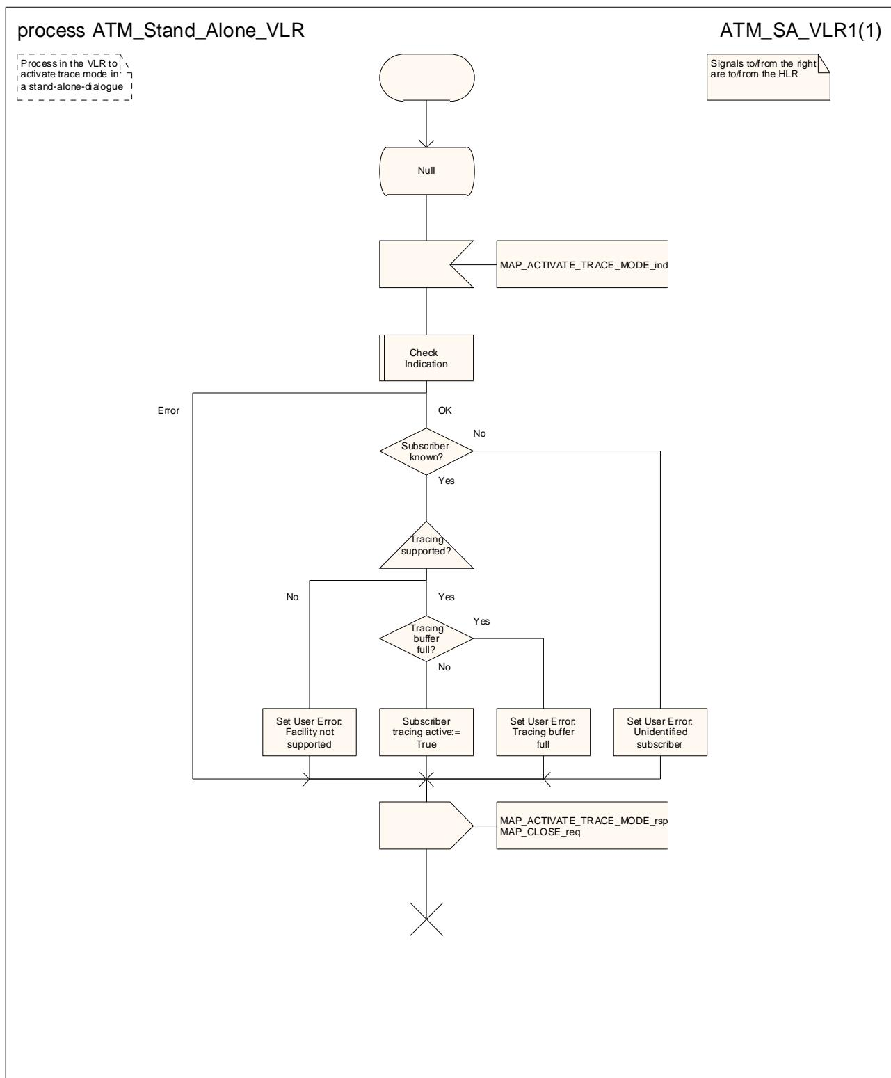
Figure 20.2/10: Process ATM\_Standalone\_VLR
