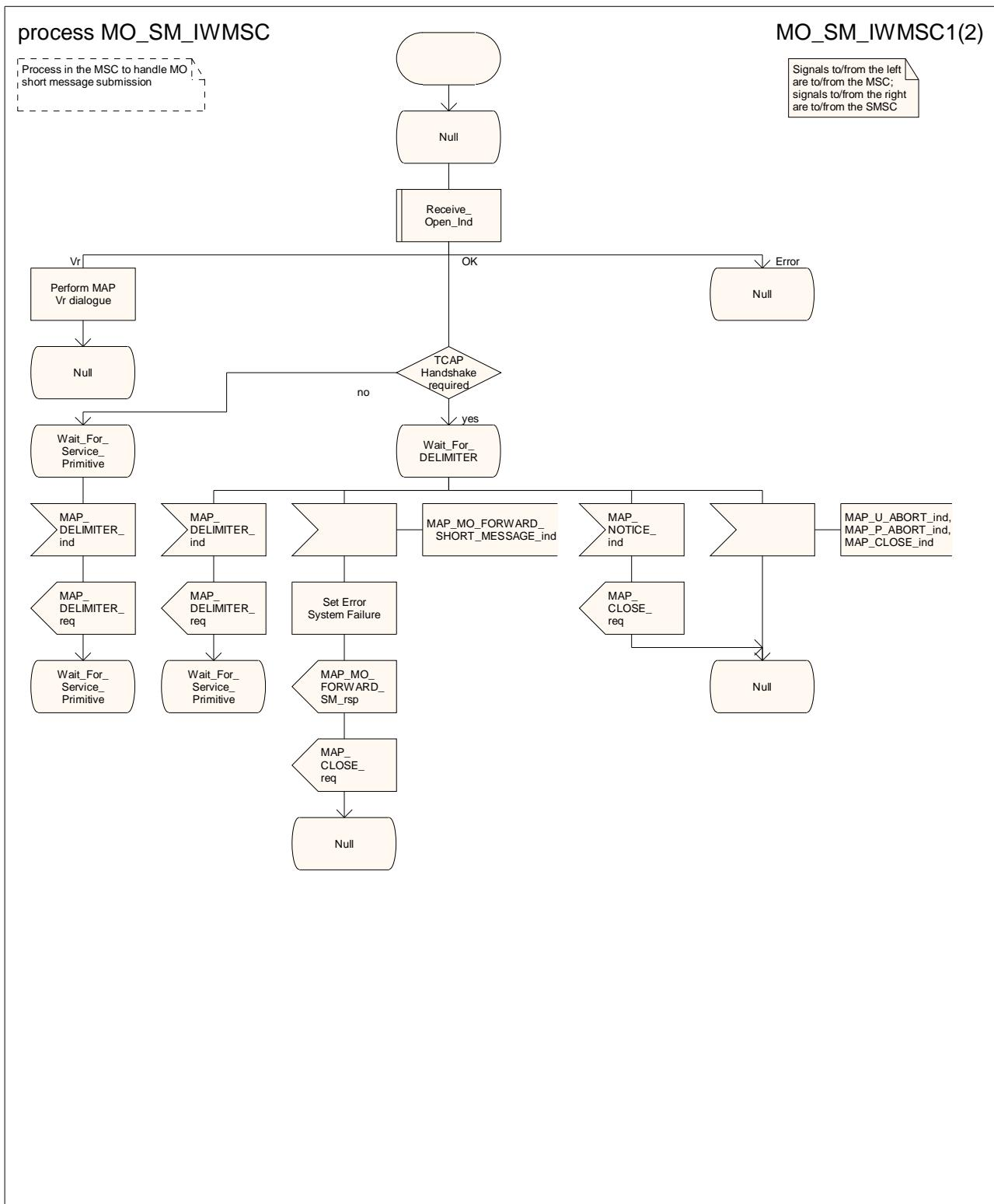
Figure 23.2/5 (sheet 1 of 2): Process MO\_SM\_IWMSC
