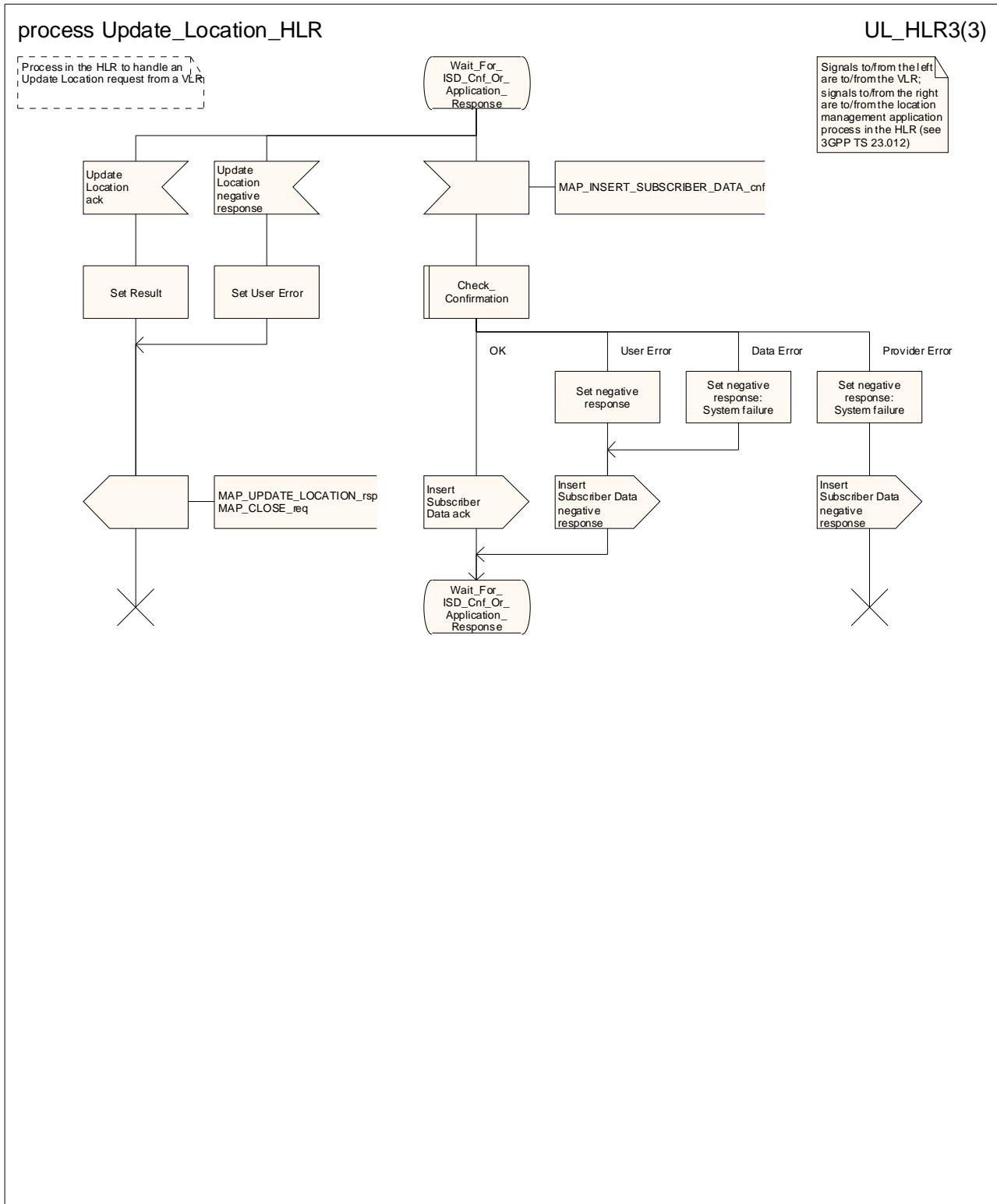
Figure 19.1.1/13 (sheet 3 of 3): Process Update\_Location\_HLR
