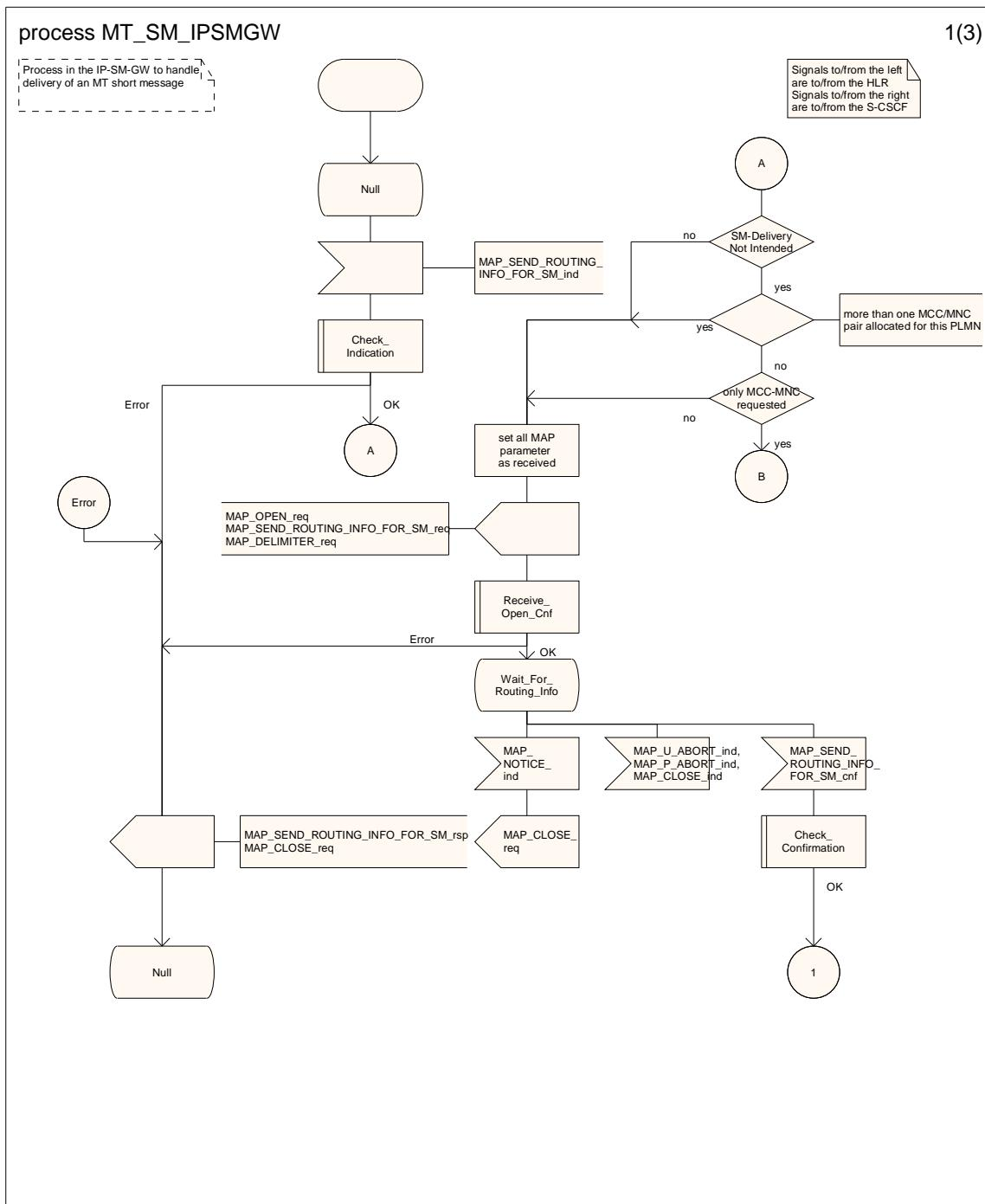
Figure 23.3/15 (sheet 1 of 3): Process MT\_SM\_IPSMGW
