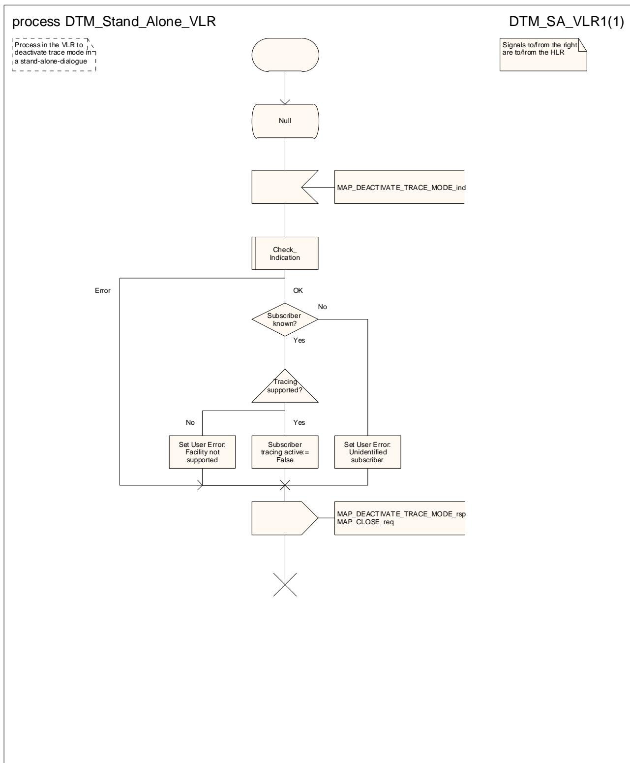
Figure 20.2/14: Process DTM\_Standalone\_VLR
