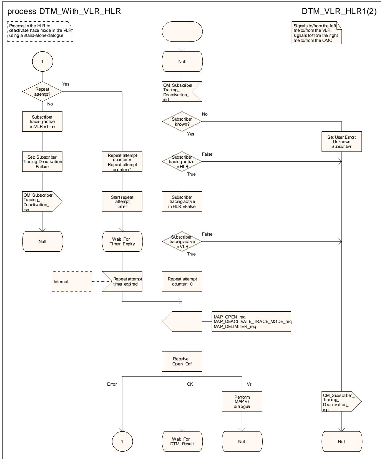
Figure 20.2/12 (sheet 1 of 2): Process DTM\_with\_VLR\_HLR
