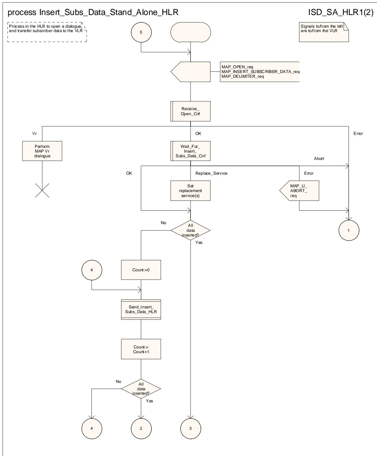
**Figure 25.7/3 (sheet 1 of 2): Process Insert\_Subs\_Data\_Stand\_A lone\_HLR**
