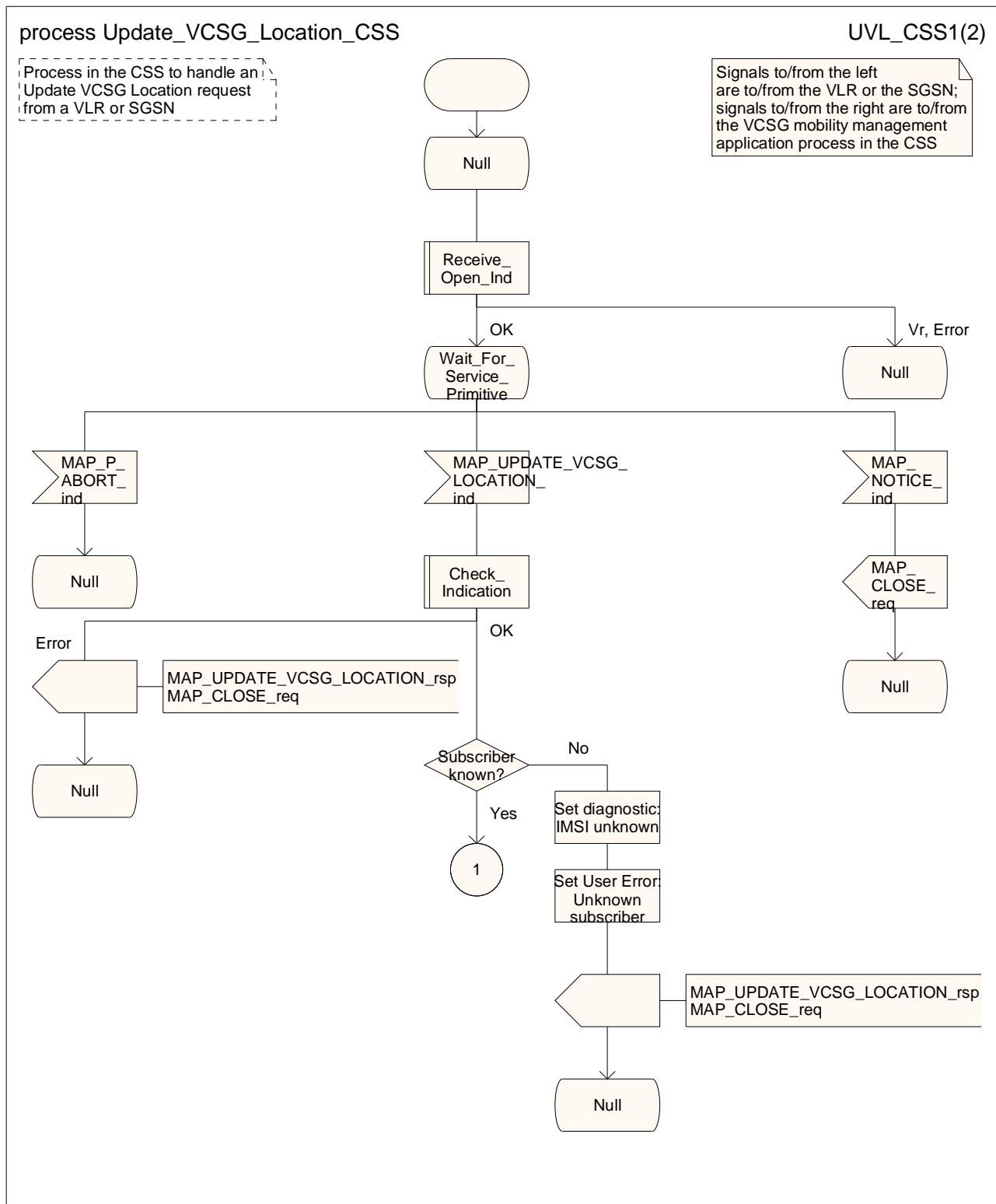
Figure 19.1.1A/4 (sheet 1 of 2): Process Update\_VCSG\_Location\_CSS
