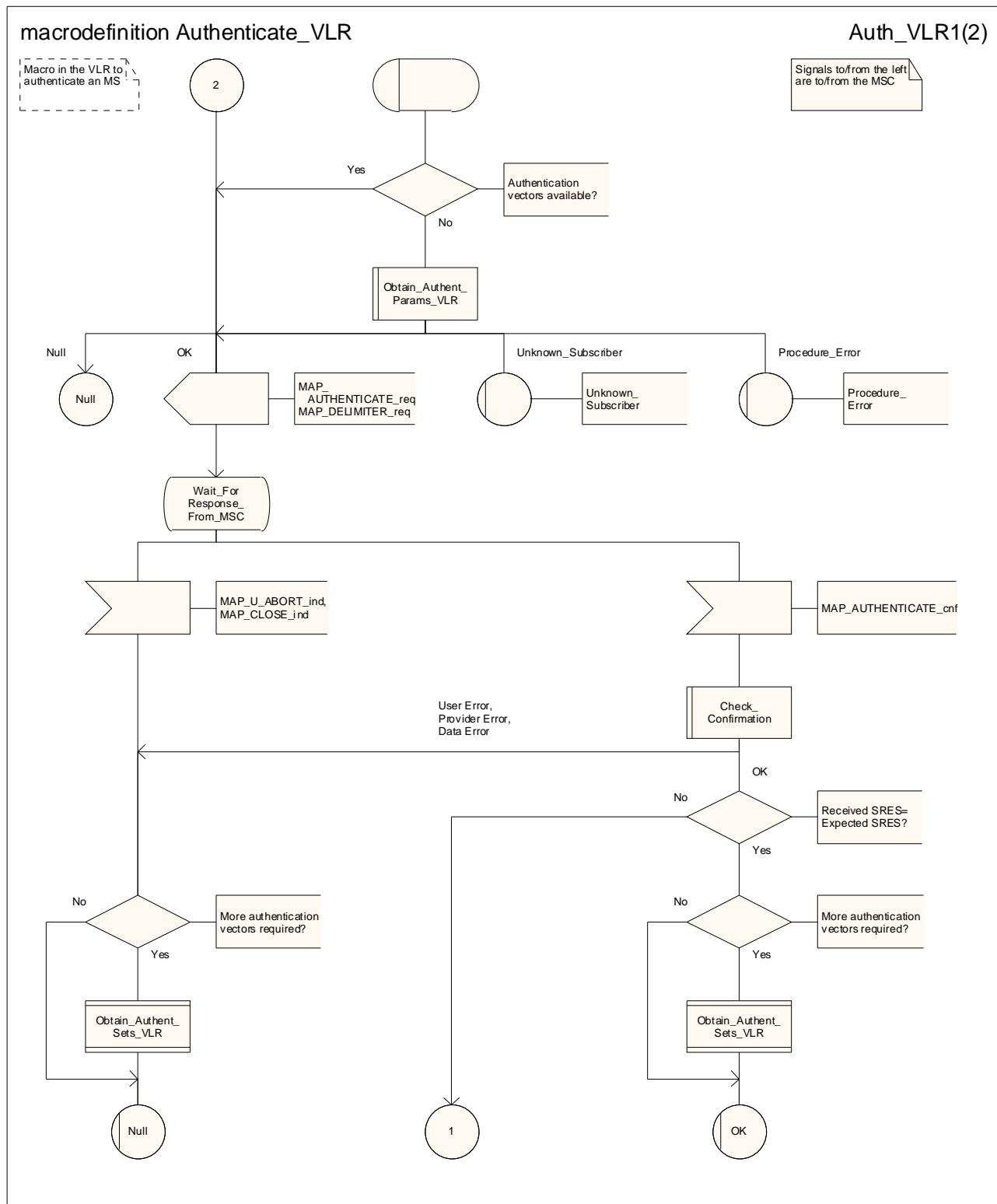
**Figure 25.5/2 (sheet 1 of 2): Macro Authenticate\_VLR**
