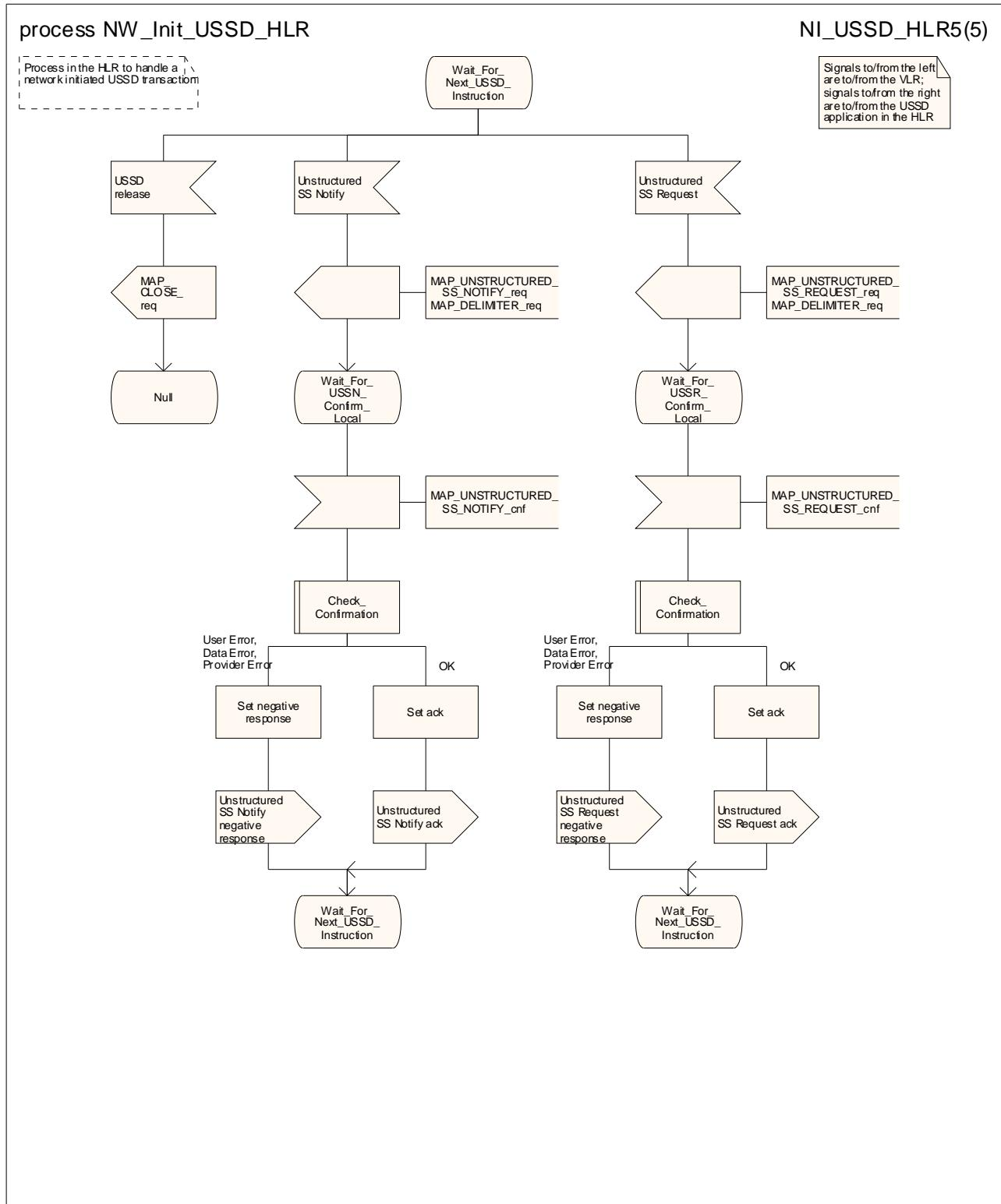
Figure 22.10.4/1 (sheet 5 of 5): Process NW\_Init\_USSD\_HLR
