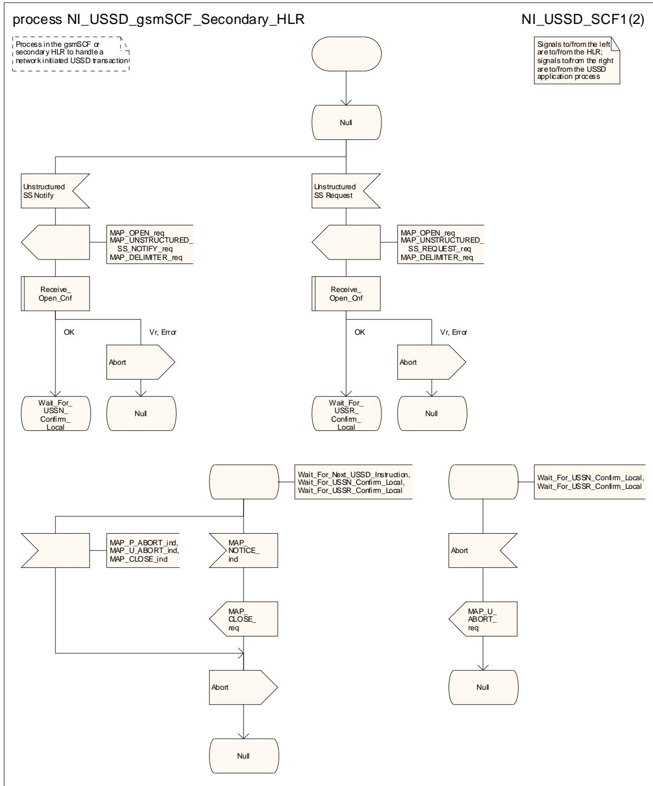
Figure 22.10.5/1 (sheet 1 of 2): Process NW\_Init\_USSD\_gsmSCF\_secondary\_HLR
