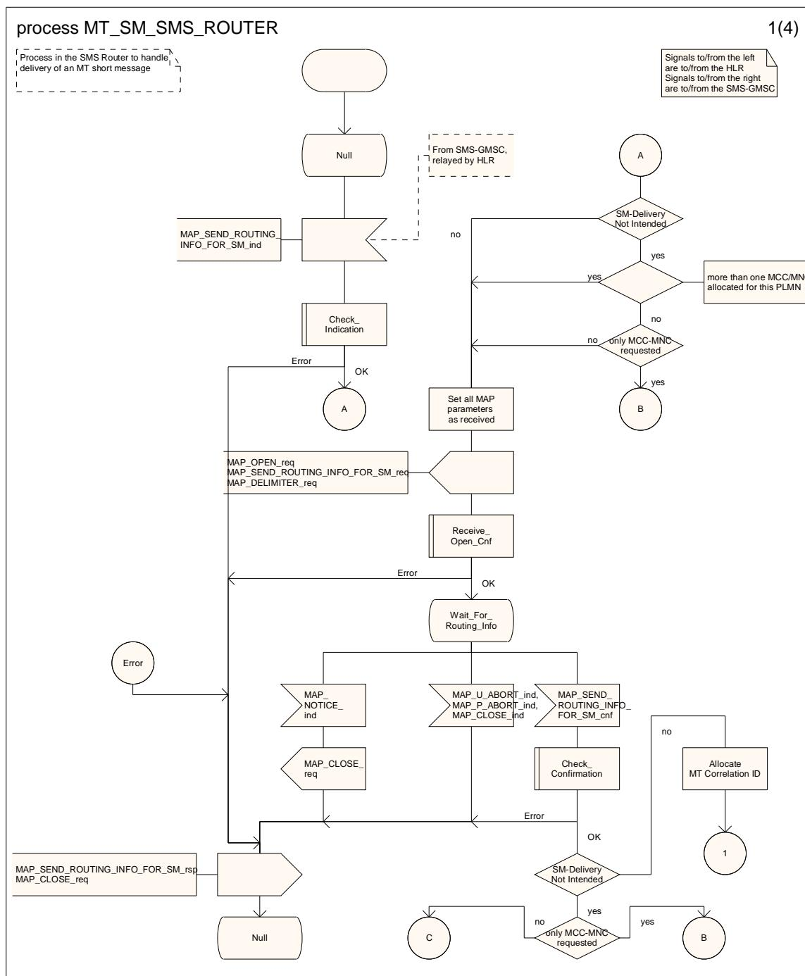
**Figure 23.3/14 (sheet 1 of 4): Process MT\_SM\_SMS\_ROUTER**
