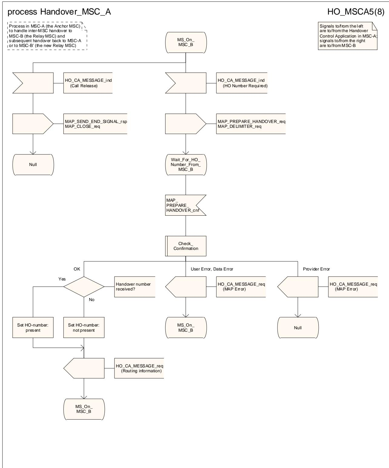
Figure 19.2/4 (sheet 5 of 8): Process HO\_MSC\_A
