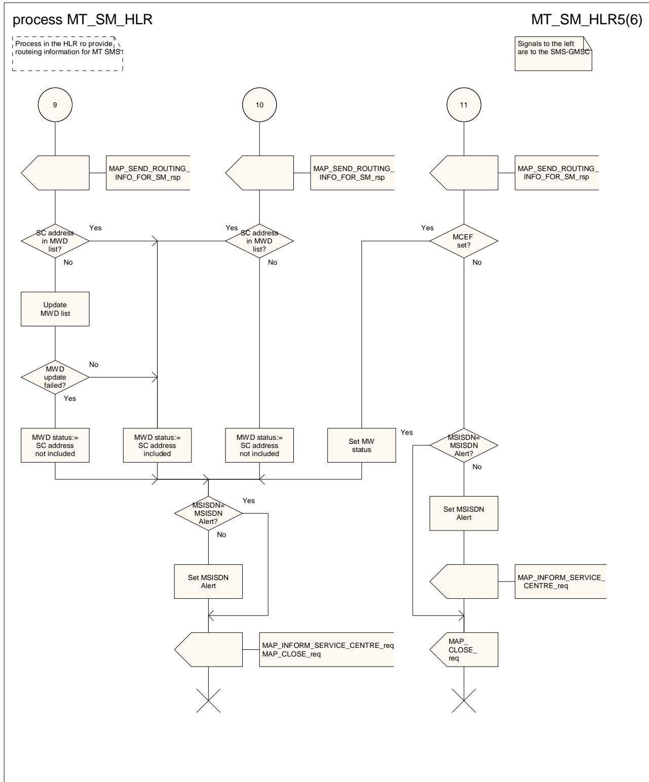
Figure 23.3/5 (sheet 5 of 6): Process MT\_SM\_HLR
