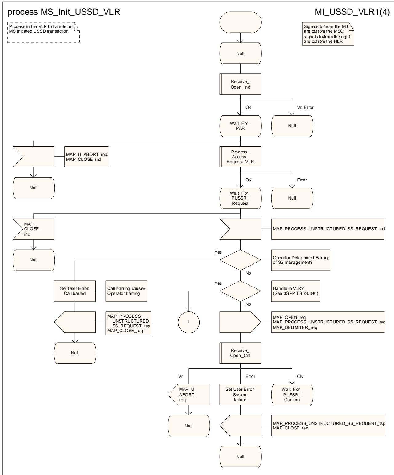
Figure 22.9.3/1 (sheet 1 of 4): Process MS\_Init\_USSD\_VLR
