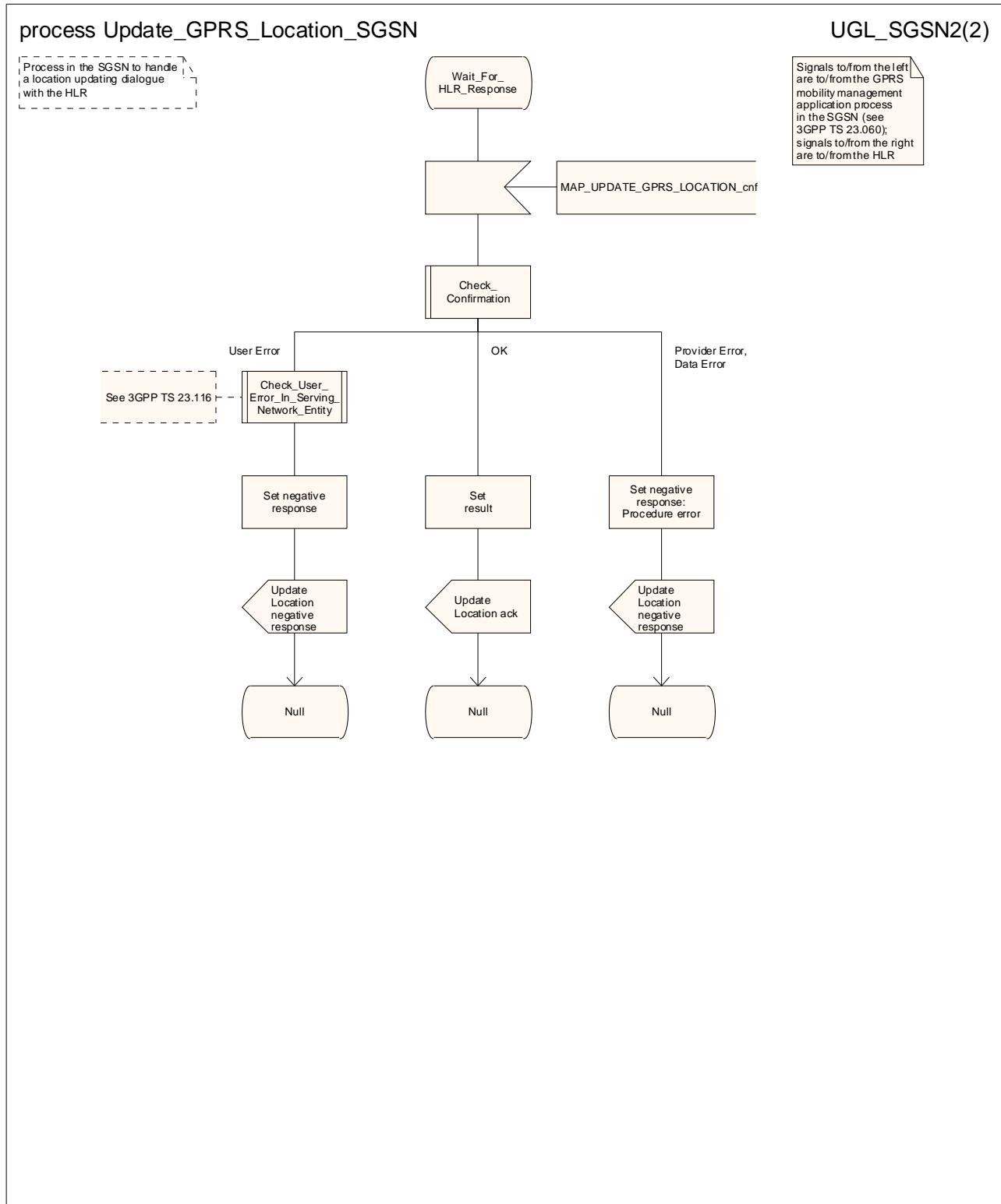
Figure 19.1.1/12 (sheet 2 of 2): Process Update\_GPRS\_Location\_SGSN
