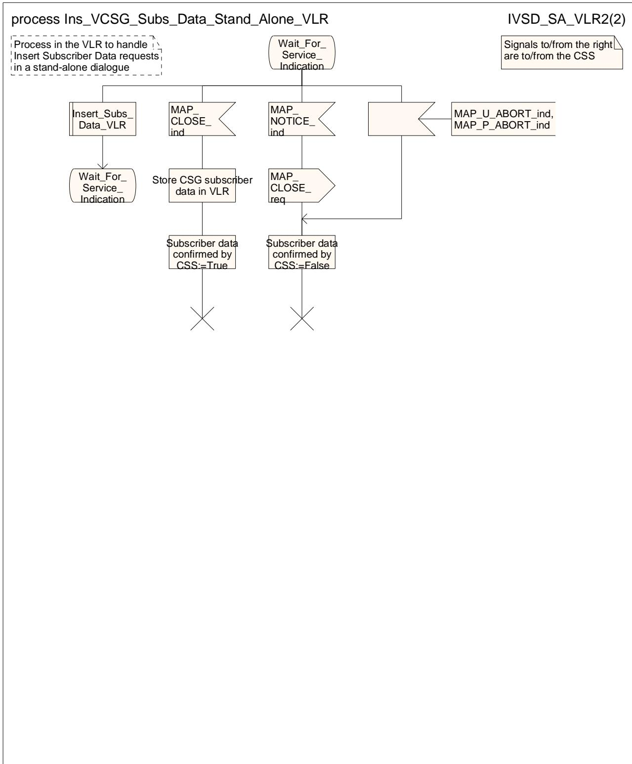
Figure 20.3A/8 (sheet 2 of 2): Process Ins\_VCSG\_Subs\_Data\_Stand\_Alone\_VLR
