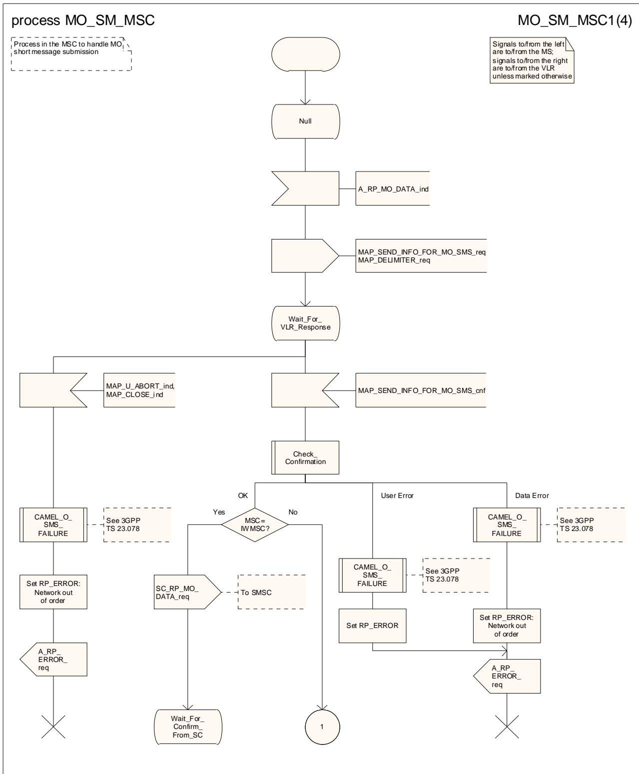
Figure 23.2/2 (sheet 1 of 4): Process MO\_SM\_MSC
