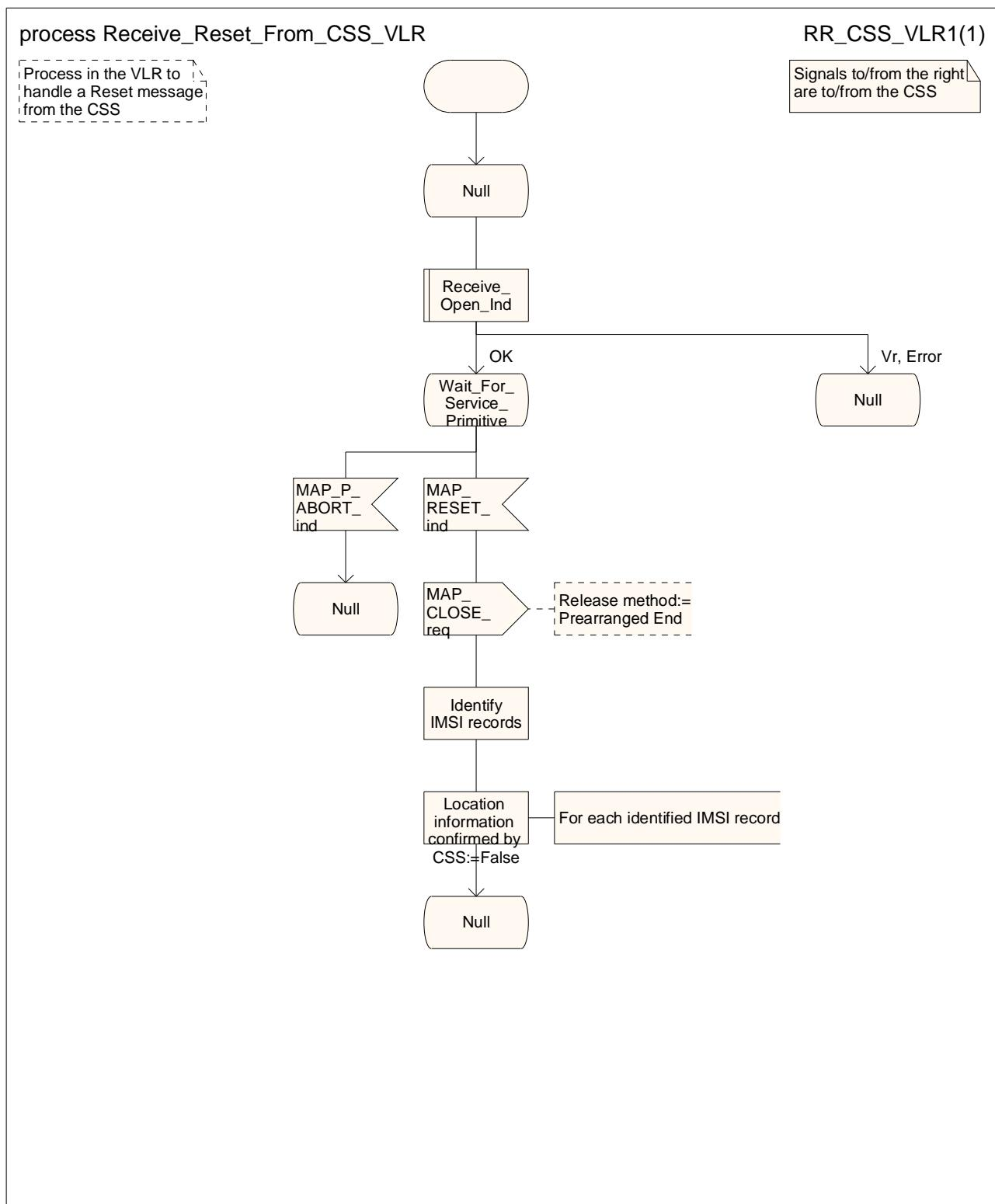
Figure 19.3.3/6: Process Receive\_Reset\_From\_CSS\_VLR
