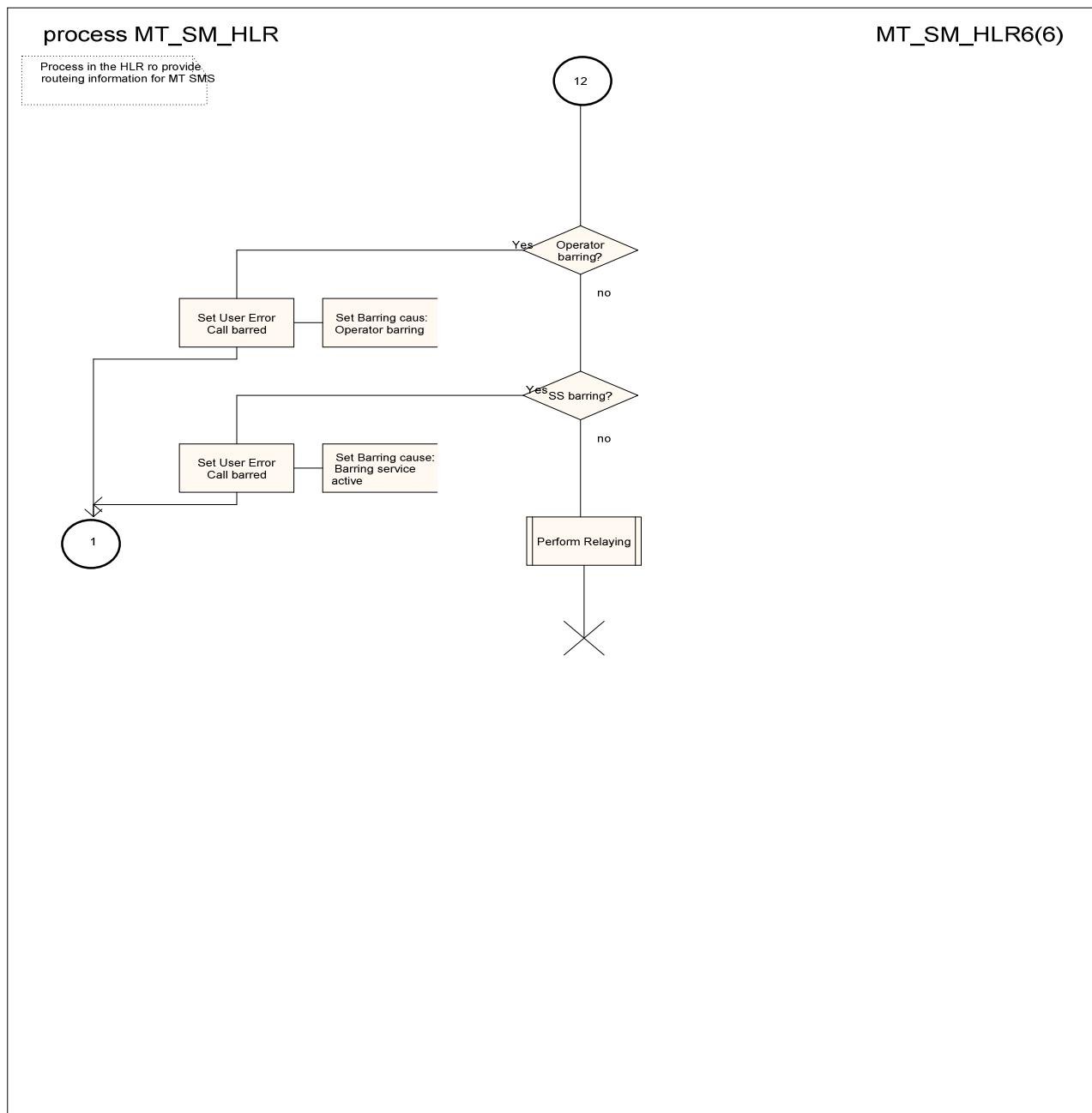
Figure 23.3/5 (sheet 6 of 6): Process MT\_SM\_HLR
