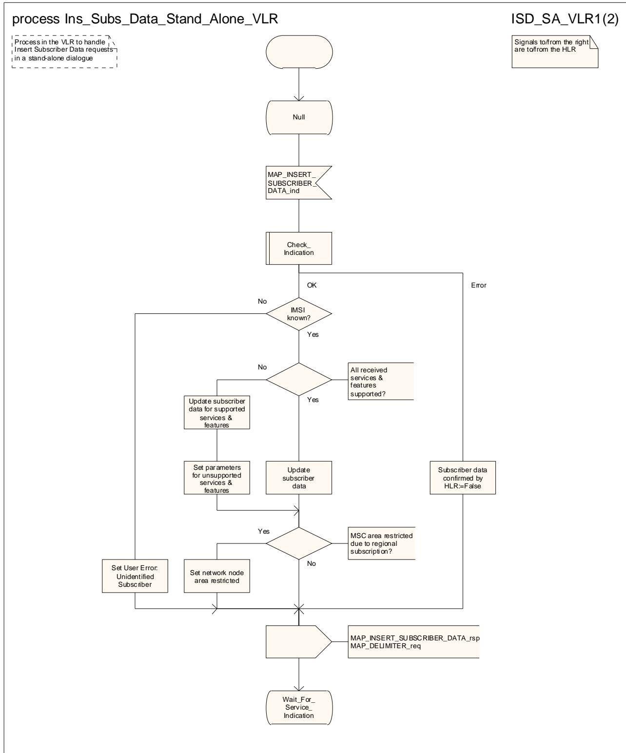
**Figure 20.3/9 (sheet 1 of 2): Process Ins\_Subs\_Data\_Stand\_Alone\_VLR**
