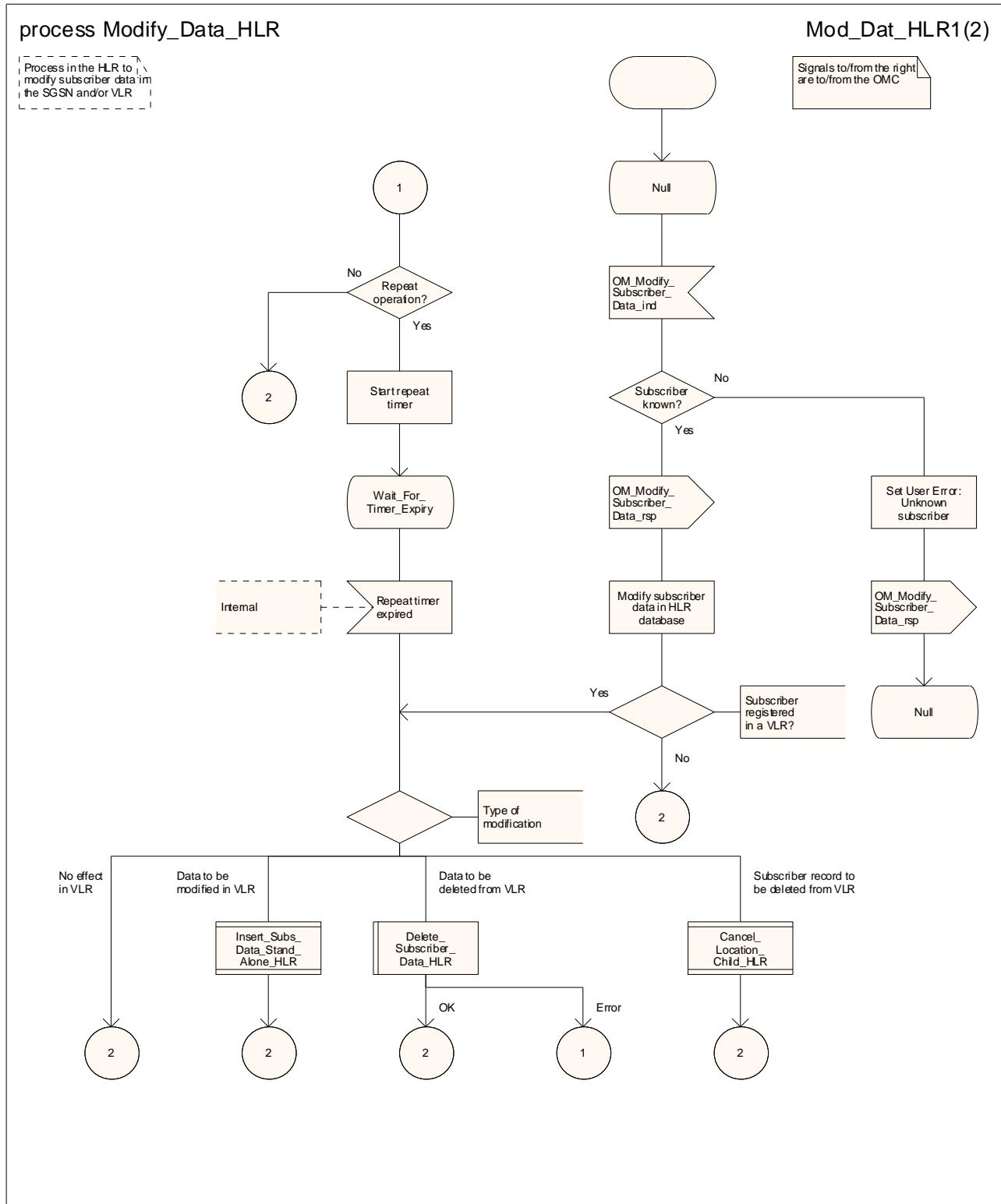
Figure 20.3/6 (sheet 1 of 2): Process Modify\_Data\_HLR
