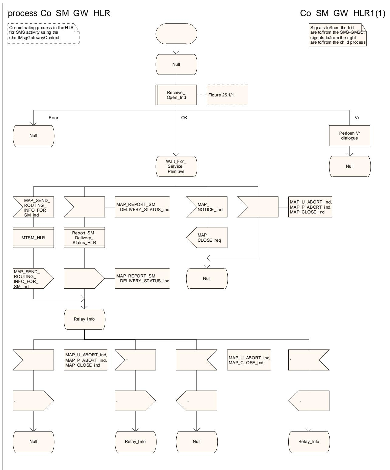
**Figure 23.1/2: Process Co\_SM\_Gateway\_HLR**
