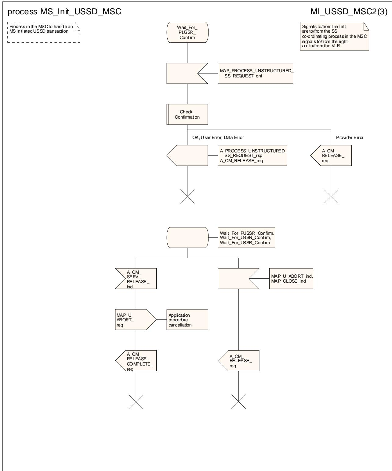
Figure 22.9.2/1 (sheet 2 of 3): Process MS\_Init\_USSD\_MSC
