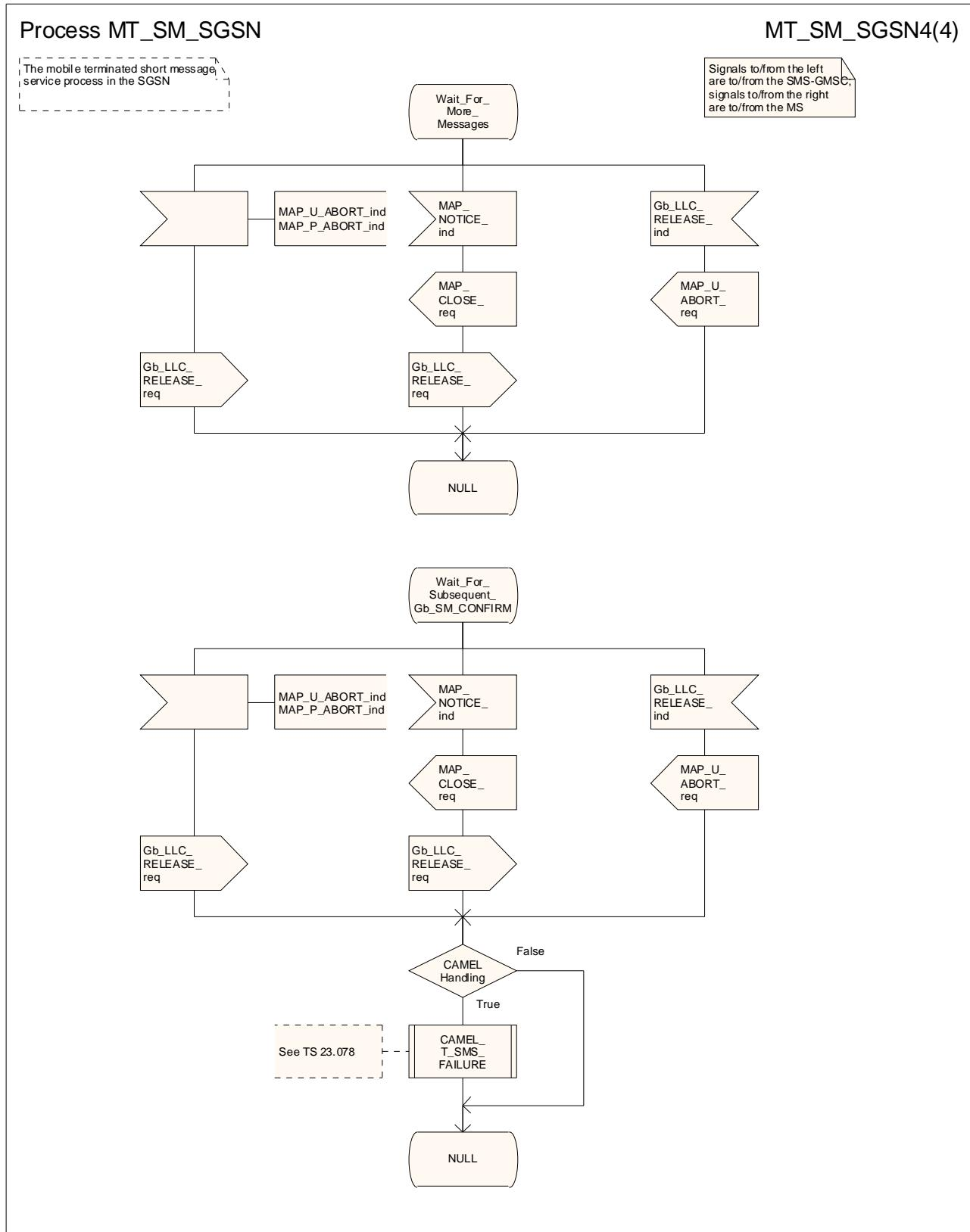
Figure 23.3/10 (sheet 4 of 4): Process MT\_SM\_SGSN
