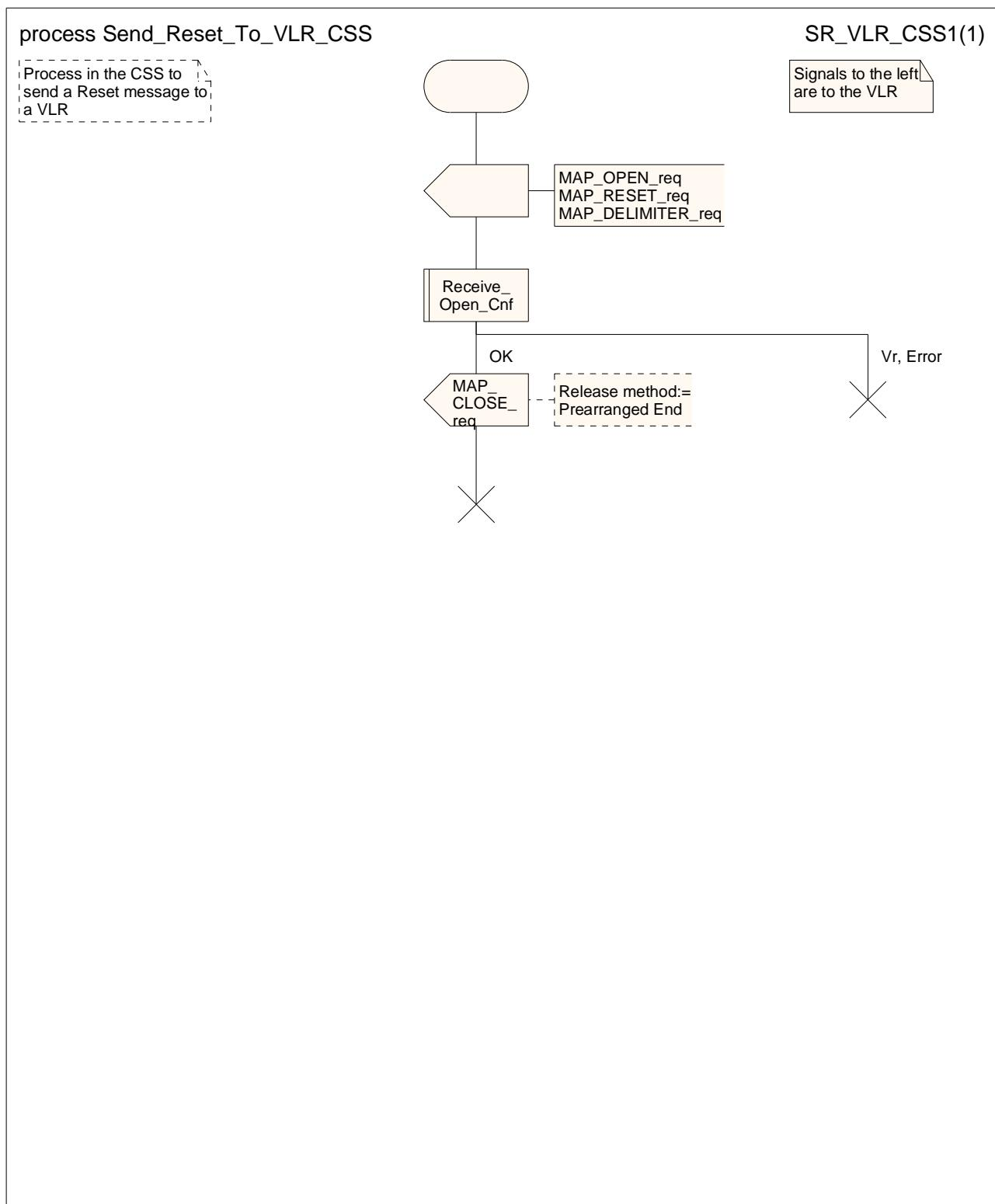
**Figure 19.3.3/4: Process Send\_Reset\_To\_VLR\_CSS**
