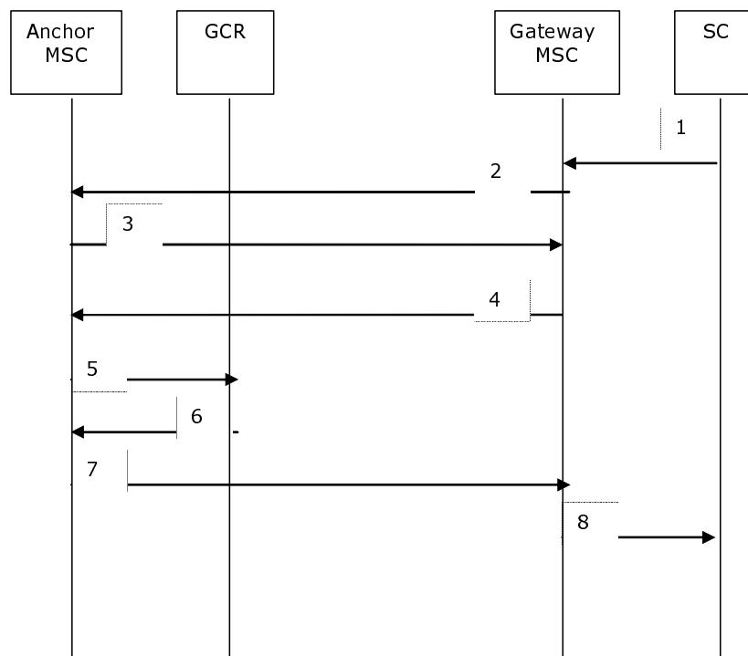
**Figure 23.7/1: Mobile terminated short message for VGCS service procedures**
