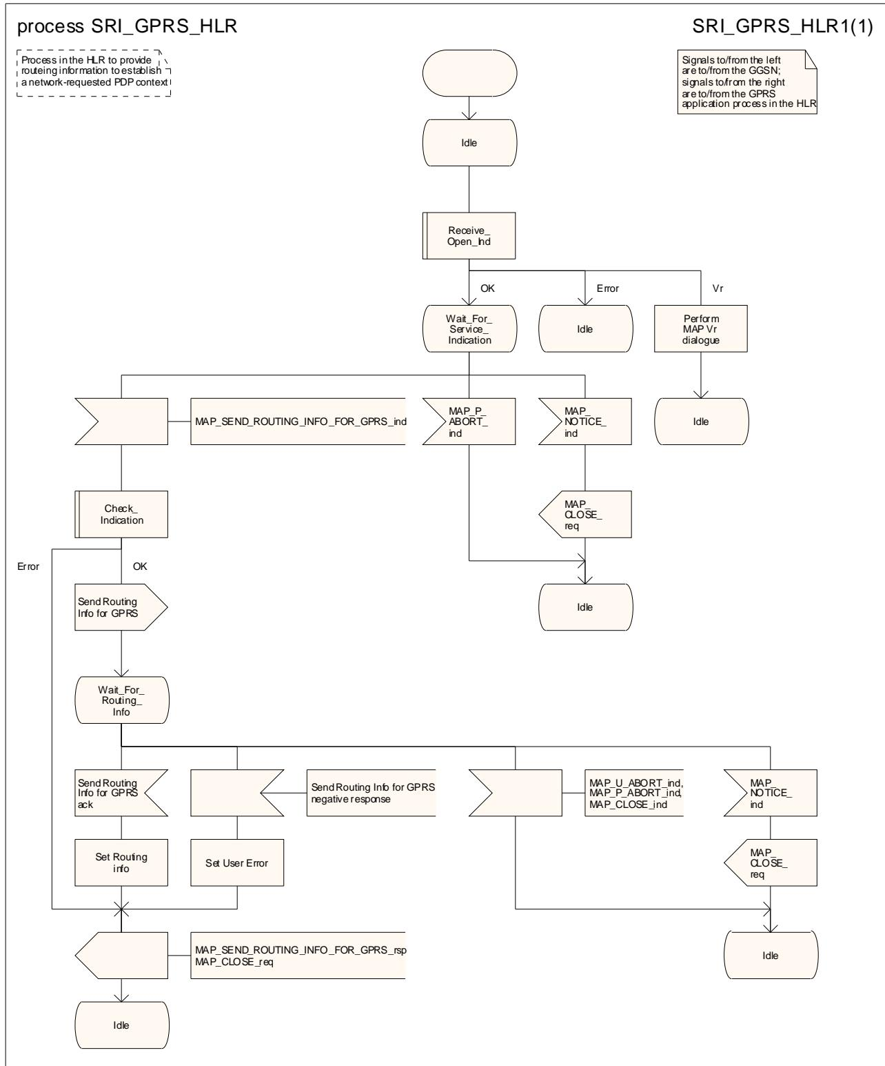
Figure 24.1/2: Process SRI\_GPRS\_HLR
