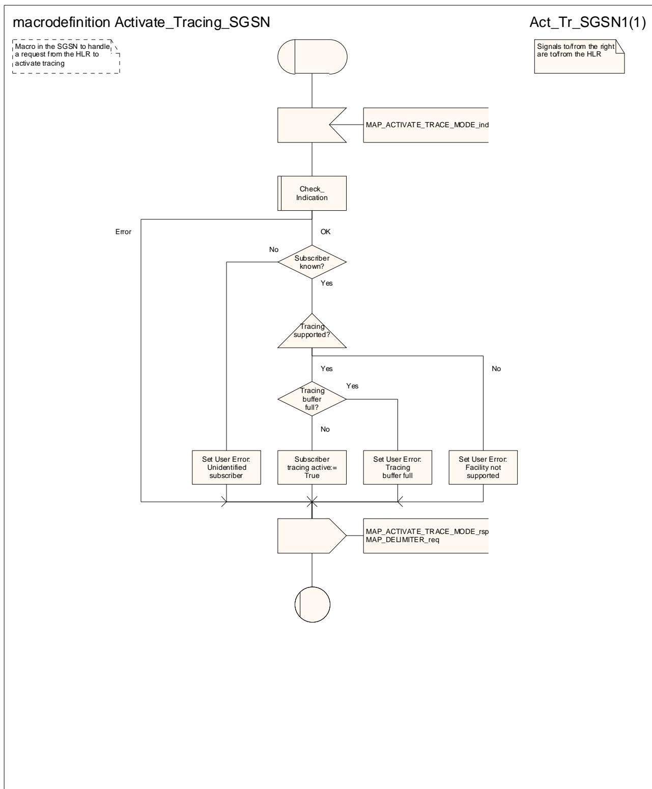
**Figure 25.9/5: Macro Activate\_Tracing\_SGSN**
