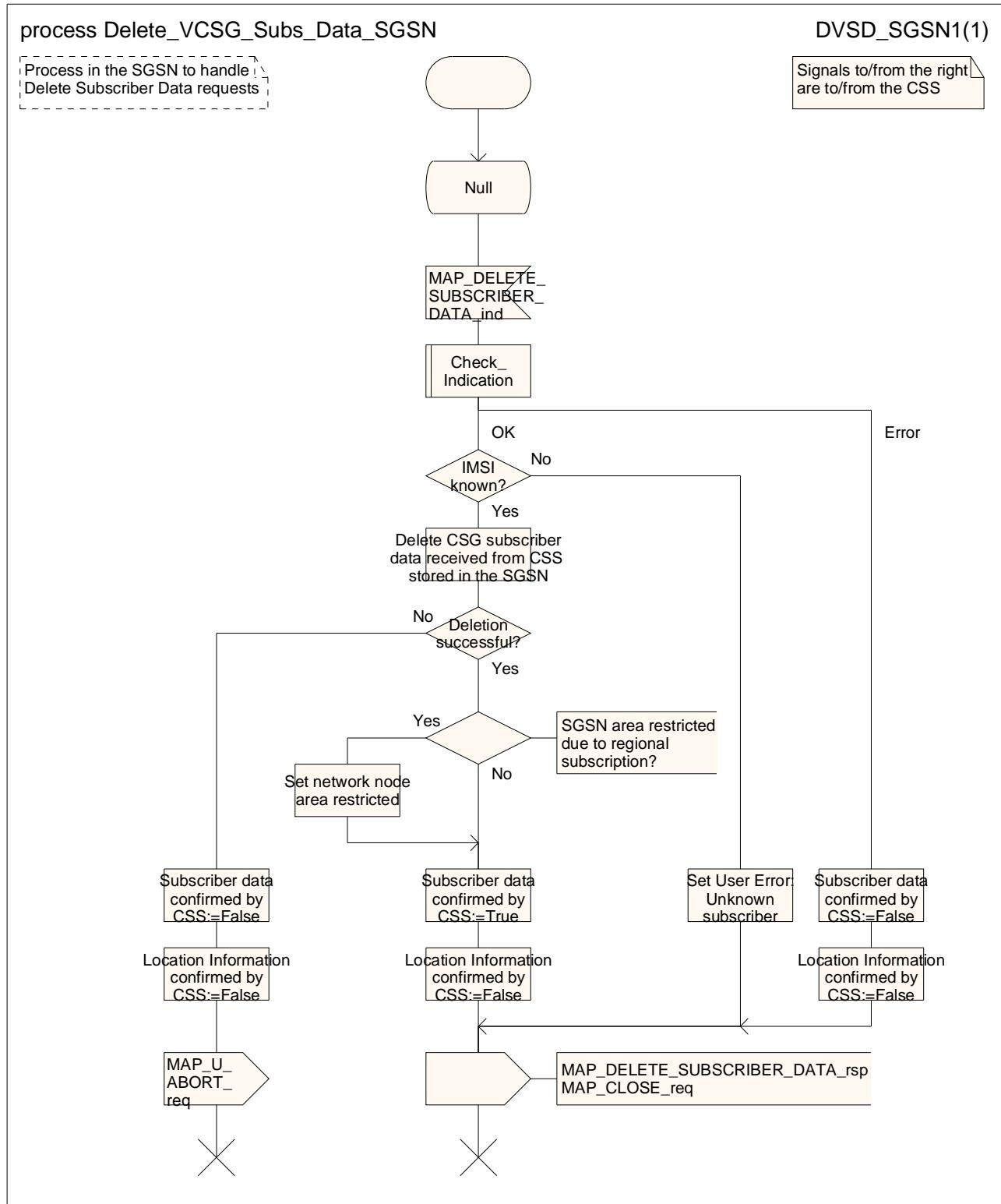
Figure 20.3A/11: Process Delete\_VCSG\_Subs\_Data\_SGSN
