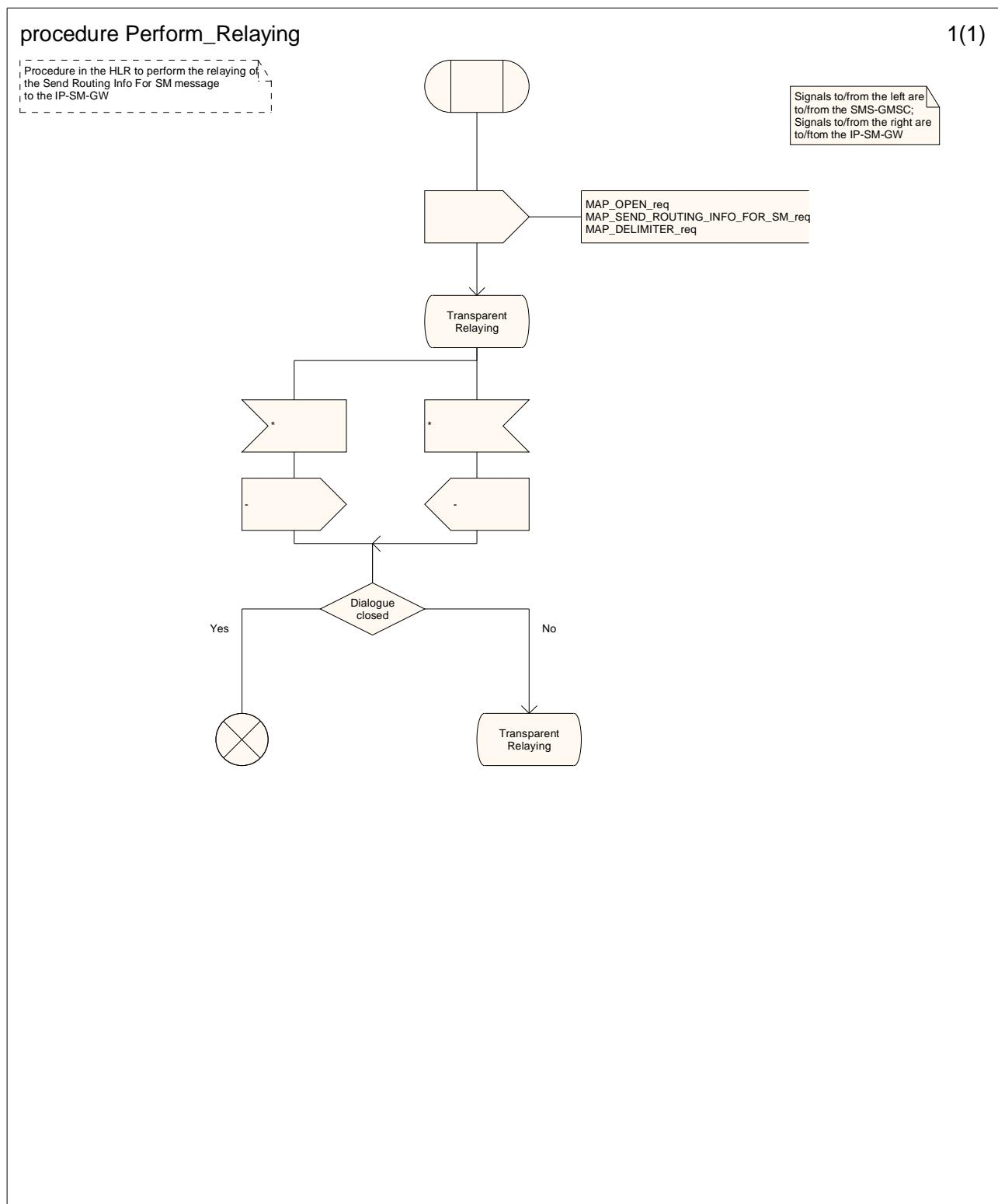
**Figure 23.3/5a (sheet 1 of 1): Procedure Perform\_Relaying**
