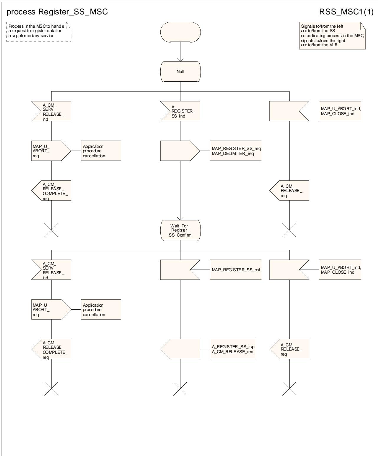
Figure 22.2.2/1: Process Register\_SS\_MSC
