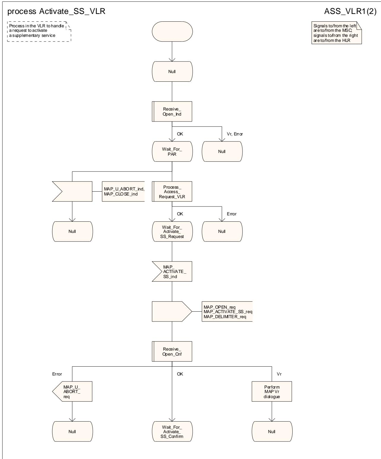
**Figure 22.4.3/1 (sheet 1 of 2): Process Activate\_SS\_VLR**
