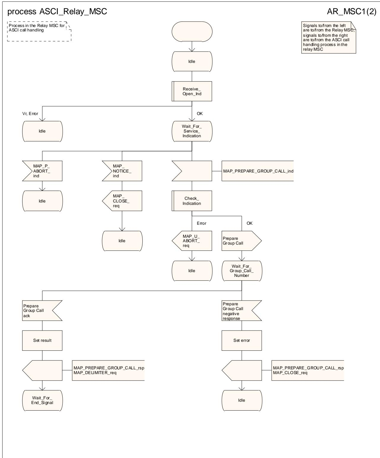
Figure 21.4/3 (sheet 1 of 2): Process ASCI\_Relay\_MSC
