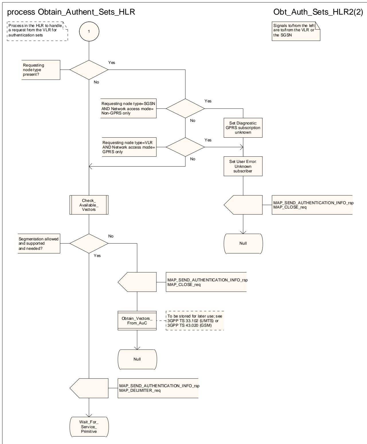
Figure 25.5/6 (sheet 2 of 2): Process Obtain\_Authent\_Sets\_HLR
