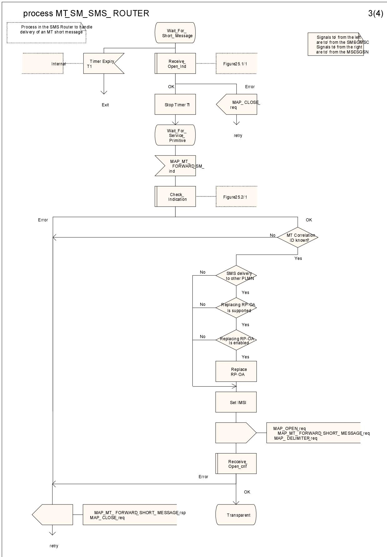
Figure 23.3/14 (sheet 3 of 4): Process MT\_SM\_SMS\_ROUTER
