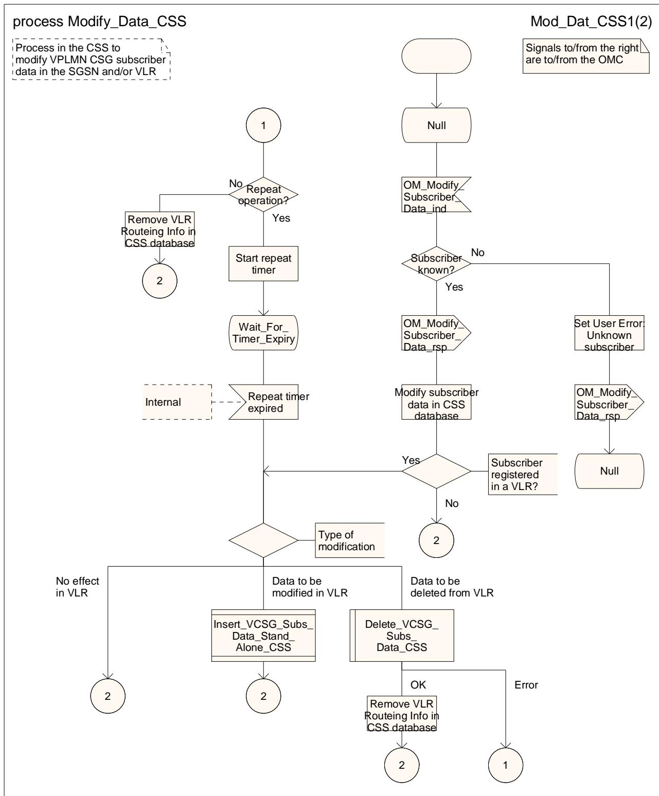
Figure 20.3A/6 (sheet 1 of 2): Process Modify\_Data\_CSS
