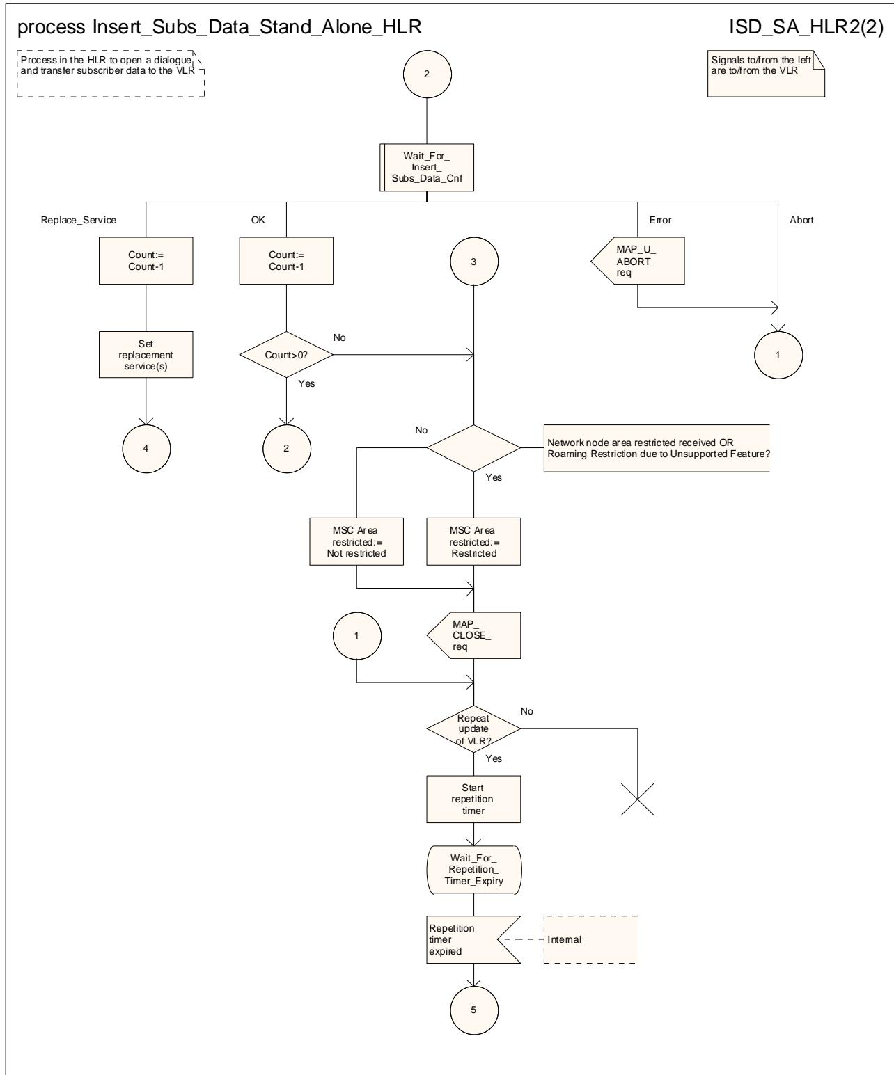
Figure 25.7/3 (sheet 2 of 2): Process Insert\_Subs\_Data\_Stand\_Alone\_HLR
