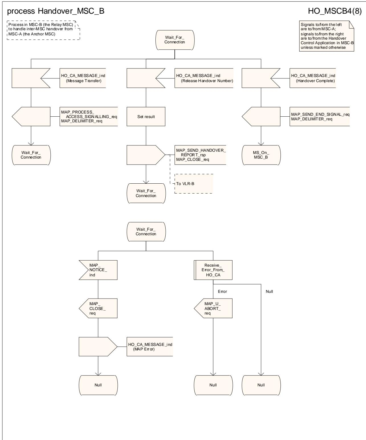
Figure 19.2/5 (sheet 4 of 8): Process HO\_MSC\_B
