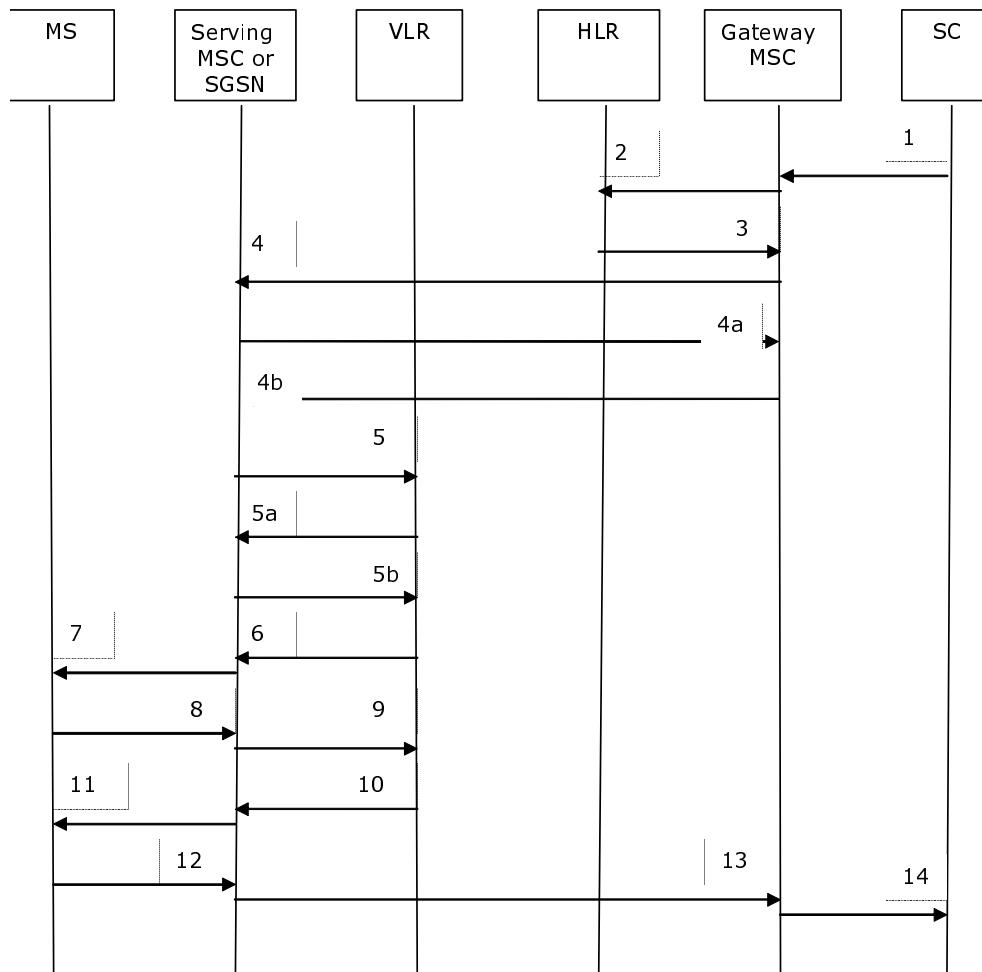
**Figure 23.3/1: Mobile terminated short message service procedures**
