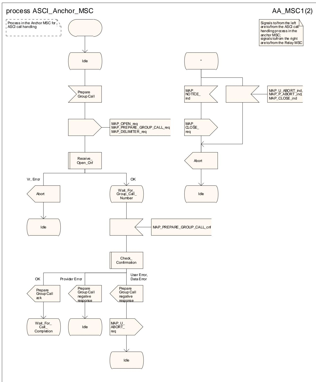
Figure 21.4/2 (sheet 1 of 2): Process ASCI\_Anchor\_MSC
