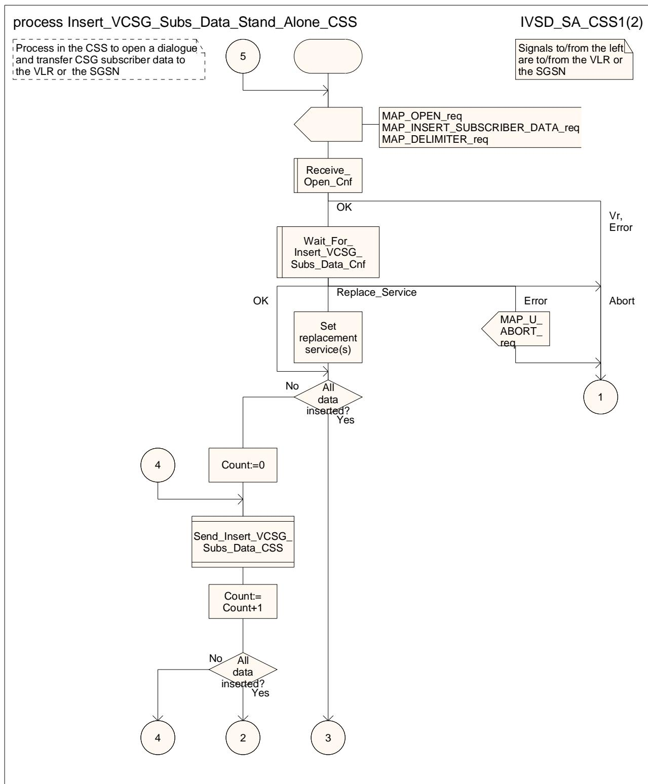
Figure 25.7/8 (sheet 1 of 2): Process Insert\_VCSG\_Subs\_Data\_Stand\_Alone\_CSS
