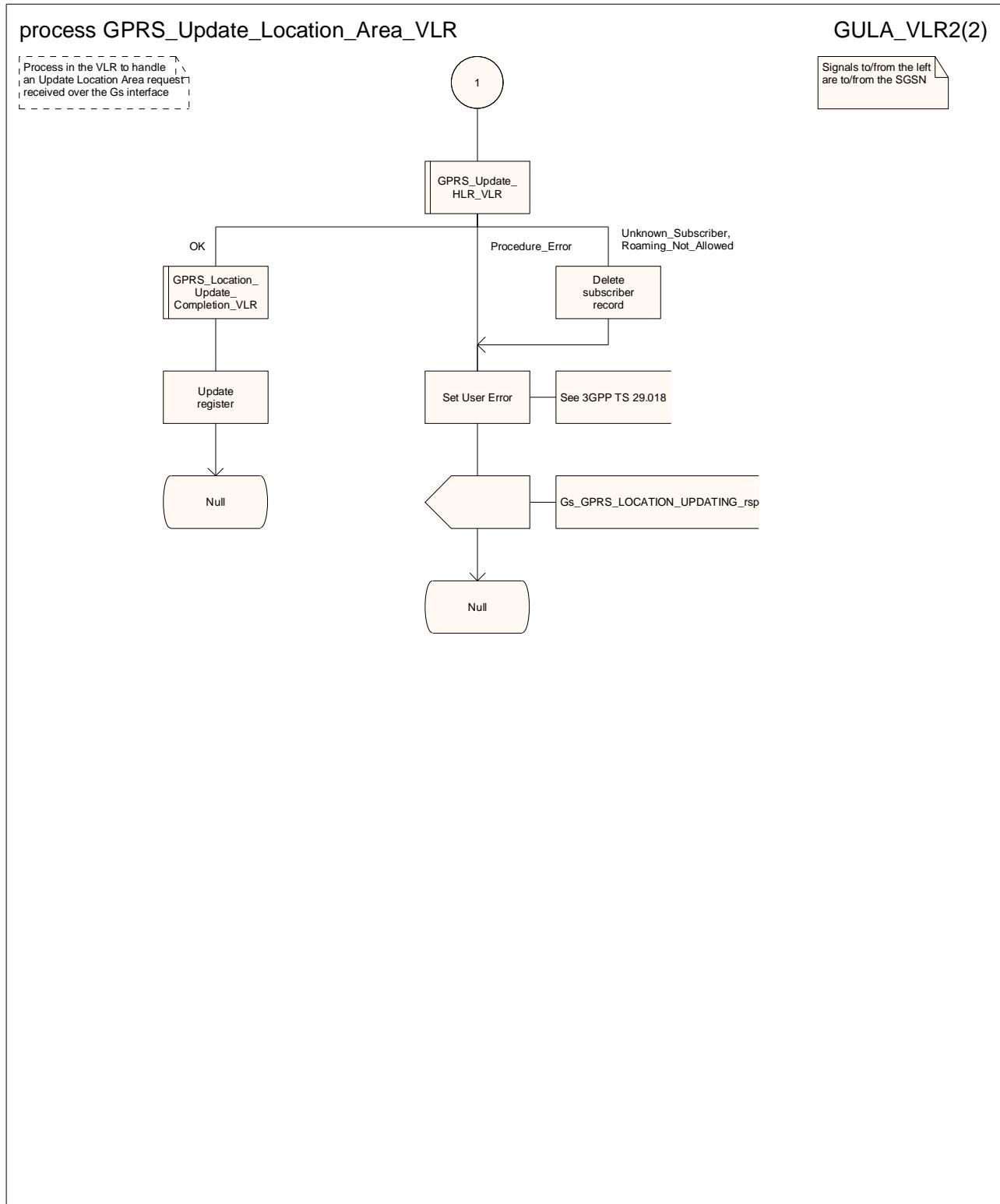
Figure 19.1.1/8 (sheet 2 of 2): Process GPRS\_Update\_Location\_Area\_VLR
