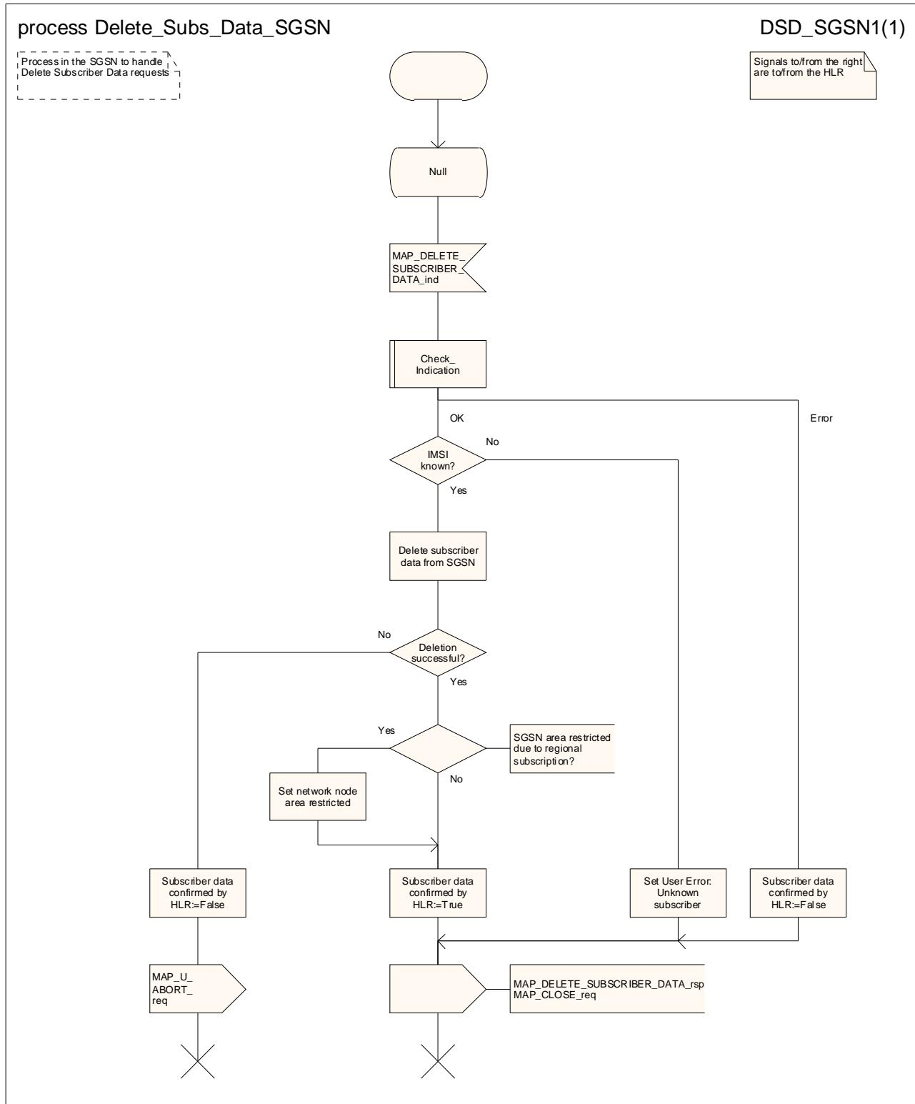
**Figure 20.3/12: Process Delete\_Subs\_Data\_SGSN**
