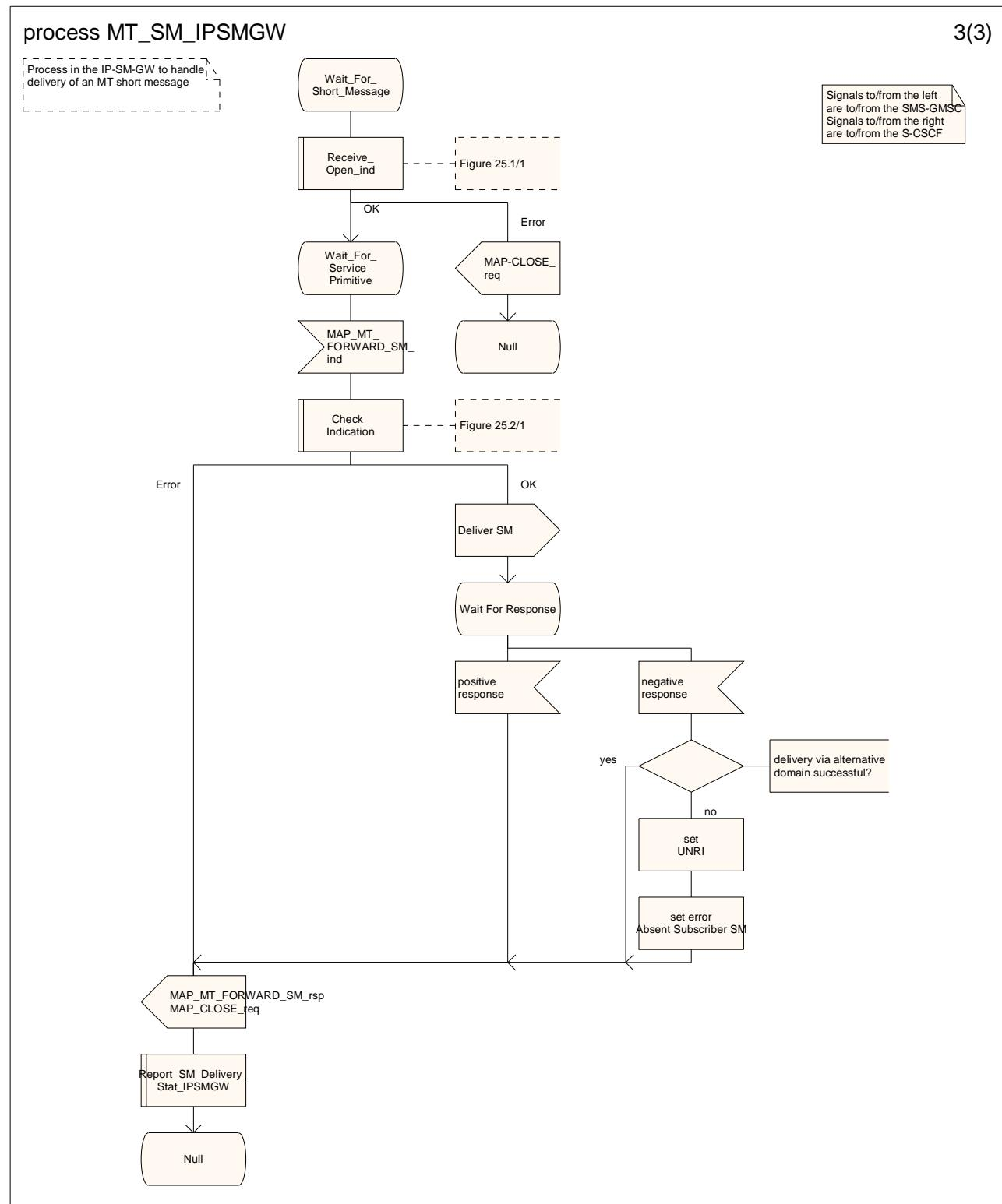
Figure 23.3/15 (sheet 3 of 3): Process MT\_SM\_IPSMGW
