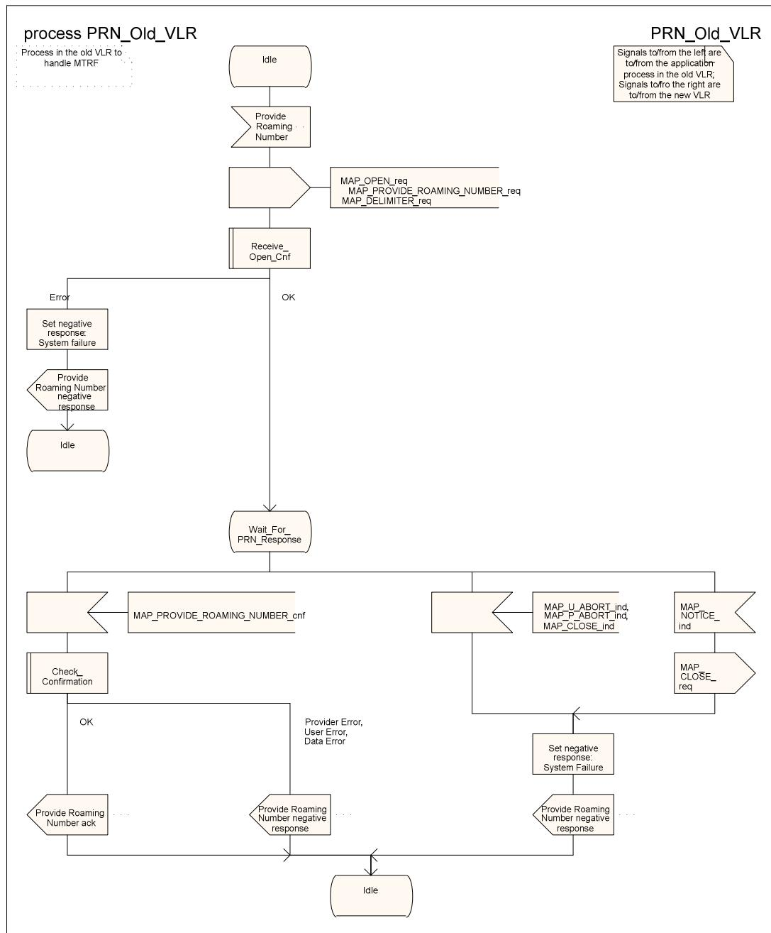
Figure 21.2/11: Process PRN\_Old\_VLR
