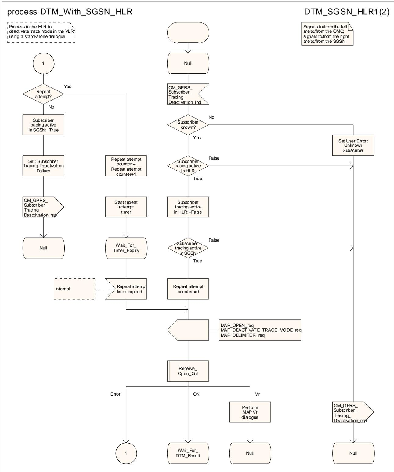
Figure 20.2/13 (sheet 1 of 2): Process DTM\_With\_SGSN\_HLR
