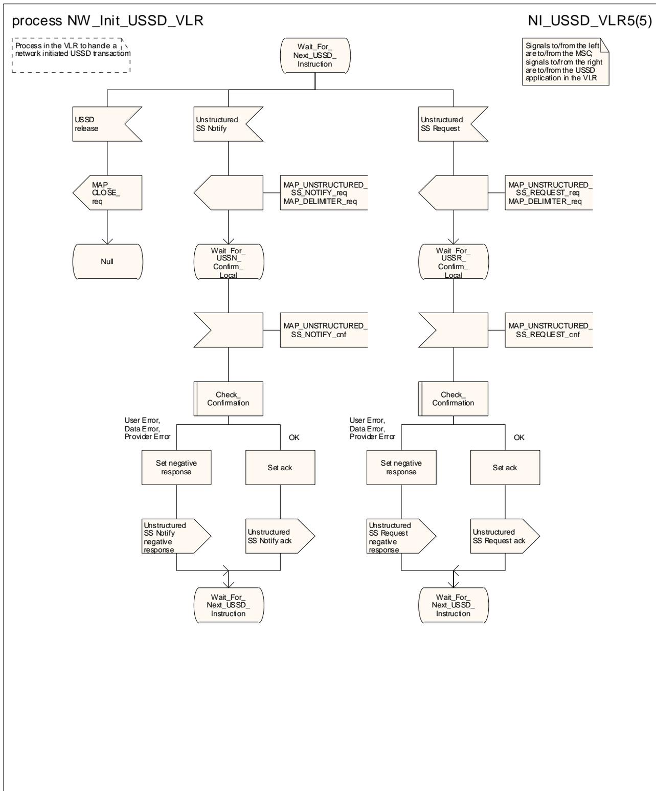
Figure 22.10.3/1 (sheet 5 of 5): Process NW\_Init\_USSD\_VLR
