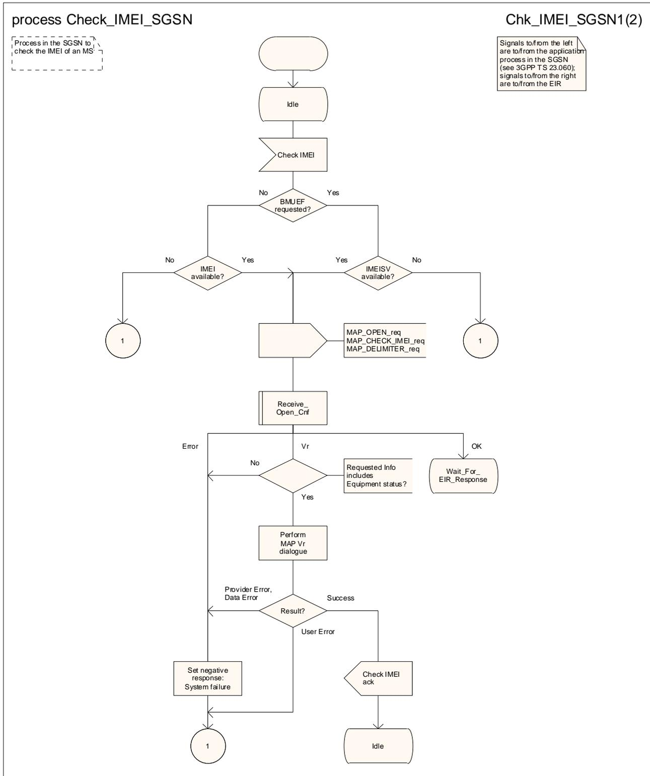
Figure 25.6/3 (sheet 1 of 2): Process Check\_IMEI\_SGSN
