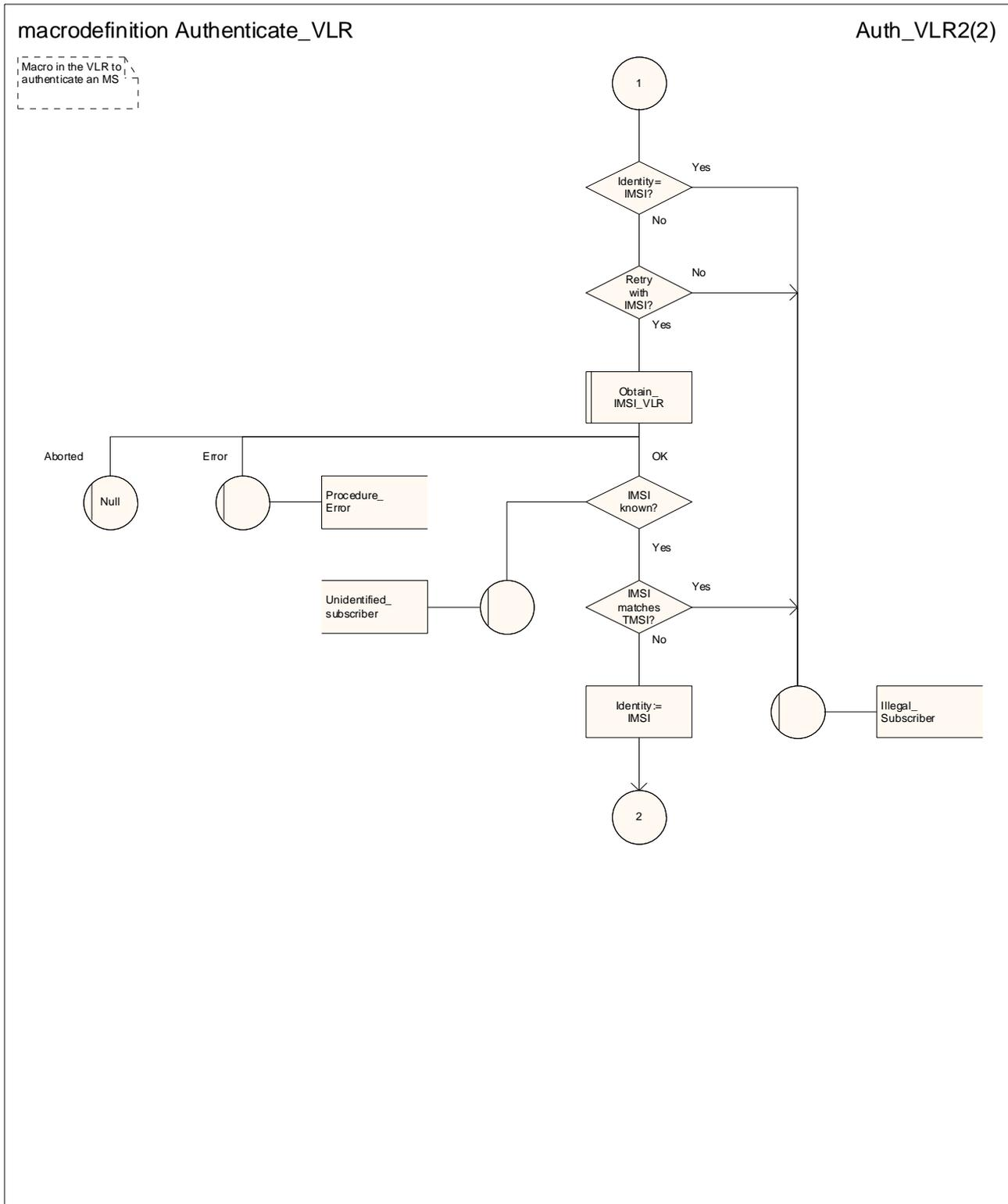
Figure 25.5/2 (sheet 2 of 2): Macro Authenticate\_VLR
