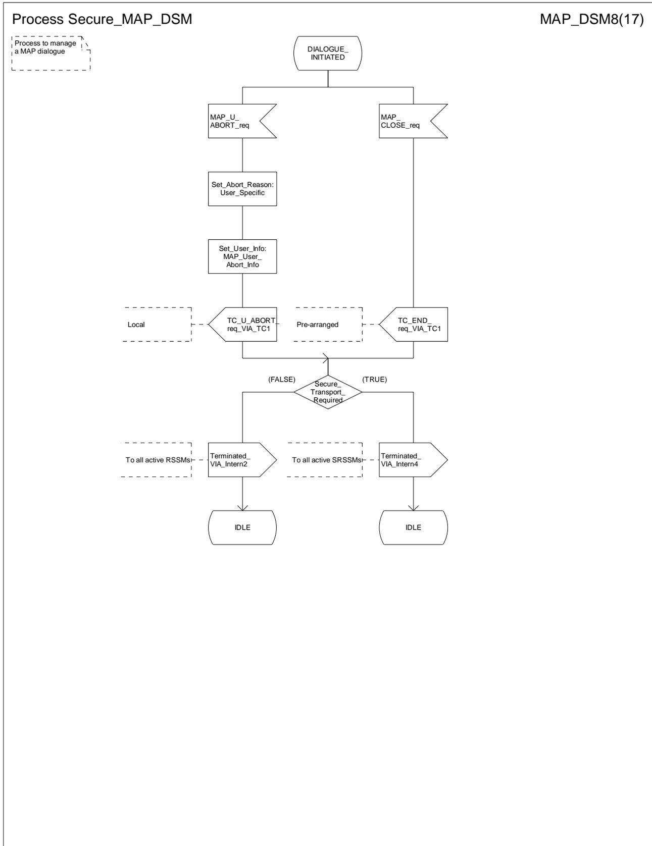
Figure 15.6/3h: Process Secure\_MAP\_DSM (sheet 8)
