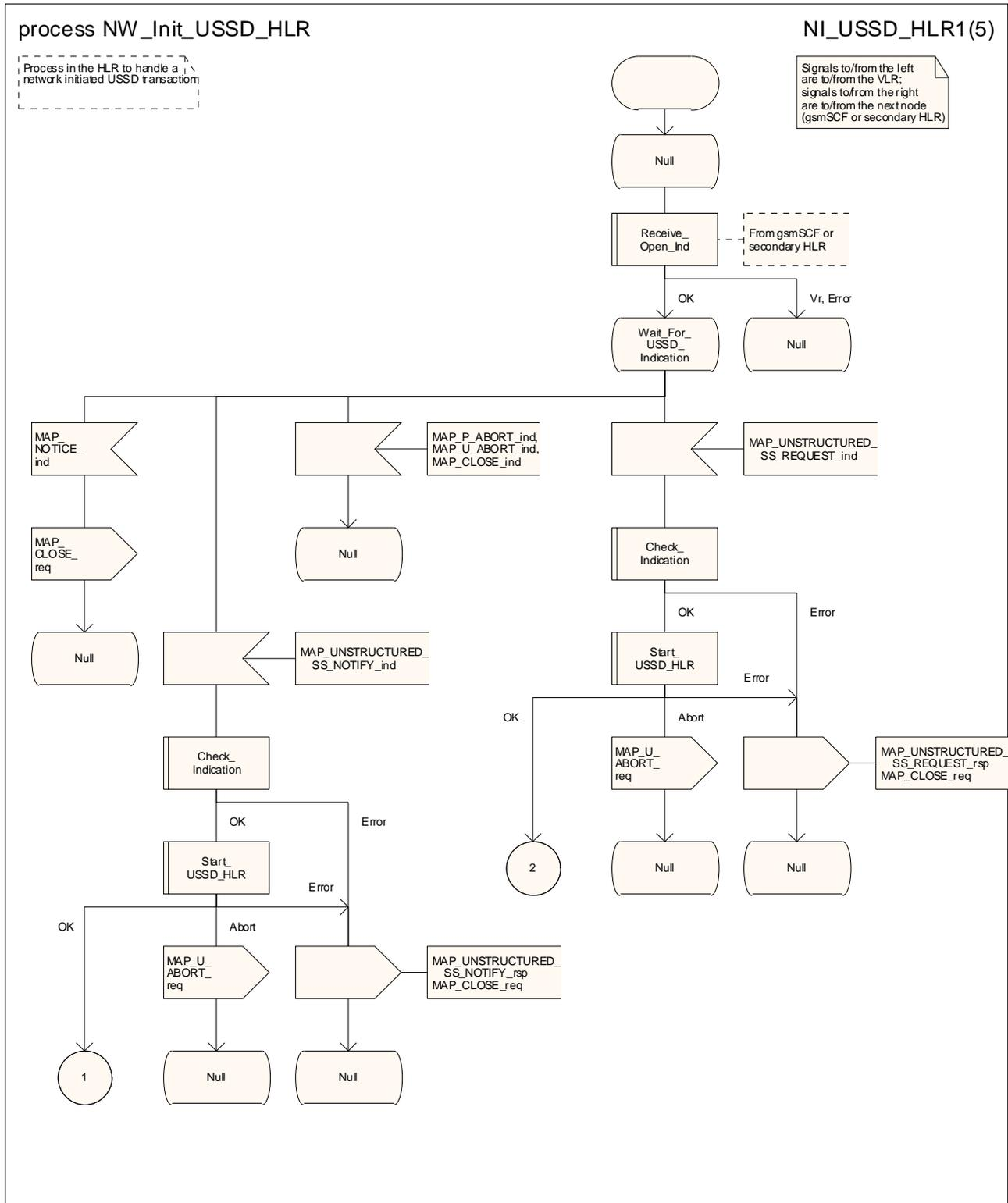
Figure 22.10.4/1 (sheet 1 of 5): Process NW\_Init\_USSD\_HLR
