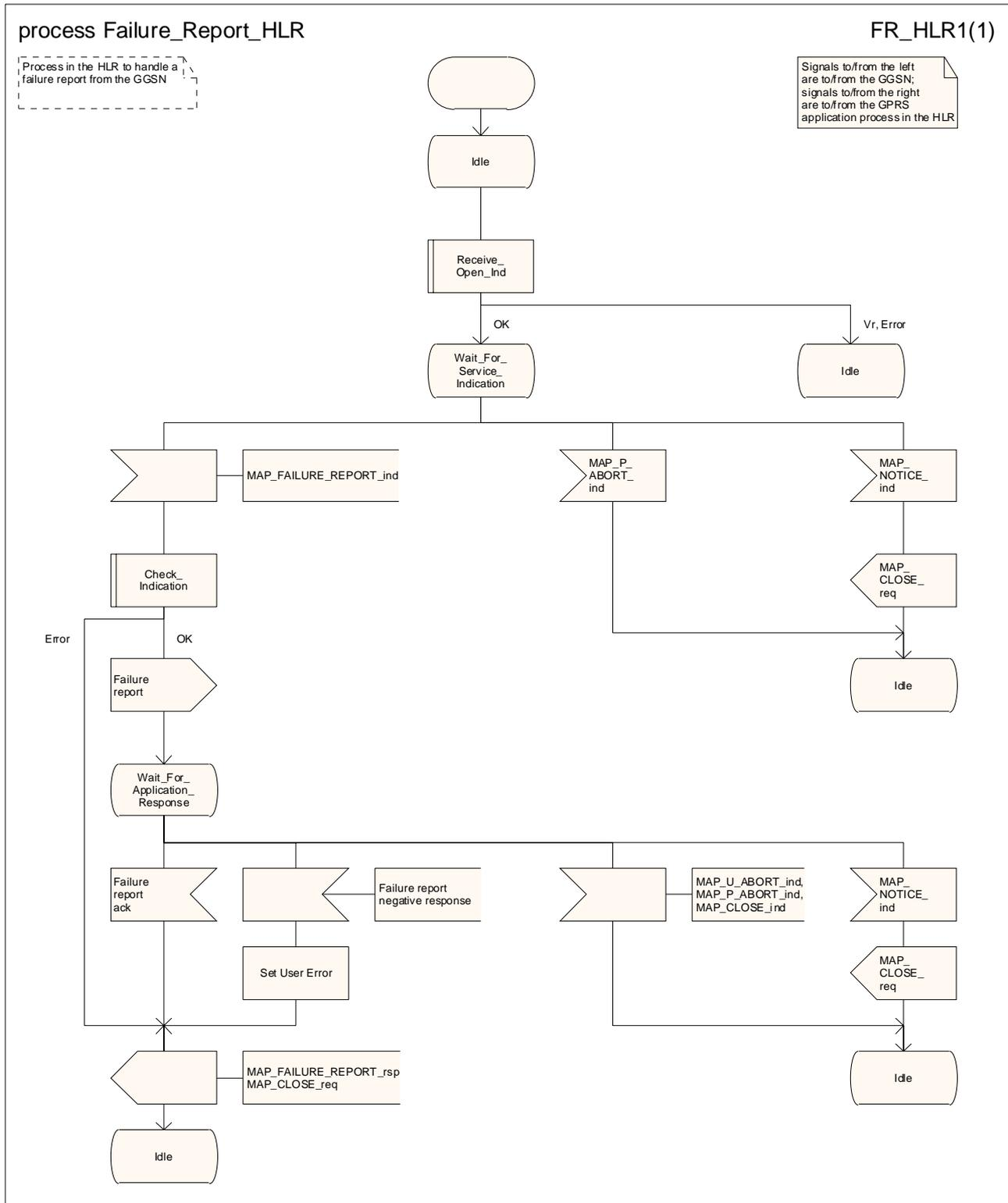
Figure 24.2/2: Process Failure\_Report\_HLR
