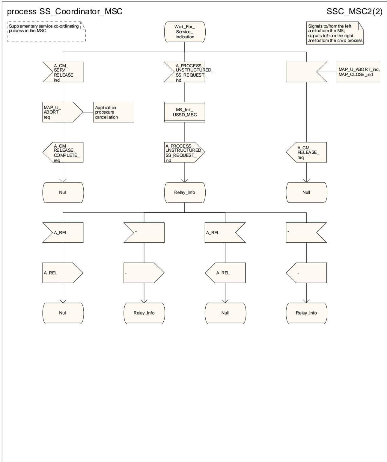
Figure 22.1/1 (sheet 2 of 2): Process SS\_Coordinator\_MSC
