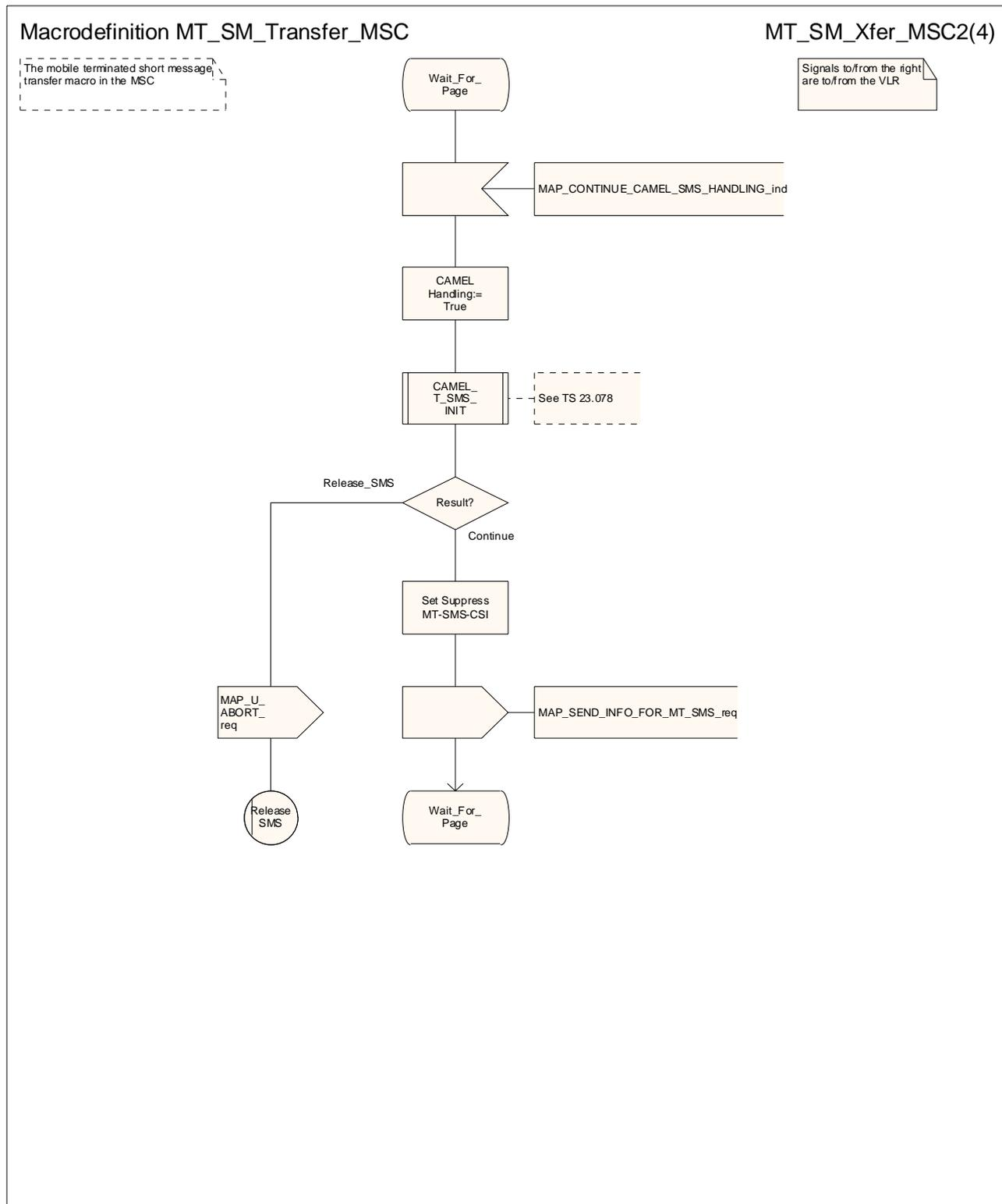
Figure 23.3/7 (sheet 2 of 4): Macro MT\_SM\_Transfer\_MSC
