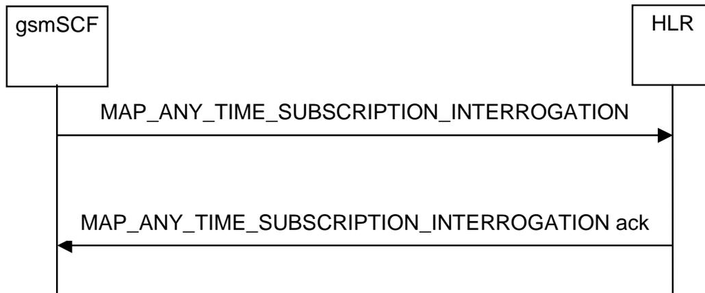
**Figure 24A.2/1: Message flow for any time subscription interrogation**
