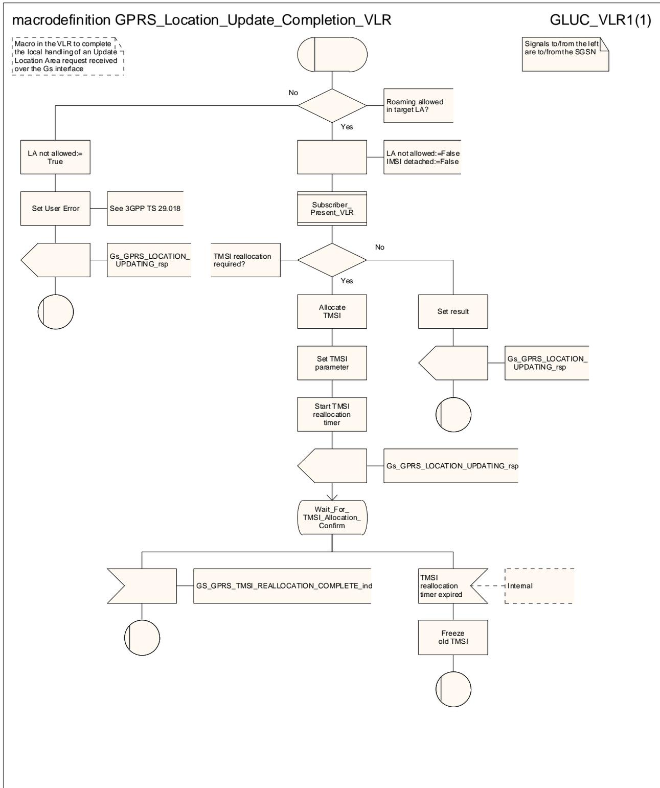
Figure 19.1.1/9: Macro GPRS\_Location\_Update\_Completion\_VLR
