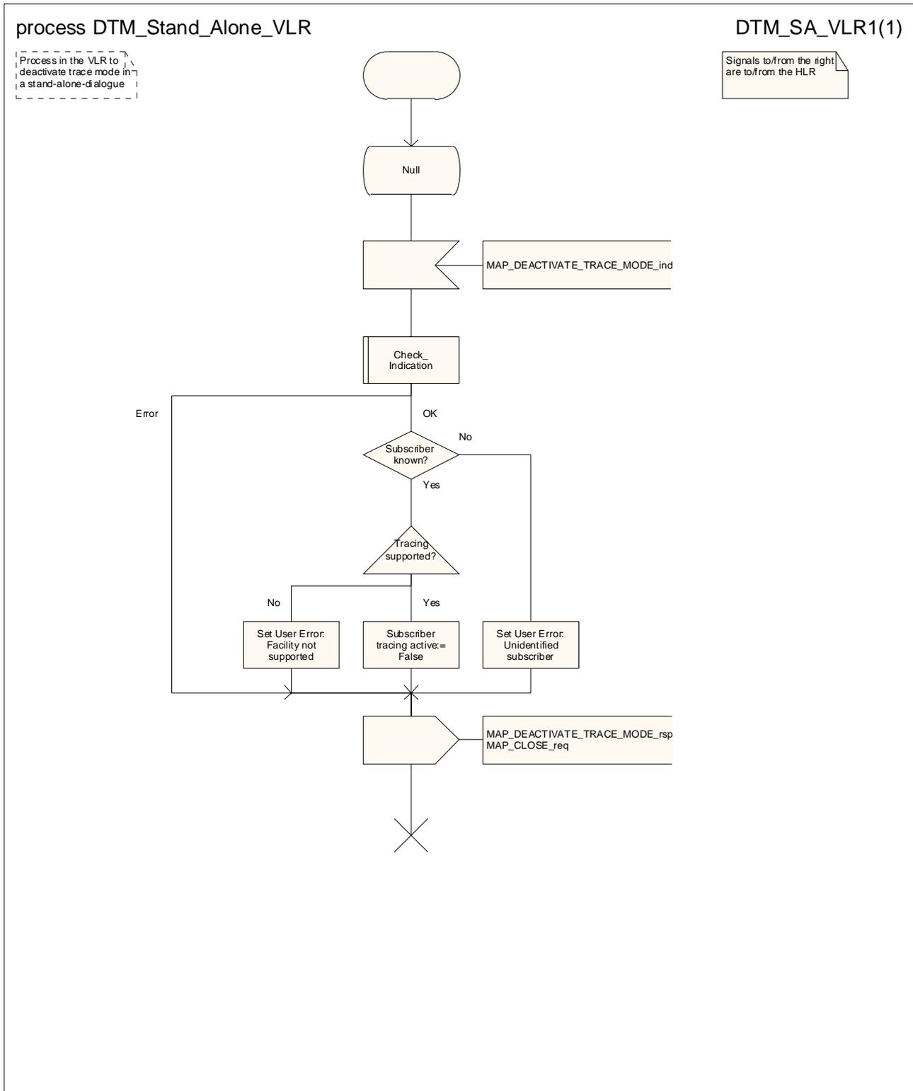
Figure 20.2/14: Process DTM\_Stand\_Alone\_VLR
