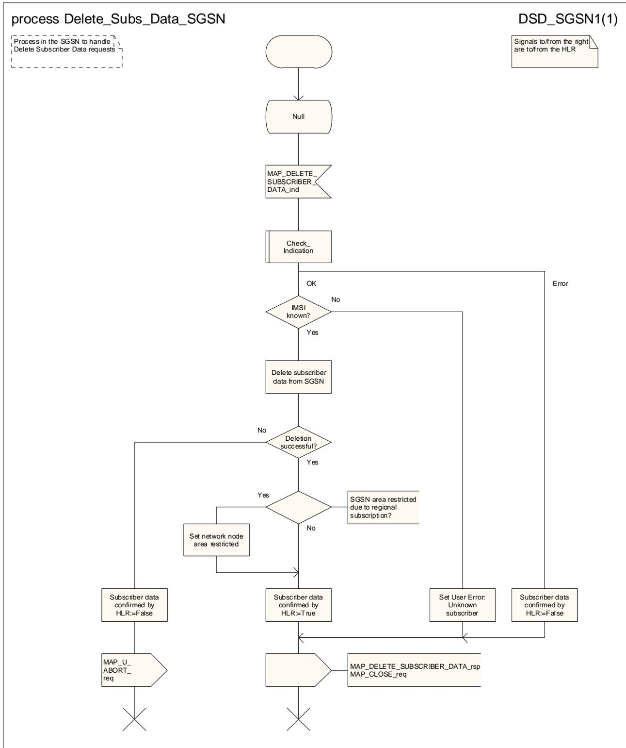
Figure 20.3/12: Process Delete\_Subs\_Data\_SGSN
