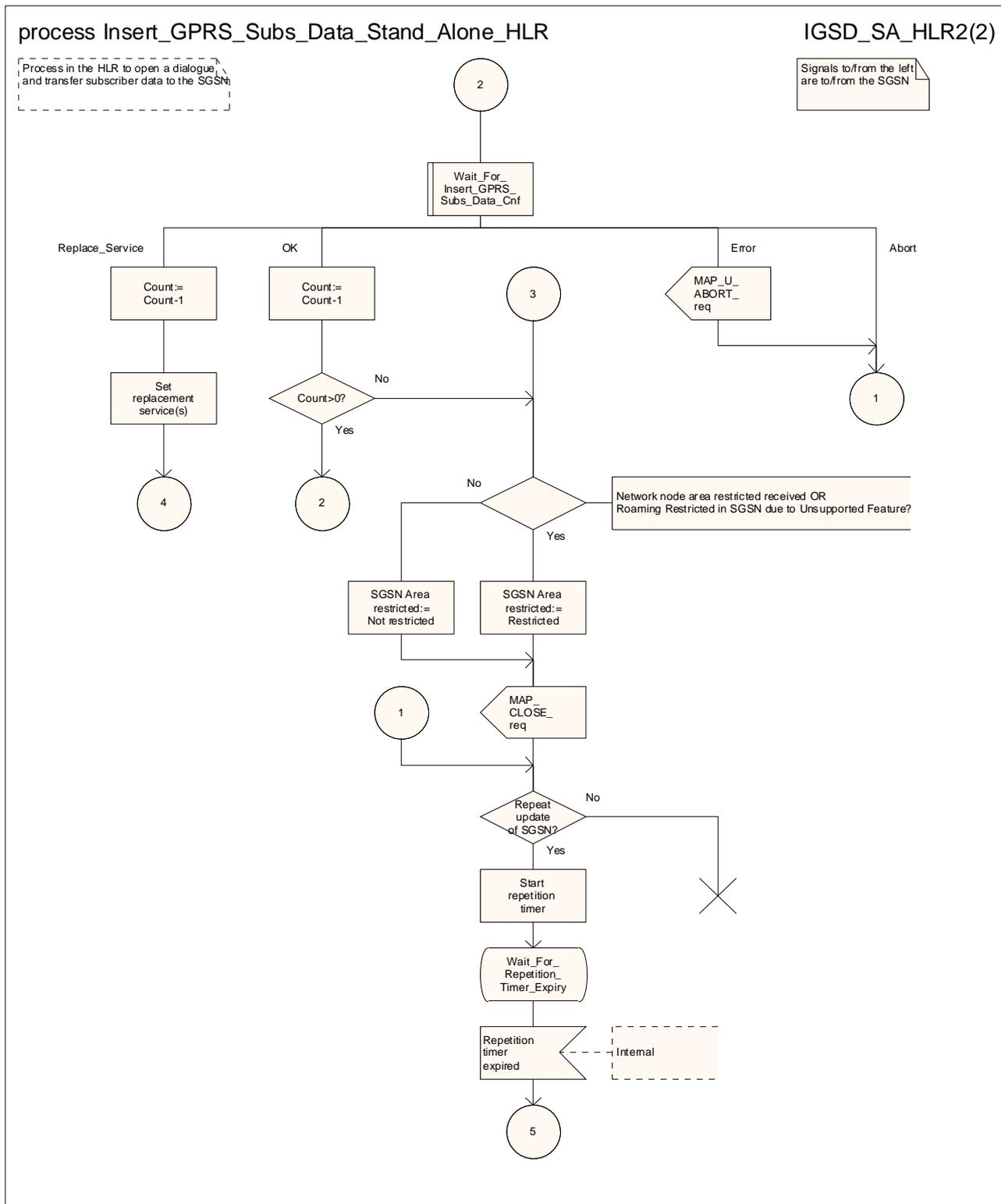
Figure 25.7/4 (sheet 2 of 2): Process Insert\_GPRS\_Subst\_Data\_Stand\_Alone\_HLR
