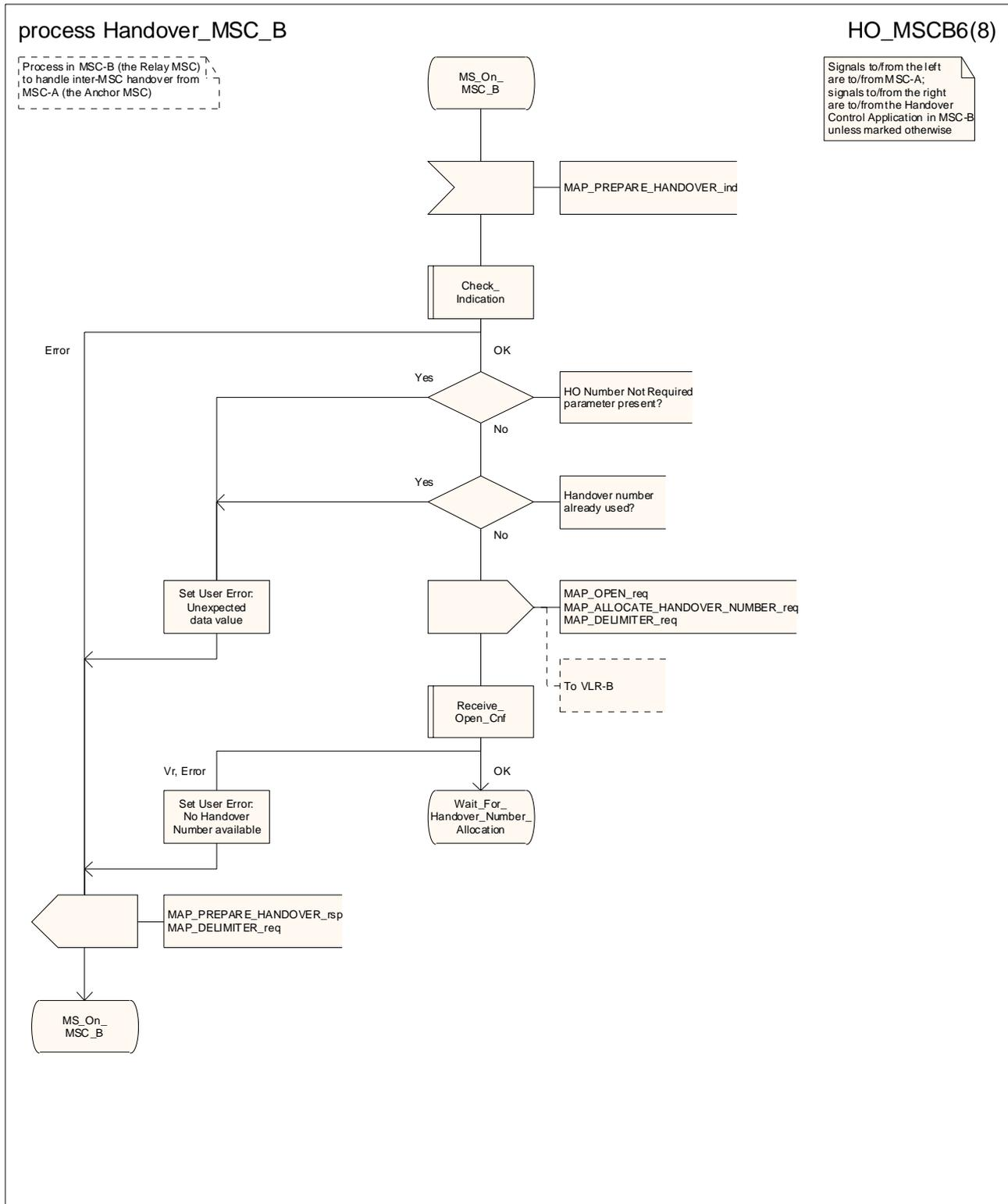
Figure 19.2/5 (sheet 6 of 8): Process HO\_MSC\_B
