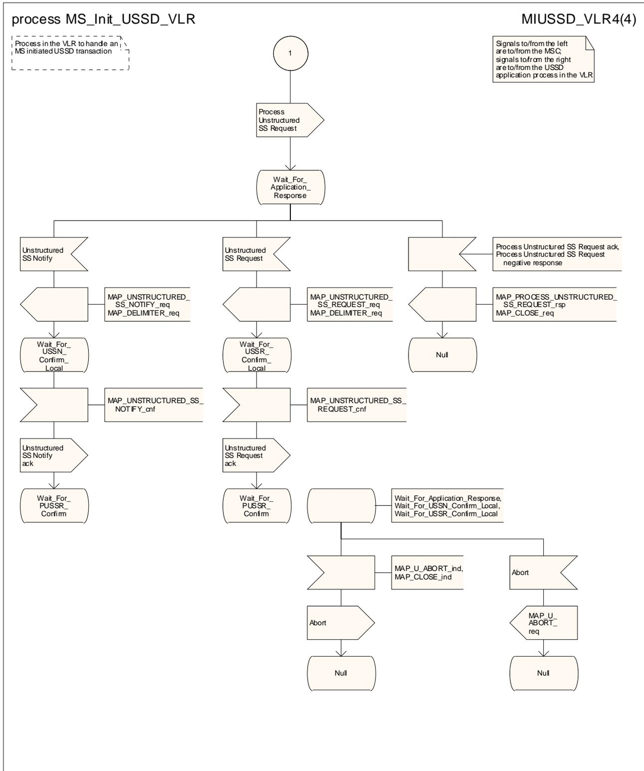
Figure 22.9.3/1 (sheet 4 of 4): Process\_MS\_Init\_USSD\_VLR
