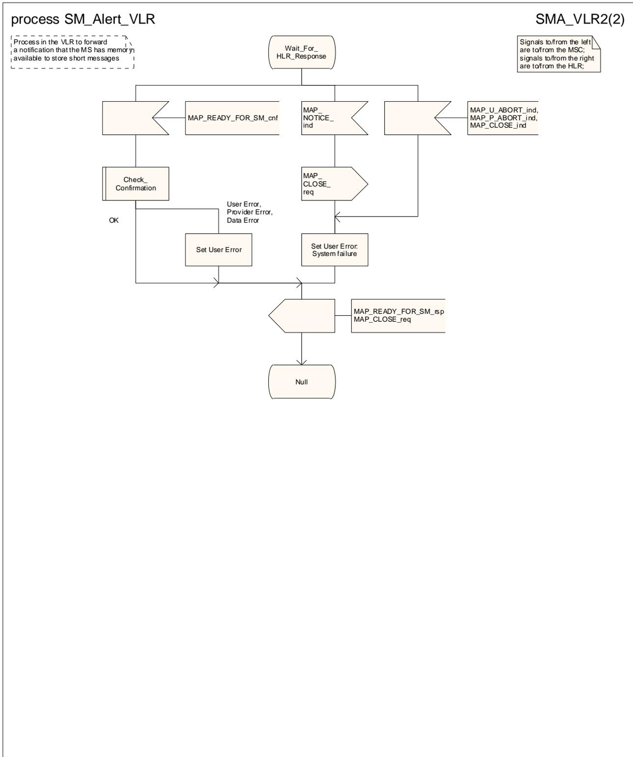
Figure 23.4/5 (sheet 2 of 2): Procedure SM\_Alert\_VLR
