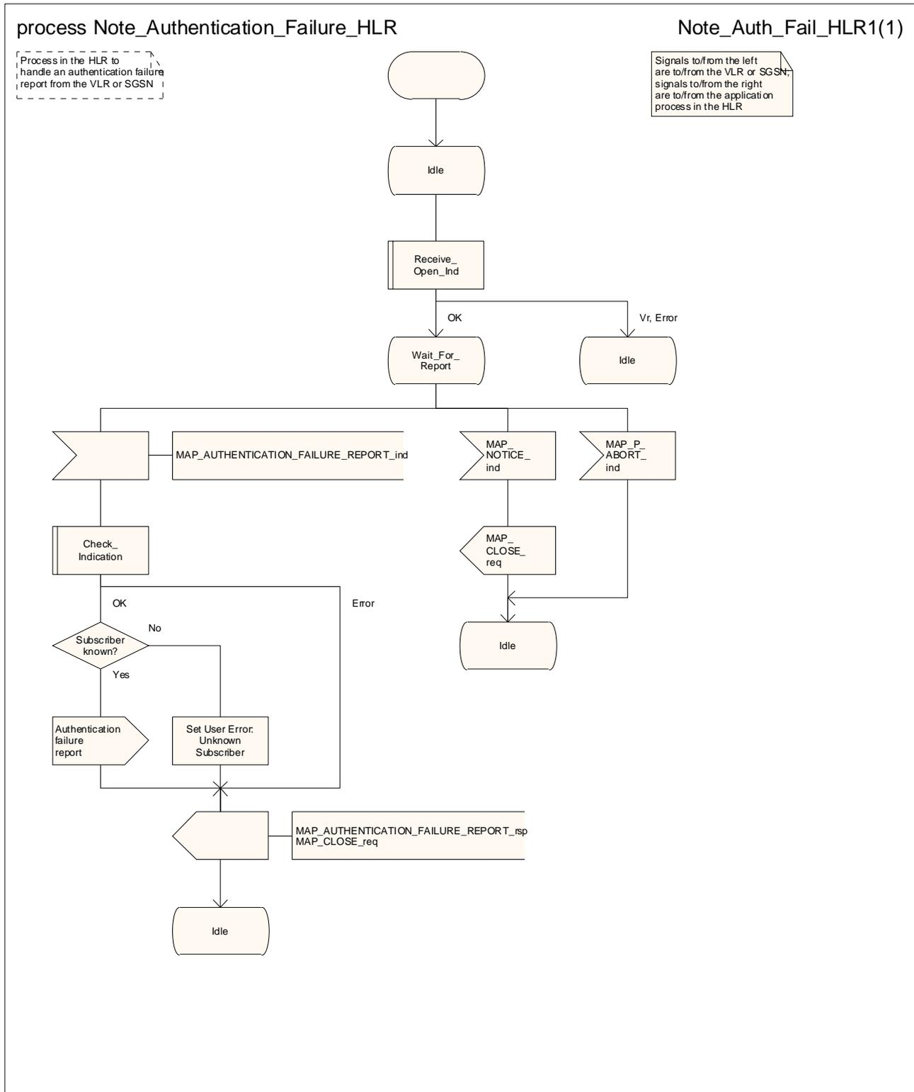
Figure 25.5/11: Process Note\_Authentication\_Failure\_HLR
