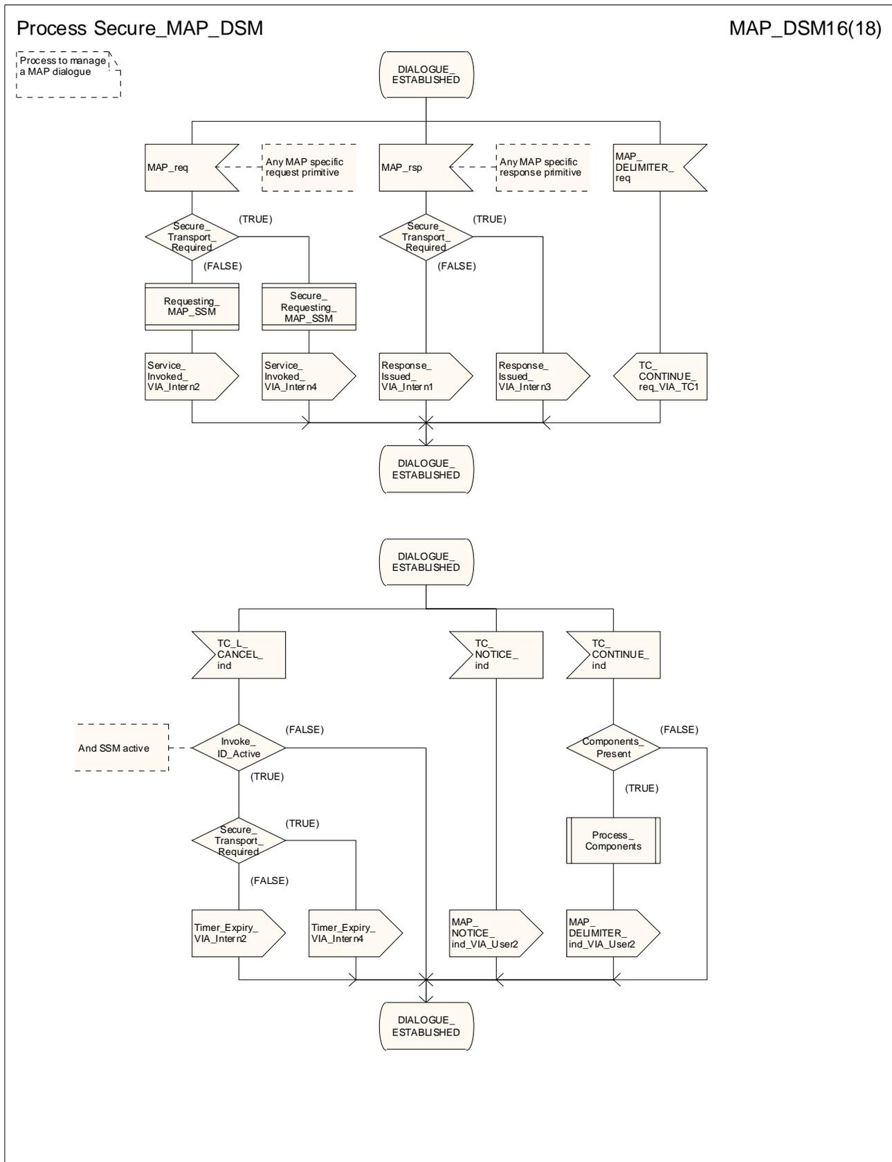
Figure 15.6/3p: Process Secure\_MAP\_DSM (sheet 16)
