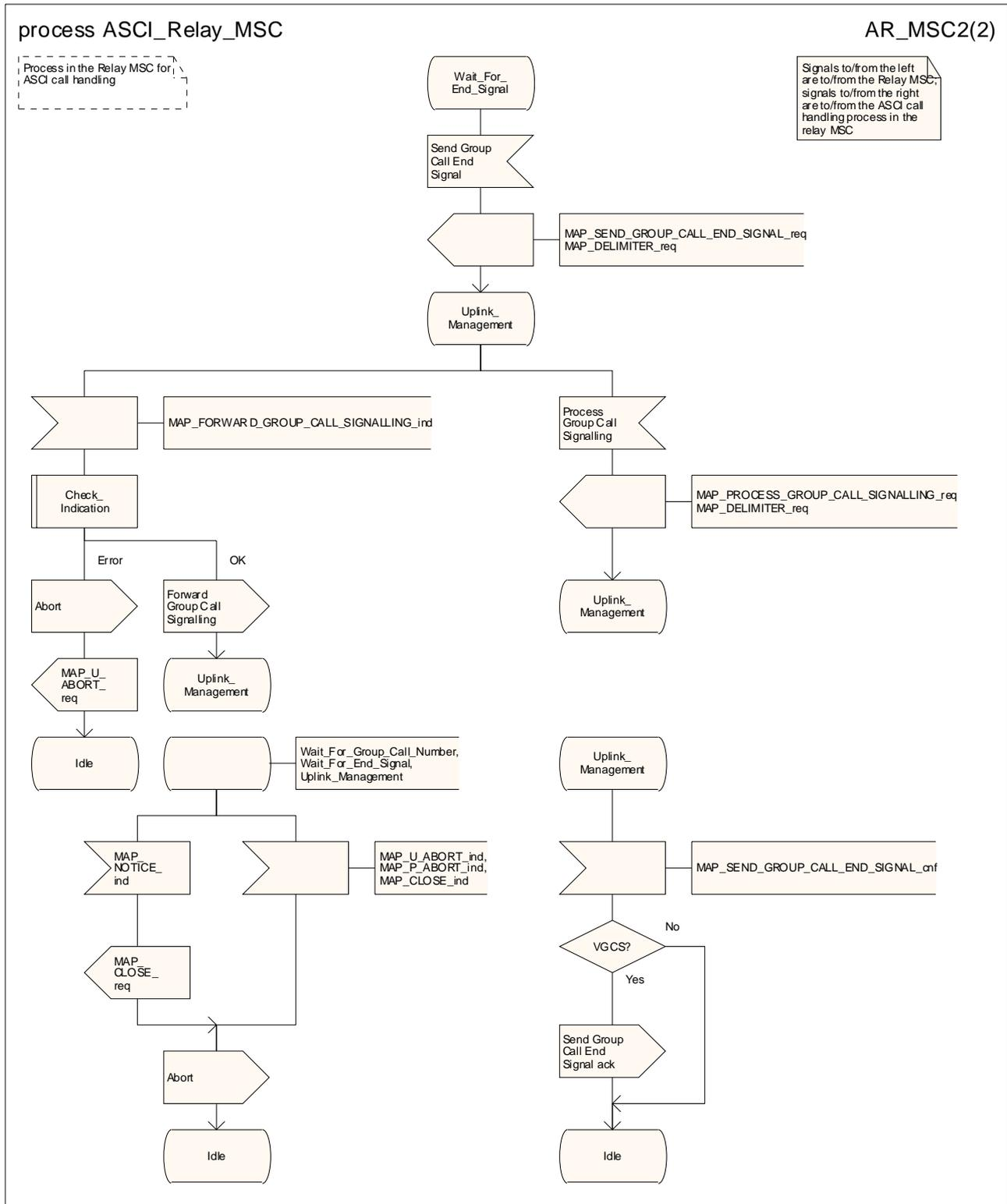
Figure 21.4/3 (sheet 2 of 2): Process ASCII\_Relay\_MSC
