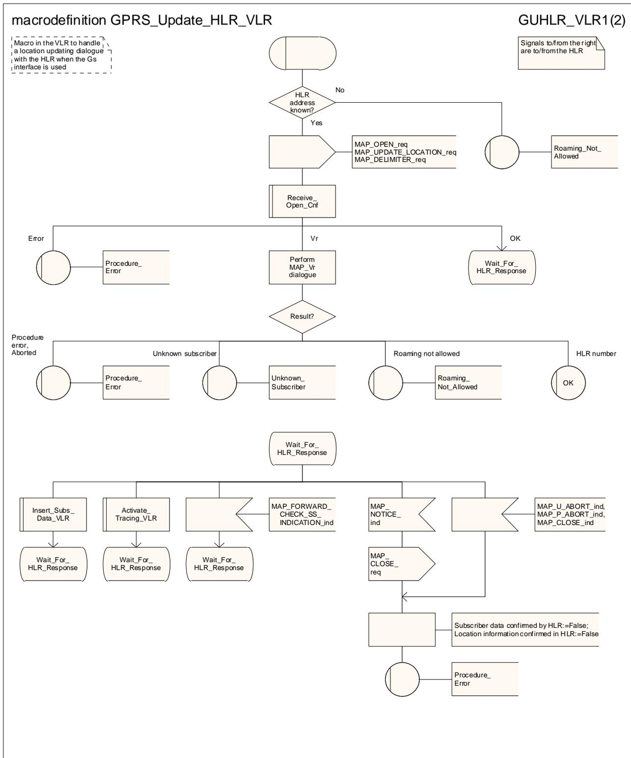
Figure 19.1.1/10 (sheet 1 of 2): Macro GPRS\_Update\_HLR\_VLR
