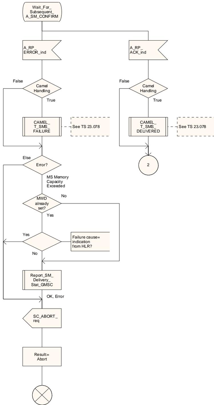
Figure 23.3/4 (sheet 2 of 8): Procedure MT\_SM\_Delivery\_Attempt\_GMSC
