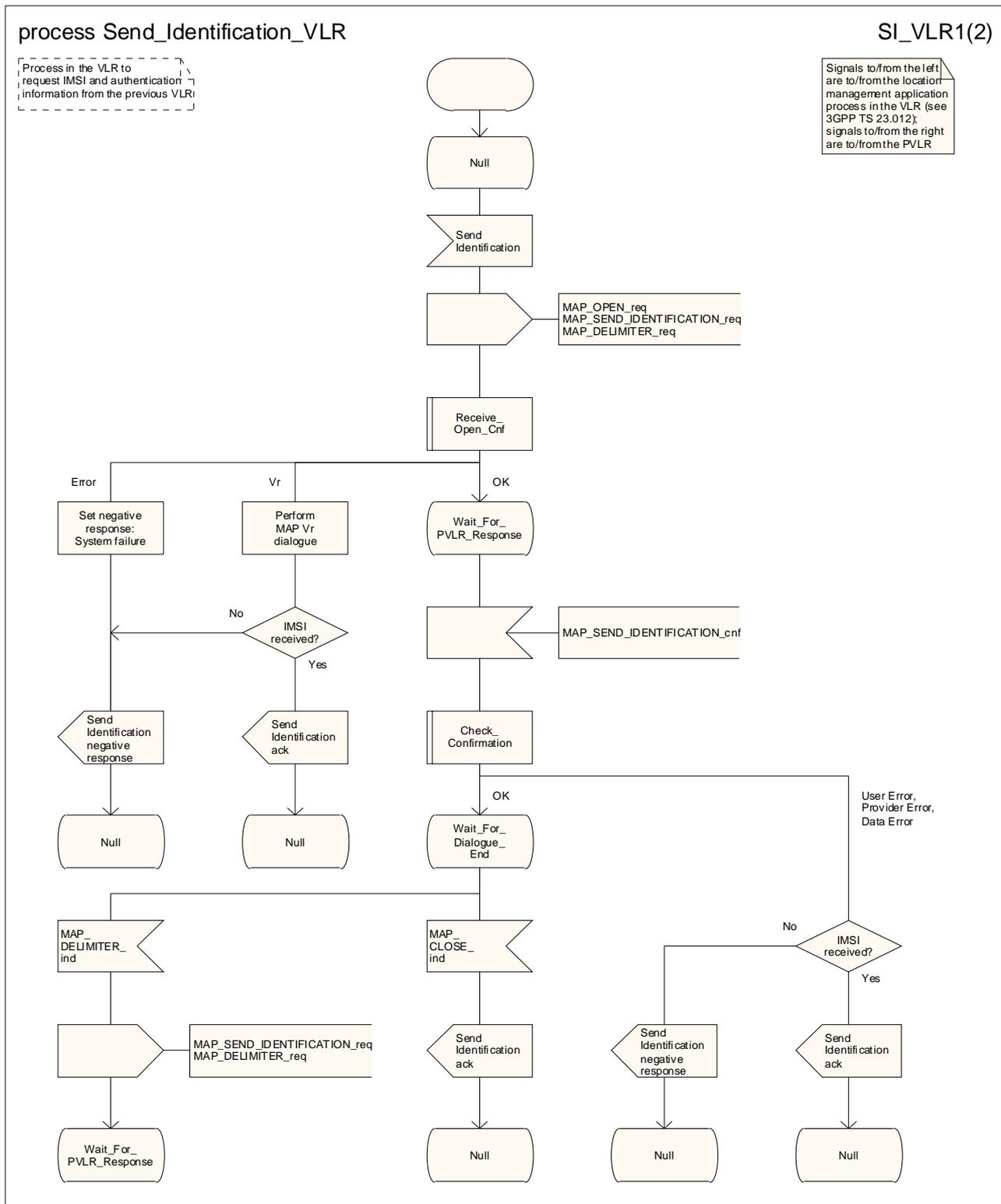
Figure 19.1.1/7 (sheet 1 of 2): Process Send\_Identification\_VLR
