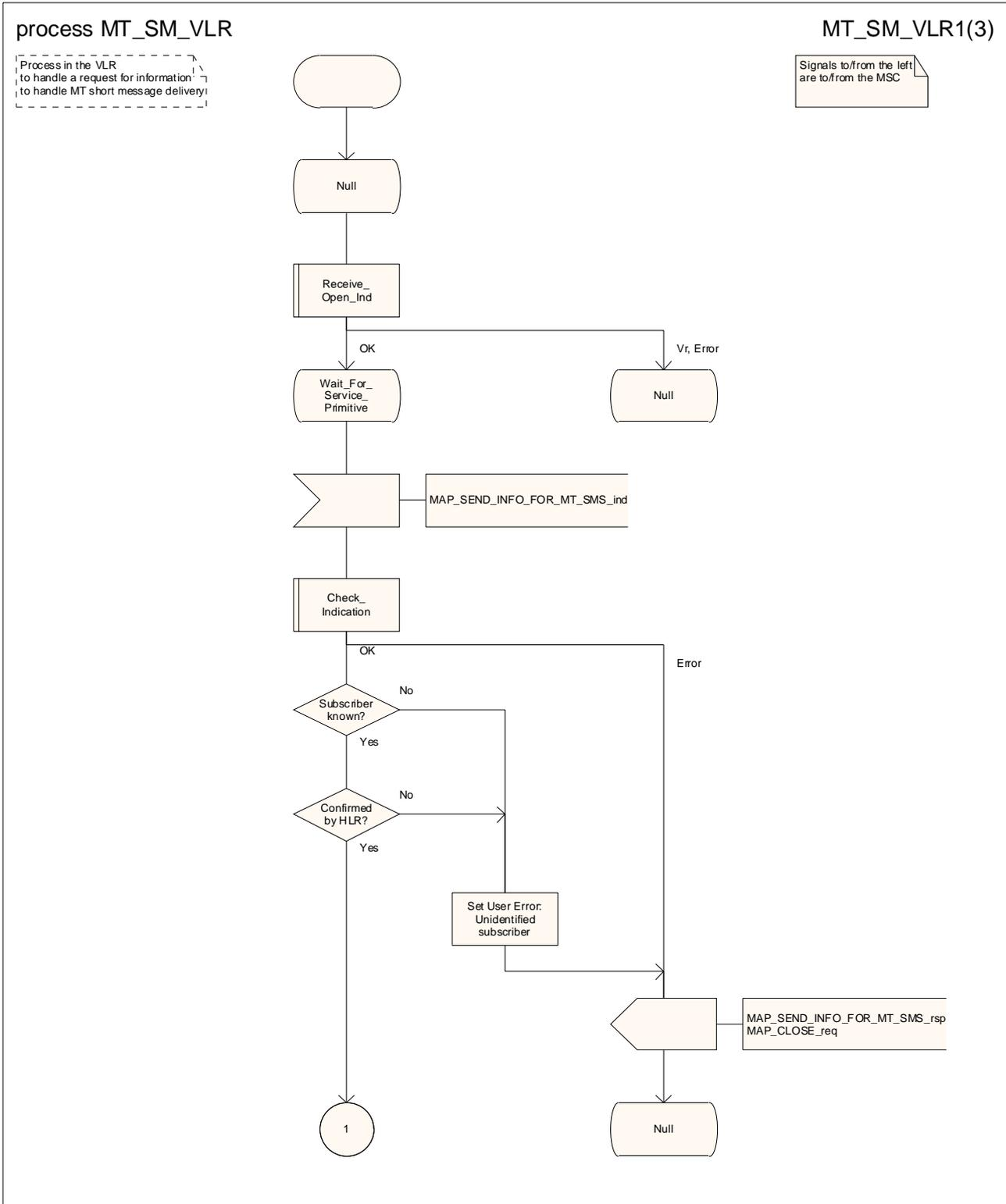
Figure 23.3/9 (sheet 1 of 3): Process MT\_SM\_VLR
