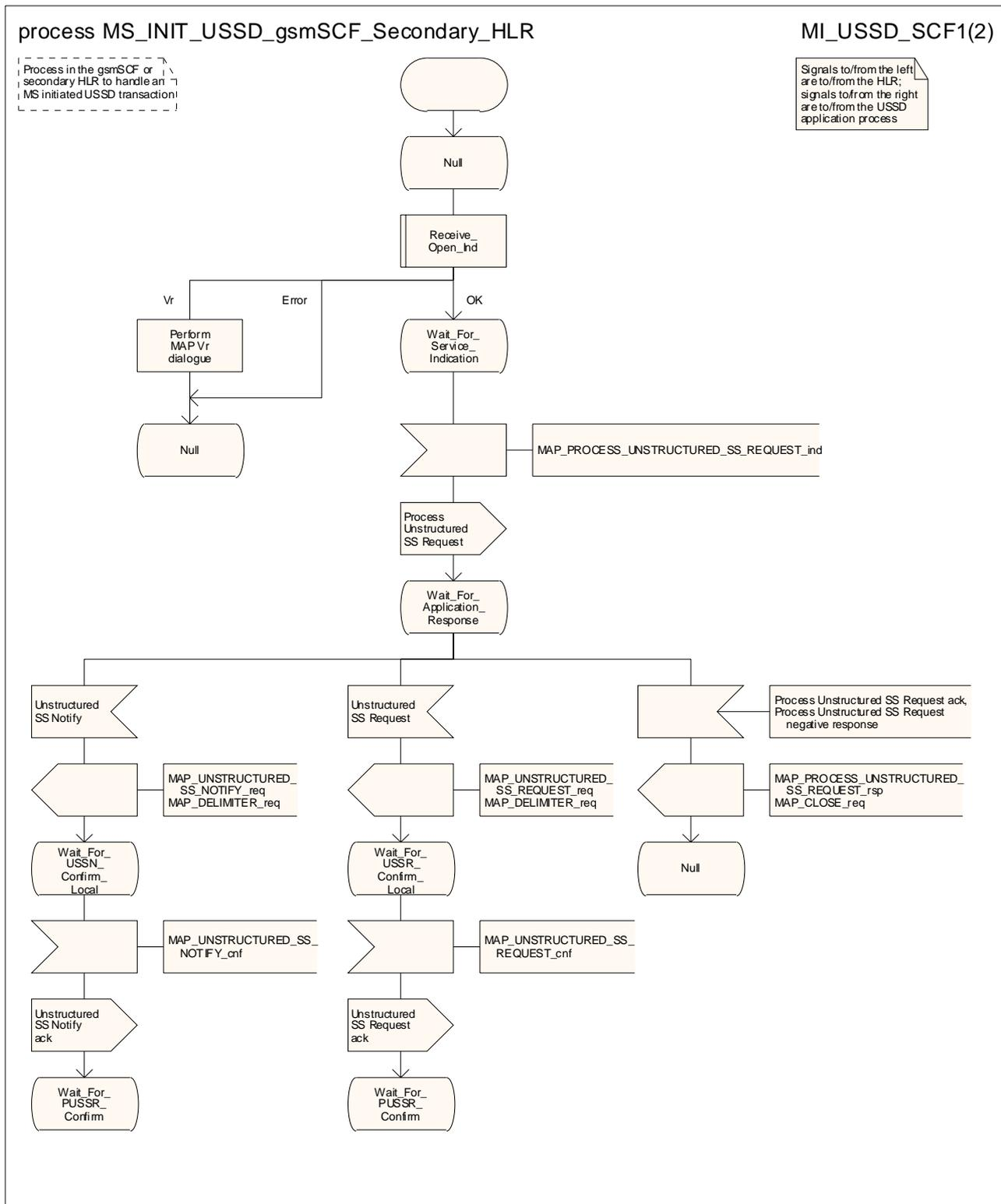
Figure 22.9.5/1 (sheet 1 of 2): Process MS\_Init\_USSD\_gsmSCF\_Secondary\_HLR
