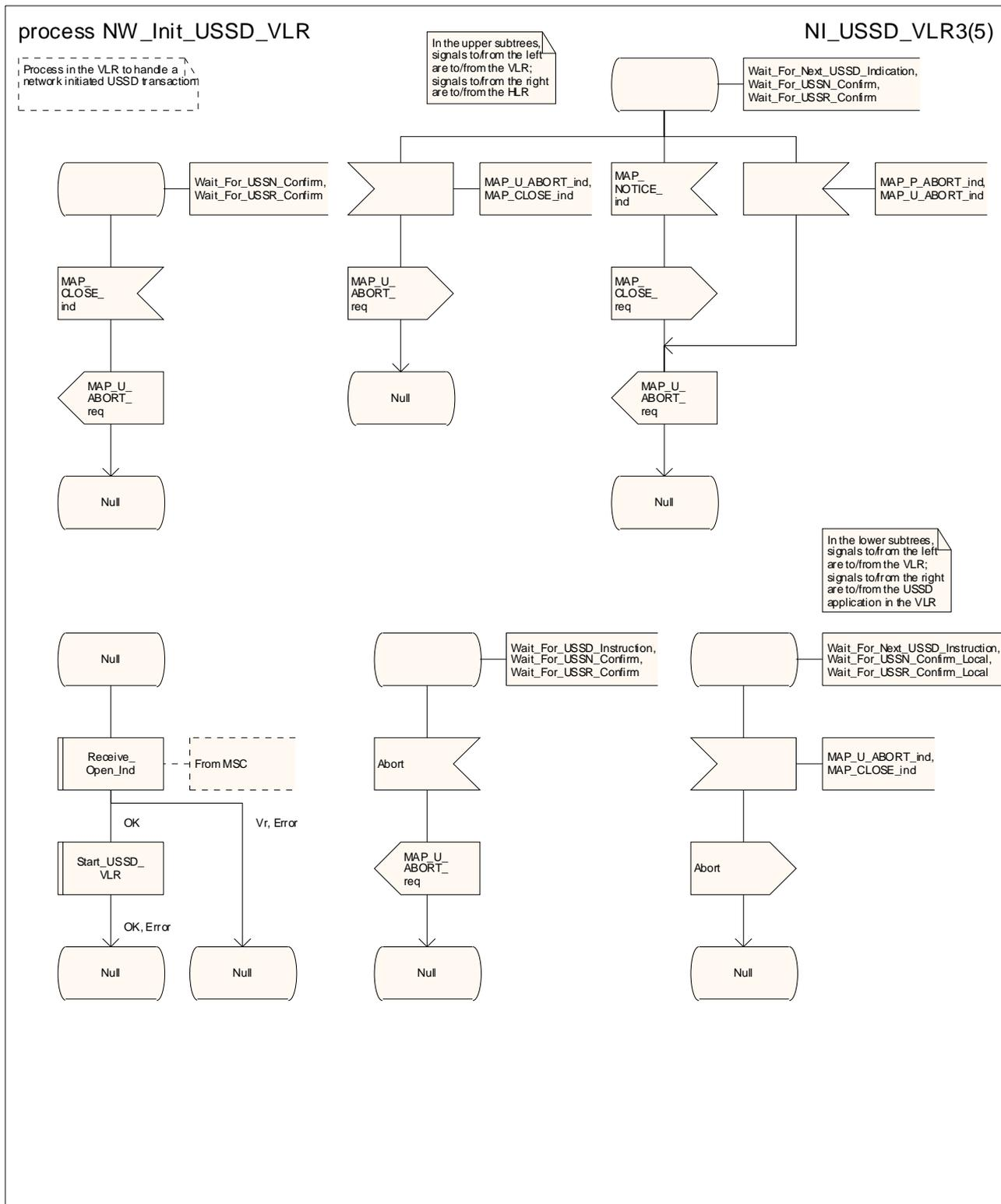
Figure 22.10.3/1 (sheet 3 of 5): Process NW\_Init\_USSD\_VLR
