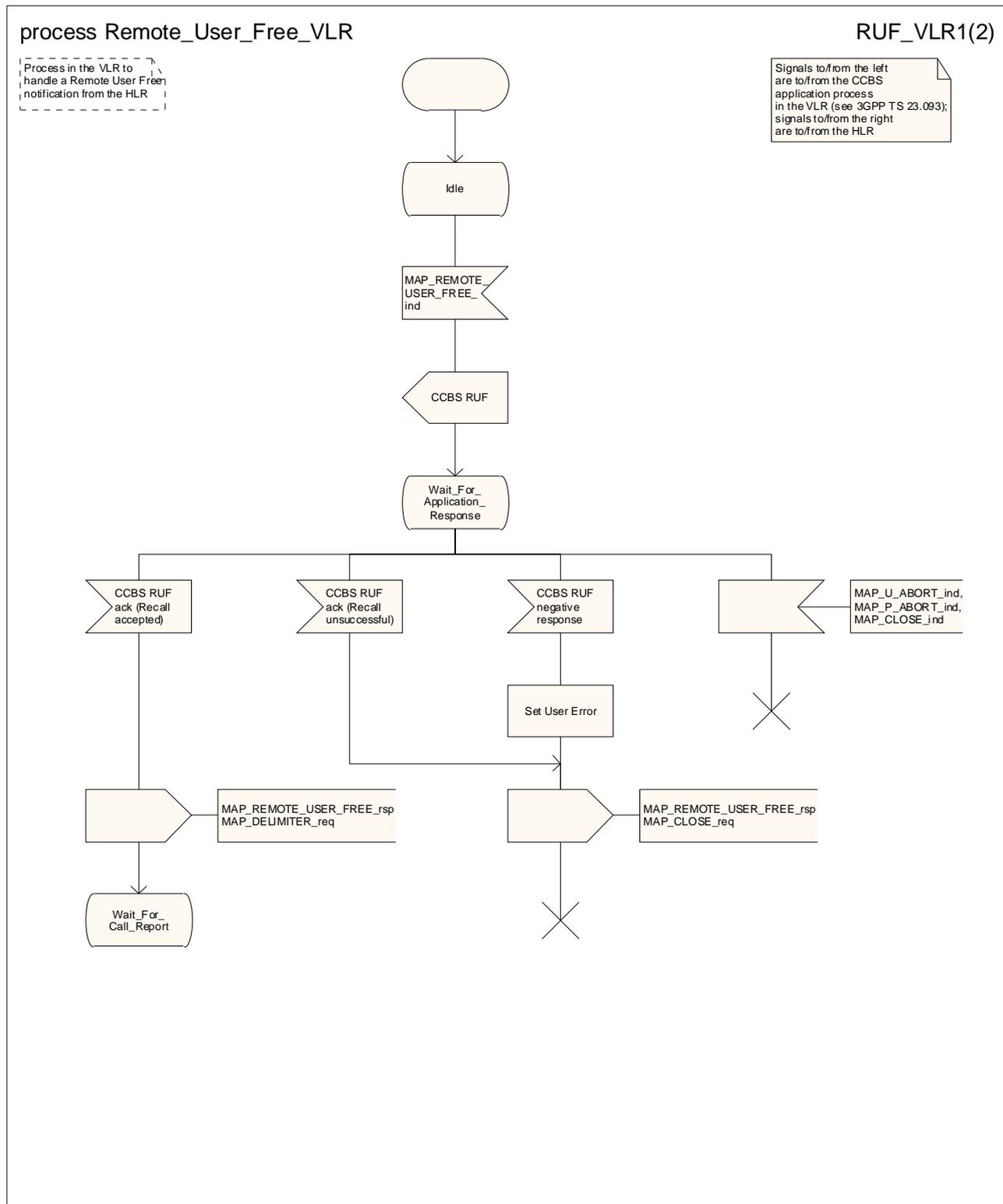
Figure 21.6/15 (sheet 1 of 2): Process Remote\_User\_Free\_VLR
