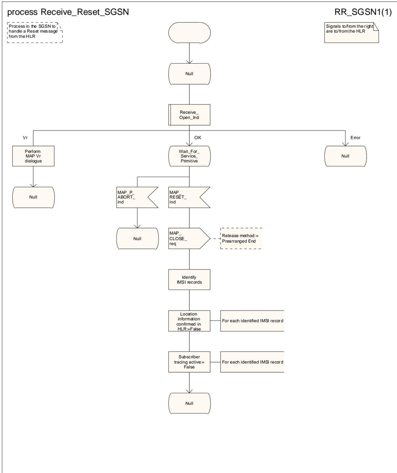
Figure 19.3.2/7: Process Receive\_Reset\_SGSN
