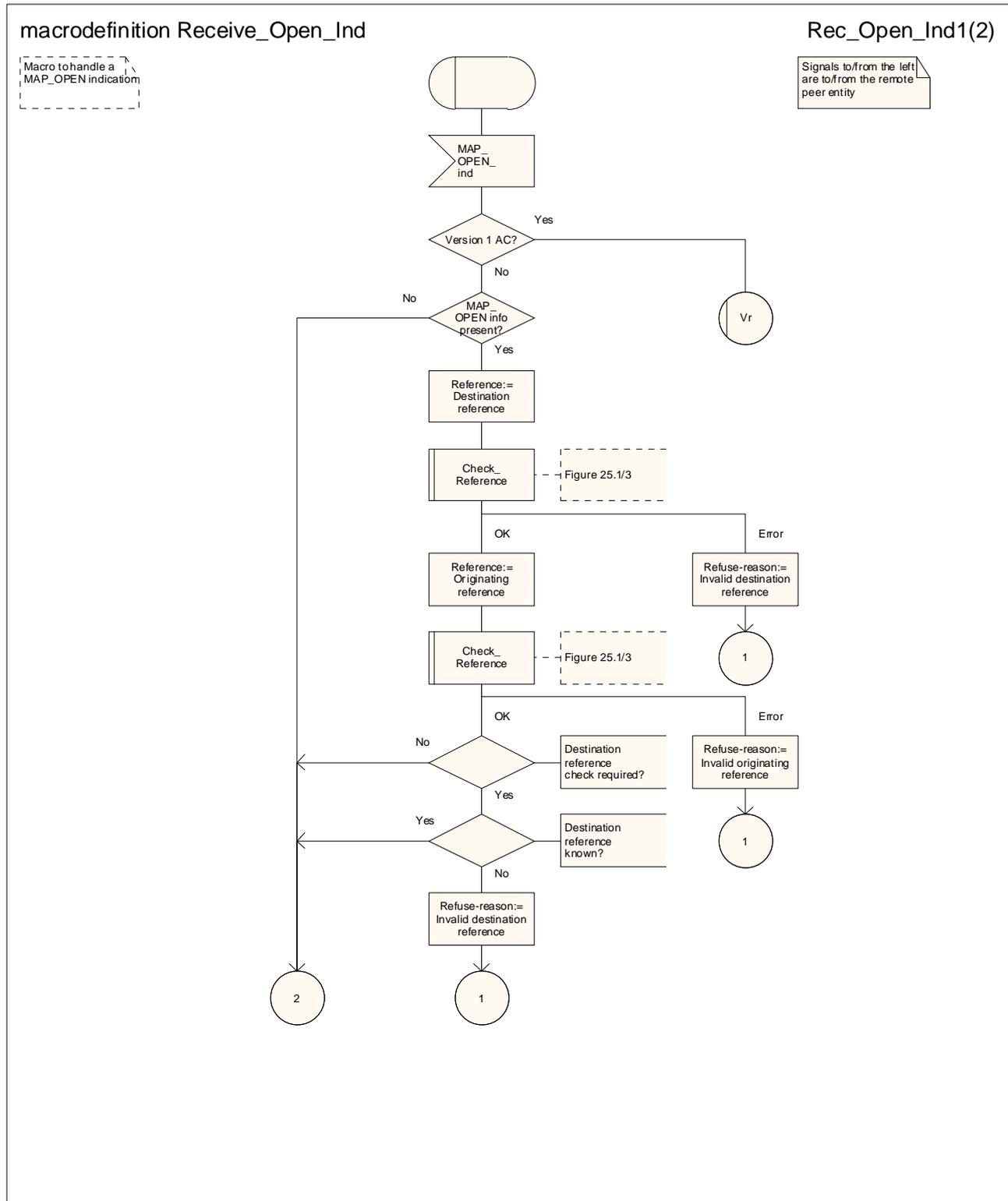
Figure 25.1/1 (sheet 1 of 2): Macro Receive\_Open\_Ind
