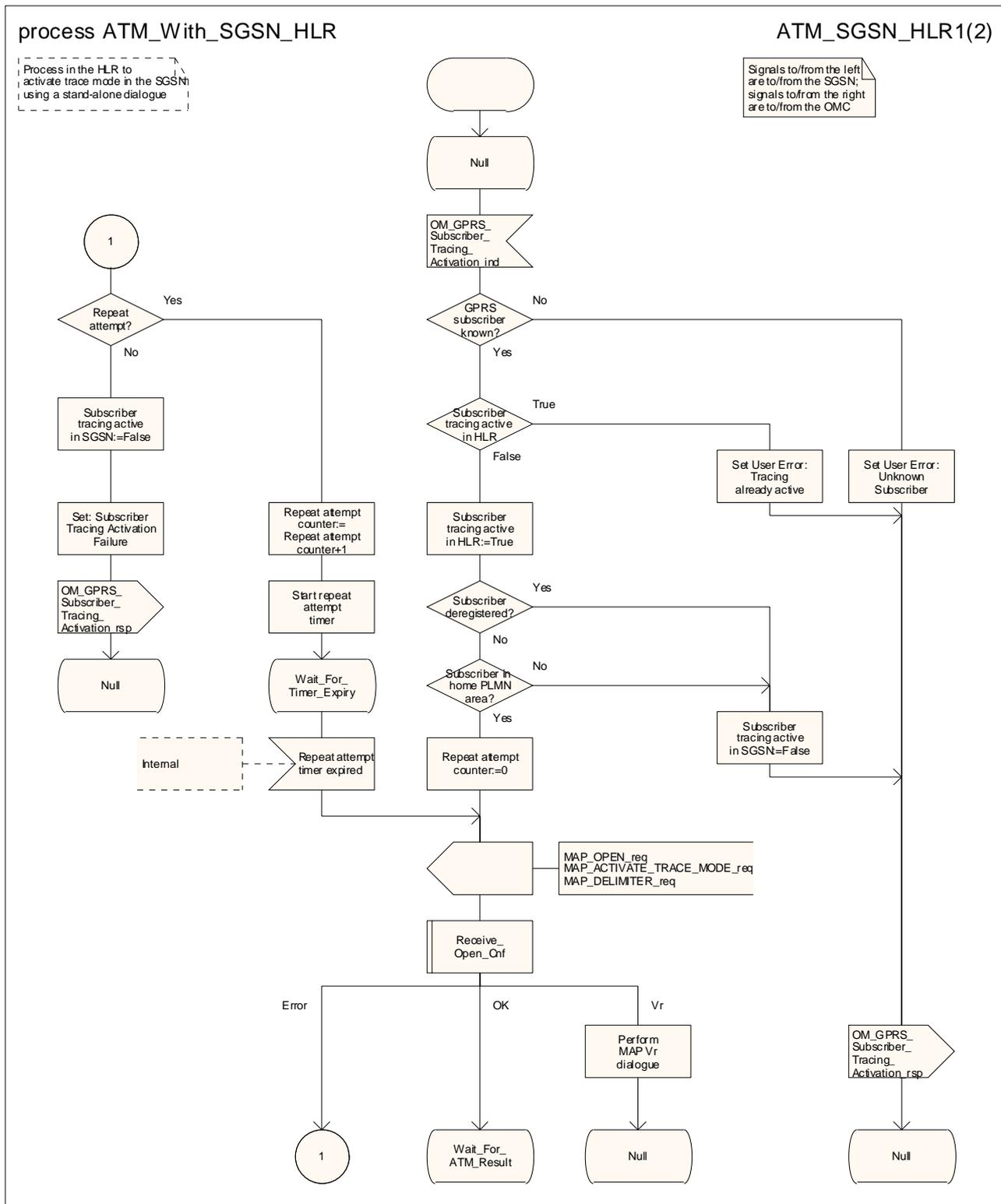
Figure 20.2/9 (sheet 1 of 2): Process ATM\_With\_SGSN\_HLR
