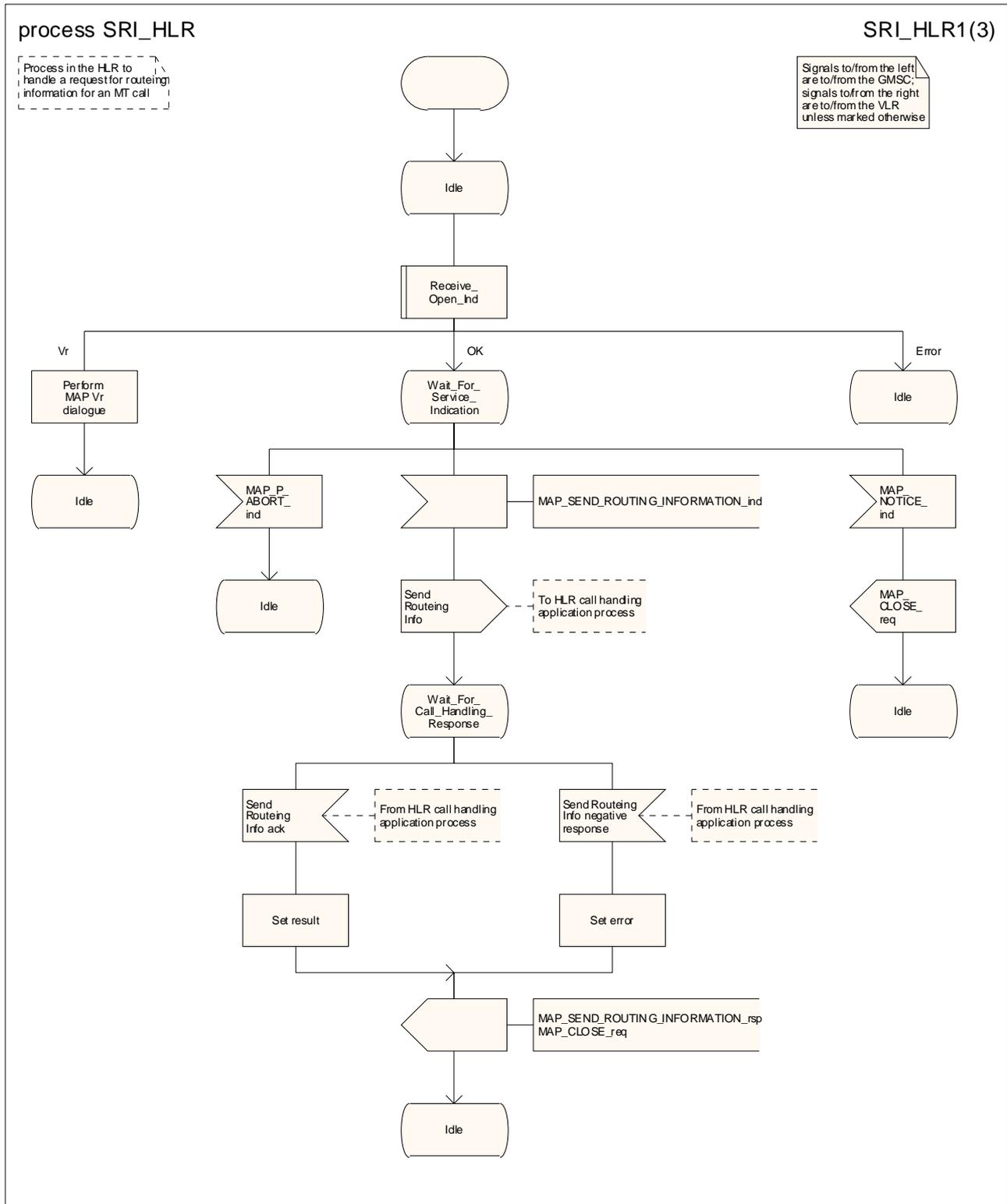
Figure 21.2/7 (sheet 1 of 3): Process SRI\_HLR
