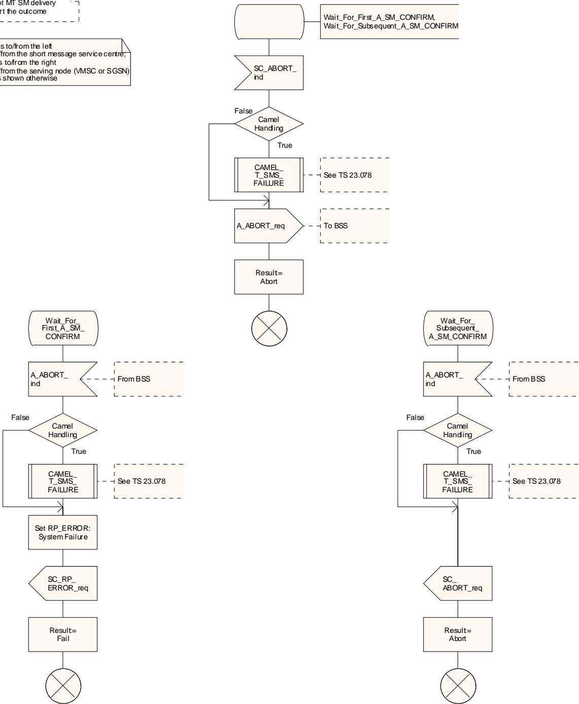
Figure 23.3/4 (sheet 6 of 8): Procedure MT\_SM\_Delivery\_Attempt\_GMSC
