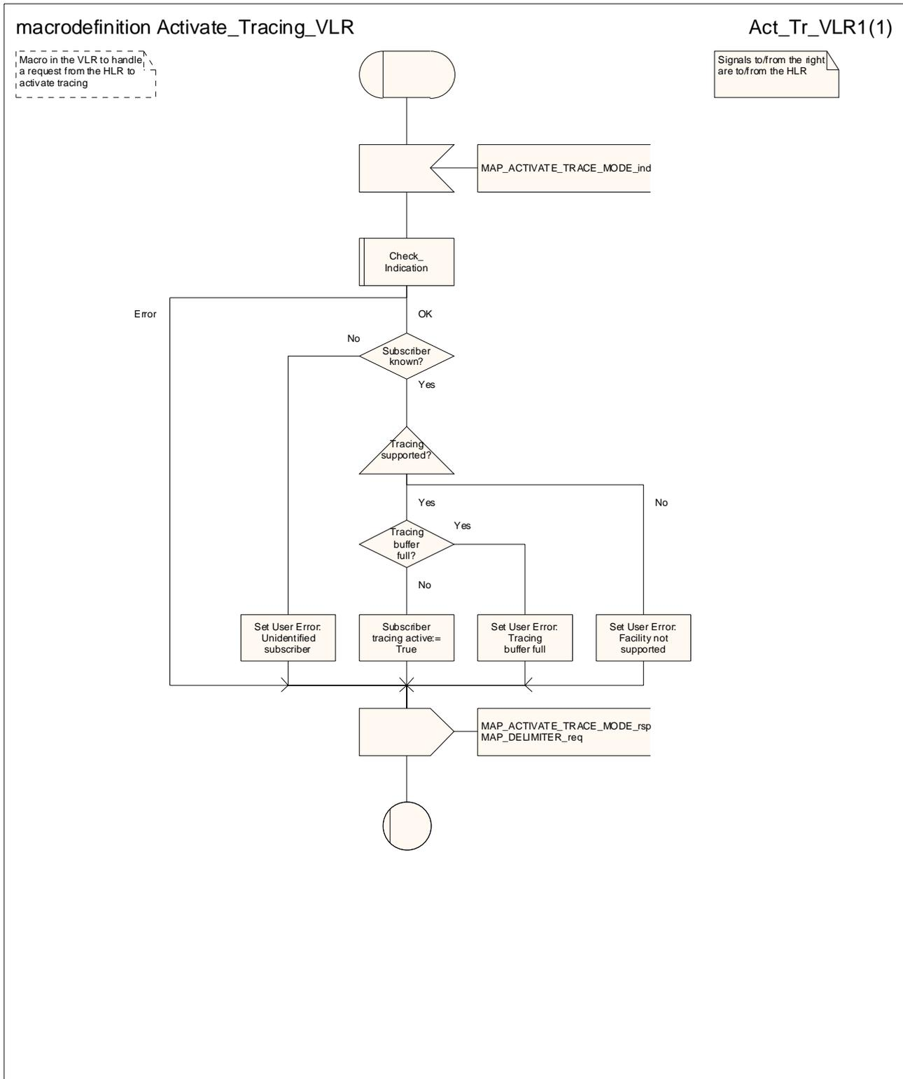
Figure 25.9/4: Macro Activate\_Tracing\_VLR
