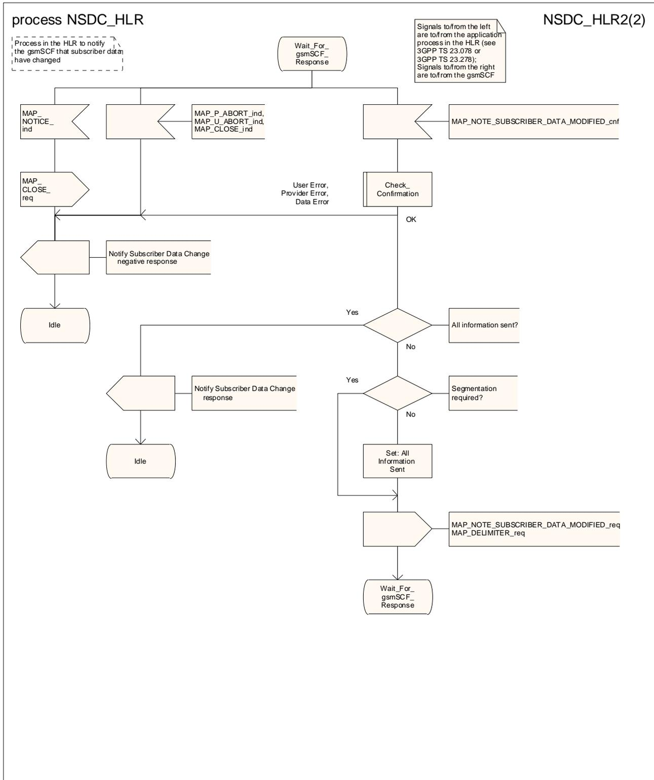
Figure 24A.4/2 (sheet 2 of 2): Process NSDC\_HLR
