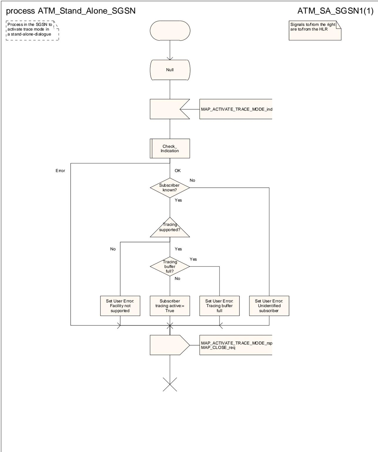
Figure 20.2/11: Process ATM\_Stand\_Alone\_SGSN
