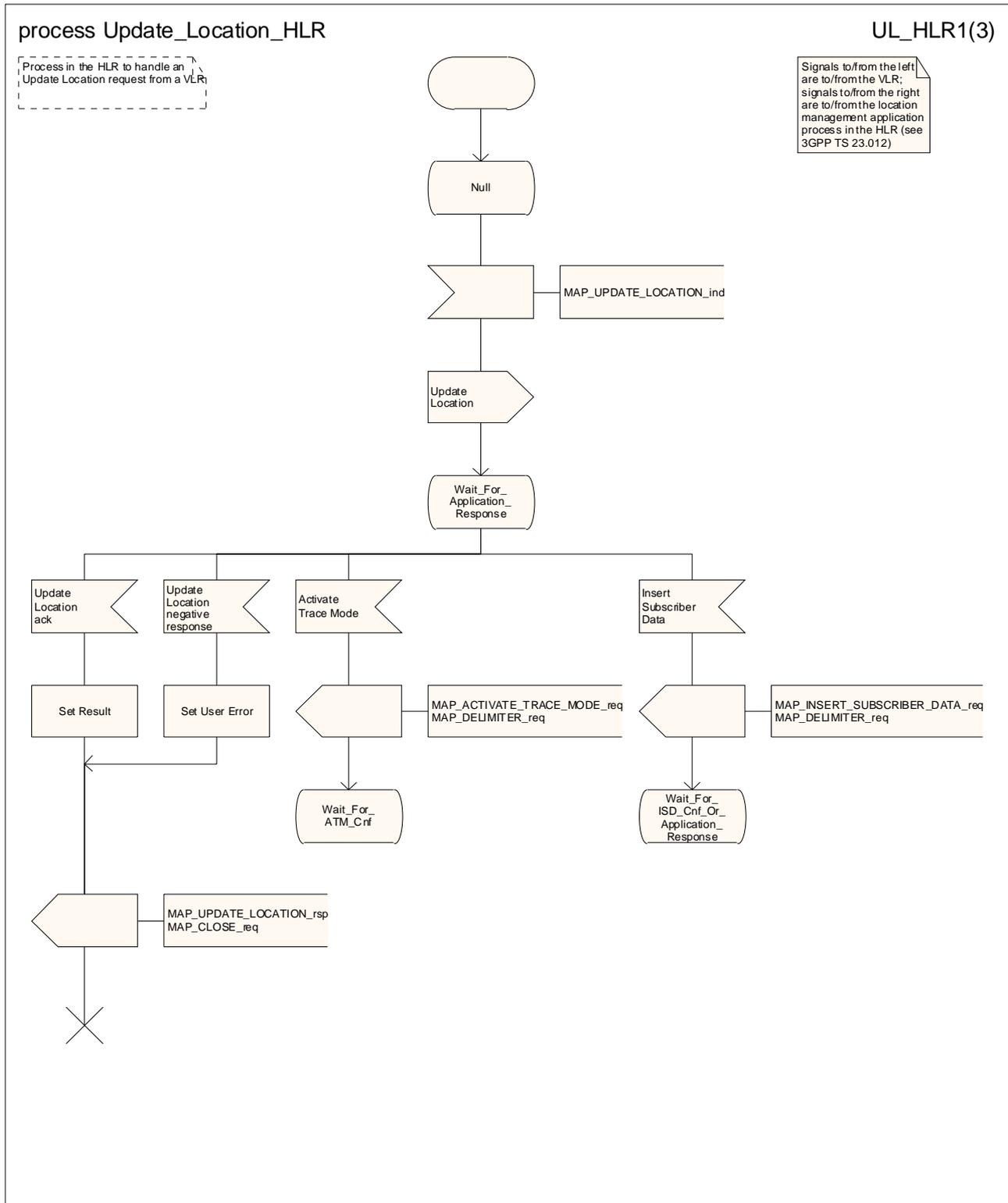
Figure 19.1.1/13 (sheet 1 of 3): Process Update\_Location\_HLR
