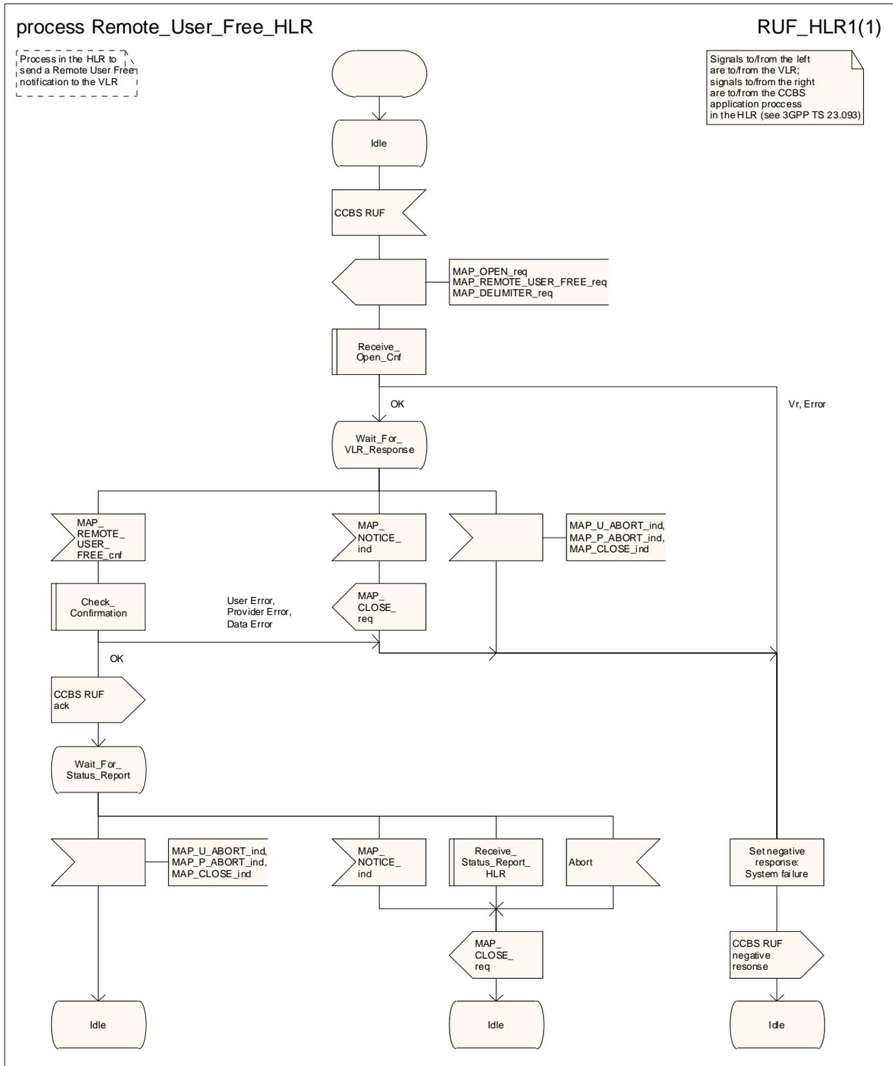
Figure 21.6/14: Process Remote\_User\_Free\_HLR
