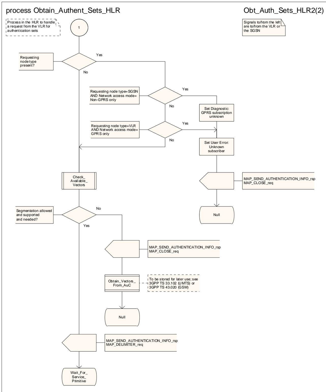
Figure 25.5/5 (sheet 2 of 2): Process Obtain\_Authent\_Sets\_HLR
