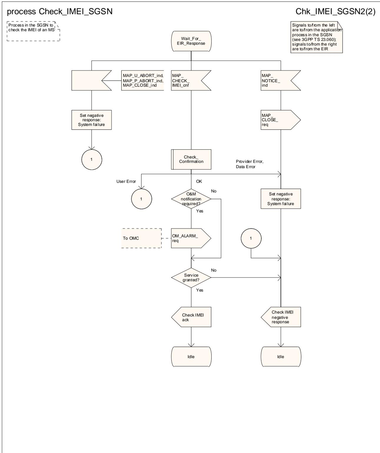
Figure 25.6/3 (sheet 2 of 2): Process Check\_IMEI\_SGSN
