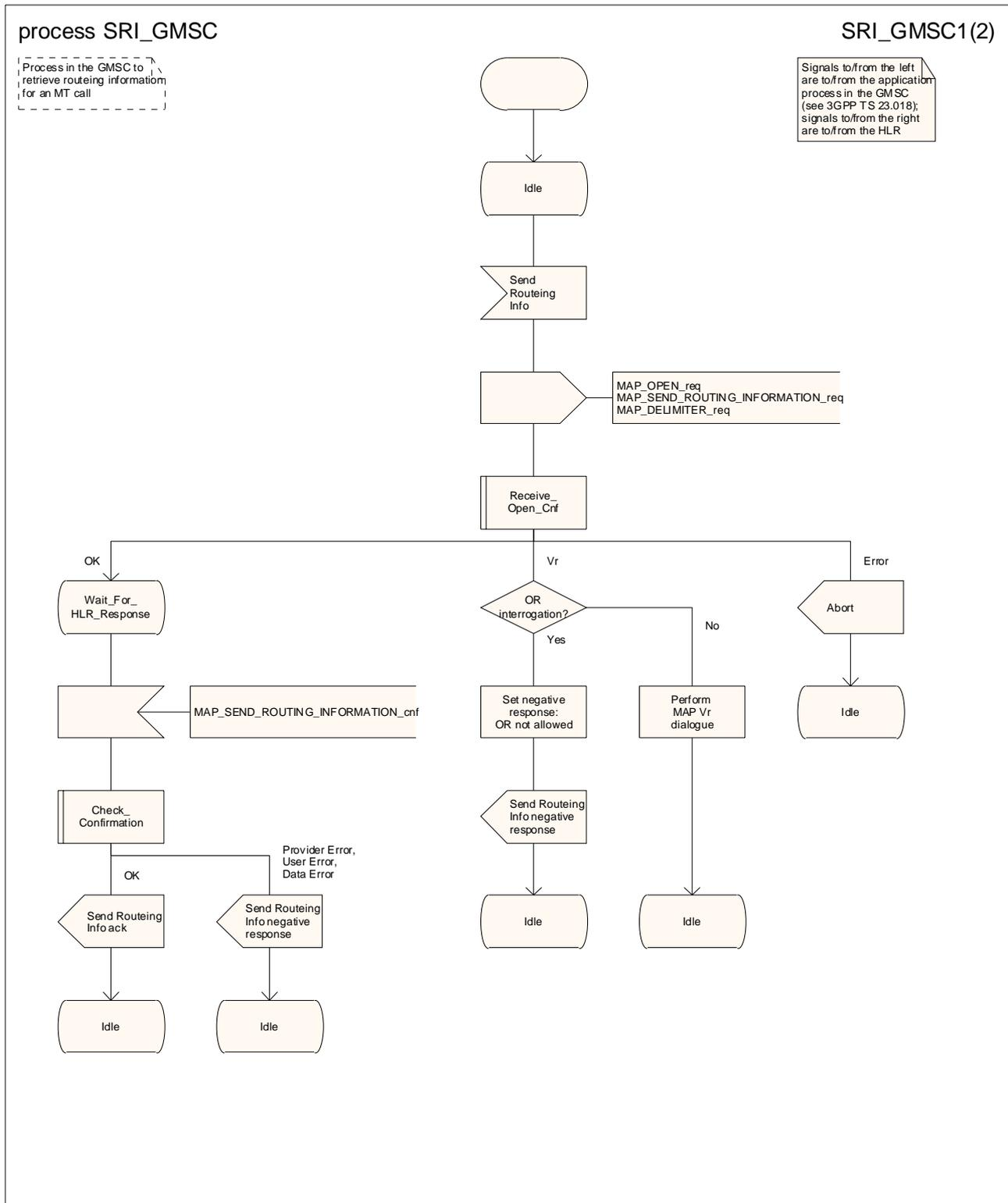
Figure 21.2/6 (sheet 1 of 2): Process SRI\_GMSC
