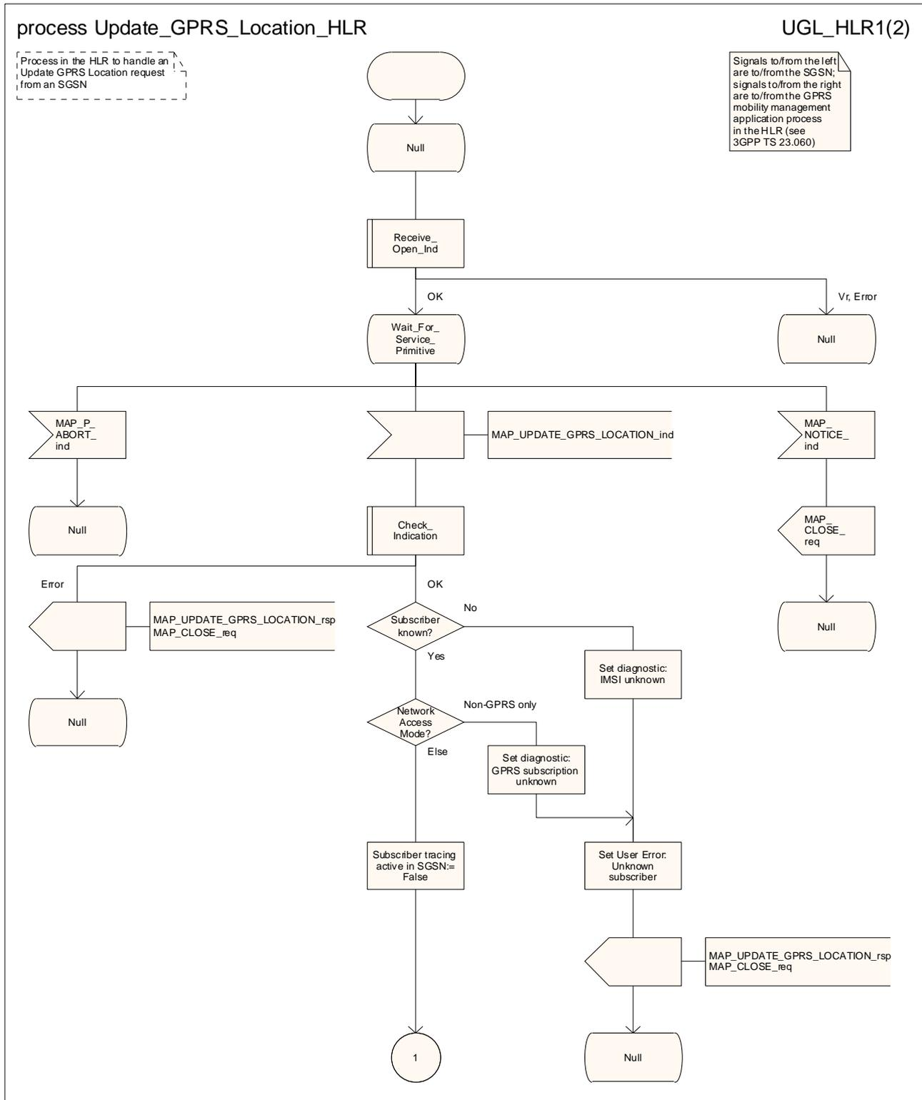
Figure 19.1.1/14 (sheet 1 of 2): Process Update\_GPRS\_Location\_HLR
