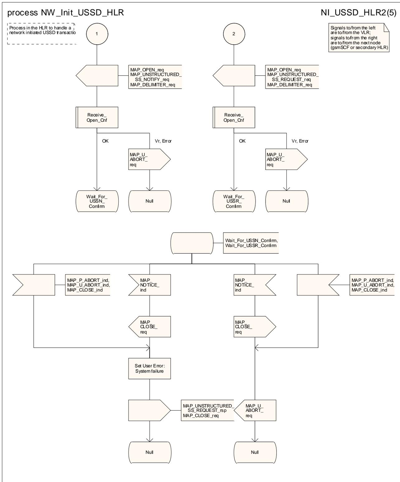
Figure 22.10.4/1 (sheet 2 of 5): Process NW\_Init\_USSD\_HLR
