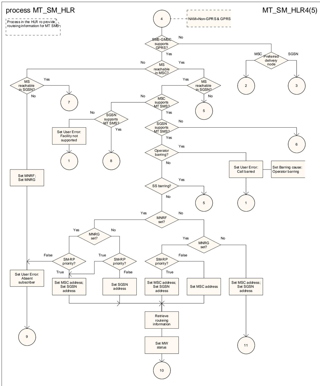
Figure 23.3/5 (sheet 4 of 5): Process MT\_SM\_HLR
