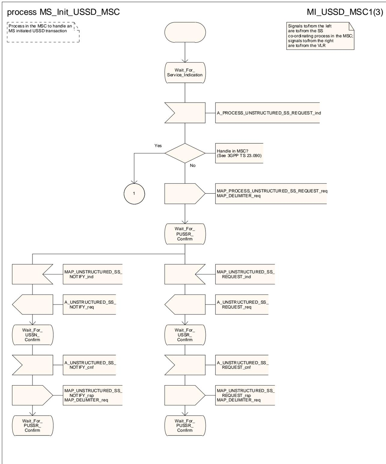
Figure 22.9.2/1 (sheet 1 of 3): Process MS\_Init\_USSD\_MSC
