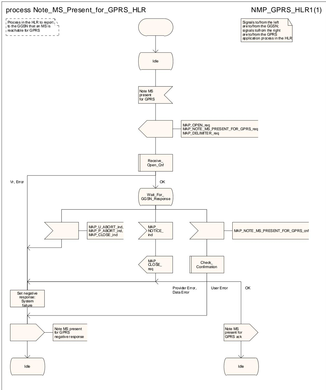
Figure 24.3/1: Process Note\_MS\_Present\_For\_GPRS\_HLR
