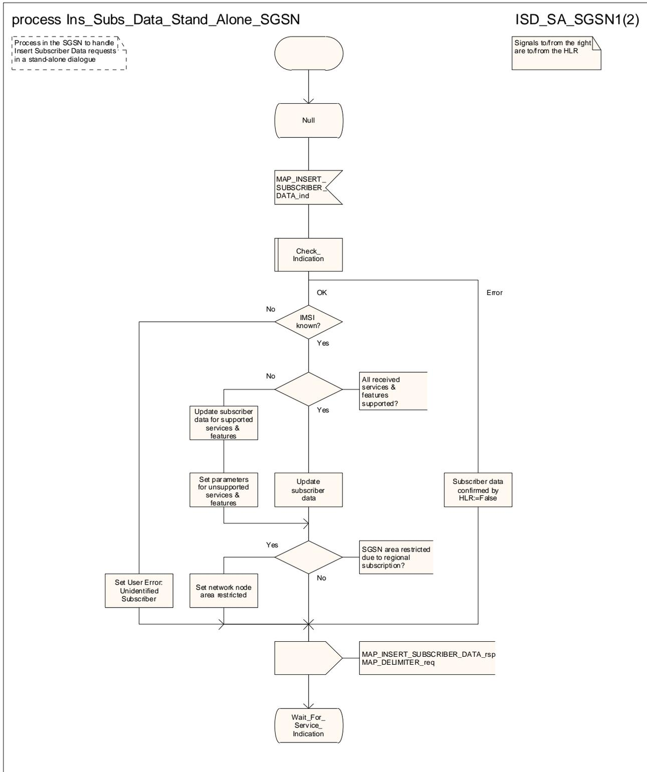
Figure 20.3/11 (sheet 1 of 2): Process Ins\_Subscriber\_Data\_Stand\_Alone\_SGSN
