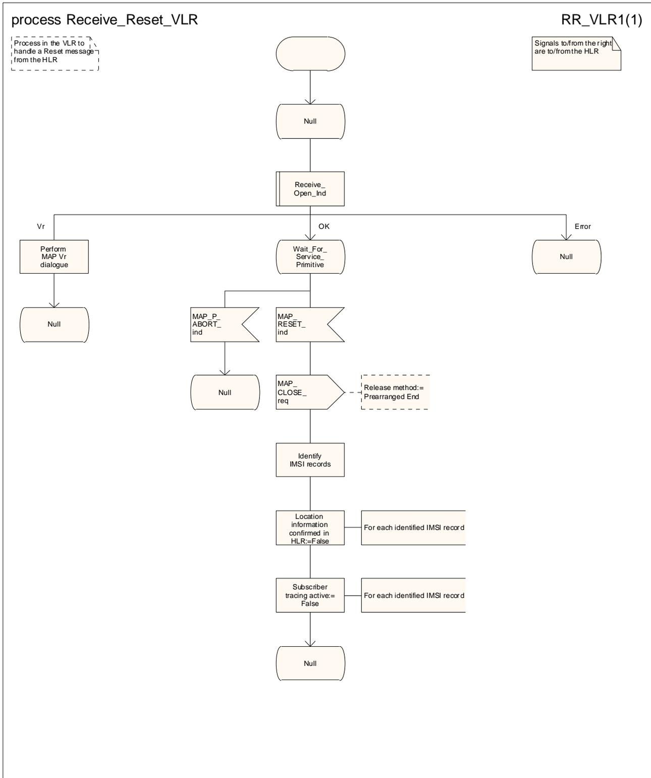
Figure 19.3.2/6: Process Receive\_Reset\_VLR
