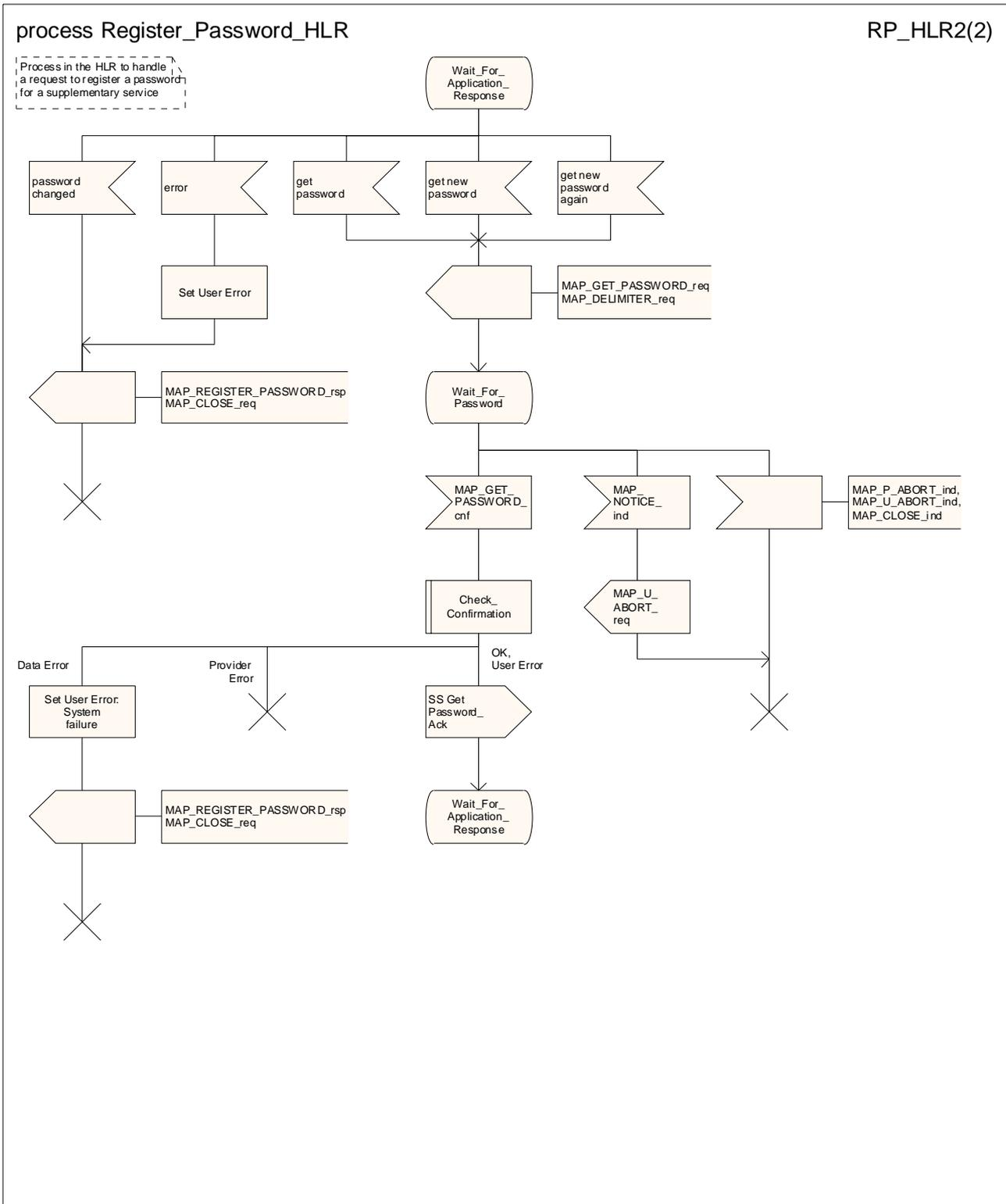
Figure 22.8.4/1 (sheet 2 of 2): Process Register\_PW\_HLR
