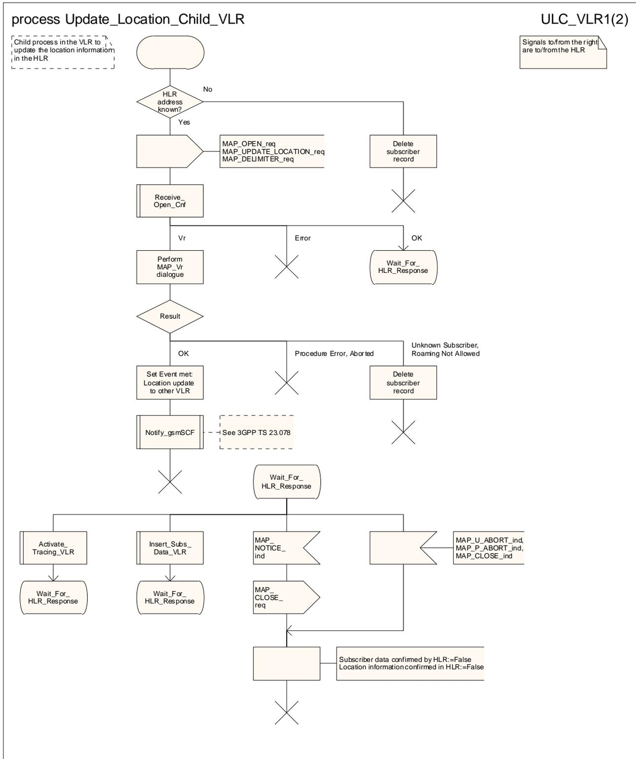
Figure 25.4/4 (sheet 1 of 2): Process Update\_Location\_Child\_VLR
