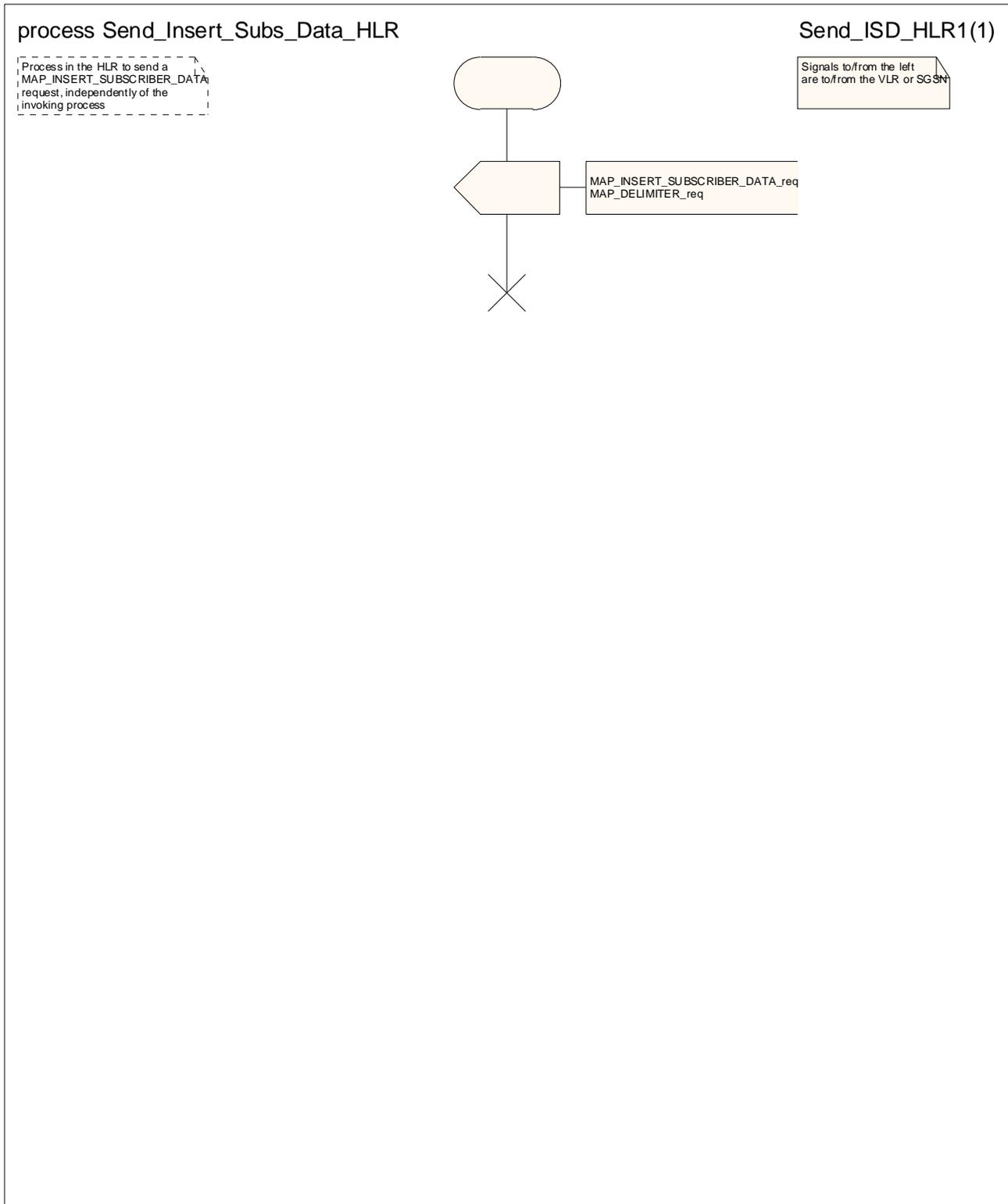
Figure 25.7/7: Process Send\_Insert\_Subscriber\_Data\_HLR
