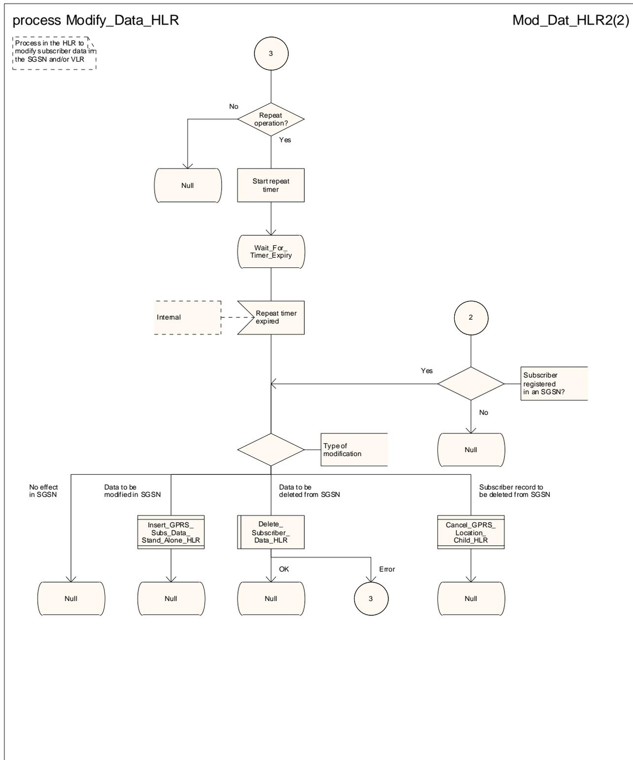
Figure 20.3/6 (sheet 2 of 2): Process Modify\_Data\_HLR
