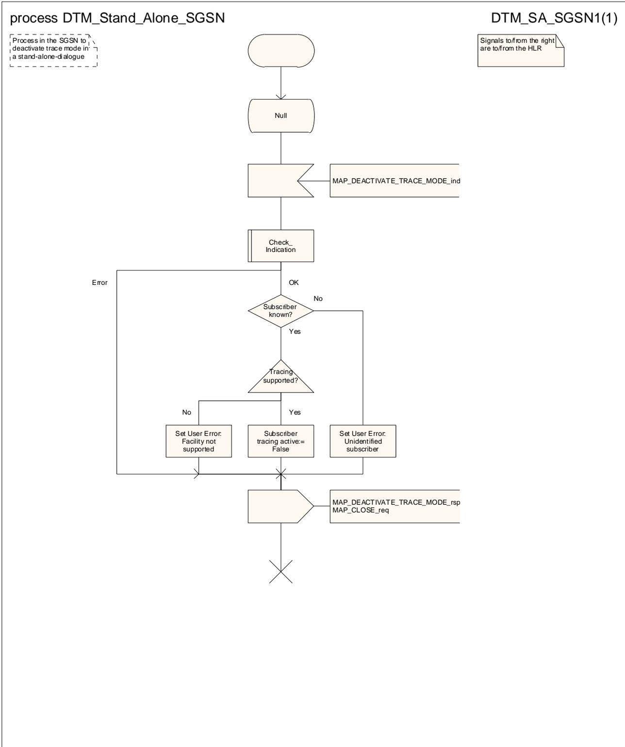
Figure 20.2/15: Process DTM\_Stand\_Alone\_SGSN
