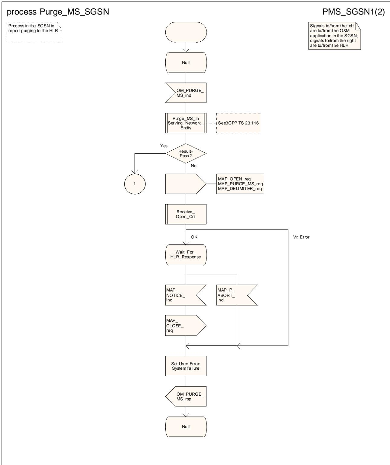
Figure 19.1.4/4 (sheet 1 of 2): Process Purge\_MS\_SGSN
