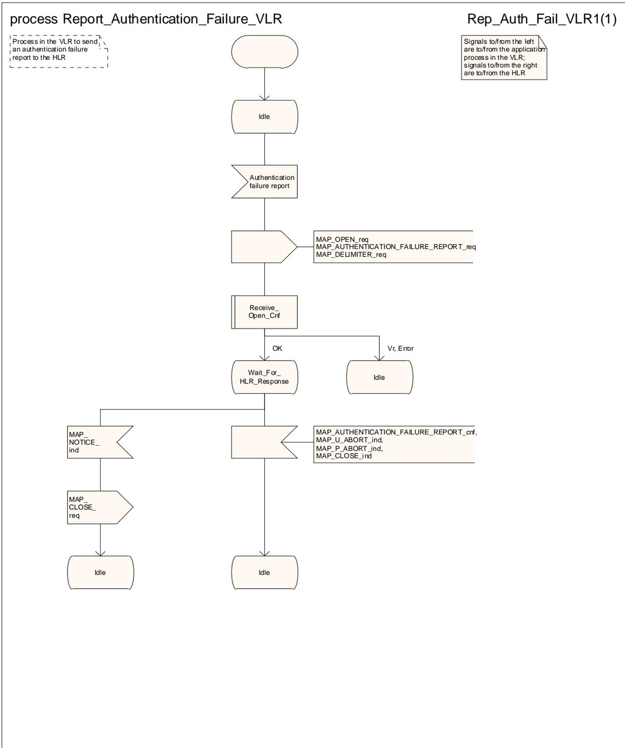
Figure 25.5/9: Process Report\_Authentication\_Failure\_VLR
