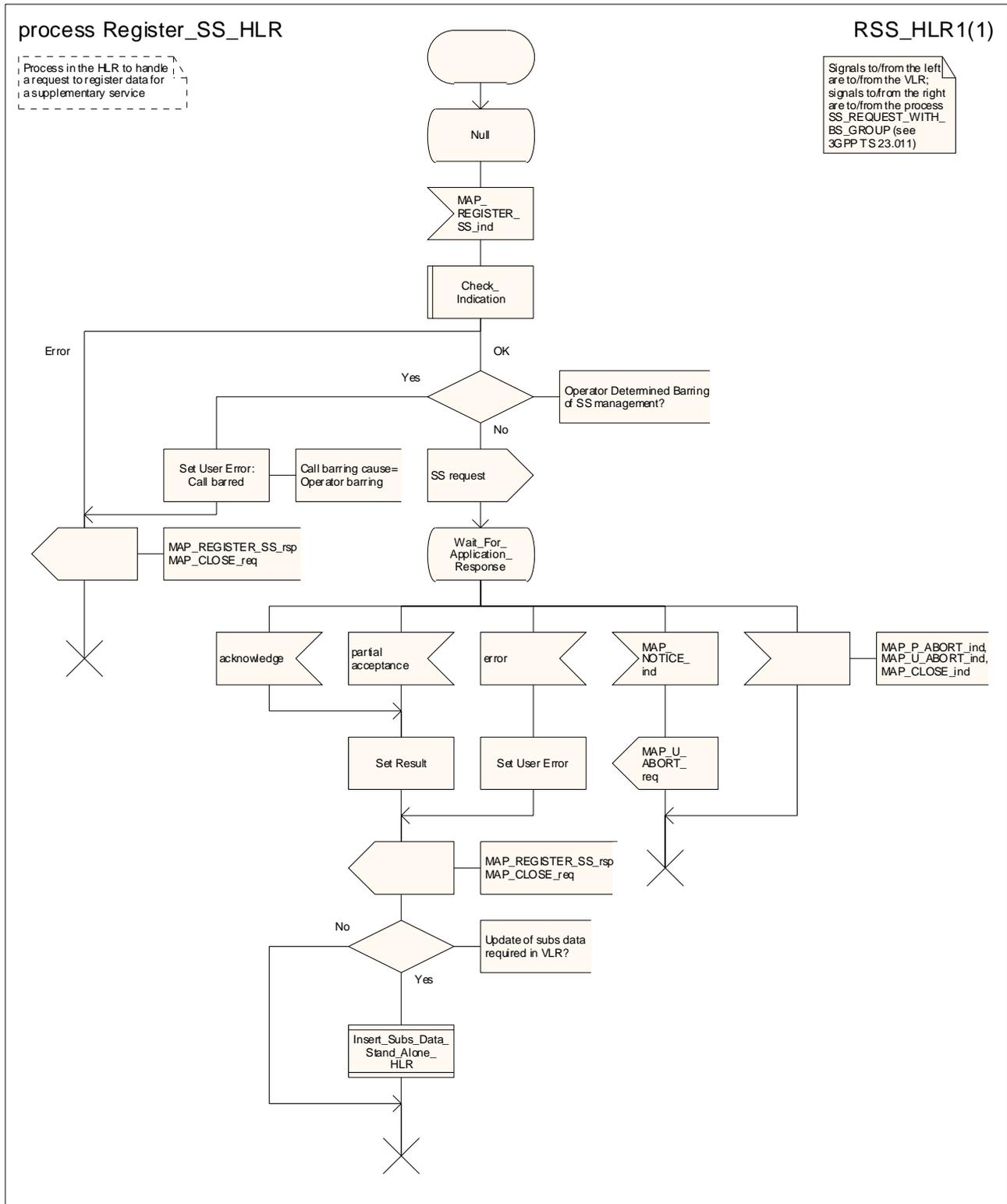
Figure 22.2.4/1: Process Register\_SS\_HLR
