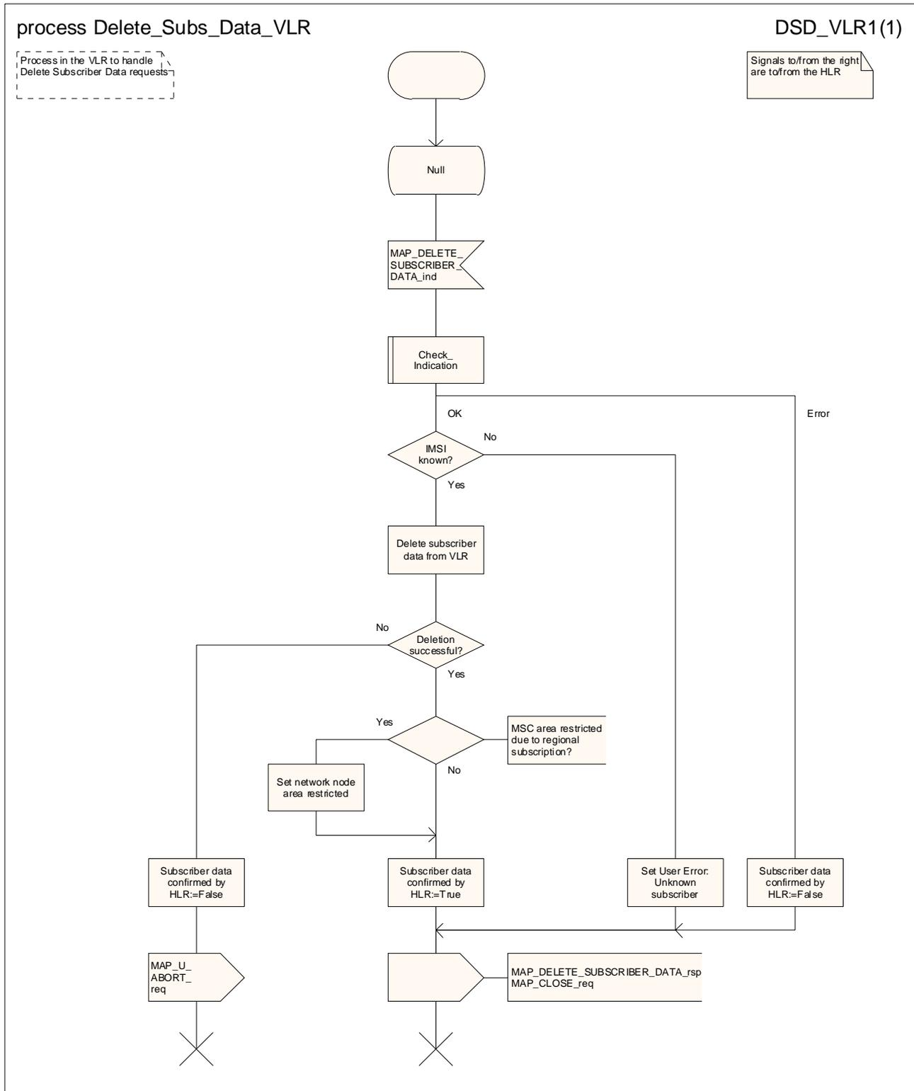
Figure 20.3/10: Process Delete\_Subs\_Data\_VLR
