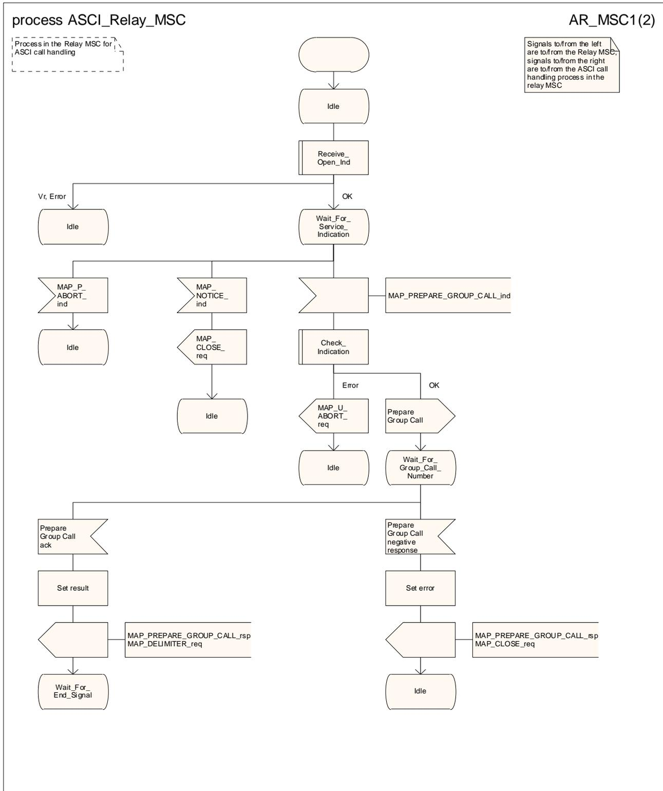
Figure 21.4/3 (sheet 1 of 2): Process ASCII\_Relay\_MSC
