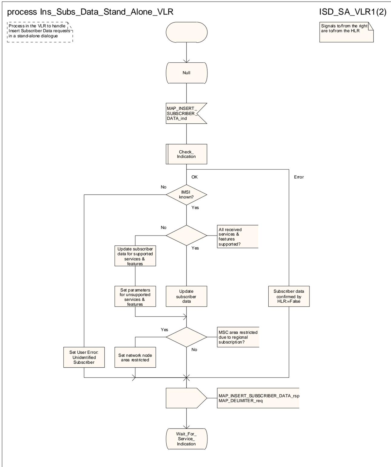
Figure 20.3/9 (sheet 1 of 2): Process Ins\_Subscriber\_Data\_Stand\_Alone\_VLR
