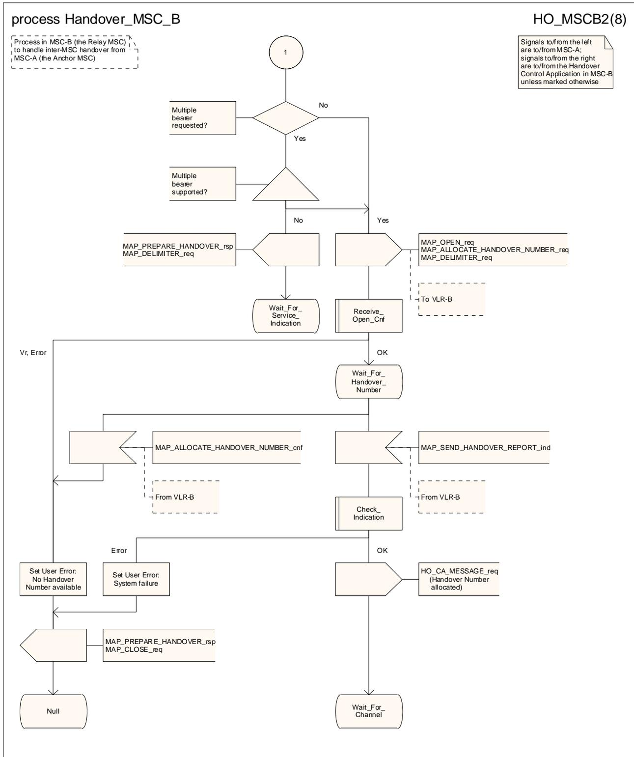
Figure 19.2/5 (sheet 2 of 8): Process HO\_MSC\_B
