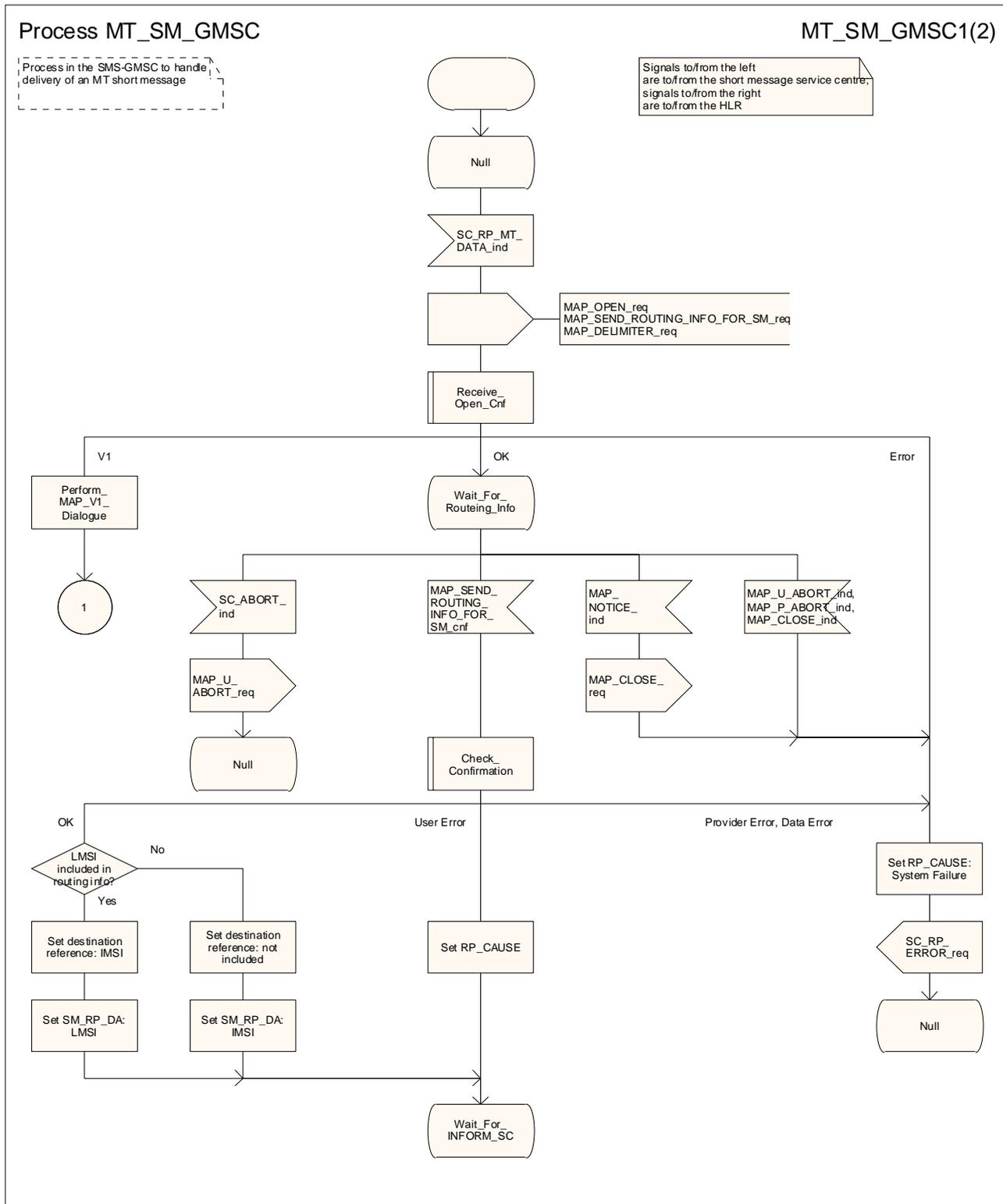
Figure 23.3/3 (sheet 1 of 2): Process MT\_SM\_GMSC
