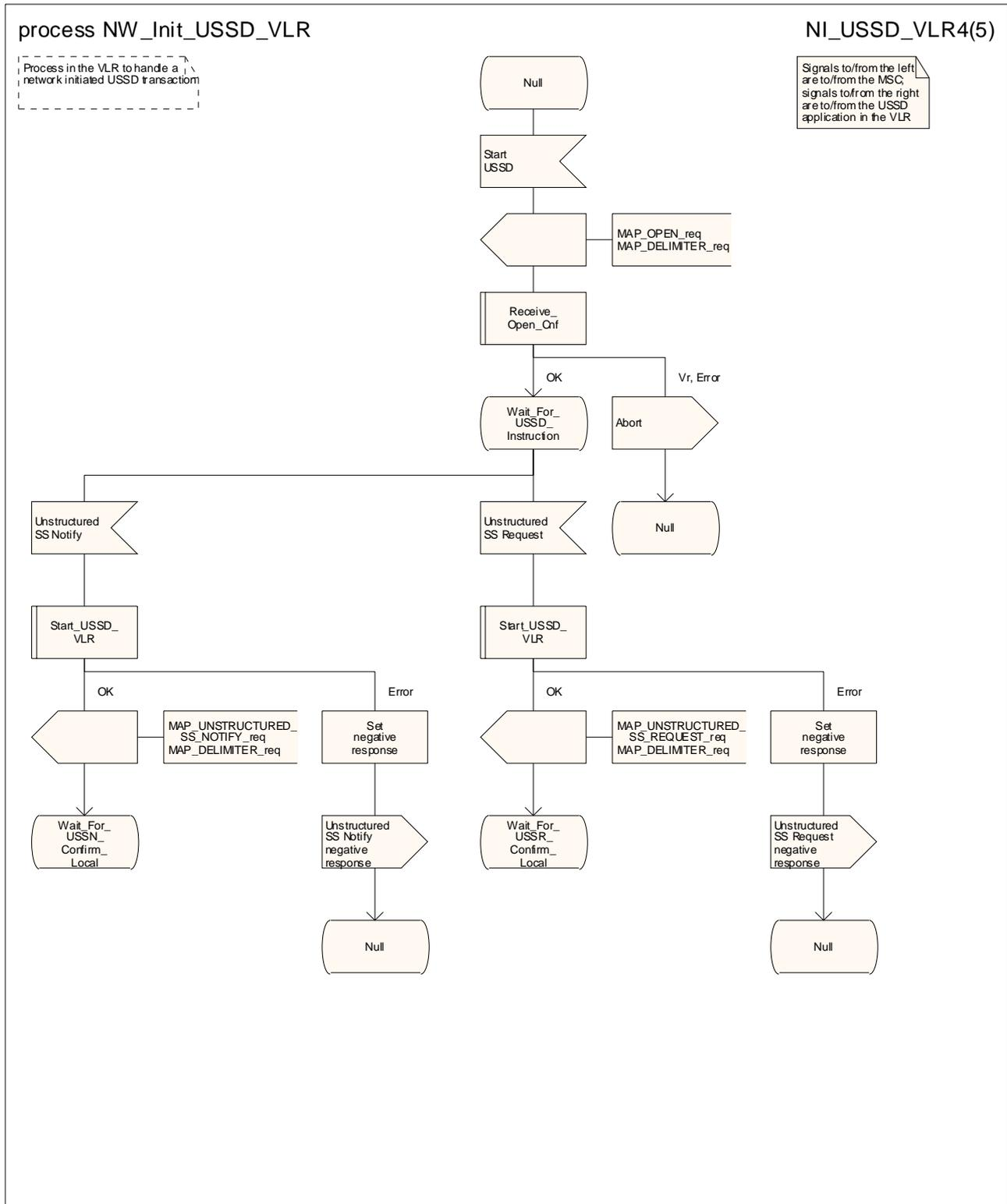
Figure 22.10.3/1 (sheet 4 of 5): Process NW\_Init\_USSD\_VLR
