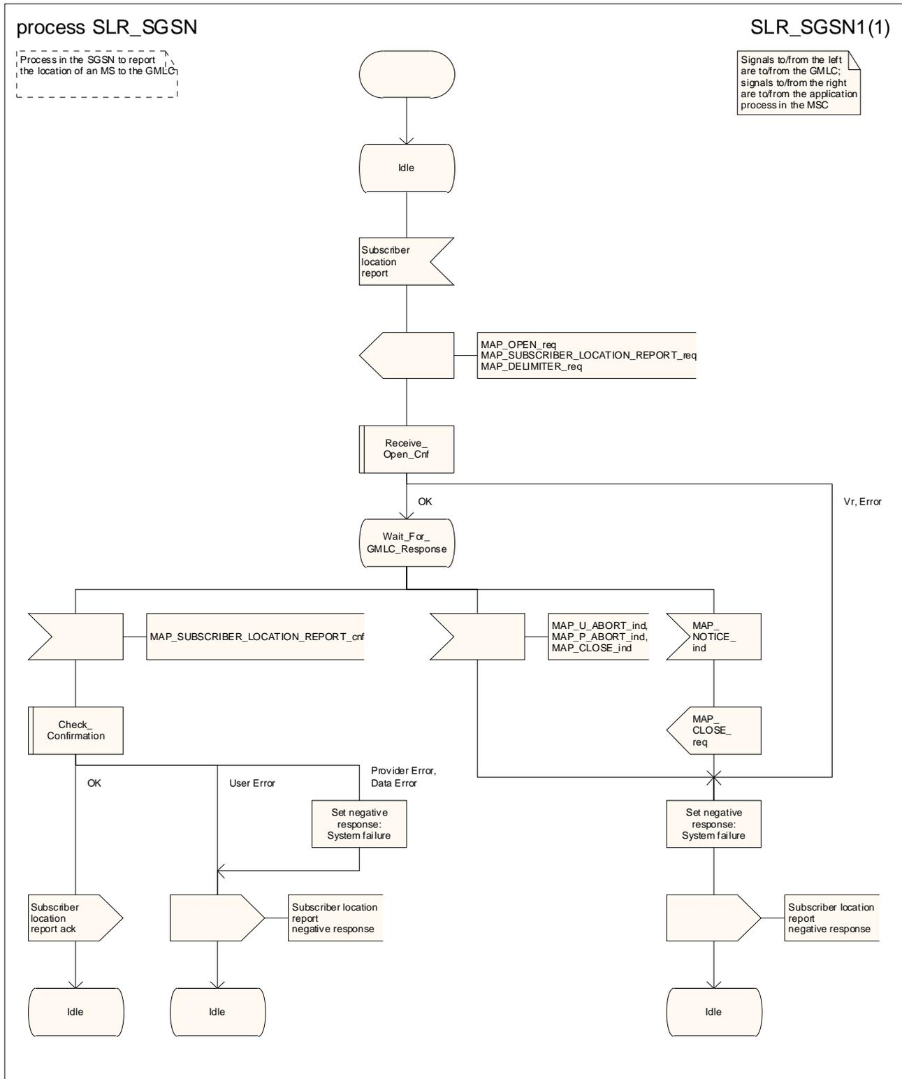
Figure 24B.3/3: Process SLR\_SGSN
