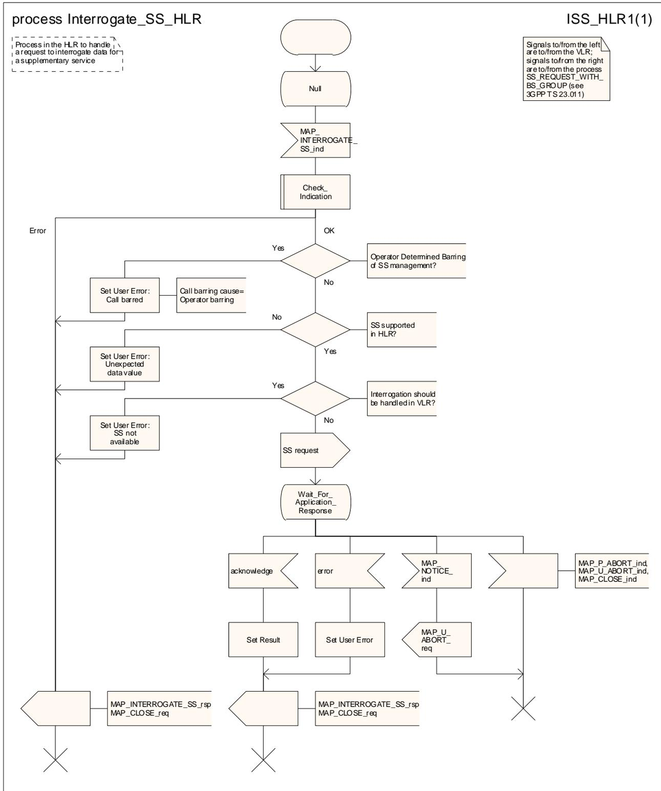
Figure 22.6.4/1: Process Interrogate\_SS\_HLR
