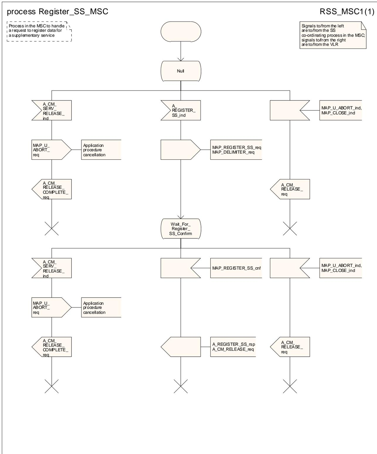
Figure 22.2.2/1: Process Register\_SS\_MSC
