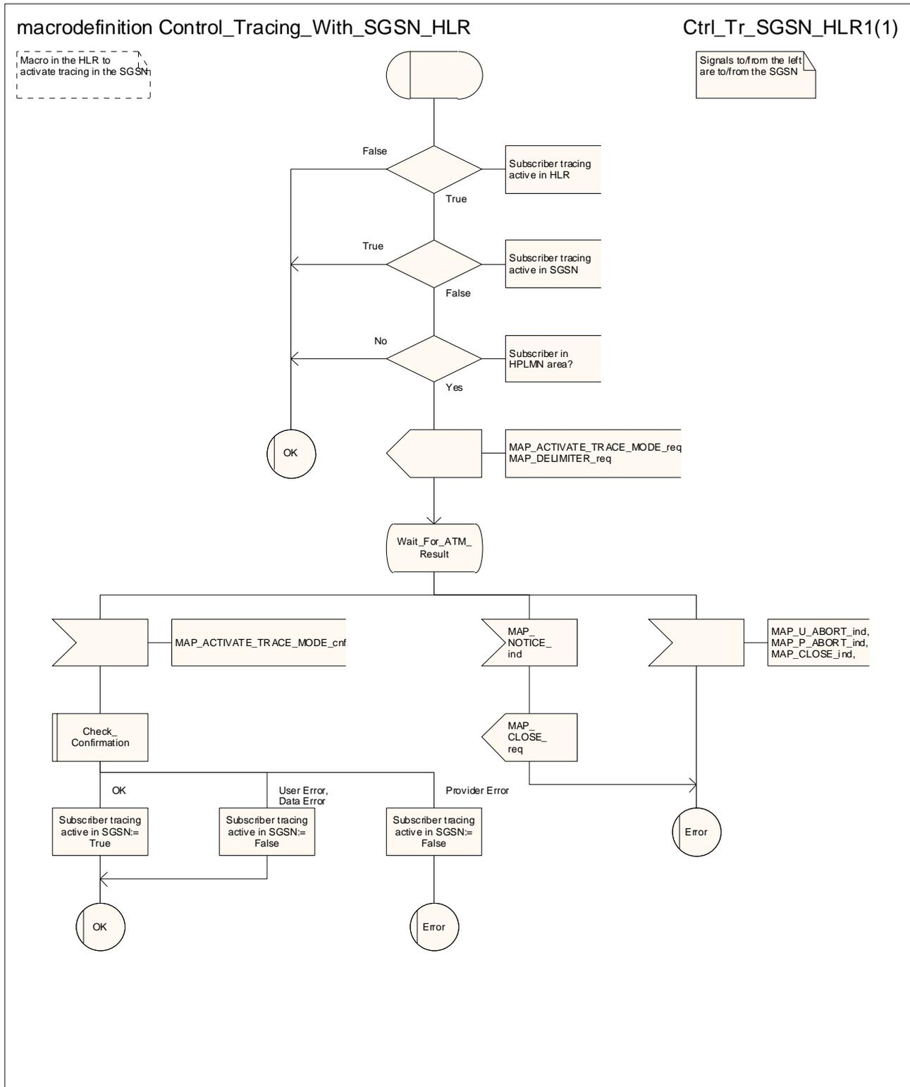
Figure 25.9/7: Macro Control\_Tracing\_With\_SGSN\_HLR
