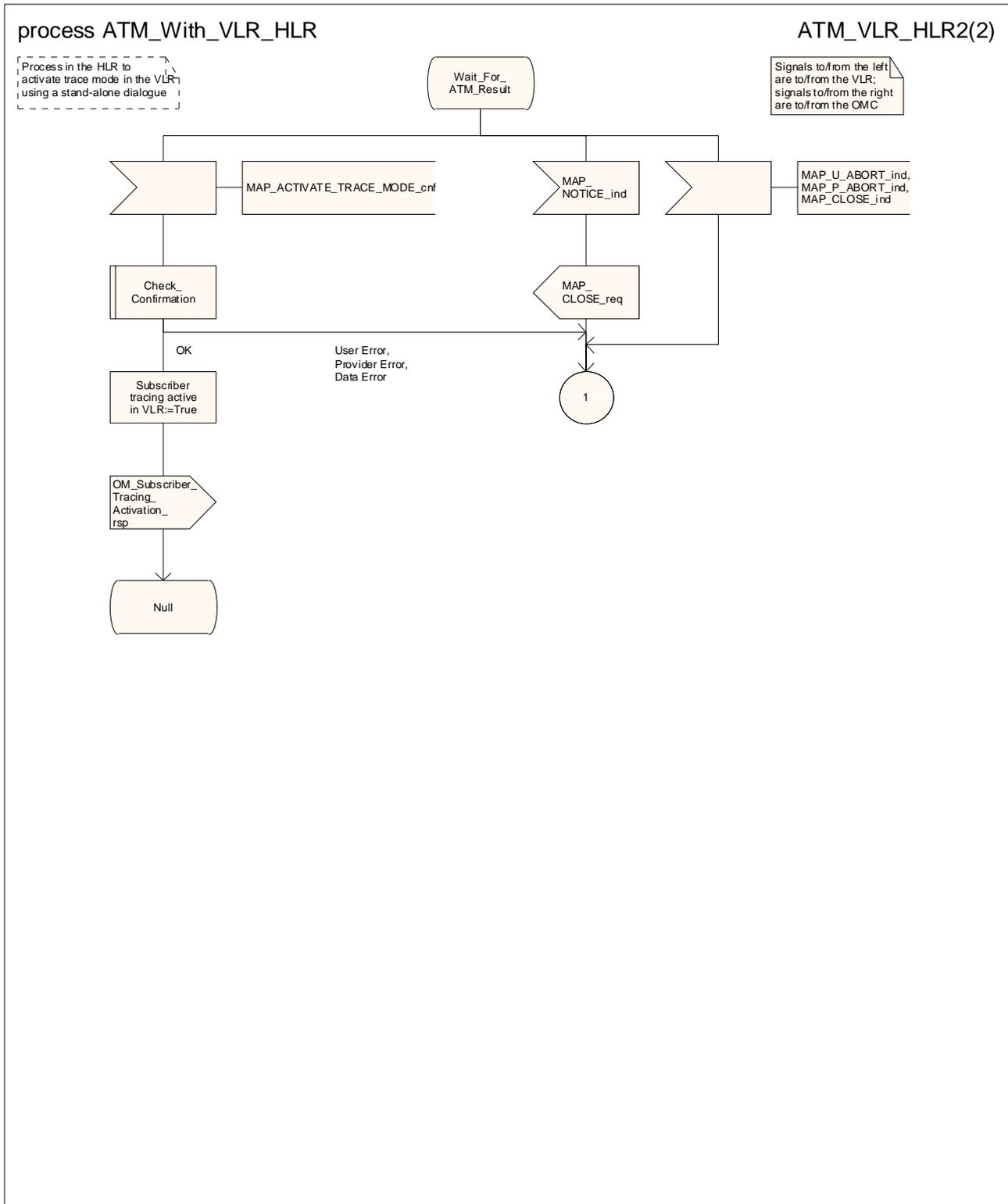
Figure 20.2/8 (sheet 2 of 2): Process ATM\_With\_VLR\_HLR
