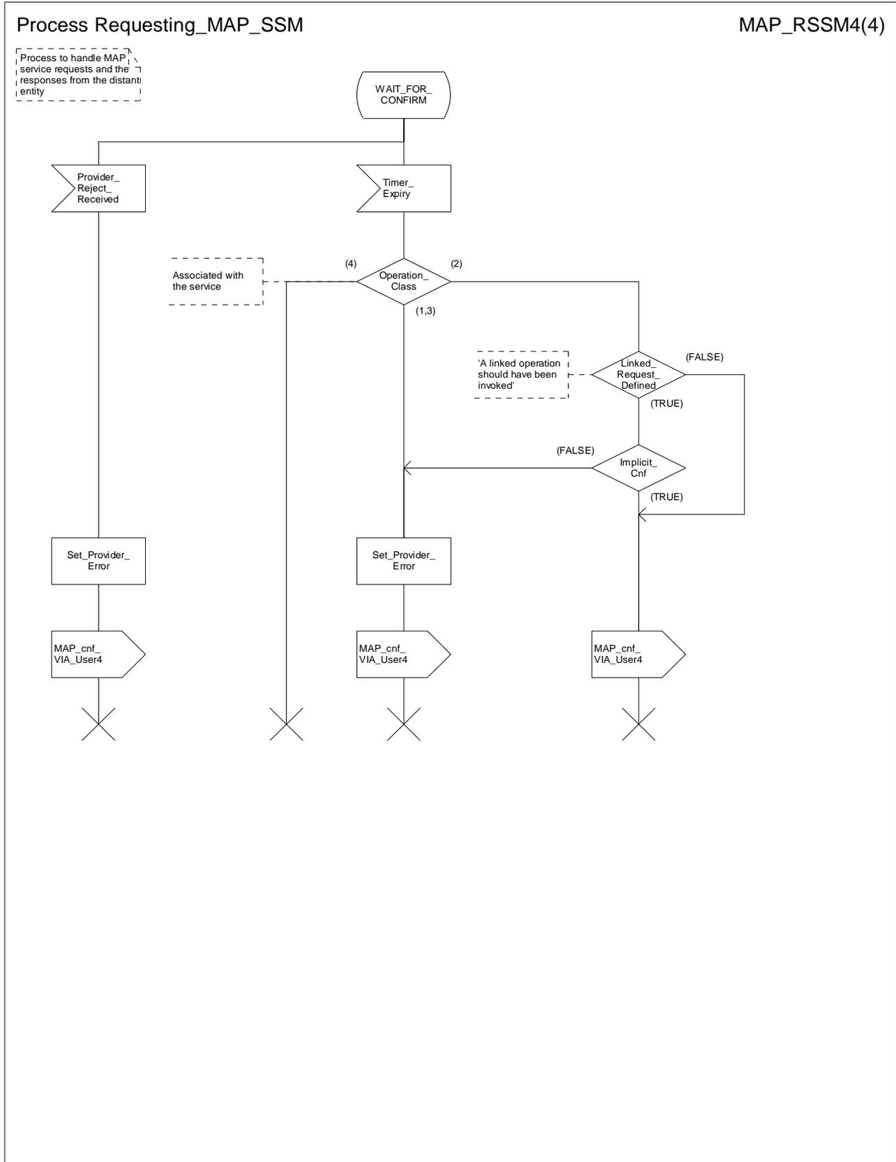
Figure 15.6/6d: Process Requesting\_MAP\_SSM (sheet 4)
