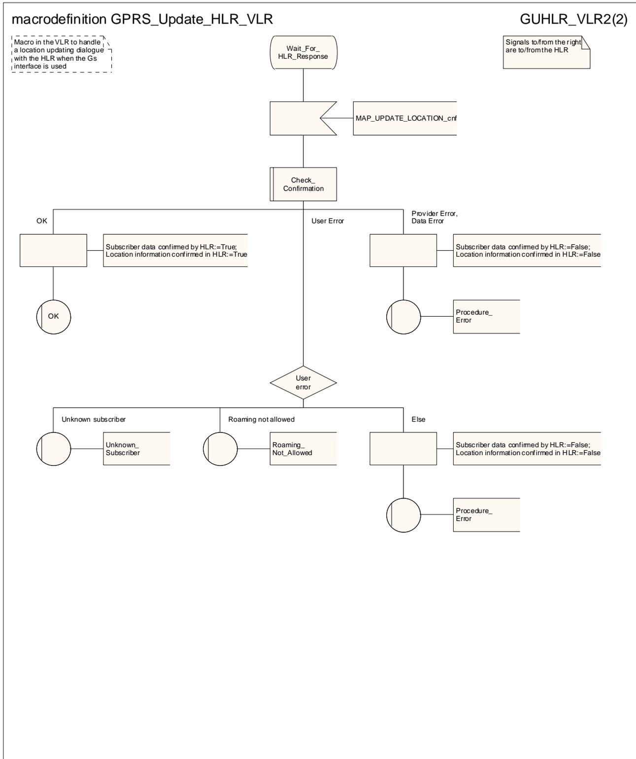
Figure 19.1.1/10 (sheet 2 of 2): Macro GPRS\_Update\_HLR\_VLR
