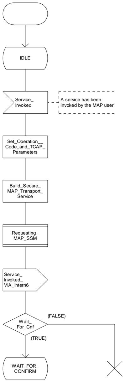
Figure 15.6/7a: Process Secure\_Requesting\_MAP\_SSM (sheet 1)
