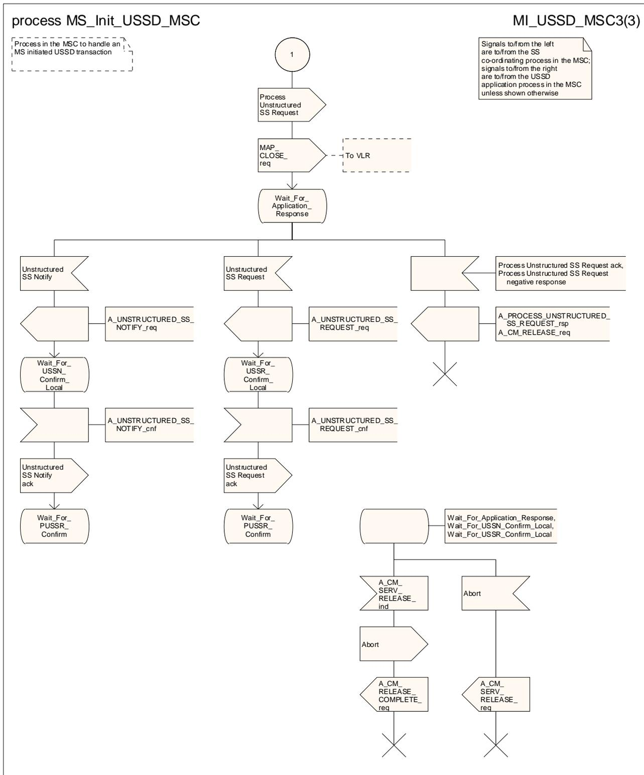
Figure 22.9.2/1 (sheet 3 of 3): Process MS\_Init\_USSD\_MSC
