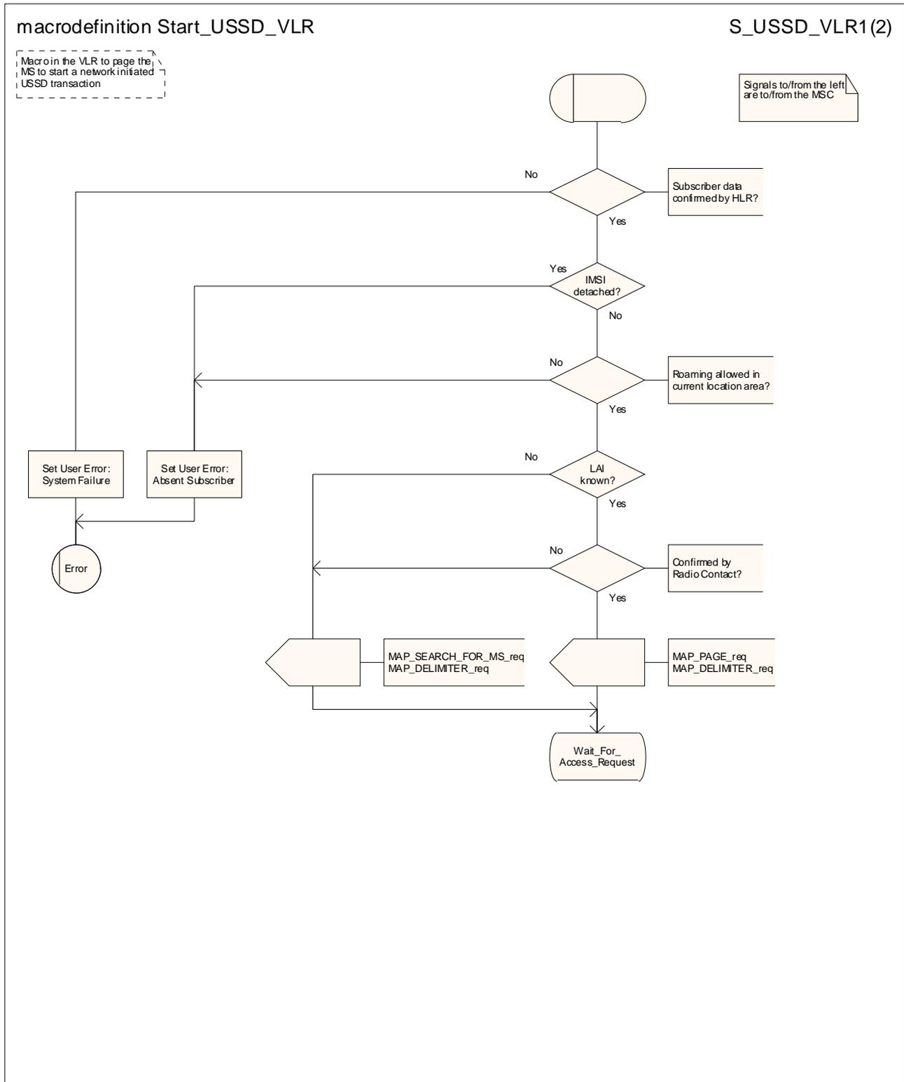
Figure 22.10.3/2 (sheet 1 of 2): Macro Start\_USSD\_VLR
