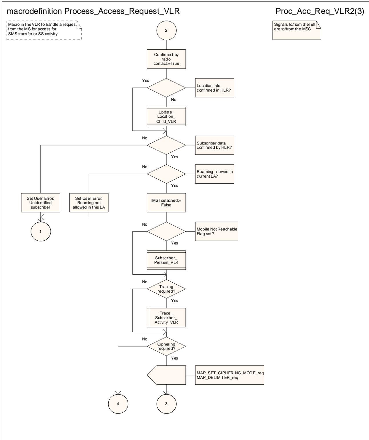
Figure 25.4/2 (sheet 2 of 3): Macro Process\_Access\_Request\_VLR
