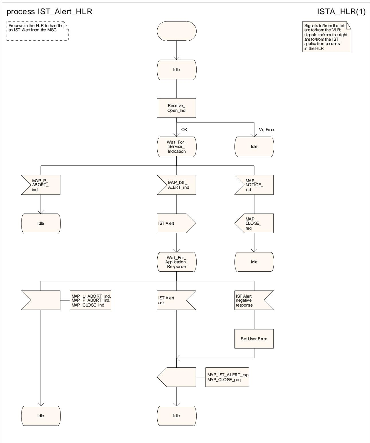
Figure 21.9/4: Process IST\_Alert\_HLR
