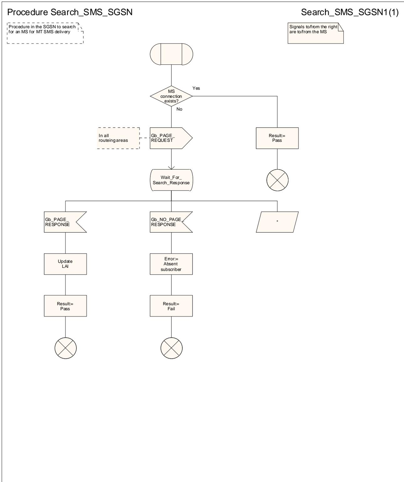
Figure 23.3/13 (sheet 1 of 1): Procedure Search\_SMS\_SGSN
