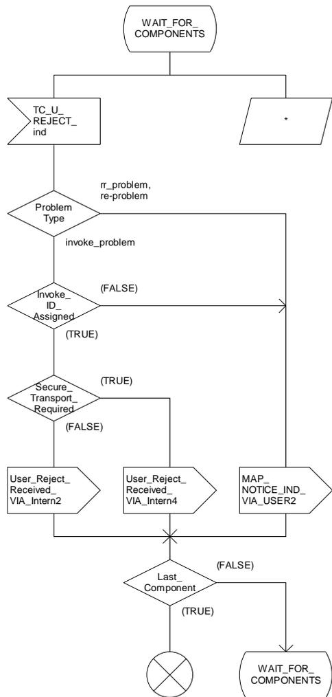
Figure 15.6/4e: Procedure Process\_Components (sheet 5)
