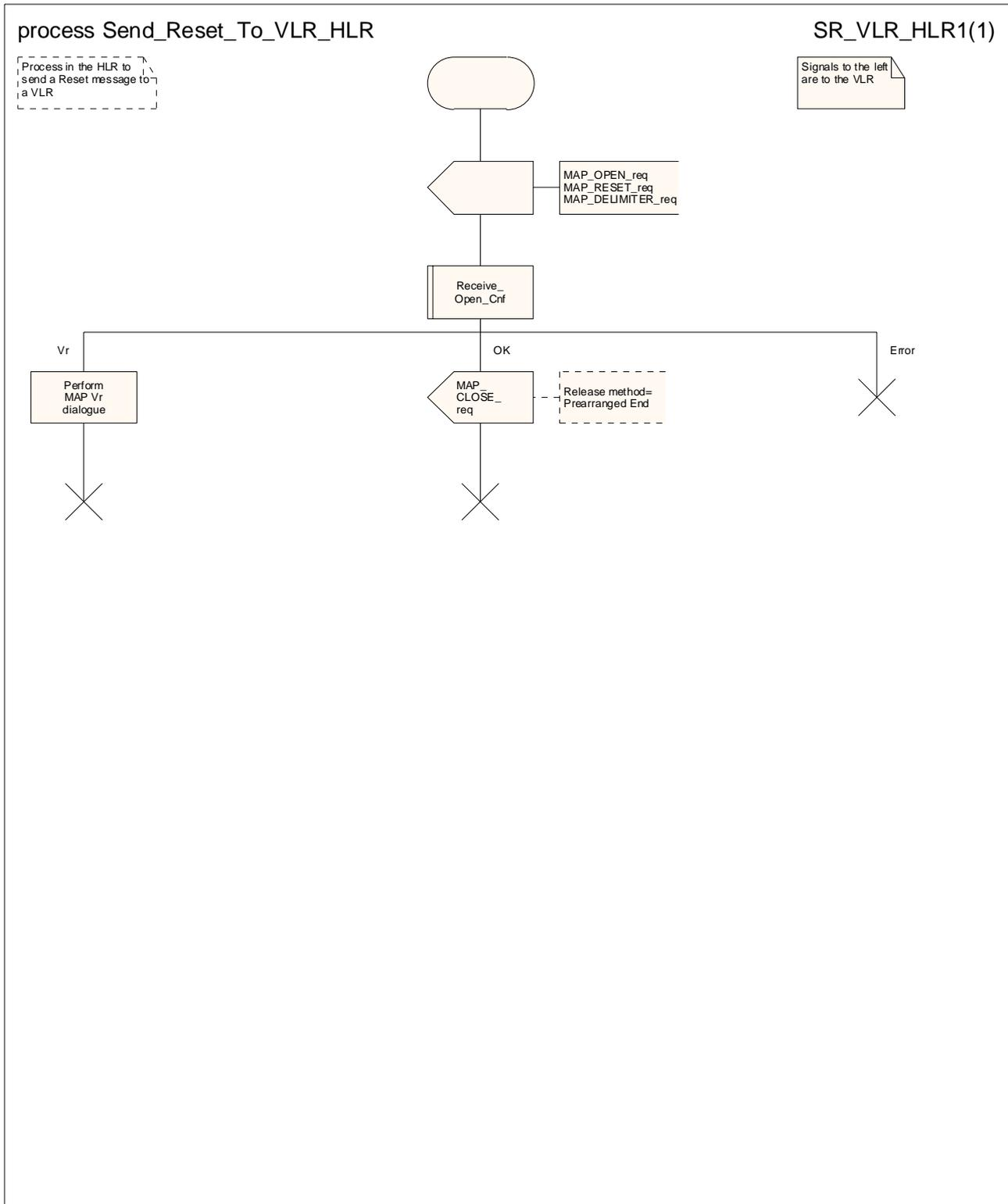
Figure 19.3.2/4: Process Send\_Reset\_To\_VLR\_HLR
