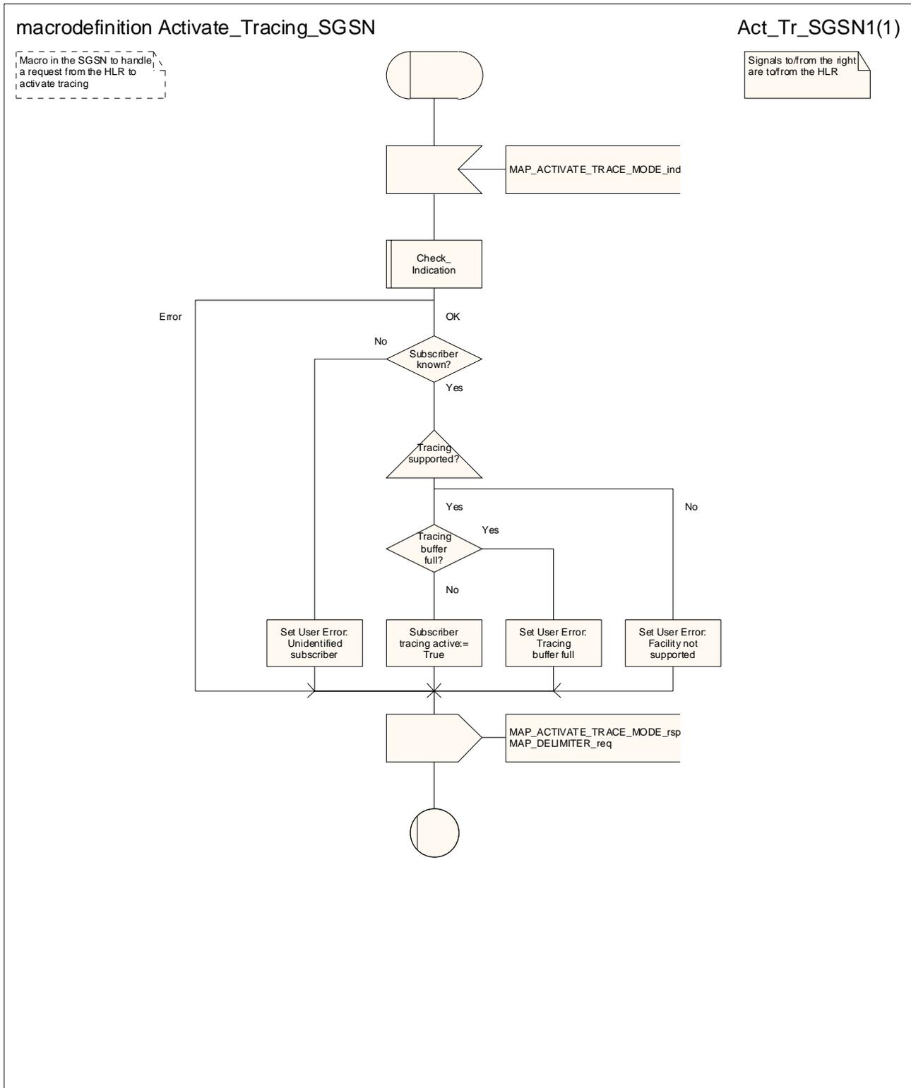
Figure 25.9/5: Macro Activate\_Tracing\_SGSN
