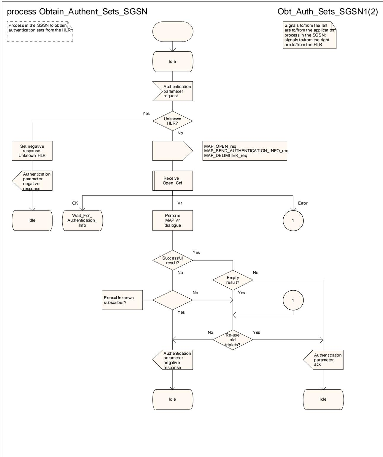
Figure 25.5/5 (sheet 1 of 2): Process Obtain\_Authent\_Sets\_SGSN
