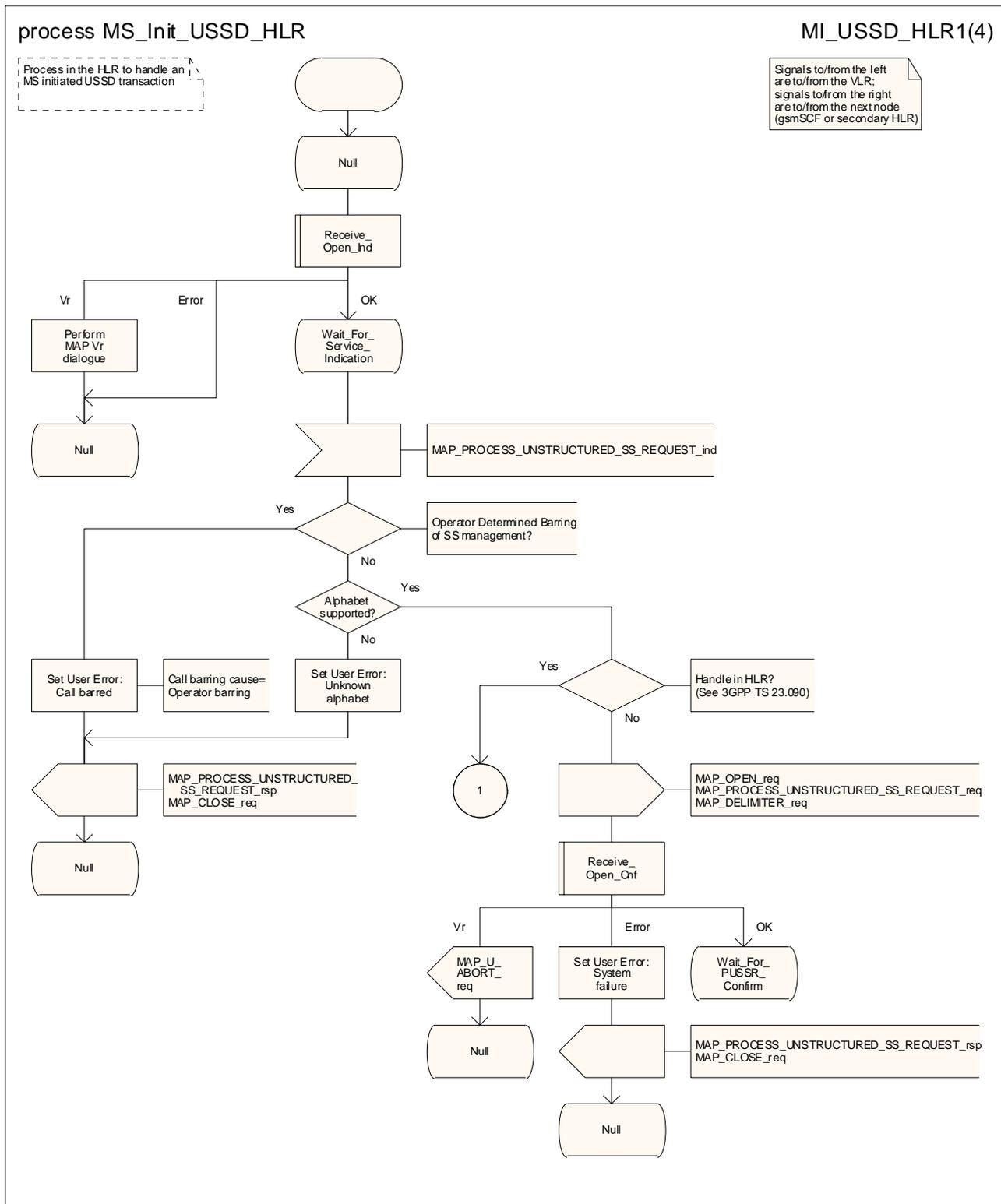
Figure 22.9.4/1 (sheet 1 of 4): Process MS\_Init\_USSD\_HLR
