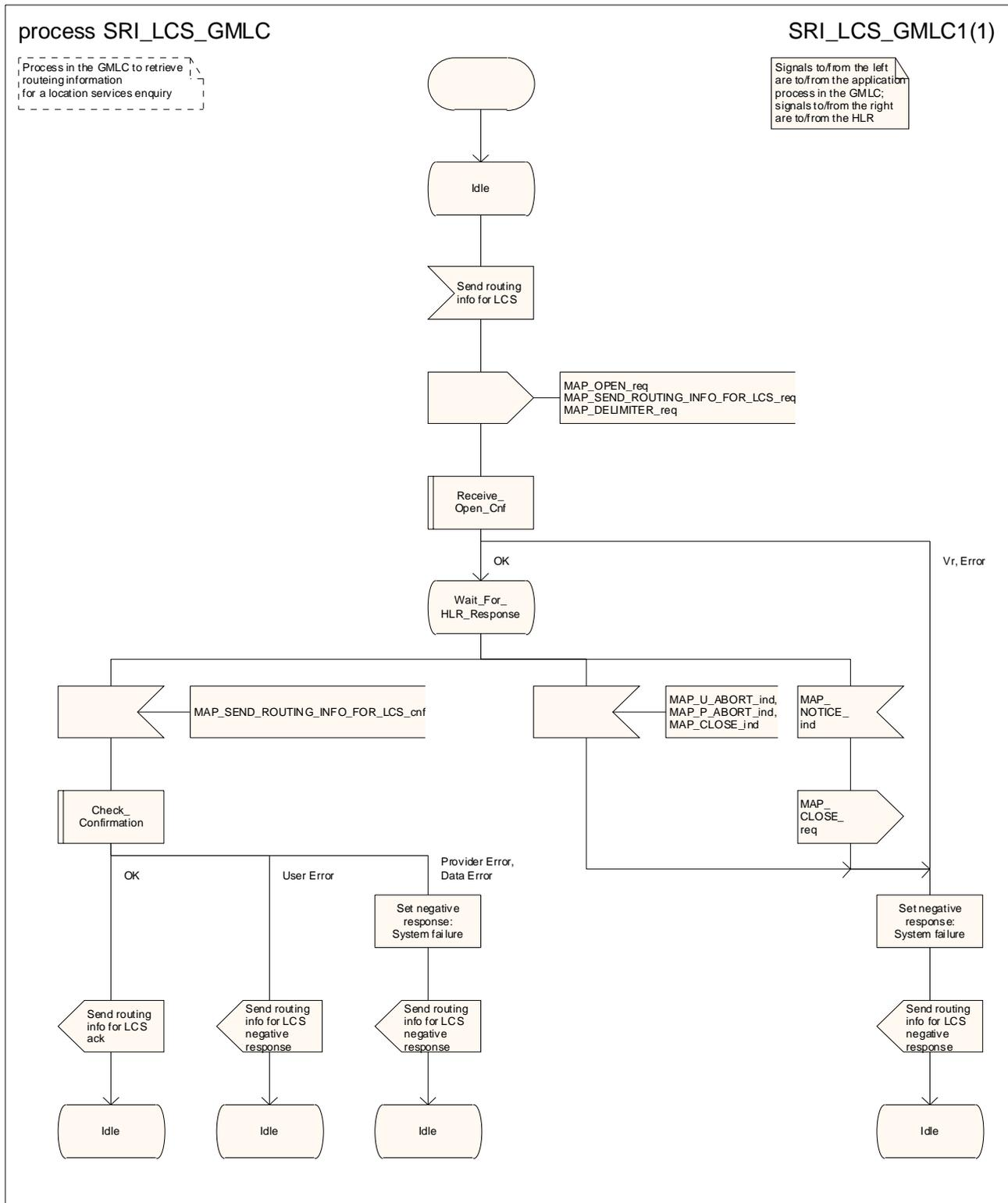
Figure 24B.1/2: Process SRI\_LCS\_GMLC
