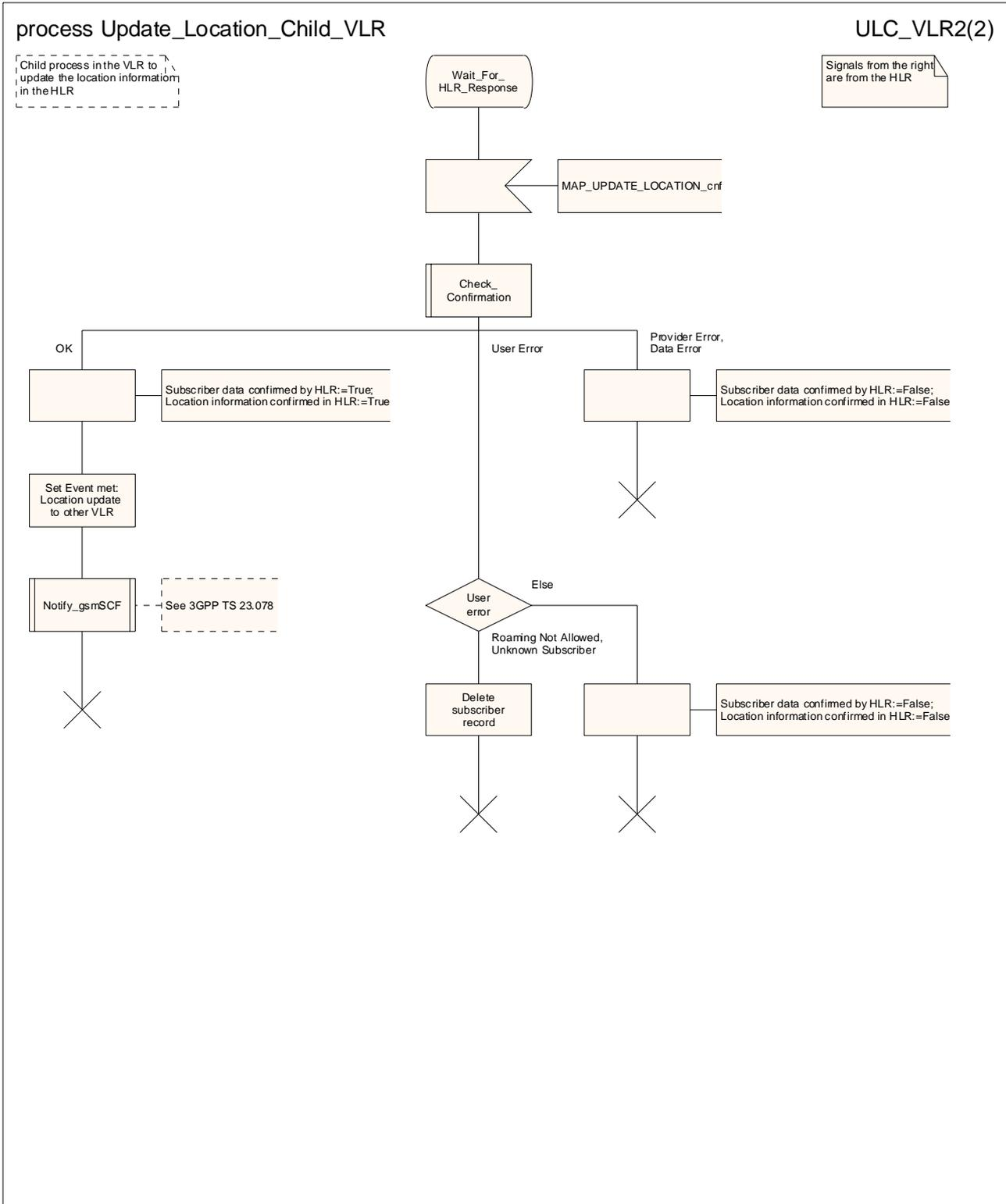
Figure 25.4/4 (sheet 2 of 2): Process Update\_Location\_Child\_VLR
