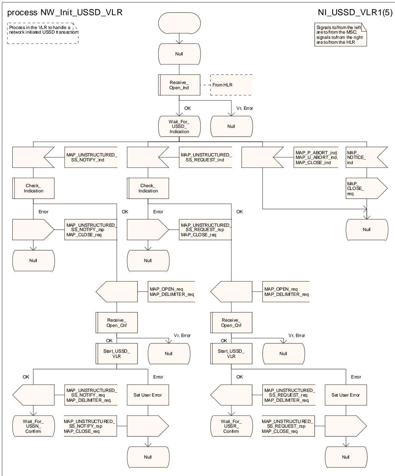
Figure 22.10.3/1 (sheet 1 of 5): Process NW\_Init\_USSD\_VLR
