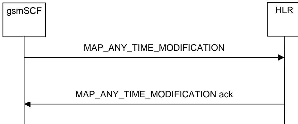
**Figure 24A.3/1: Message flow for any time modification**
