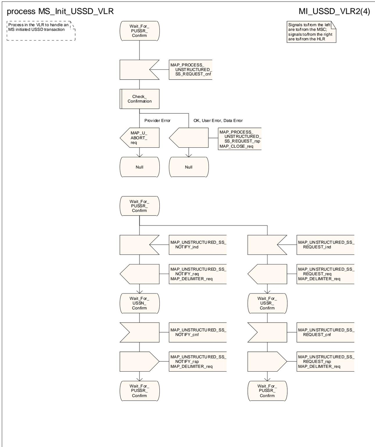
Figure 22.9.3/1 (sheet 2 of 4): Process MS\_Init\_USSD\_VLR
