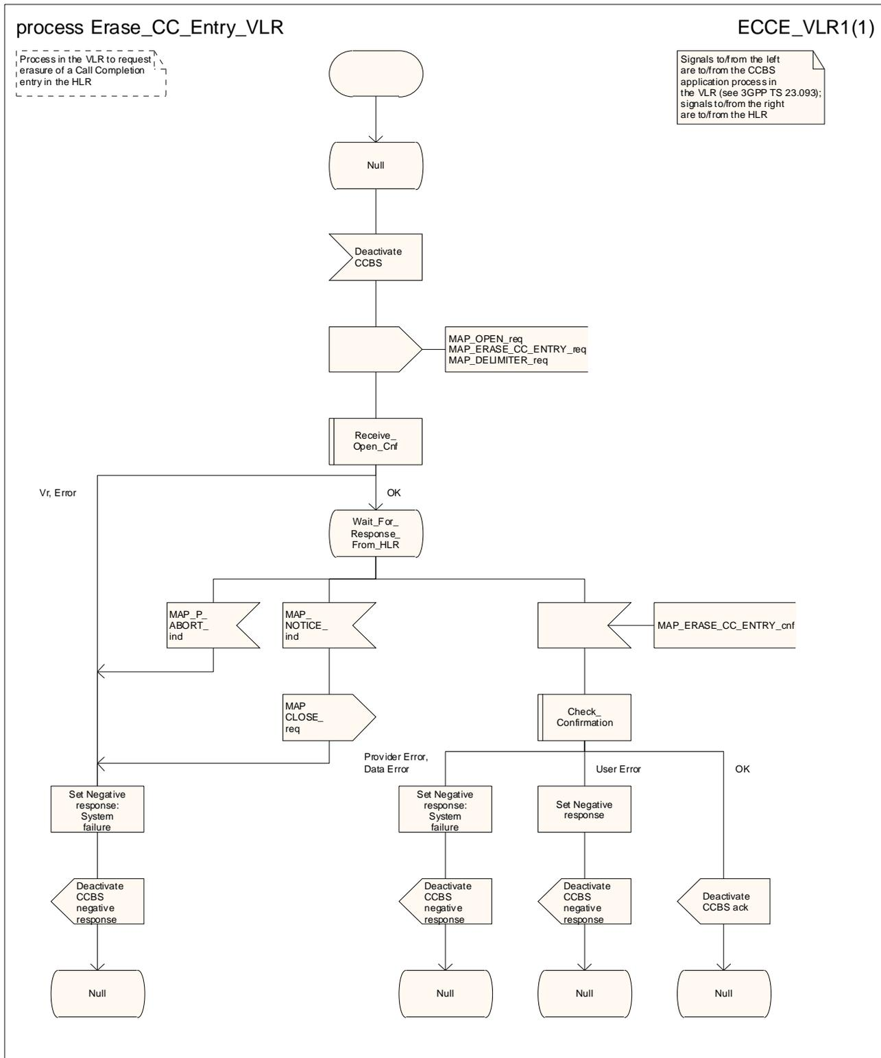
Figure 22.14.2/1: Process Erase\_CC\_Entry\_VLR
