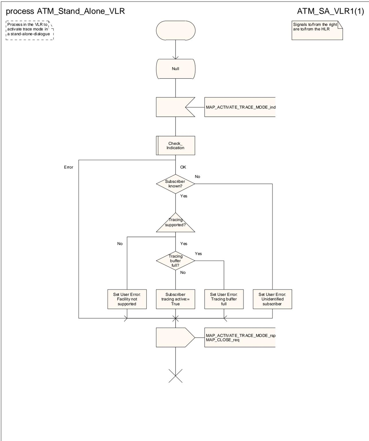
Figure 20.2/10: Process ATM\_Stand\_Alone\_VLR
