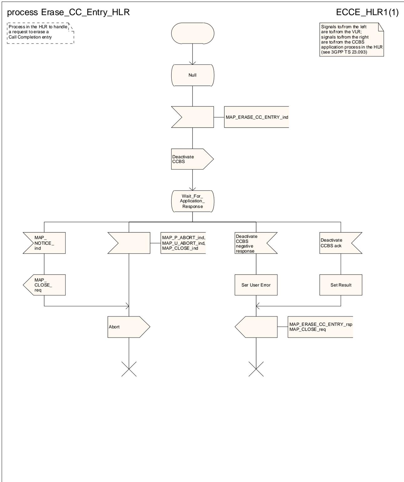
Figure 22.14.3/1: Process Erase\_CC\_Entry\_HLR
