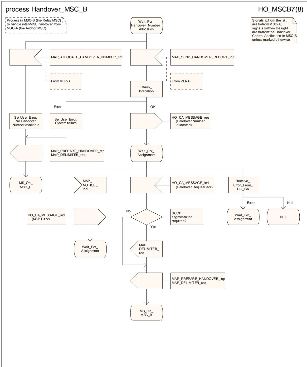
Figure 19.2/5 (sheet 7 of 8): Process HO\_MSC\_B
