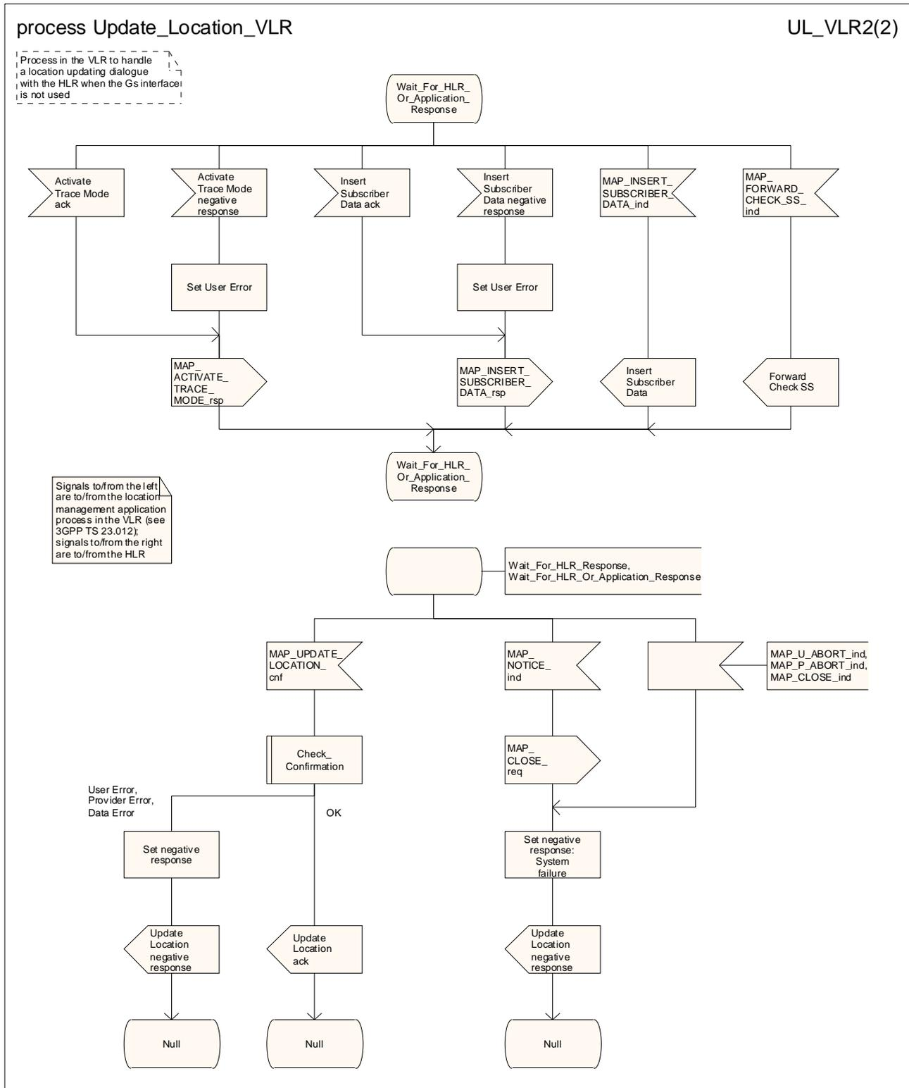
Figure 19.1.1/6 (sheet 2 of 2): Process Update\_Location\_VLR
