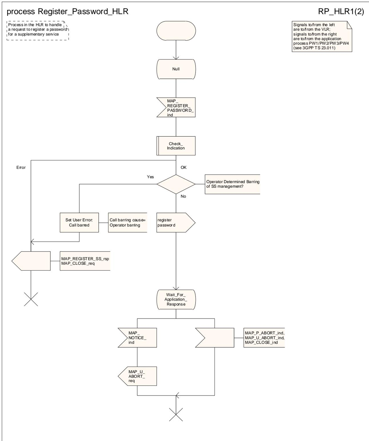
Figure 22.8.4/1 (sheet 1 of 2): Process Register\_PW\_HLR
