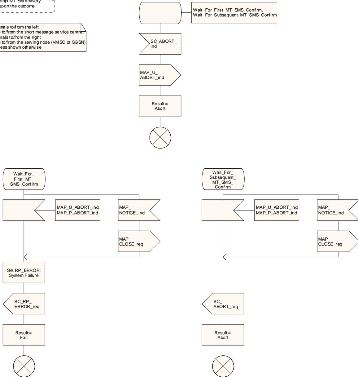
Figure 23.3/4 (sheet 7 of 8): Procedure MT\_SM\_Delivery\_Attempt\_GMSC
