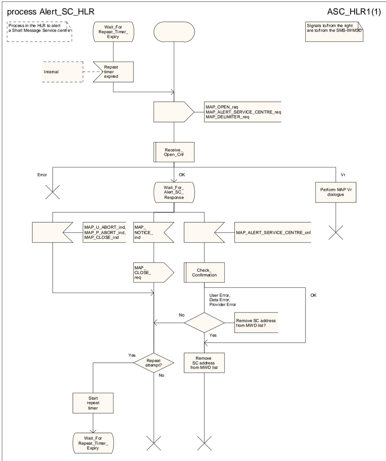
Figure 25.10/4: Process Alert\_SC\_HLR
