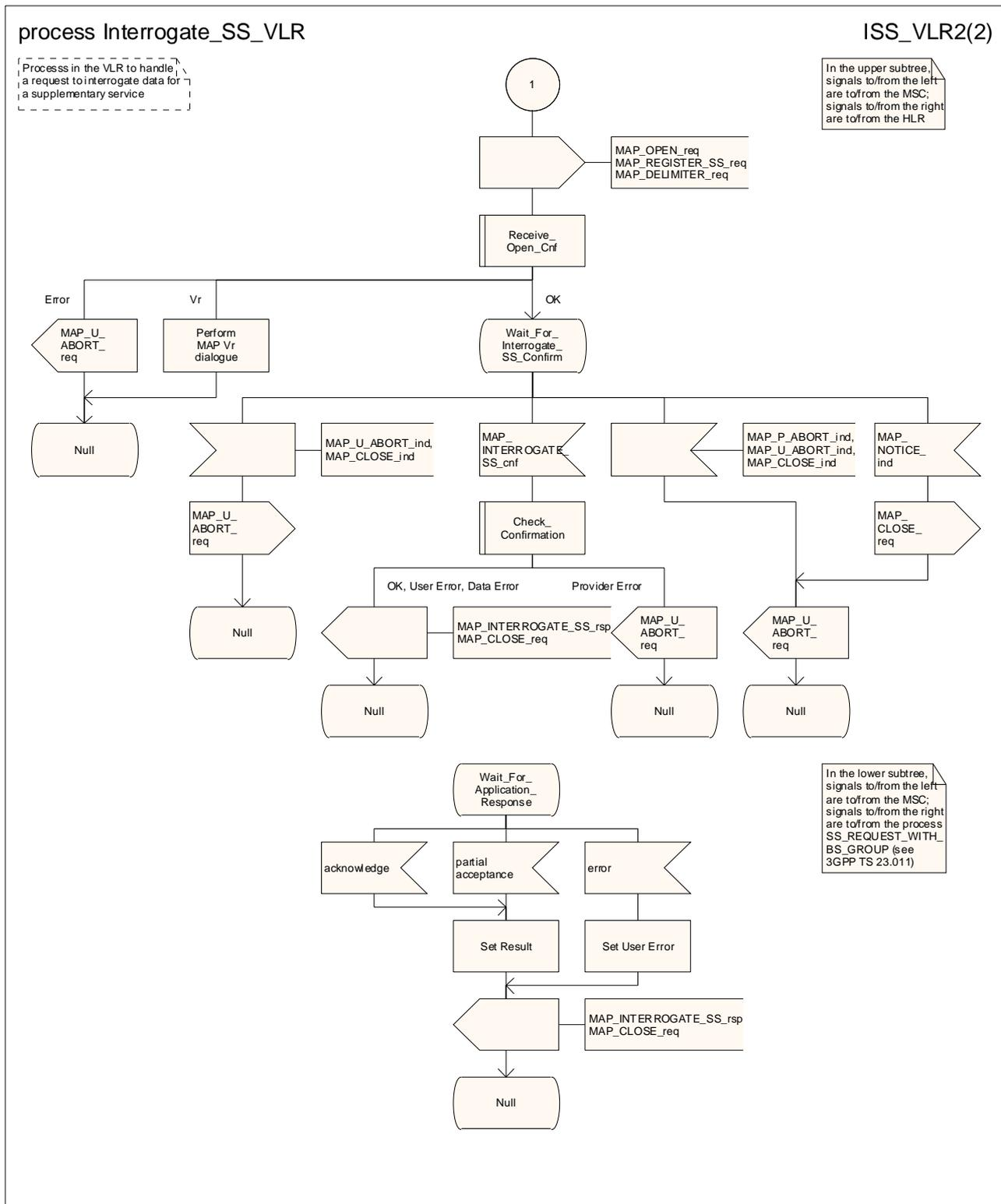
Figure 22.6.3/1 (sheet 2 of 2): Process Interrogate\_SS\_VLR
