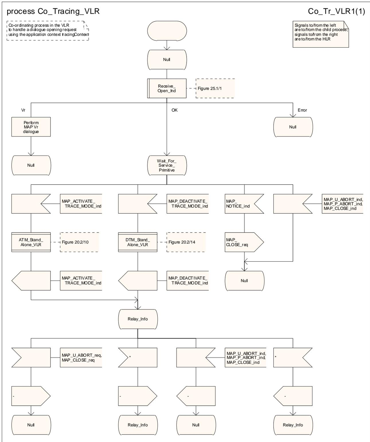
Figure 20.1/1: Process Co\_Tracing\_VLR
