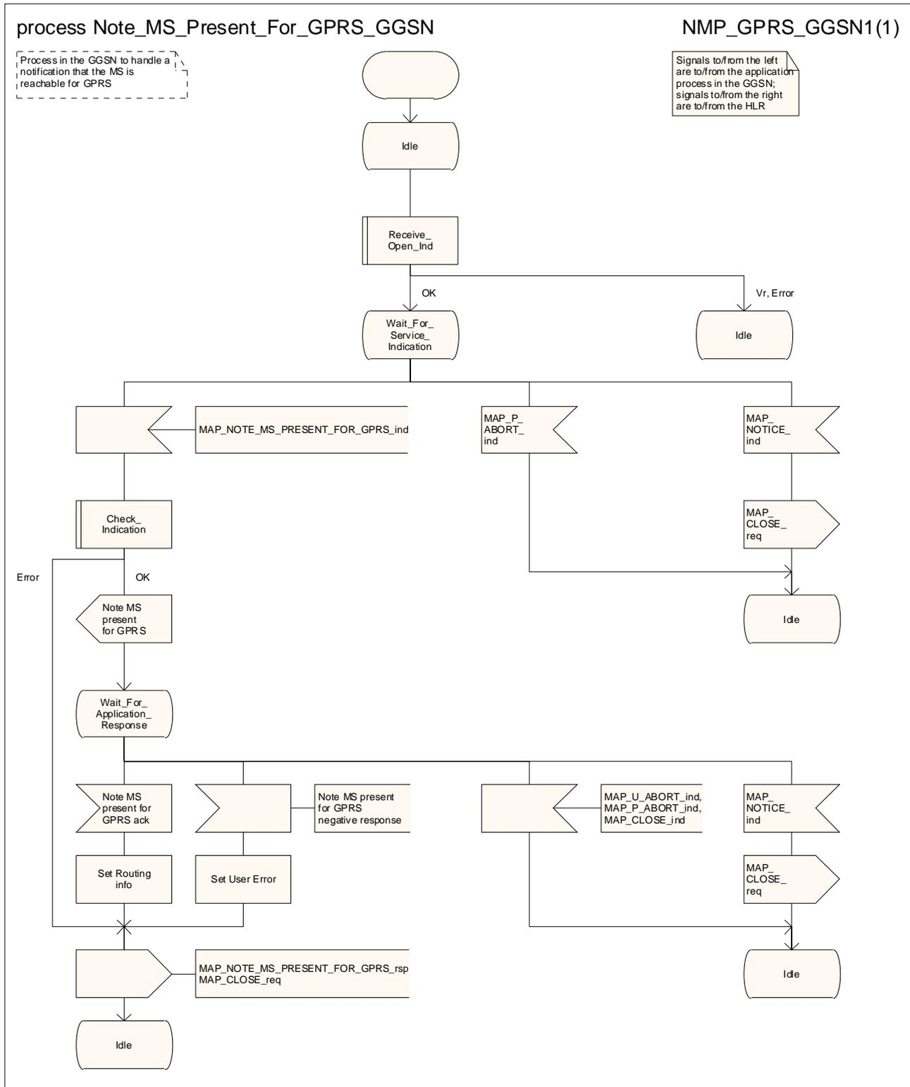
Figure 24.3/2: Process Note\_MS\_Present\_For\_GPRS\_GGSN
