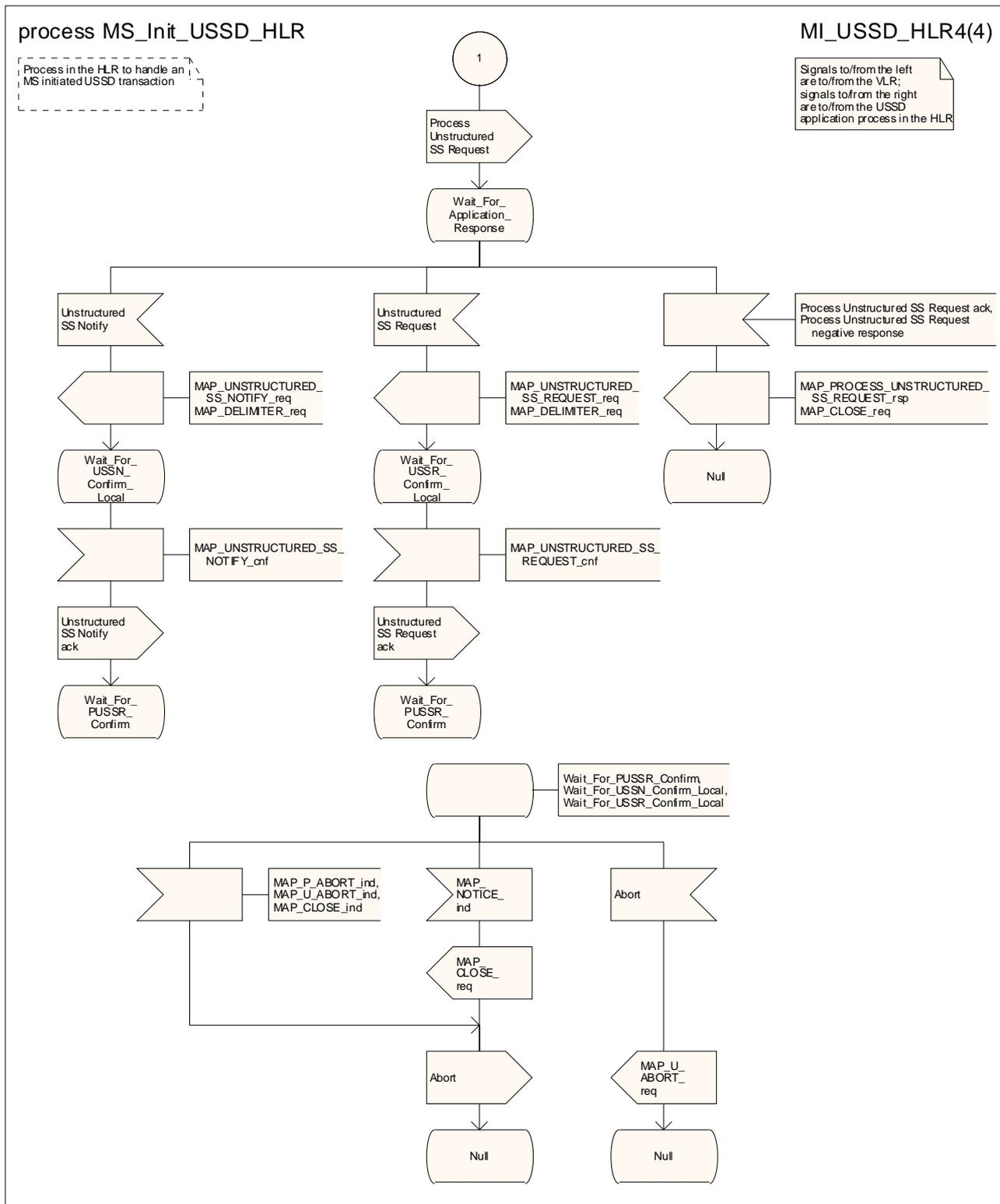
Figure 22.9.4/1 (sheet 4 of 4): Process MS\_Init\_USSD\_HLR
