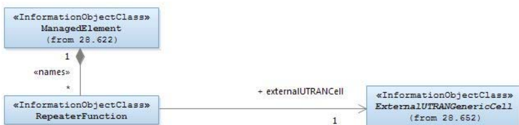
Figure 4.2.1.4: Repeater object Containment/Naming and Association diagram
