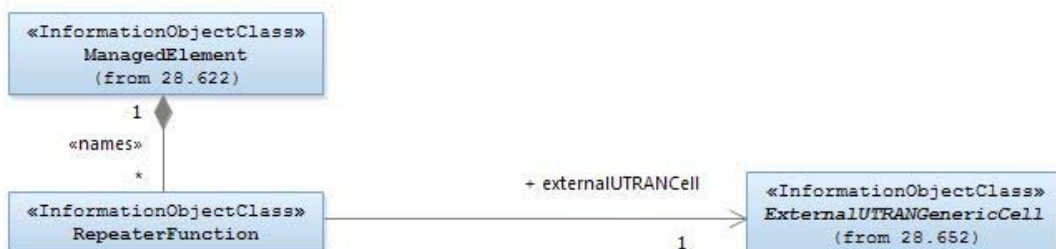
Figure 4.2.1.4: Repeater object Containment/Naming and Association diagram
