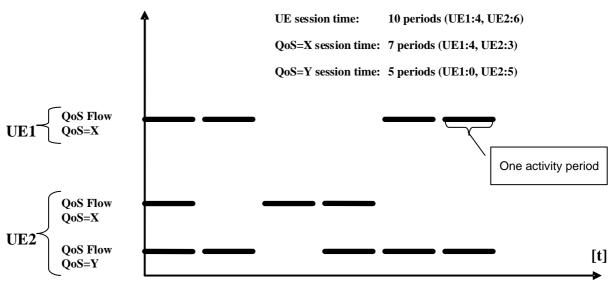
Hence a measurement QoS flow Retainability on UE level is defined (R2) to provide a measurement for the overall QoS flow Retainability.
