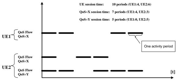
Hence a measurement QoS flow Retainability on UE level is defined (R2) to provide a measurement for the overall QoS flow Retainability.
