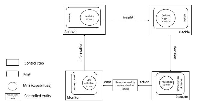
Figure 4.3.1: Overview of closed control loop information flows
