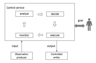
Figure 4.2.4.1: Closed control loop entities
