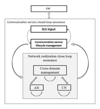
Figure 4.2.1.1: Communication service closed control loop assurance
