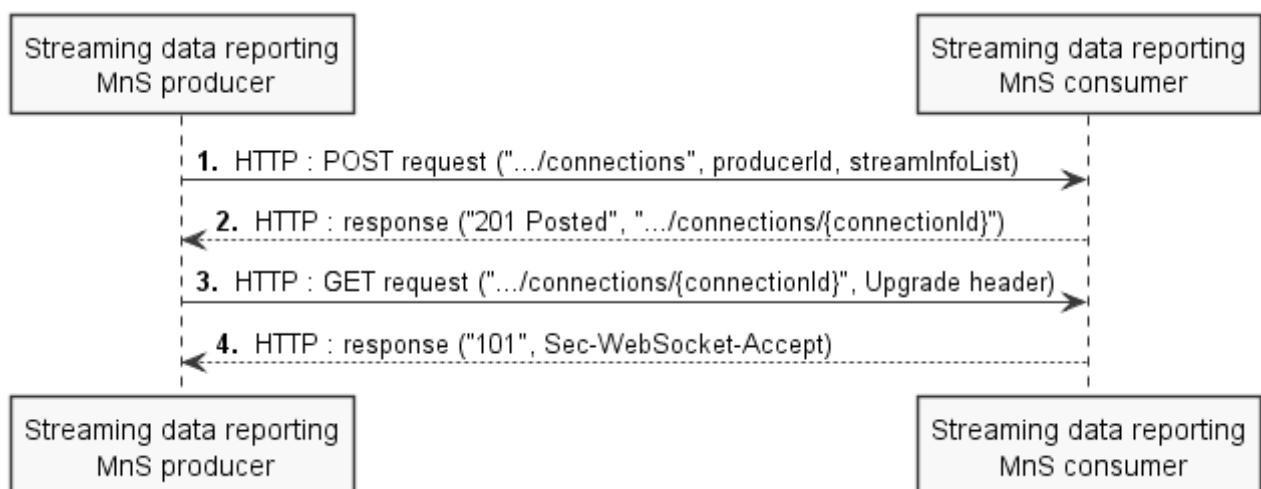
Figure 12.5.1.1.2-1: Message flow for establishing a streaming connection
