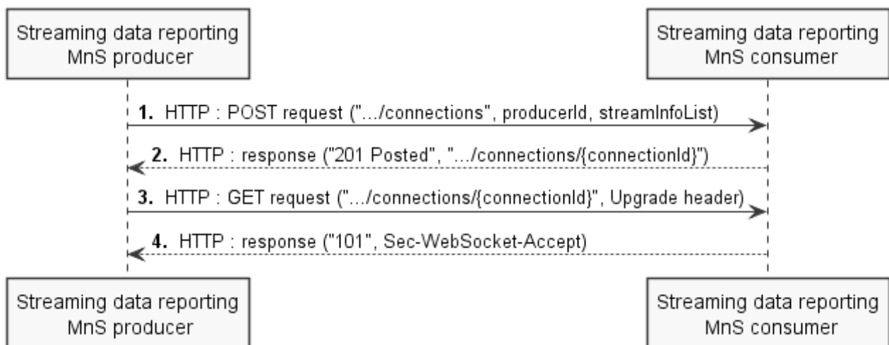
Figure 12.5.1.1.2-1: Message flow for establishing a streaming connection
