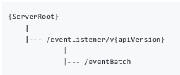
Figure 12.2.2.3.1-1: Resource URI structure of the fault supervision data report MnS for integration with ONAP VES Event Listener 7.1.1 (Resource structure section) [45]
