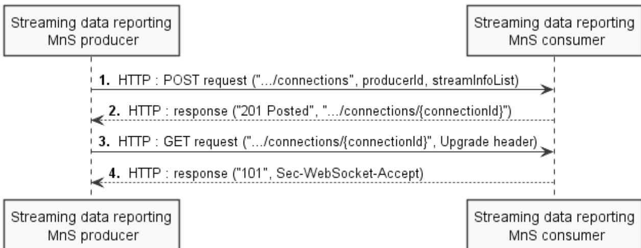
Figure 12.5.1.1.2-1: Message flow for establishing a streaming connection
