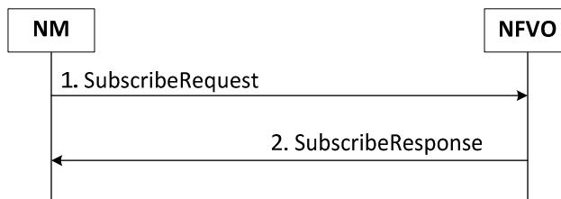
Figure 4.5.7-1: Subscribing to NSD change notifications through Os-Ma-nfvo
