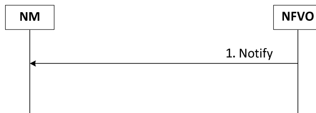
Figure 4.4.9-1: Procedure for the Notify operation
