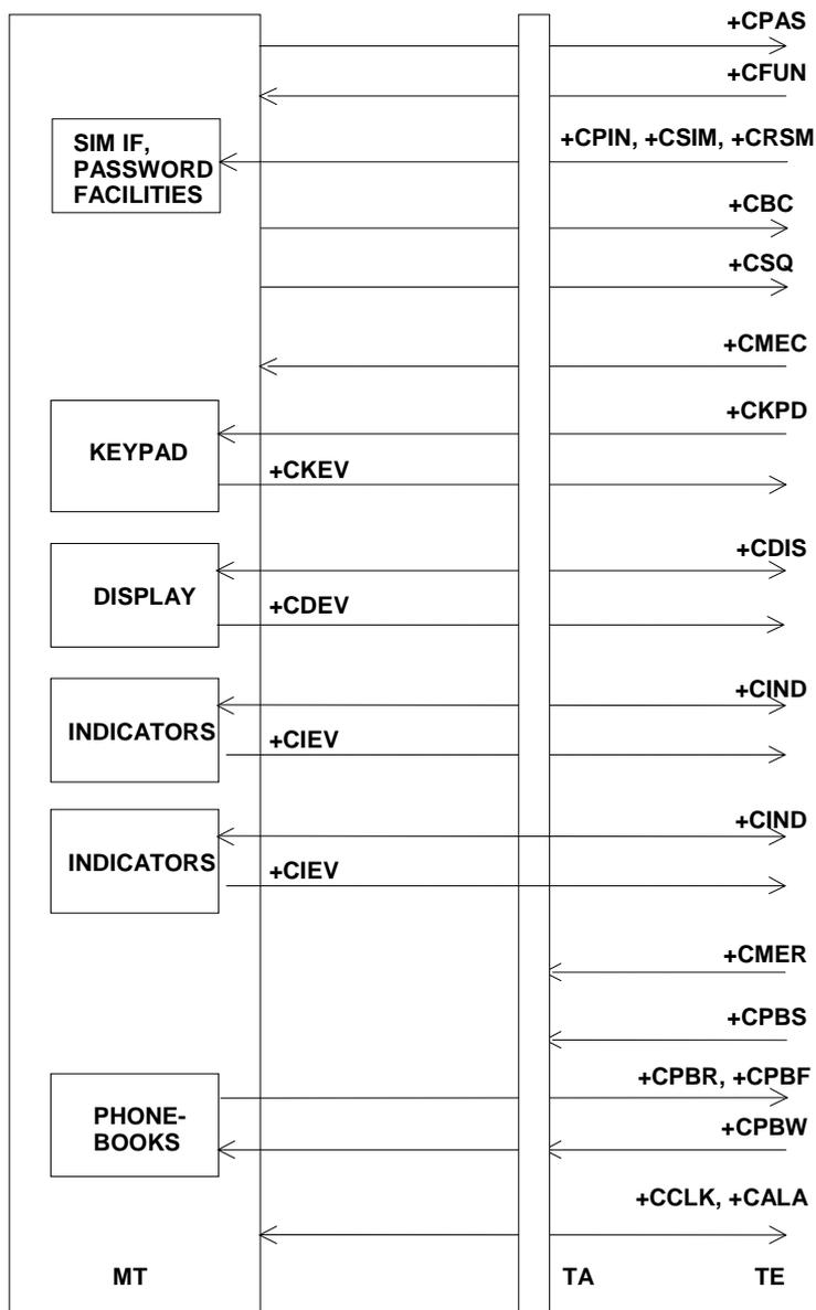
Figure 7: Mobile termination control and status commands
