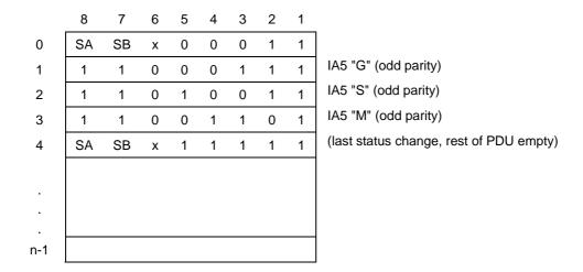
Figure 2a: Single-link RLP and multi-link RLP with status octet transfer in PDU
