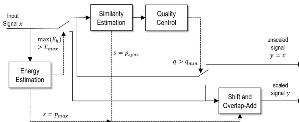
**Figure 4: Signal-based adaptation based on signal characteristics**
