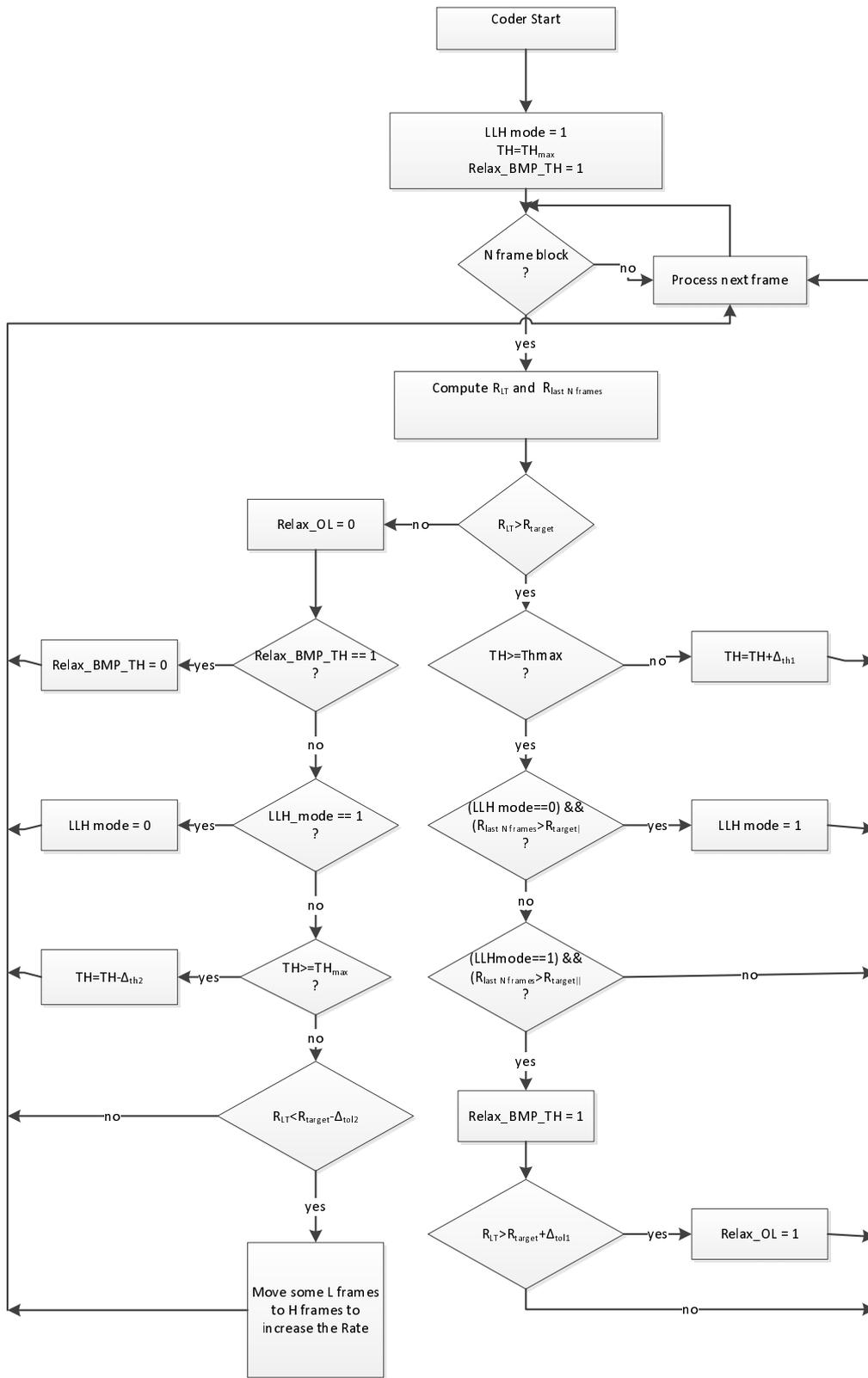
Figure 43: Average rate control in Variable Bit-Rate Coding
