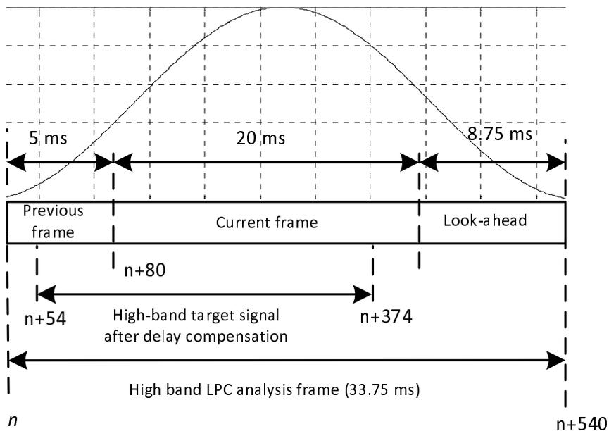
**Figure 47: SWB Highband target signal buffers**
