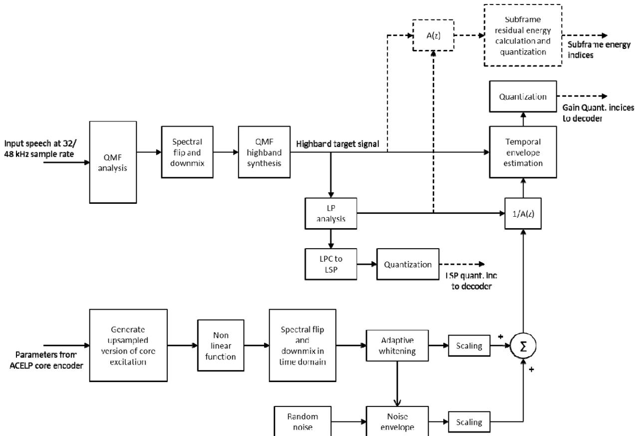
Figure 44: Time Domain Bandwidth Extension Encoder. Blocks in dashed lines are activated only at higher bit rates (24.4 kb/s or higher)
