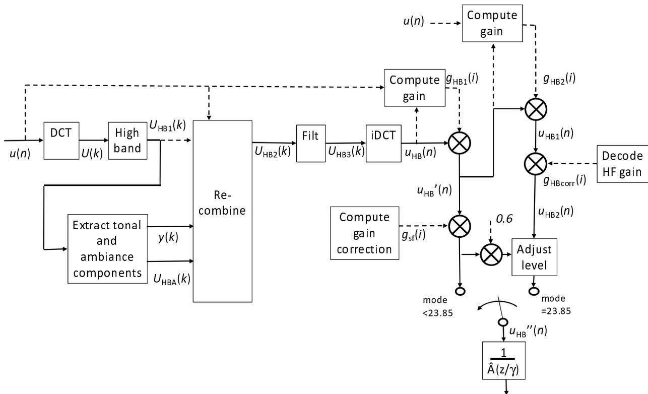
Figure 113: High-frequency band generation in AMR-WB IO modes
