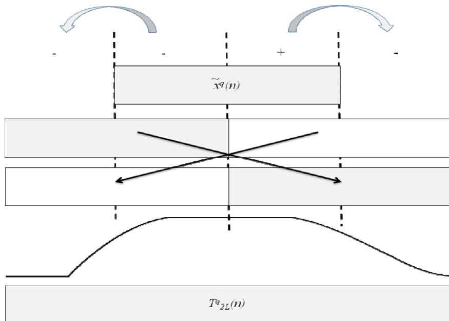
**Figure 109: Unfolding and windowing with ALDO window.**
