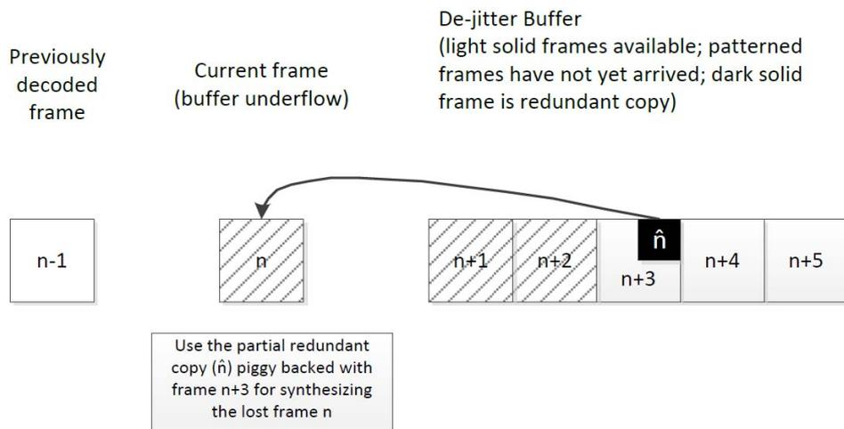
**Figure 87 : Concept of partial redundancy in channel aware mode**
