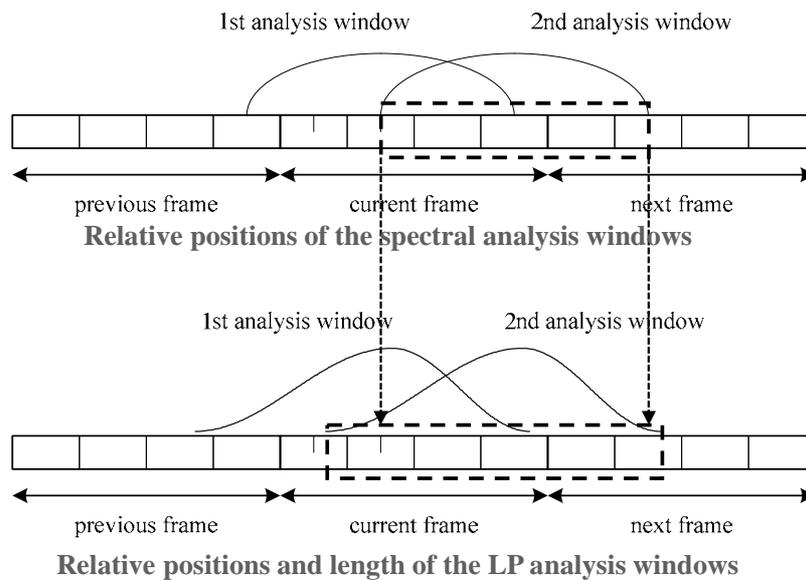
**Figure 19: LSF weighting computation with FFT spectrum**
