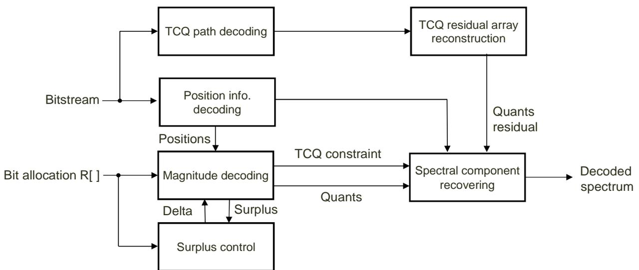
**Figure 97: Block diagram for LSB TCQ decoding**
