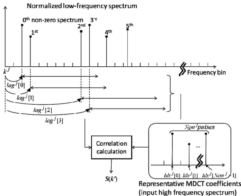
**Figure 76: Conceptual block diagram of the matching process**
