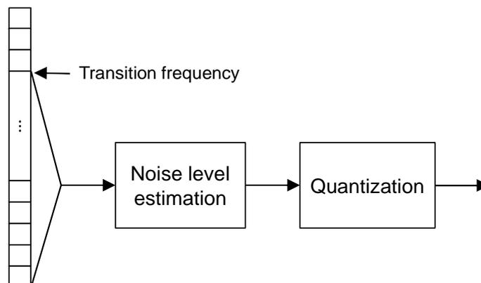
Figure 81: Noise level estimation done below the transition frequency
