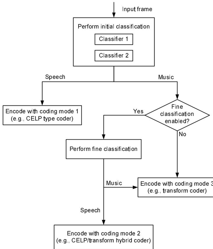
**Figure 18 : Multiple coding mode signal classification**
