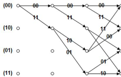
Figure 75: Trellis structure for the 4 states TCQ
