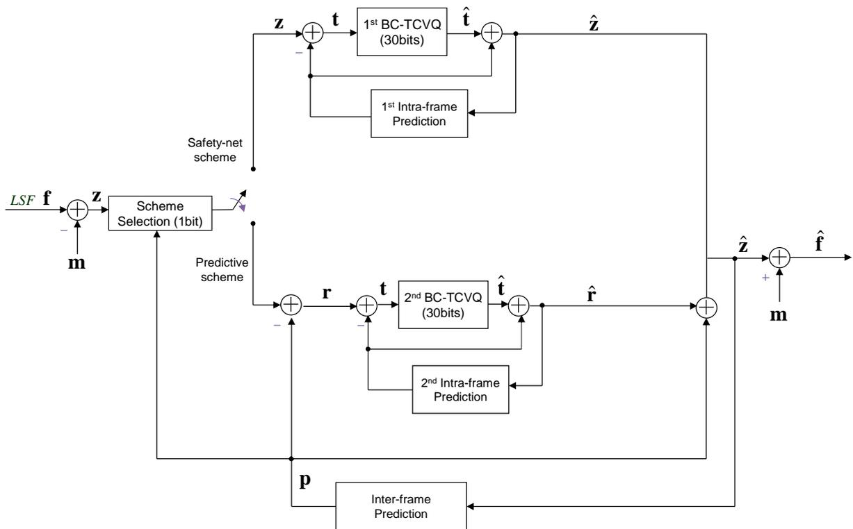
Figure 23: Block diagram of the predictive BC-TCVQ with safety-net for an encoding rate of 31bits/frame
