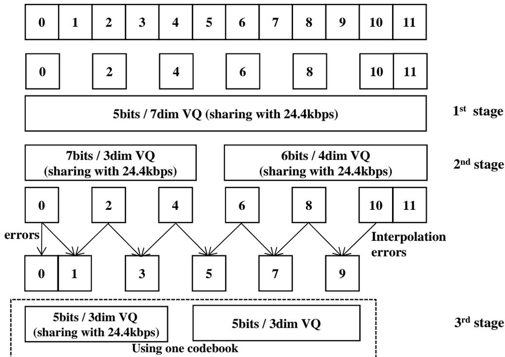
**Figure 83: VQ for HQ generic mode at 32kbps**
