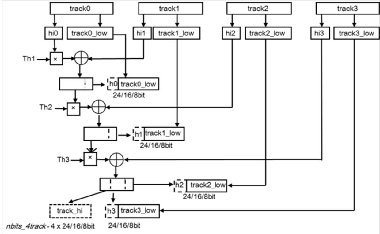
**Figure 28: Schematic diagram of 4-track joint coding**
