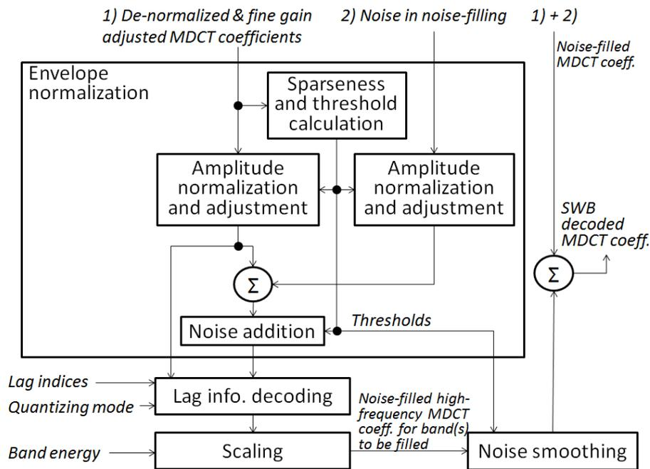
**Figure 98: Block diagram of the Normal mode PFSC decoder**
