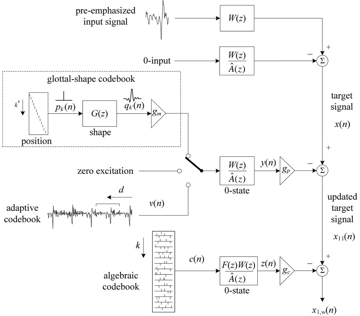
Figure 36: Schematic diagram of the excitation coding in TC mode
