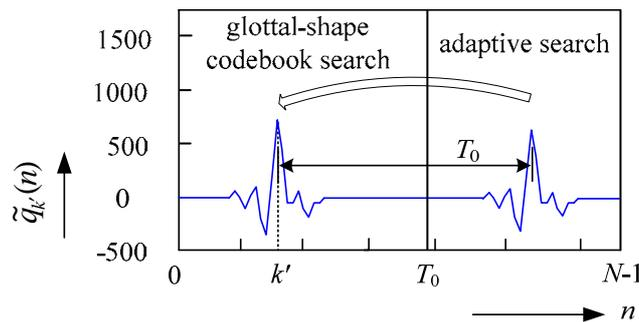
**Figure 37: Glottal-shape codevector with two impulses construction**
