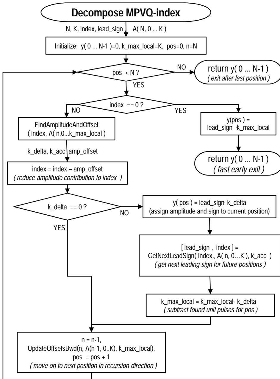
Figure 108: Detailed MPVQ-de-indexing
