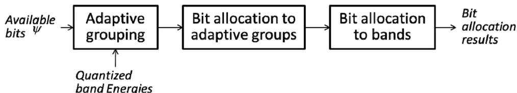
**Figure 77: Overview of the Adaptive bit allocation scheme**
