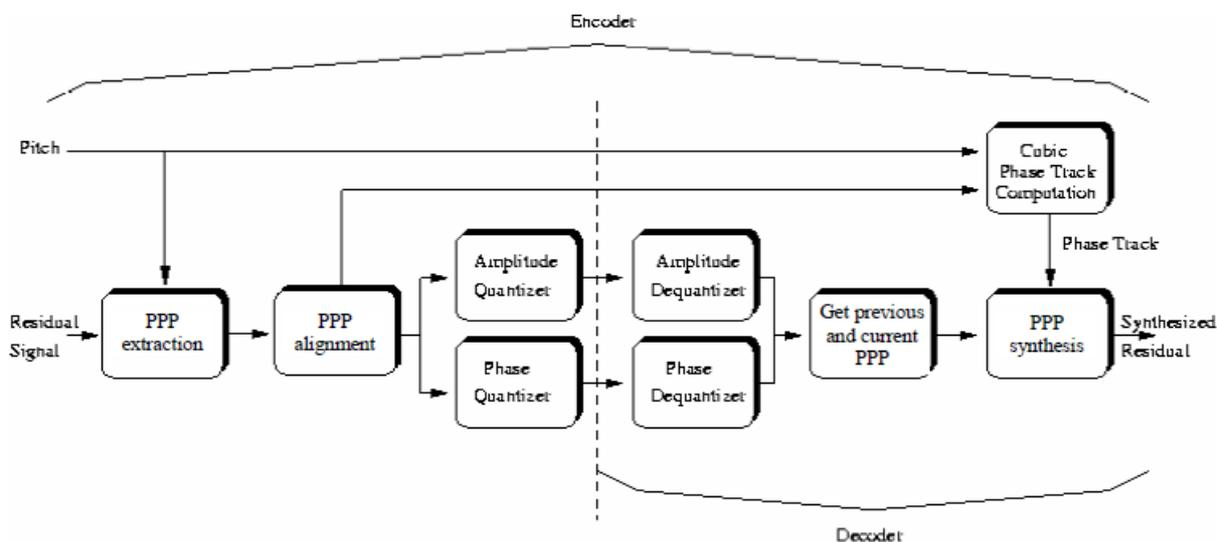
**Figure 42: Block diagram of PPP coding scheme [20]**
