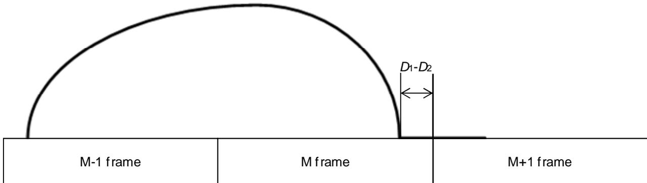
**Figure 51: Windowing of the input high-pass filtered signal**
