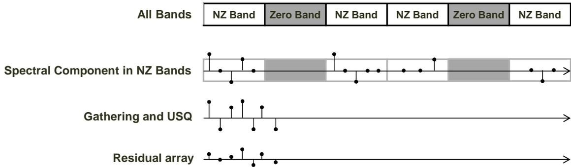
Figure 74: Concept for constructing the residual array
