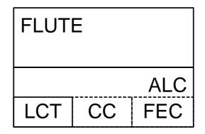
Figure 10: Building block structure of FLUTE
