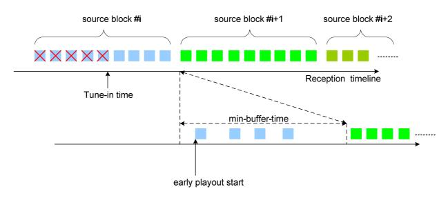
Figure G.2: Early play out of interleaved media data of a FEC protected MBMS service
