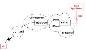
Figure 3c: MBMS network architecture model for GCS delivery
