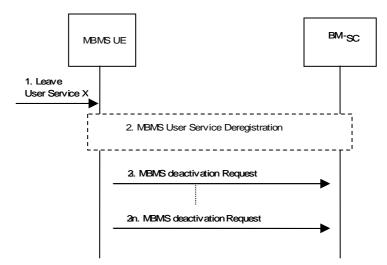
Figure 7: Termination of an MBMS user service
