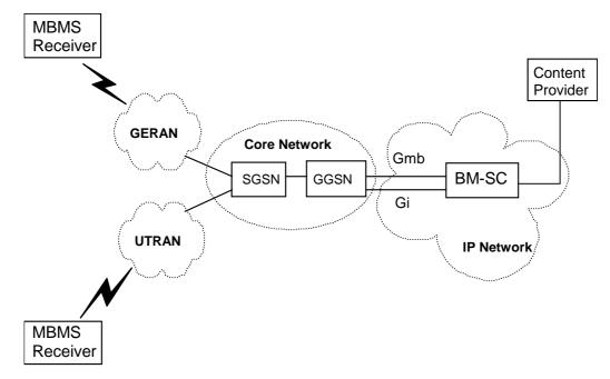
Figure 3a: MBMS network architecture model for GPRS
