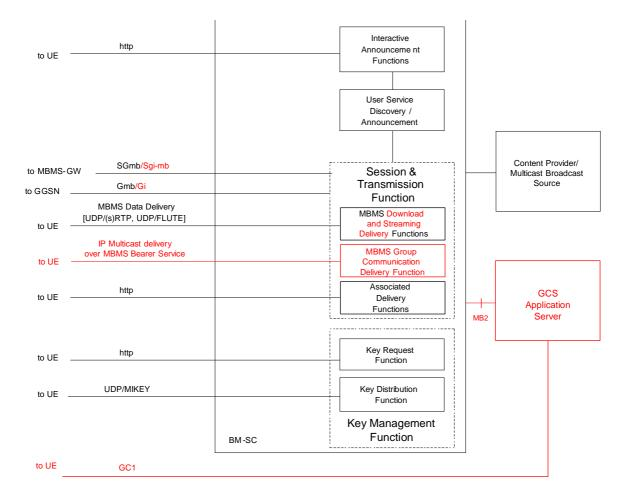
Figure 4: BM-SC sub-functional structure
