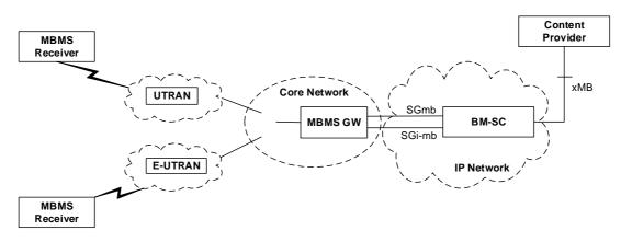
Figure 3b: MBMS network architecture model for EPS
