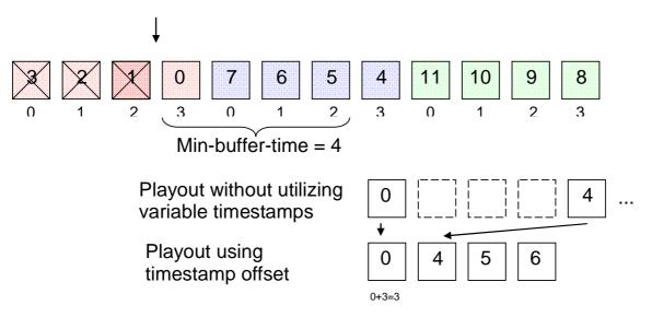
Figure G.1: Early tune-in using variable timestamps
