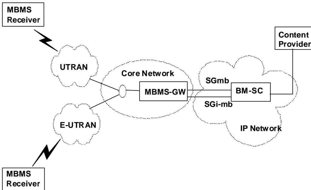
**Figure 3b: MBMS network architecture model for EPS**
