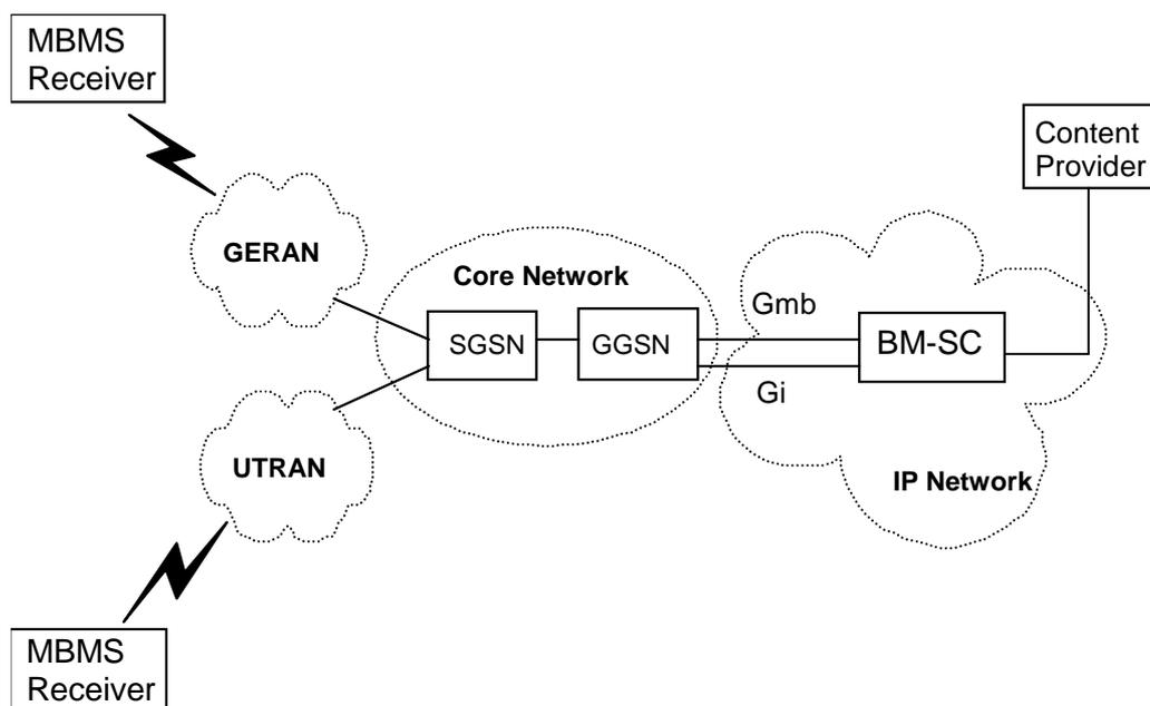
Figure 3: MBMS network architecture model for GPRS
