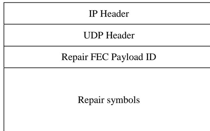
**Figure 13: Payload structure for FEC repair packets**
