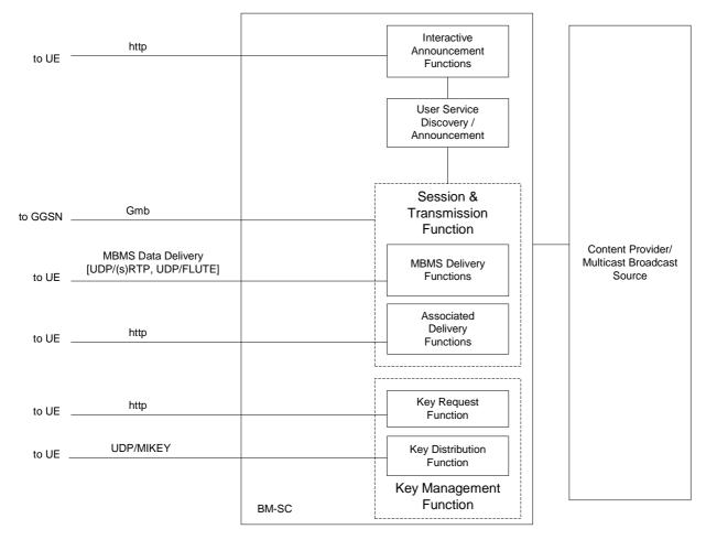
Figure 4: BM-SC sub-functional structure
