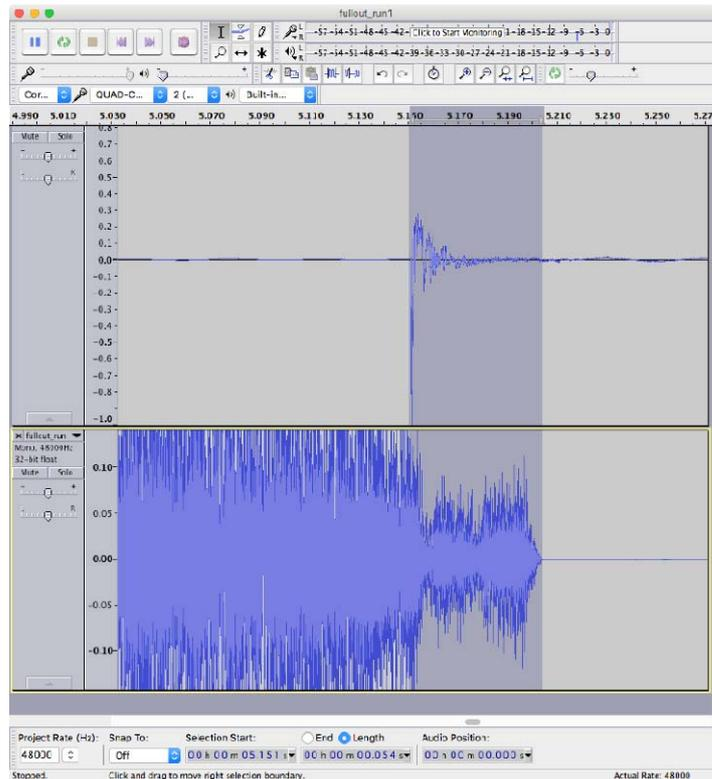
**Figure 5: Motion-to-sound (tM2S) latency measurement**
