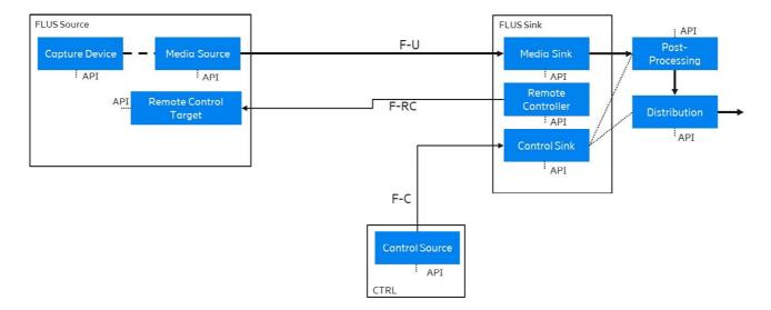
Figure A.2.3-1: Deployment with a Remote Controller co-located with a Control Sink sub-function
