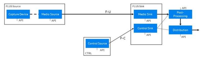
Figure A.1.3-1: Deployment with minimal FLUS sub-functions
