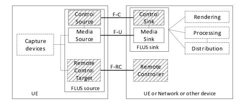
Figure 4.2-2: Sub-functions of FLUS
