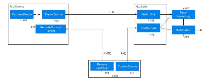
Figure A.2.2-1: Deployment with stand-alone Control Source and Remote Controller sub-functions
