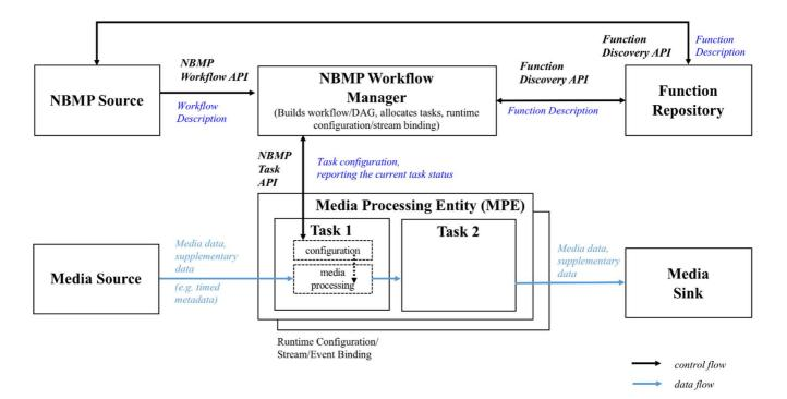
Figure X.1 – NBMP reference architecture
