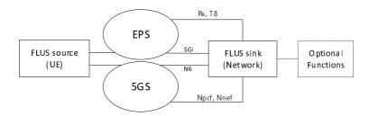
Figure 4.2-4a: Architecture for Live Uplink Streaming
