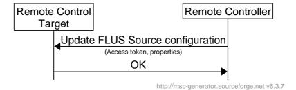
Figure 5.3.2.14-1: Remote FLUS Source Configuration update
