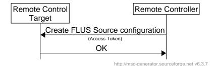
Figure 5.3.2.12-1: Remote FLUS Source configuration creation
