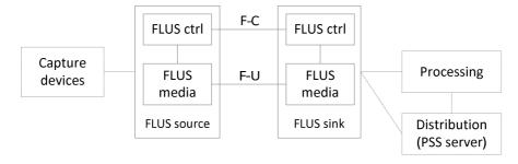
Figure 4.2-4b: Uplink streaming for PSS
