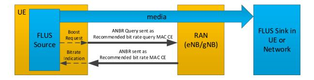
Figure 4.6.2-1 RAN signaling based uplink assistance in the FLUS system
