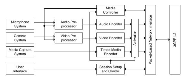
Figure 4.3-2: Functional components of a FLUS source for uplink media transmission
