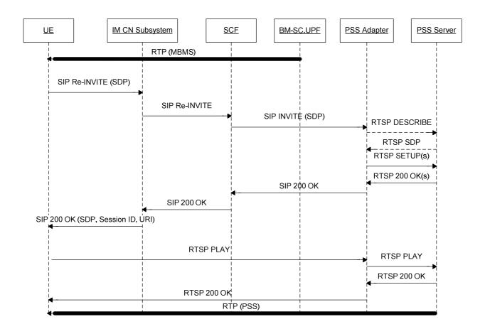
Figure 18: IMS Hybrid PSS-MBMS-to-PSS content switching
