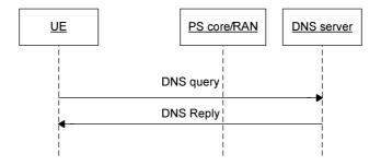
Figure 5: Service Provider Discovery with DNS
