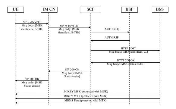
Figure 25: SIP based MBMS MSK request
