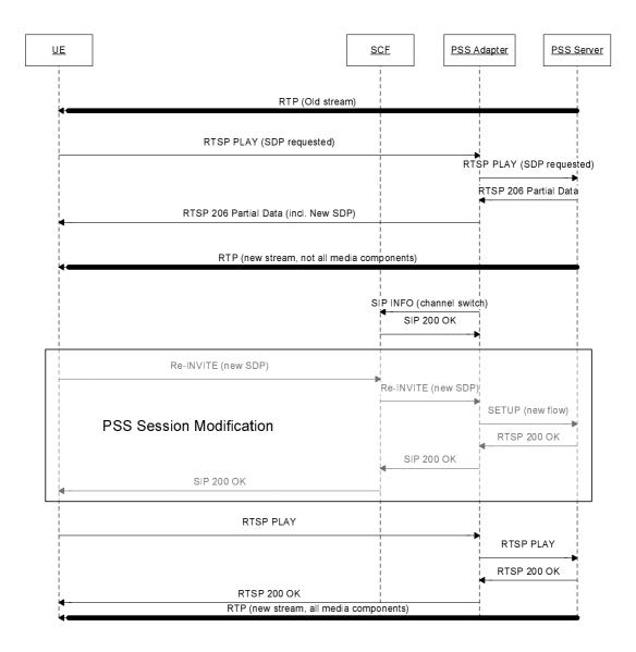
Figure 13: IMS PSS Content switching without available SDP, change of media component and/or bandwidth
