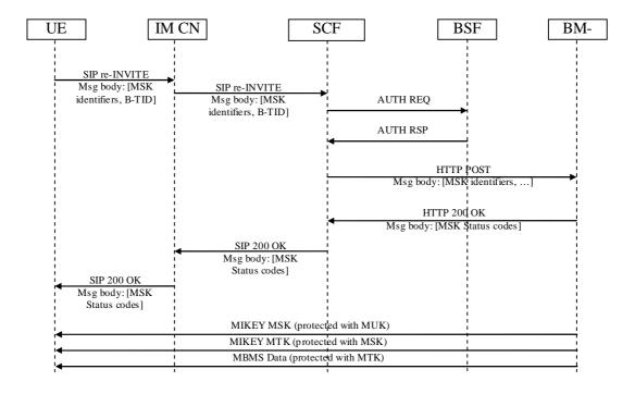
Figure 25: SIP based MBMS MSK request
