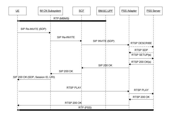
Figure 18: IMS Hybrid PSS-MBMS-to-PSS content switching
