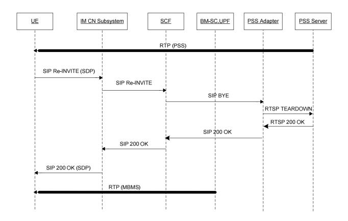
Figure 19: IMS PSS-to-MBMS content switching
