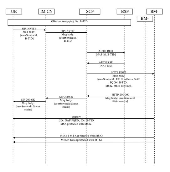
Figure 24: SIP based MBMS User Service Registration
