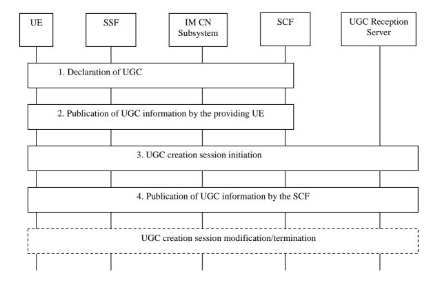
Figure 30: IMS Based UGC Provision Procedures
