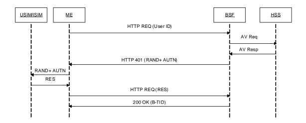
Figure 21: GBA/GAA Bootstrapping procedure
