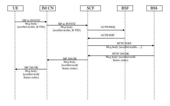
Figure 24a: SIP based MBMS User Service De-registration
