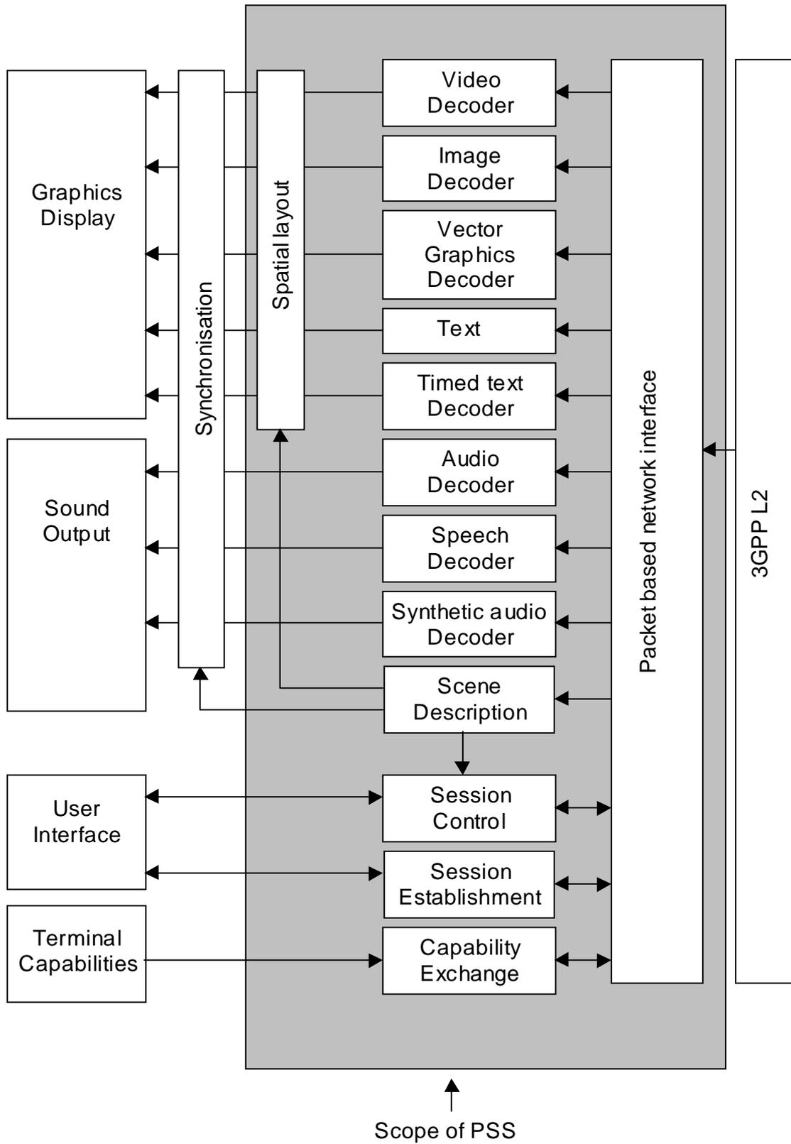
Figure 1: Functional components of a PSS client
