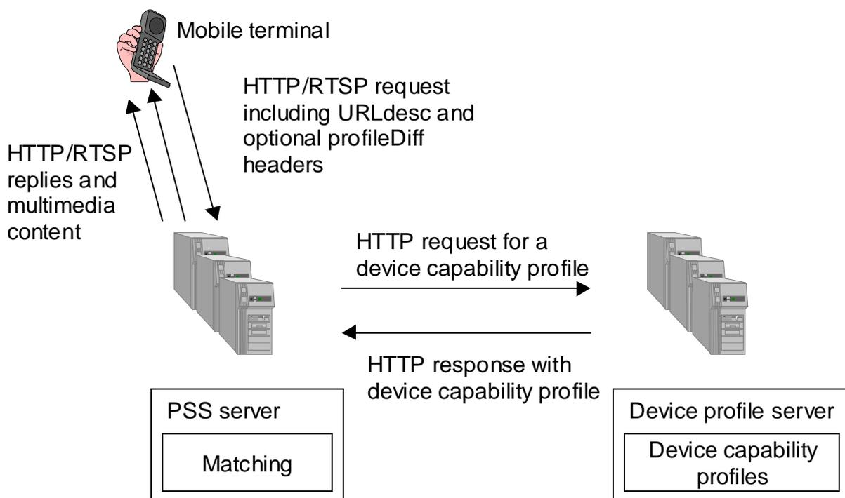
**Figure A.1: Functional components in PSS capability exchange**
