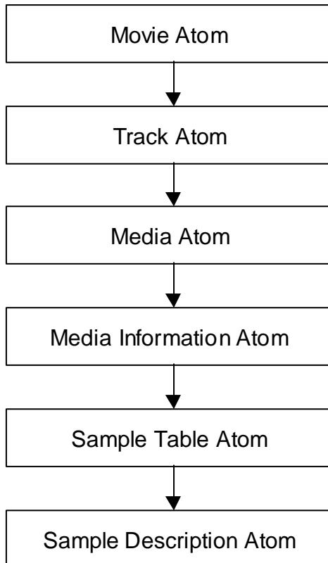
**Figure D.1: MP4 Atom Structure Hierarchy**
