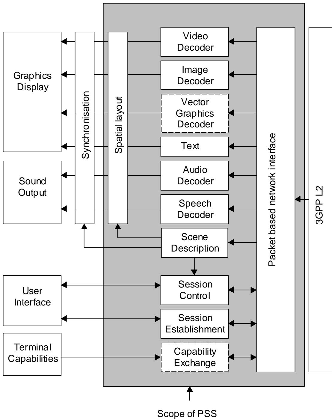
**Figure 1: Functional components of a PSS client**
